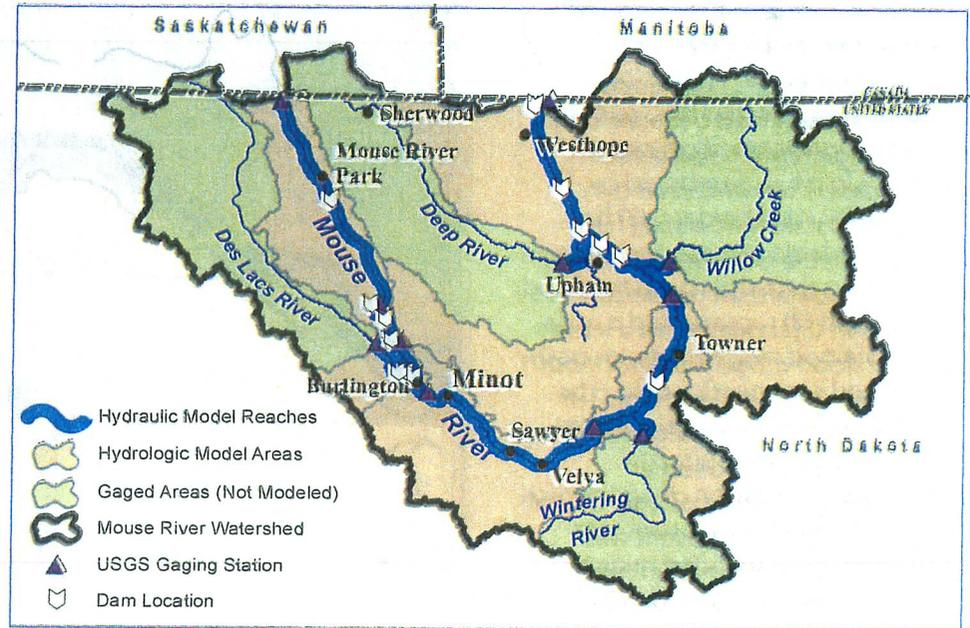
Figure 2: The hydrologic model calculated runoff from ungaged areas of the Mouse River watershed, and the hydraulic model simulated flow in the Mouse River and portions of its four major tributaries.
