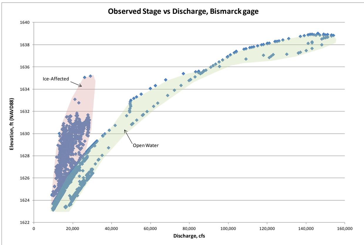
Figure 2. Stage-Discharge Flow Regimes for Open Water and Ice-Affected Flows, Bismarck, ND
