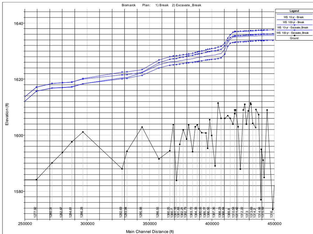
Figure 28. Existing and Alternative 3 Ice Jam Breakup profiles for 10% and 1% ACE events.
