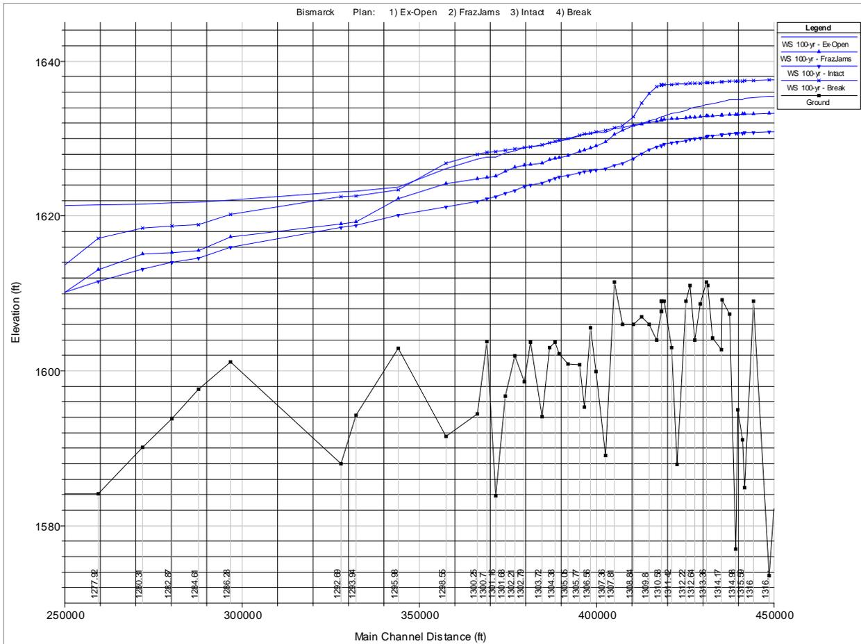
Figure 10. Comparison of 1% ACE water surface profiles for open water and ice-affected profiles
