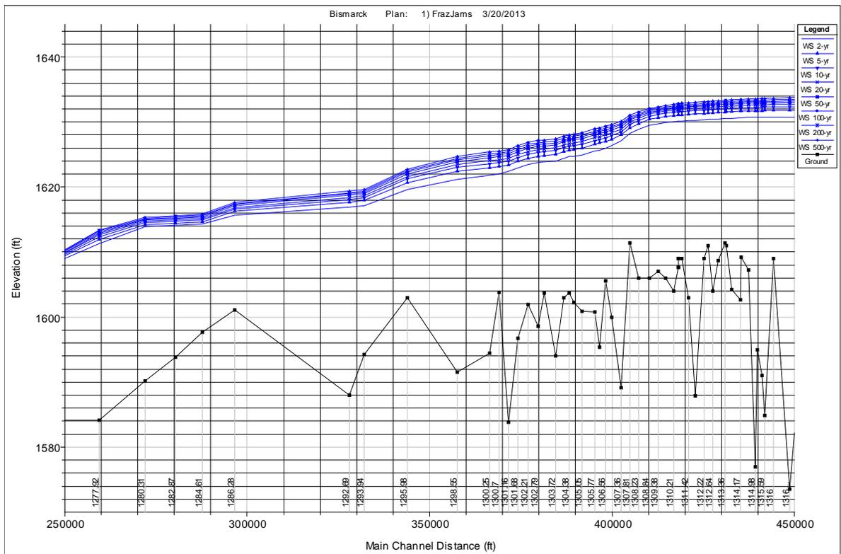
Figure 7. Existing Ice-Affected Freezeup Flow Profiles, Missouri River
