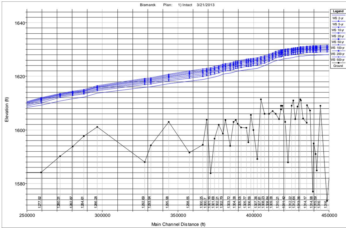
Figure 8. Ice-Affected Intact Ice Cover Profiles, Missouri River
