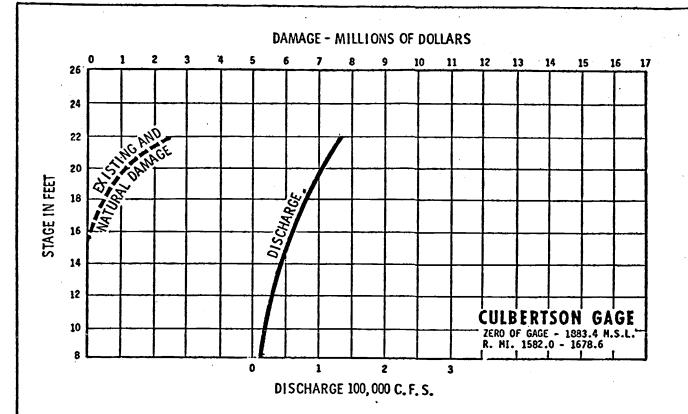
NOTE: DAMAGE CURVES ARE BASED ON ESTIMATED 1975 AVERAGE ANNUAL DAMAGES PER CROP YEAR. MISSOURI RIVER STAGE – DISCHARGE – DAMAGE CURVES RURAL AREAS
