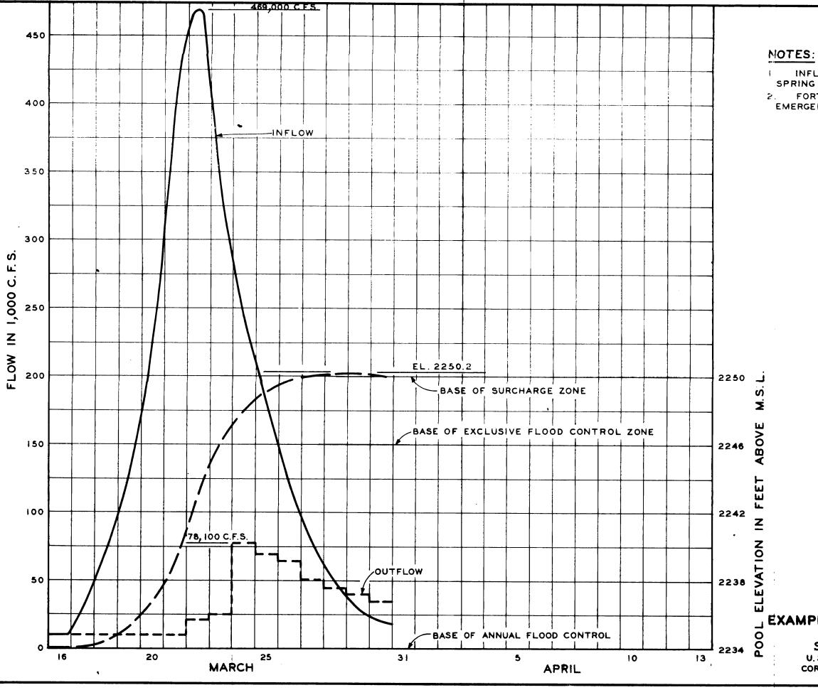
MISSOURI RIVER FORT PECK LAKE, MONTANA LEXAMPLE OF EMERGENCY REGULATION EARLY SPRING FLOOD OF SPILLWAY DESIGN MAGNITUDE U.S. ARMY ENGINEER DISTRICT, OMAHA CORPS OF ENGINEERS OMAHA, NEBRASKA OCT 1972 RES. REG. MANUAL PLATE 43
