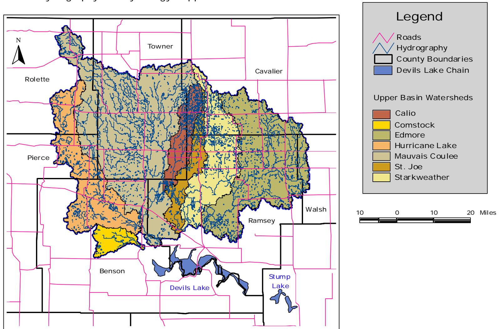
Figure 7. Physiography and hydrology of the Upper Basin of Devils Lake. The seven major watersheds are shown, along with drainages and counties.
