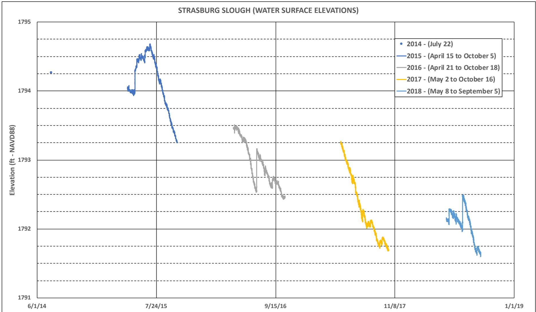
**Figure 13.** Strasburg Slough recorded water surface elevations
