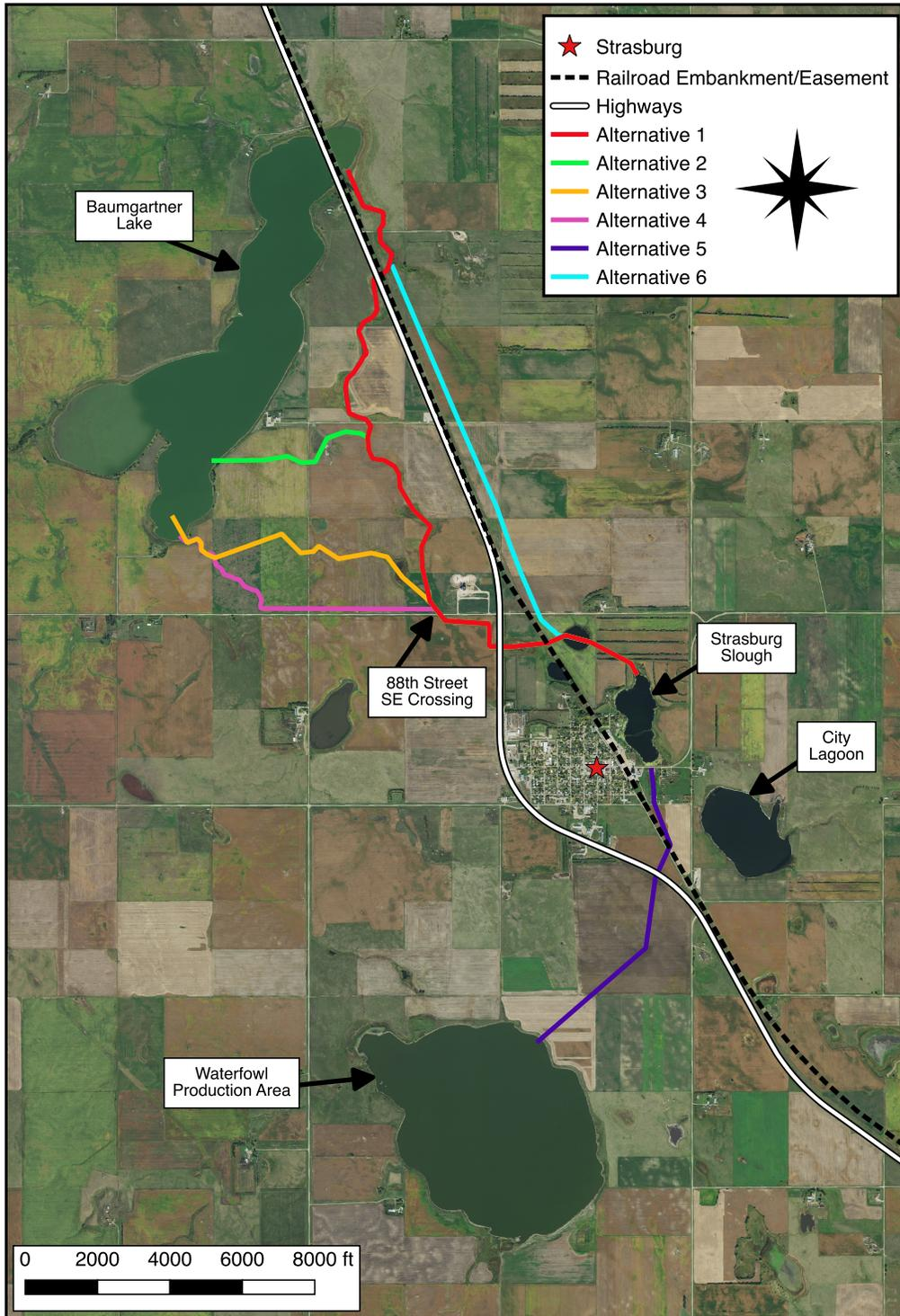
**Figure 22.** Open channel outlet alignments examined
