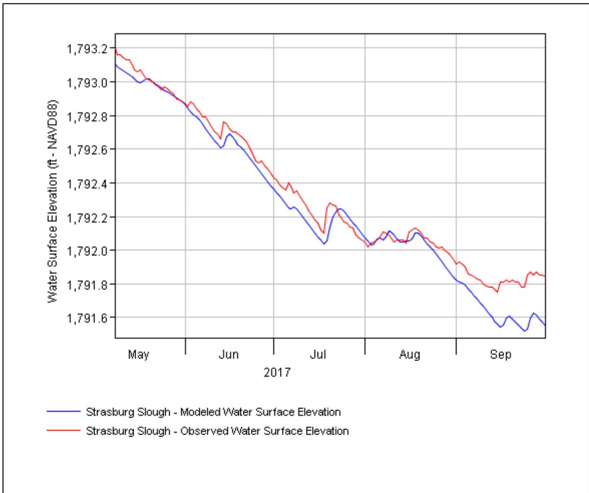
**Figure 18.** 2017 Strasburg Slough water surface comparison
