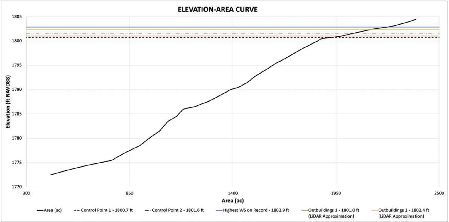
Figure 2 – Elevation-Area Curve
