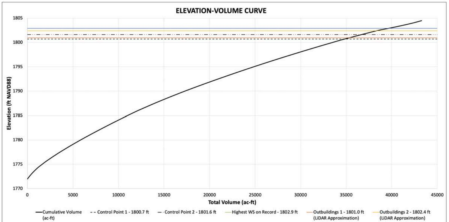
Figure 3 – Elevation-Volume Curve
