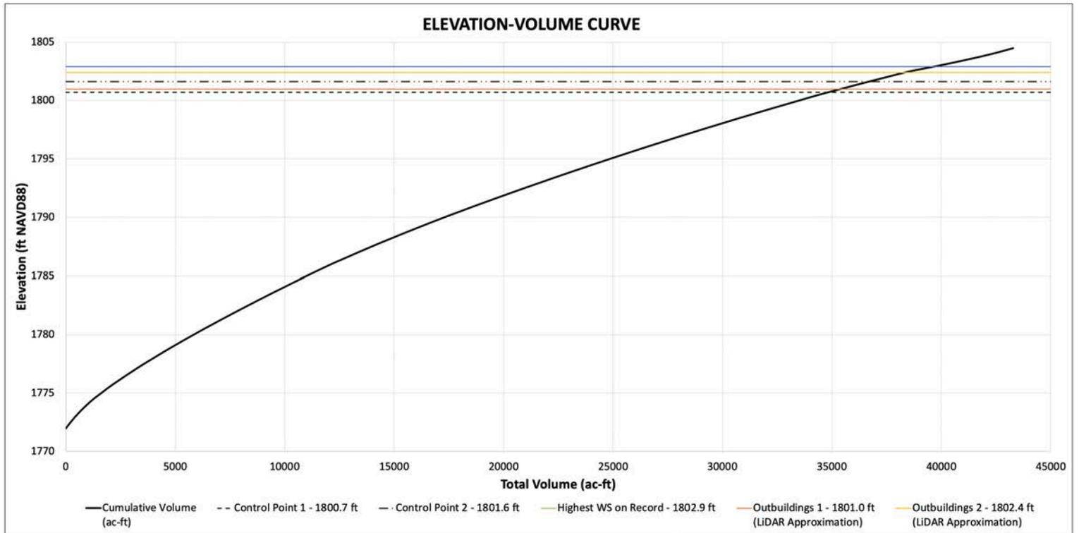
Figure 3 – Elevation-Volume Curve
