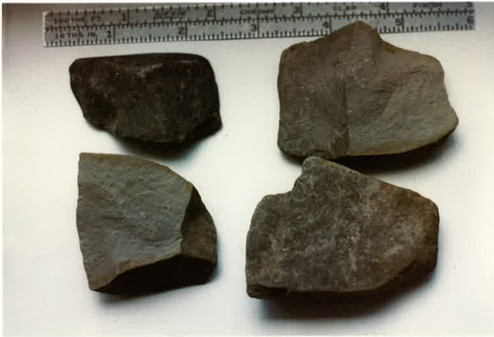
Photo No. 1 - Close-up view of some of the larger, angular shale fragments.
