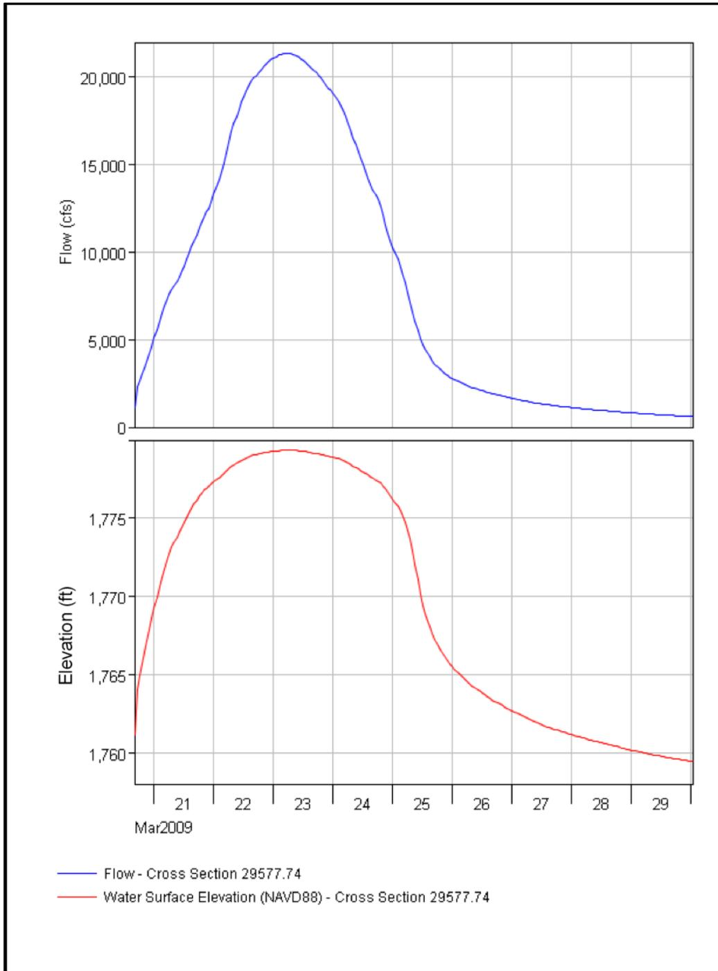
*Figure 9. 2009 modeled elevation and flow hydrographs at the USGS gage.*
