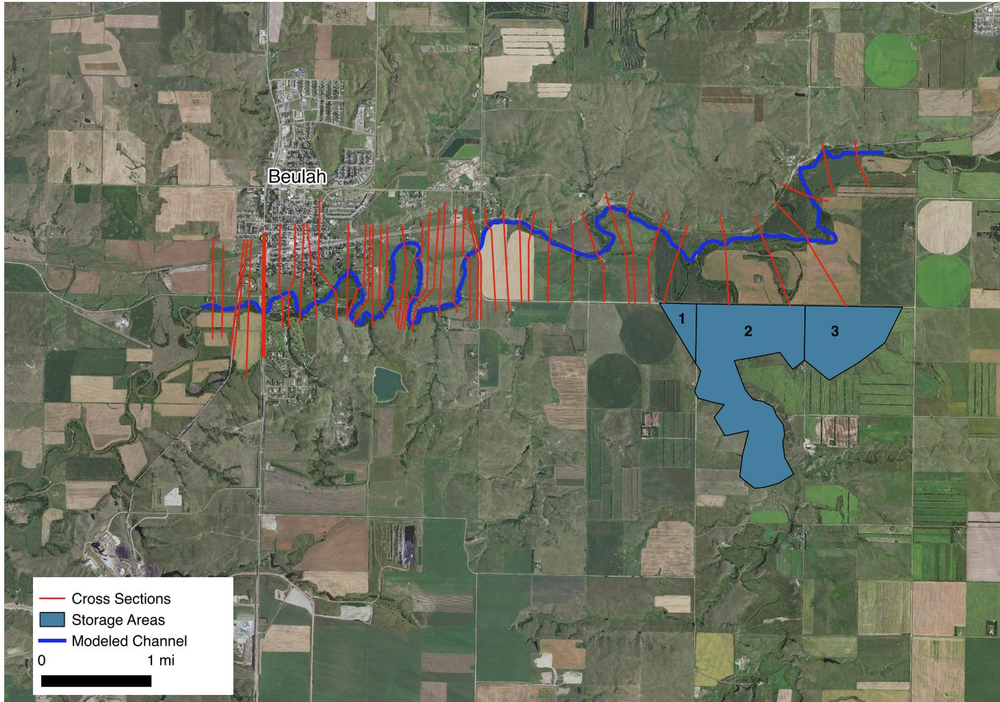
*Figure 2. Cross sections created for the Knife River model near Beulah, ND.*
