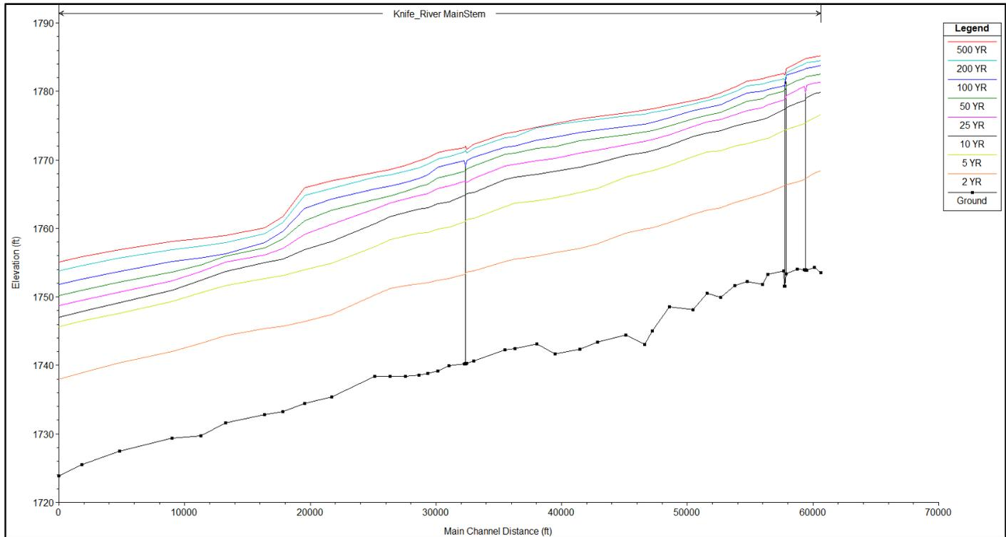
*Figure 14. Frequency events maximum water surface profile plot.*
