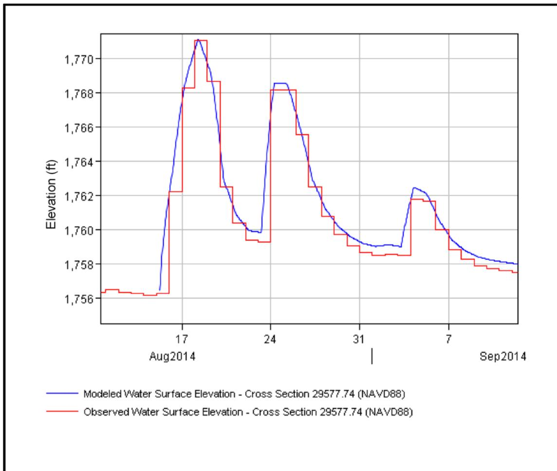
*Figure 5. 2014 USGS stream gage elevation compared to modeled water surface.*
