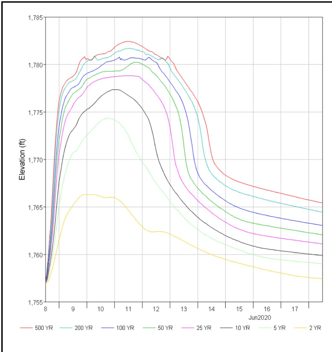
**Figure 13.** Frequency events modeled elevation plotted at the Beulah USGS gage.
