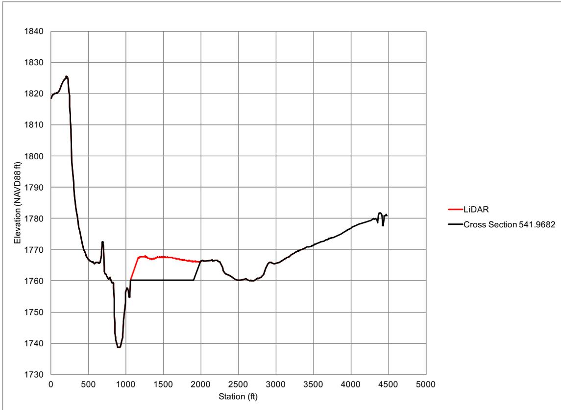
**Figure 25.** Modified hydraulic cross section 541.9682 for County Road 20 Restriction alternative.
