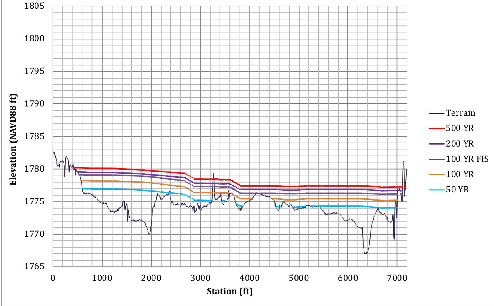
Figure 5. Water surface elevations along the alignment for East Levee A.
