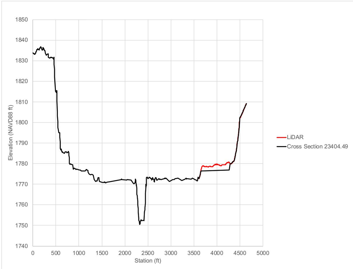
**Figure 21.** Modified hydraulic cross section 23404.49 for Lagoon Restriction 2 alternative.
