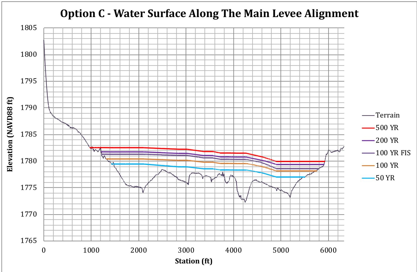
**Figure 13.** Water surface elevations along the alignment for Main Levee C.
