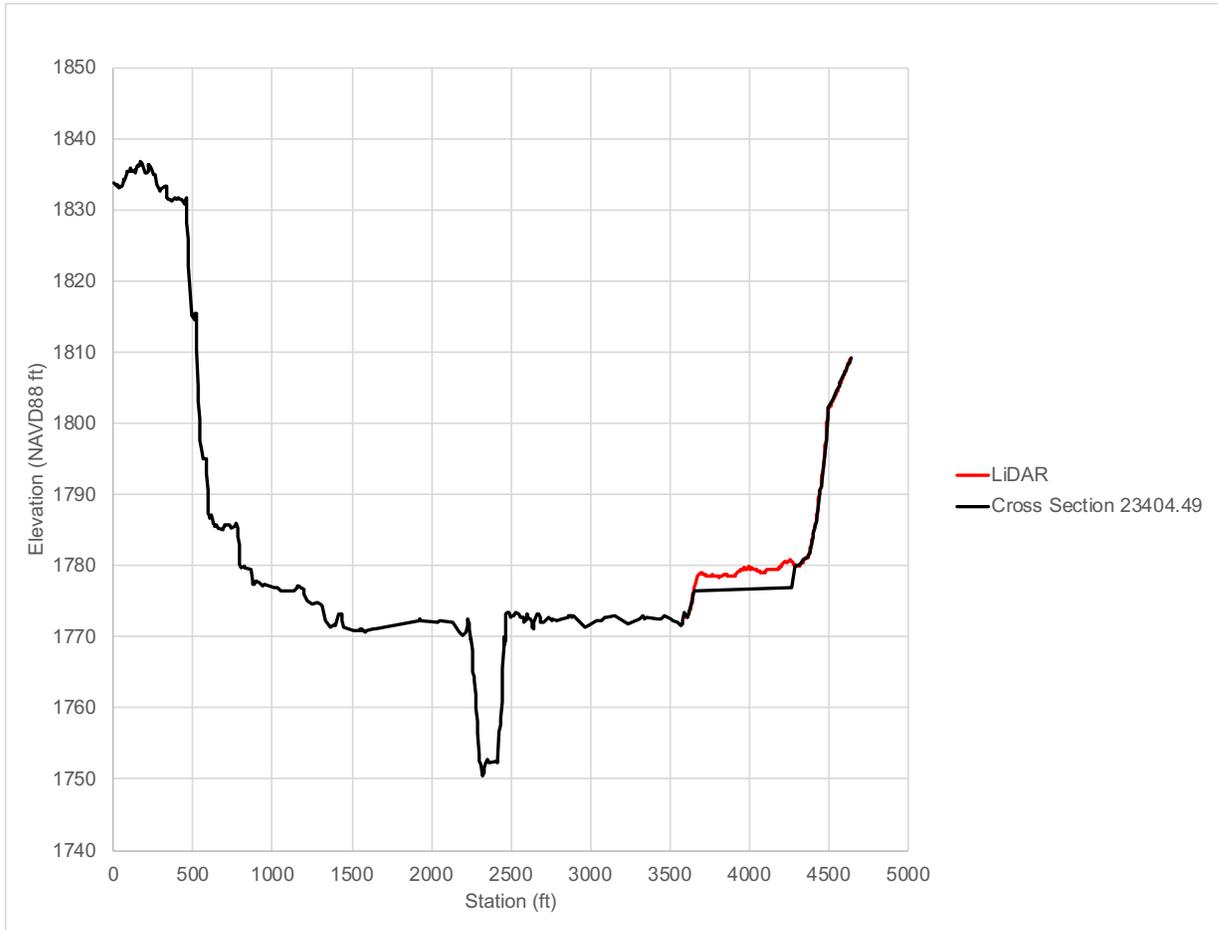
**Figure 18.** Modified hydraulic cross section 23404.49 for Lagoon Restriction 1 alternative.
