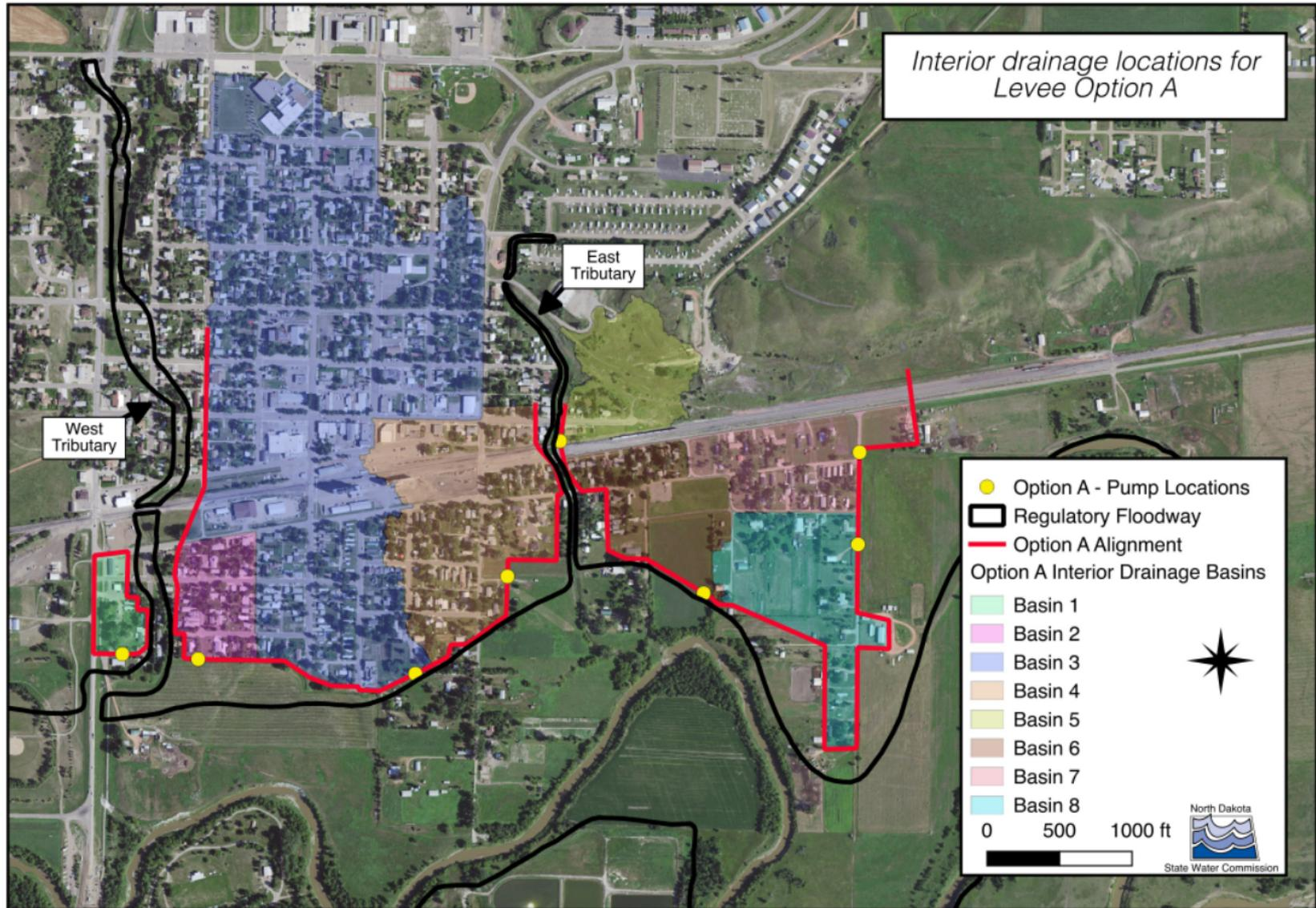
**Figure 3.** Interior drainage locations for Levee Option A.
