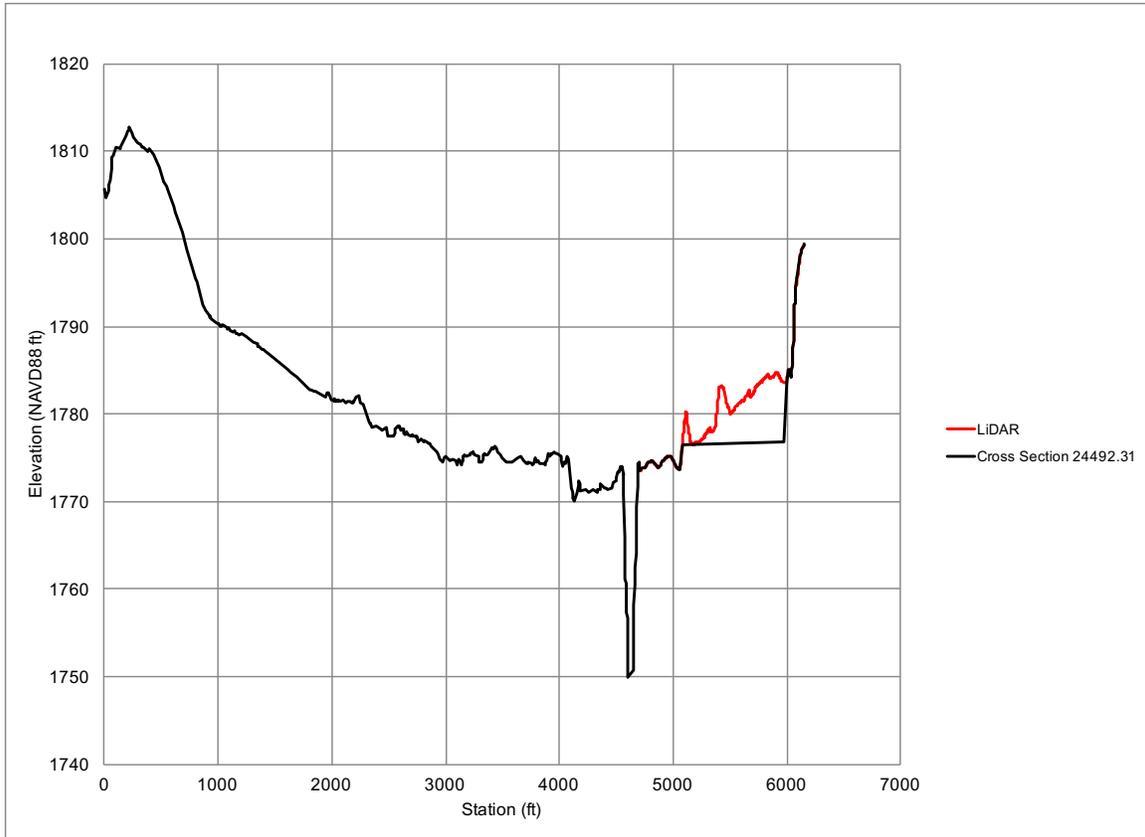
**Figure 20.** Modified hydraulic cross section 24492.31 for Lagoon Restriction 2 alternative.
