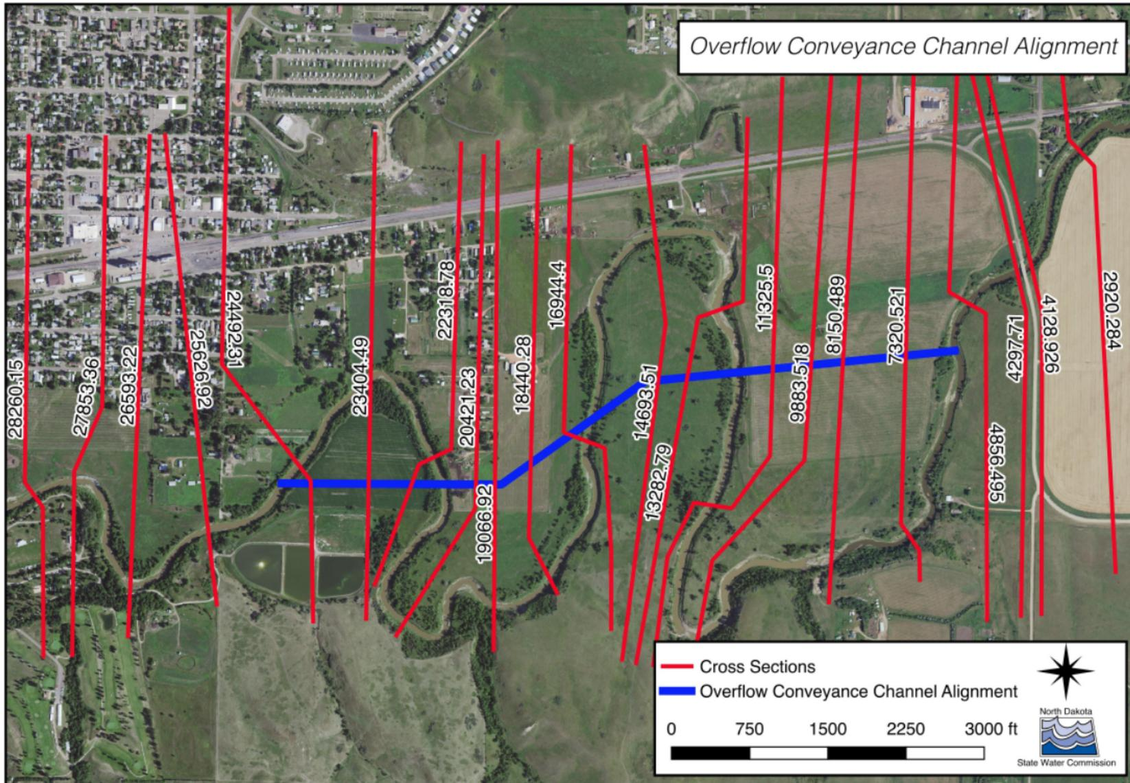
**Figure 27.** Centerline alignment for both overflow conveyance channel alternatives.
