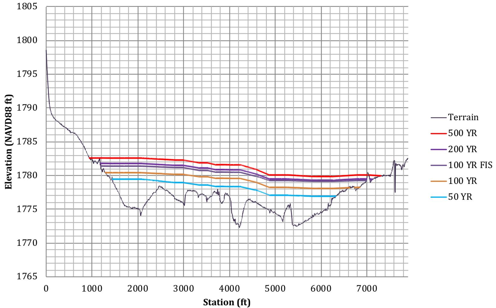
Figure 9. Water surface elevations along the alignment for Main Levee B.
