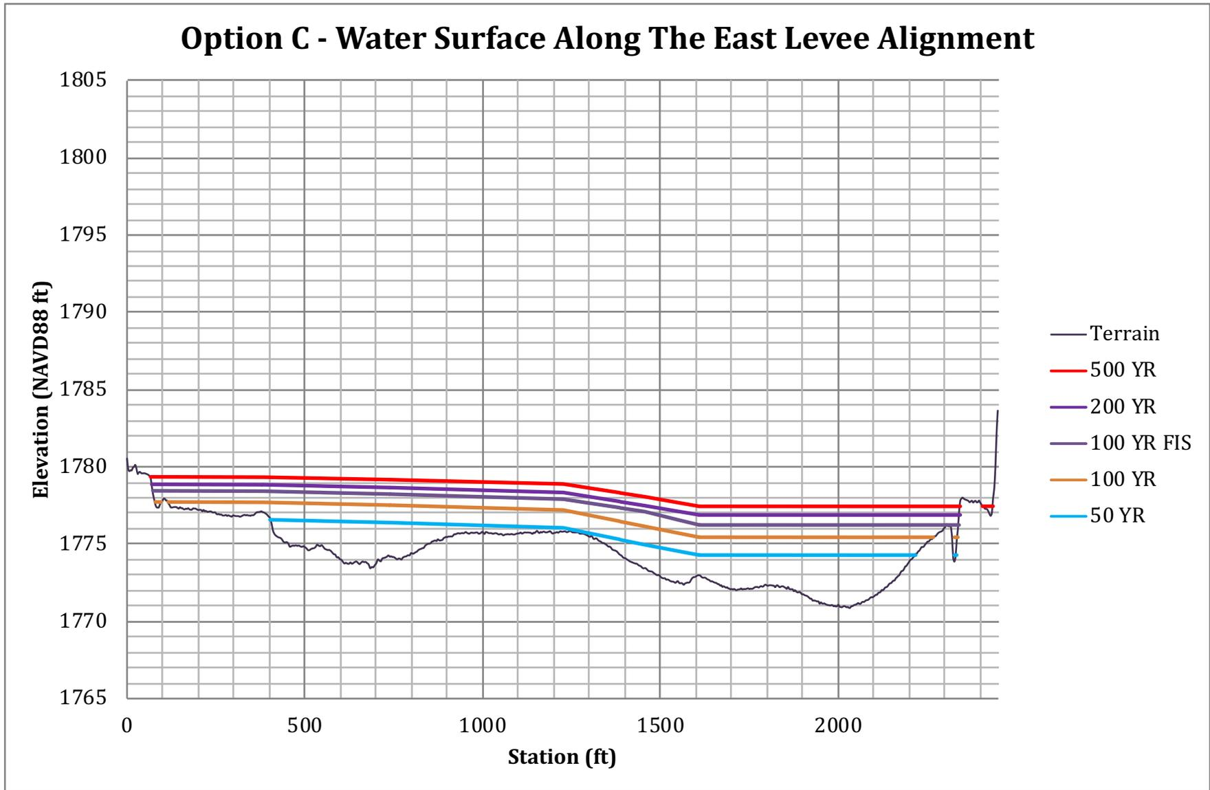
**Figure 14.** Water surface elevations along the alignment for East Levee C.
