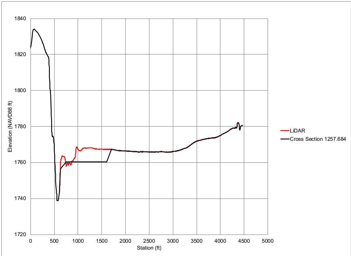
**Figure 24.** Modified hydraulic cross section 1257.684 for County Road 20 Restriction alternative.
