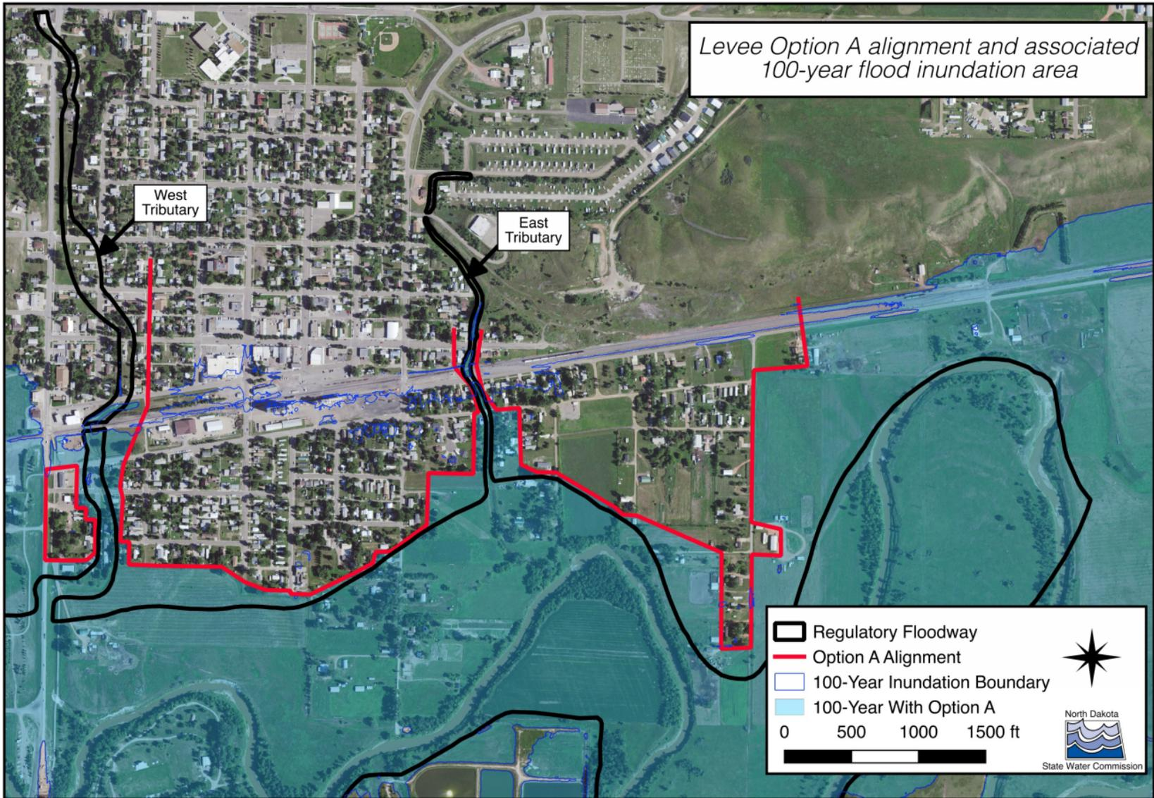
**Figure 2.** Levee Option A alignment and associated 100-year flood inundation area.
