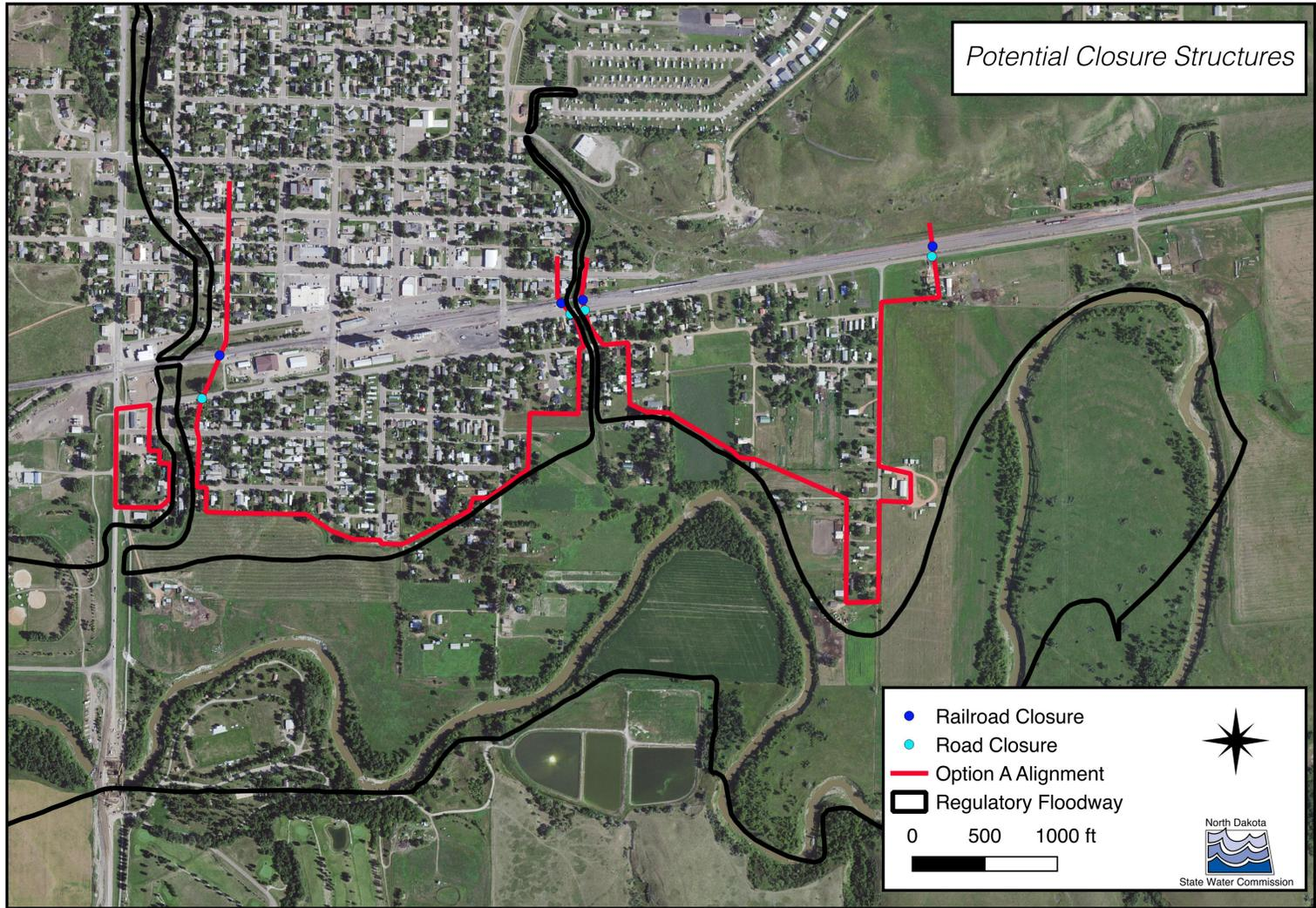
Figure 6. Locations for potential closure structures for Levee Option A.
