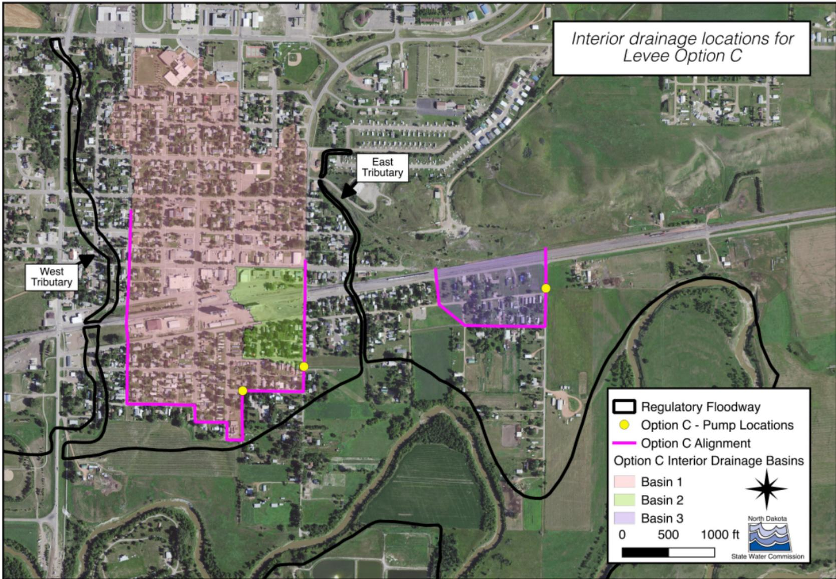
**Figure 12.** Interior drainage locations for Levee Option C.
