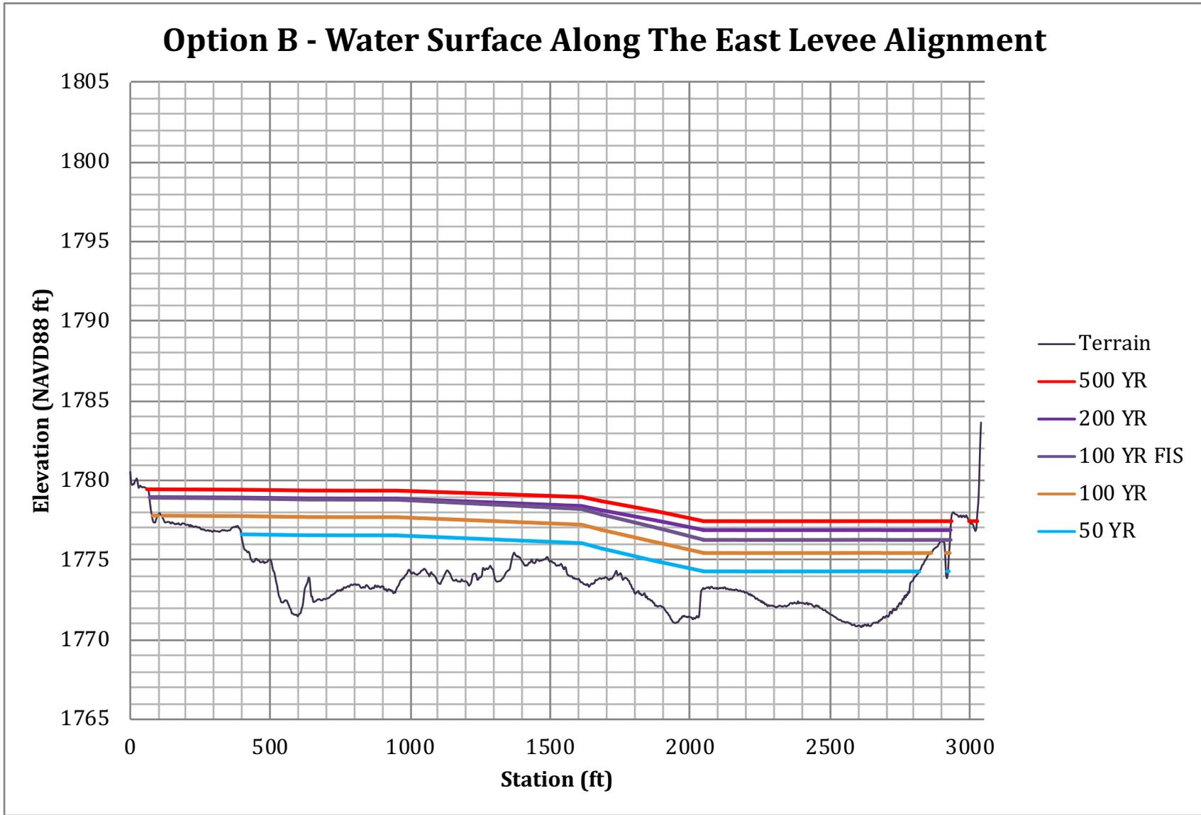
**Figure 10.** Water surface elevations along the alignment for East Levee B.
