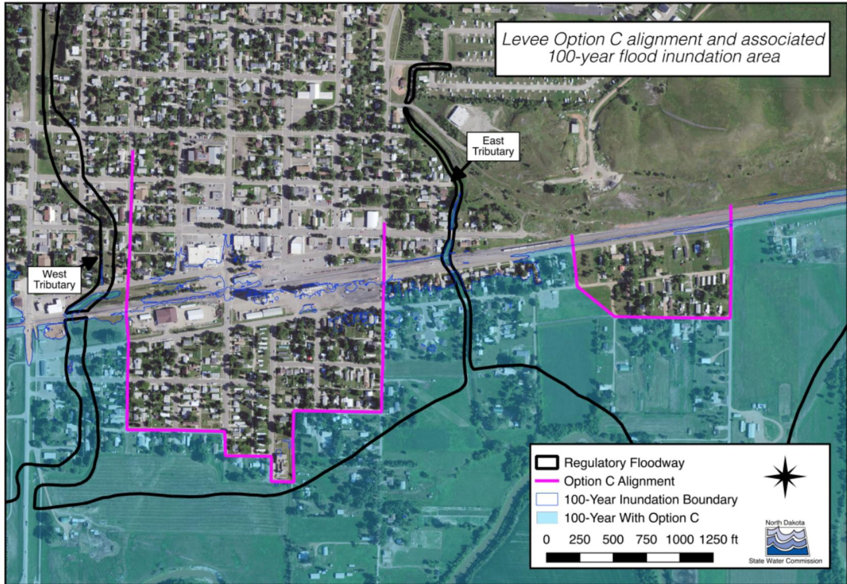
**Figure 11.** Levee Option C alignment and associated 100-year flood inundation area.
