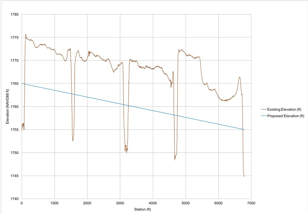
**Figure 26.** Channel invert profile for both overflow conveyance channel alternatives.
