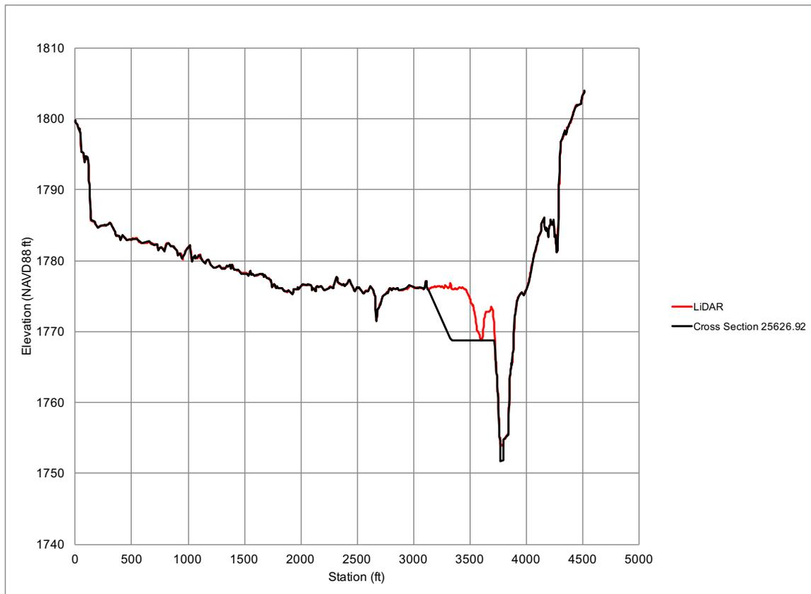
**Figure 19.** Modified hydraulic cross section 25626.92 for Lagoon Restriction 2 alternative.
