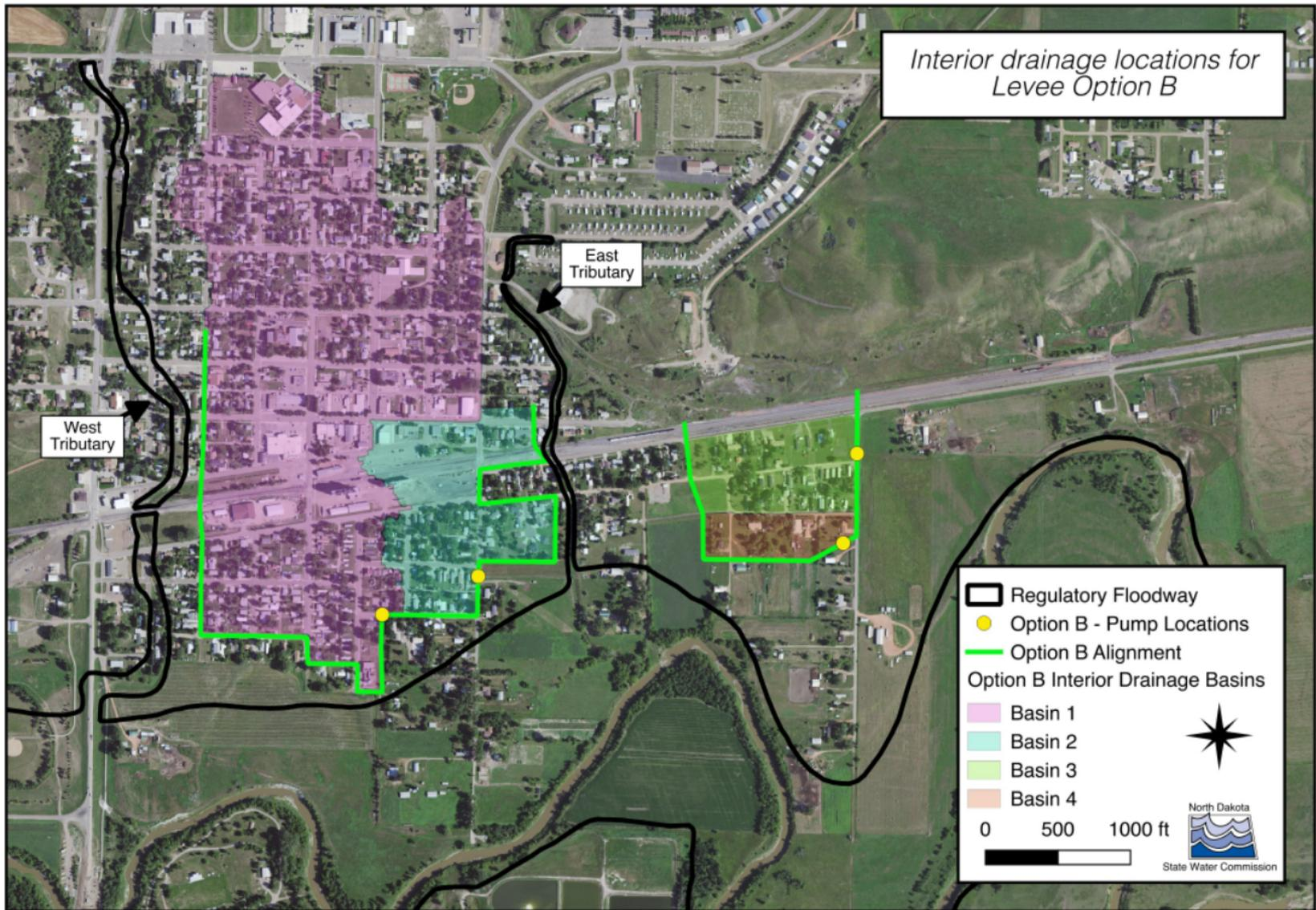
**Figure 8.** Interior drainage locations for Levee Option B.
