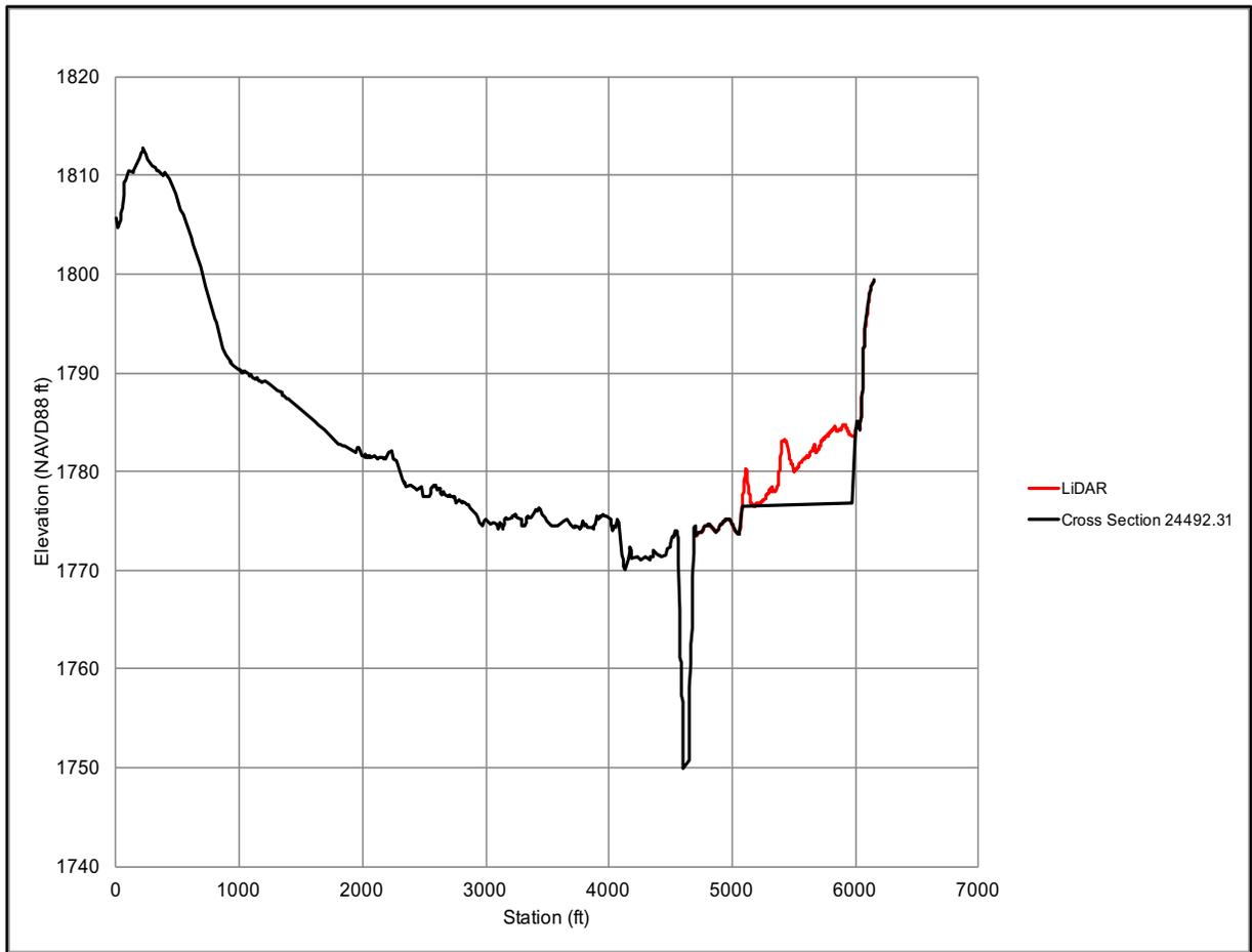
**Figure 17.** Modified hydraulic cross section 24492.31 for Lagoon Restriction 1 alternative.
