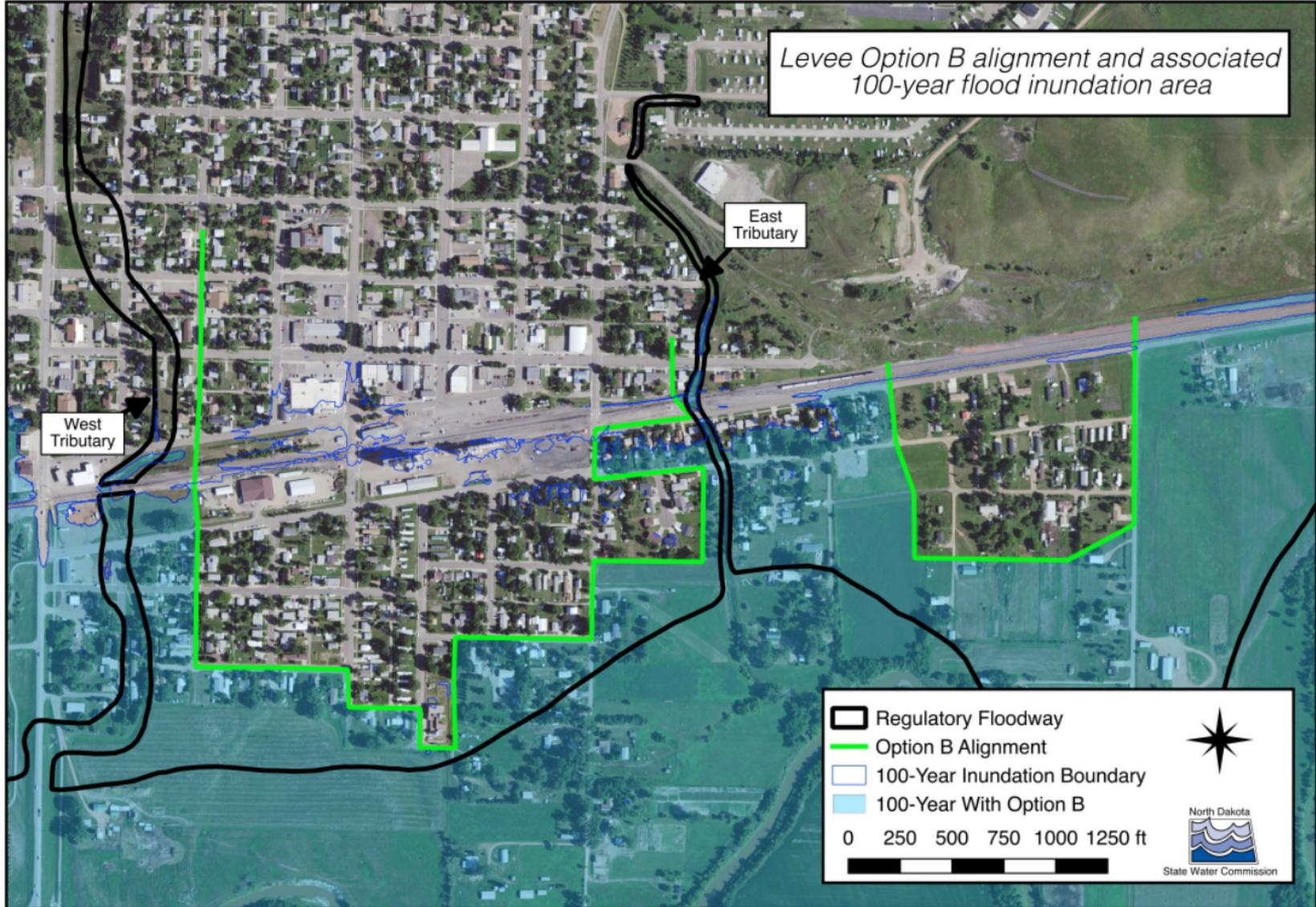
**Figure 7.** Levee Option B alignment and associated 100-year flood inundation area.
