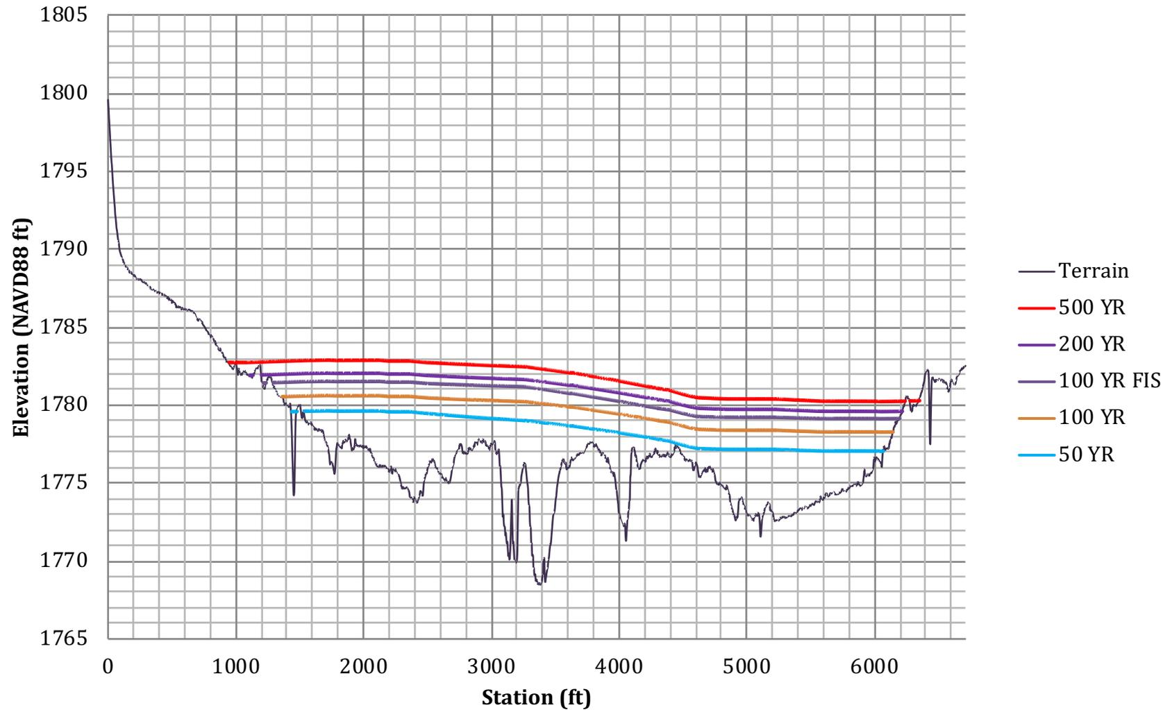
Figure 4. Water surface elevations along the alignment for Main Levee A.
