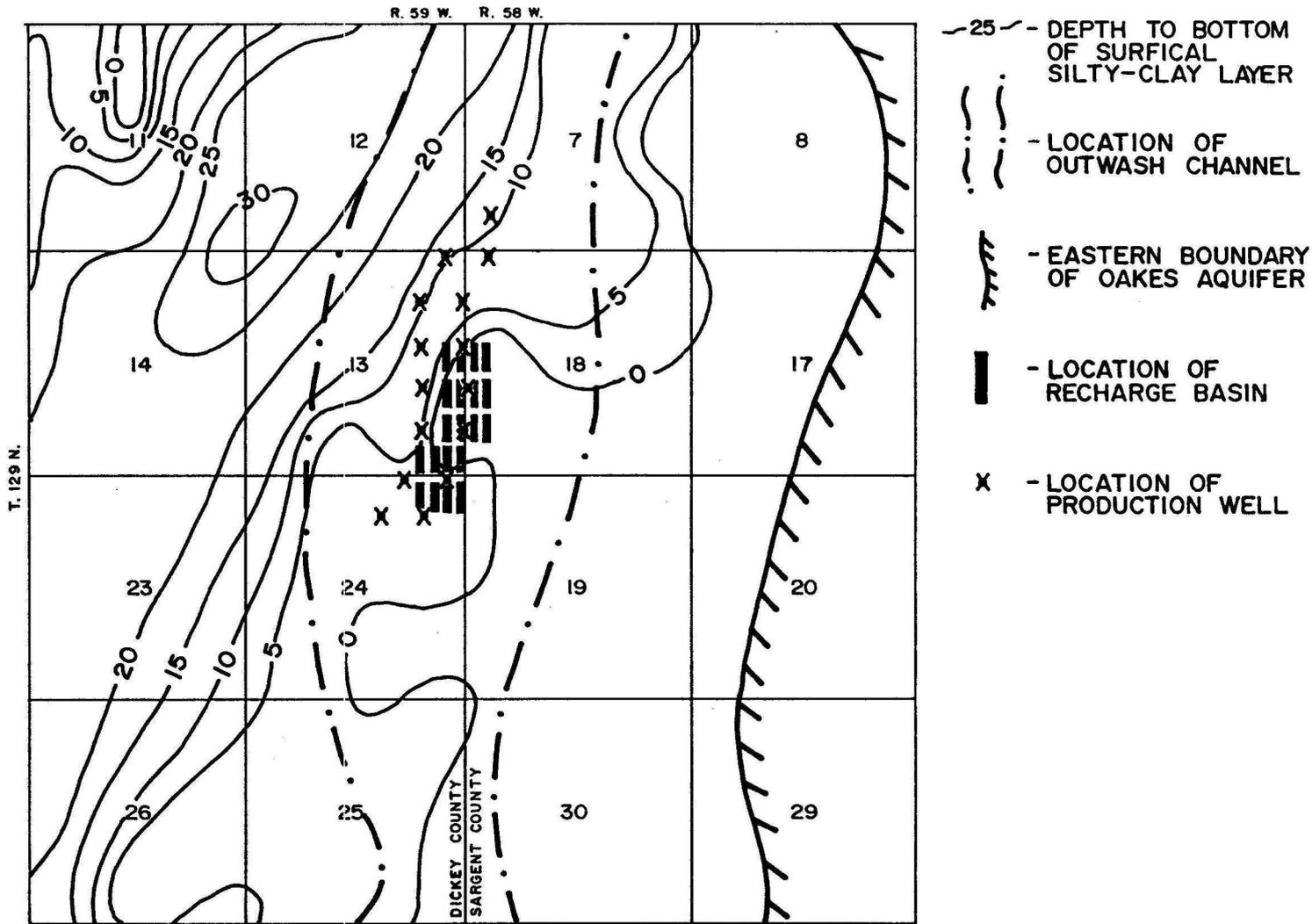
Figure 18.--Location of project-scale well field and recharge basins, based on an infiltration rate of 3 feet per day
