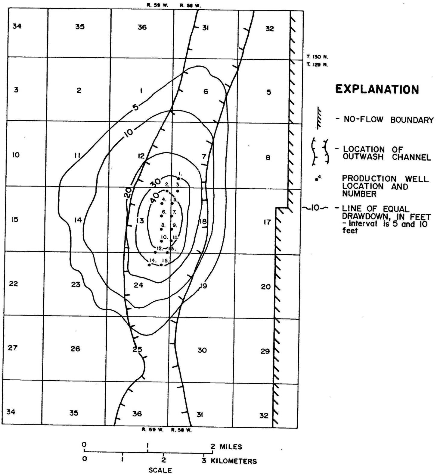
Figure 15.--Computer-simulated drawdown distribution after pumping 100 cubic feet per second for 60 days (11,900 acre-feet)
