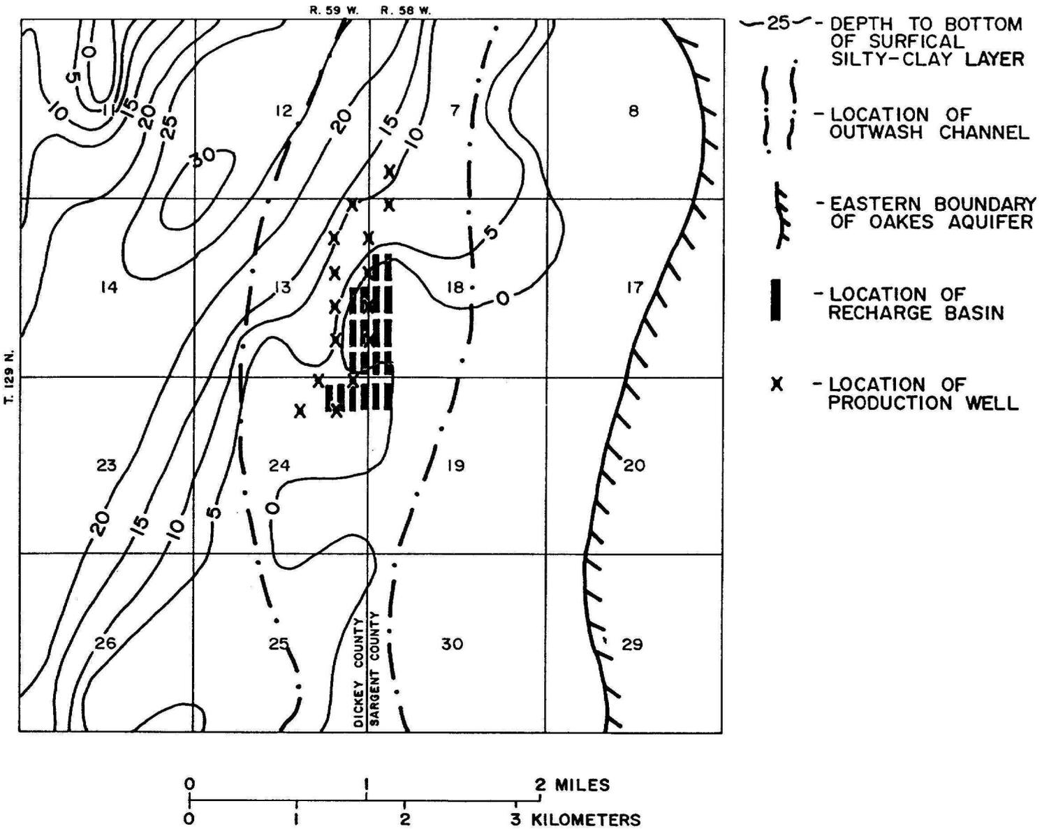
Figure 17.--Location of project-scale well field and recharge basins, based on an infiltration rate of 2 feet per day
