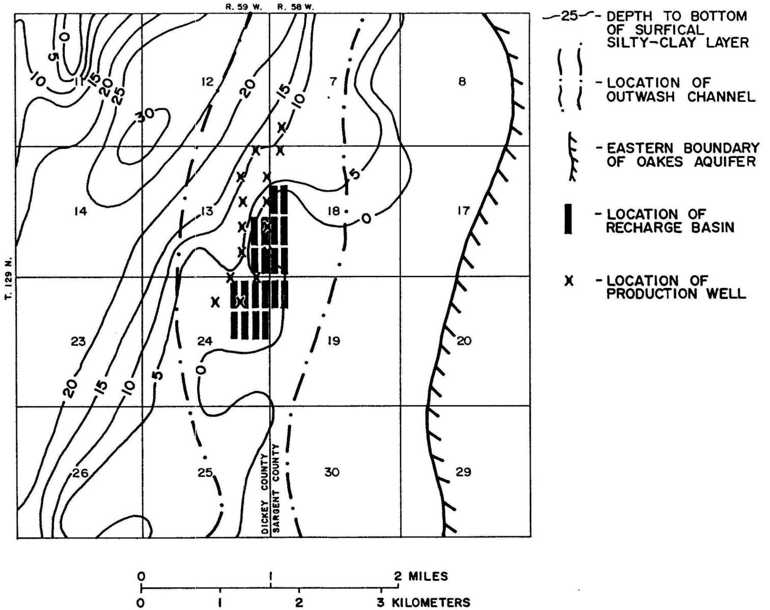
Figure 16.--Location of project-scale well field and recharge basins, based on an infiltration rate of 1 foot per day
