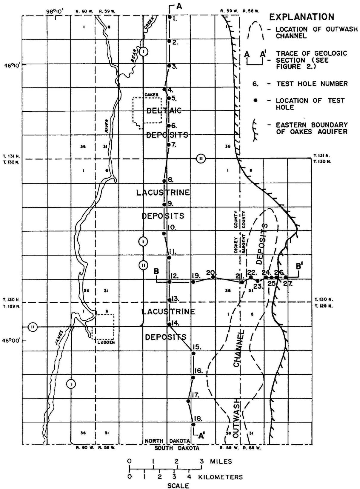
Figure 3.--Areal distribution of depositional facies in the Oakes aquifer and locations of geologic sections A-A' and B-B'
