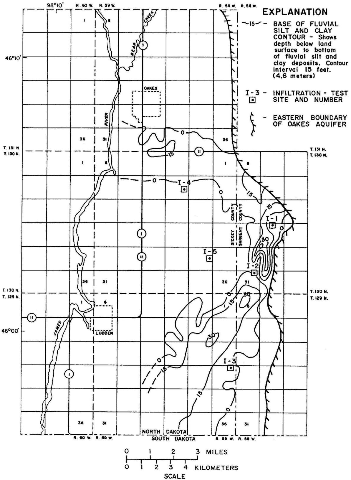
Figure 4.--Depth below land surface to bottom of fluvial silt and clay deposits
