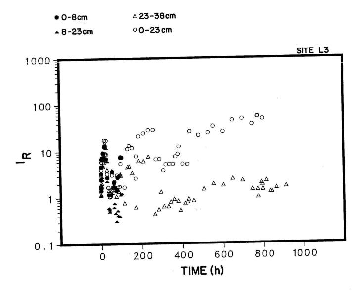
Fig. 25. Impedance ratio measurements for site L3 during the Fall 1986 large basin test.
