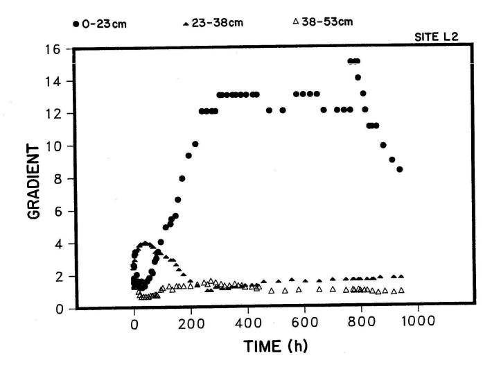
Fig. 22. Hydraulic gradient measurements for site L2 during the Fall 1986 large basin test.
