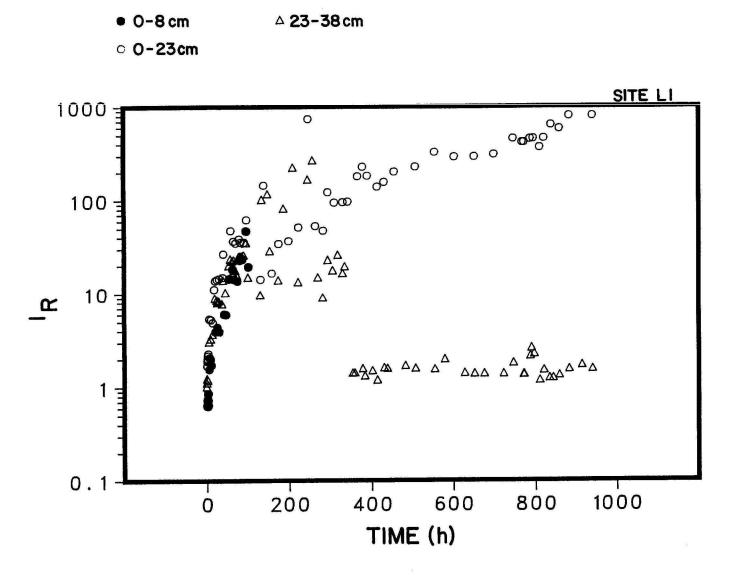
Fig. 21. Impedance ratio measurements for site L1 during the Fall 1986 large basin test.
