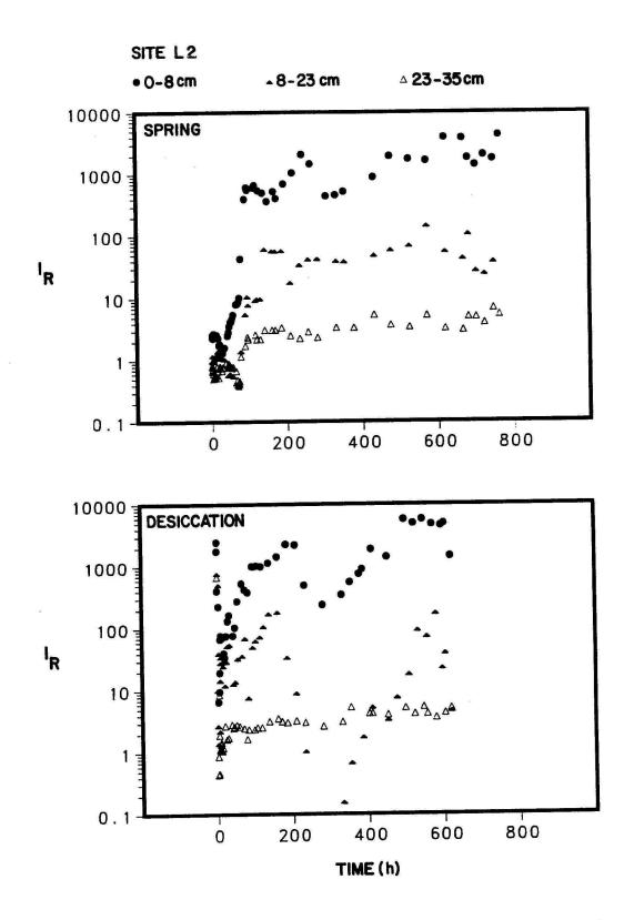
Fig. 38. Impedance ratio measurements for site L2 during the Spring 1987 test and following desiccation.
