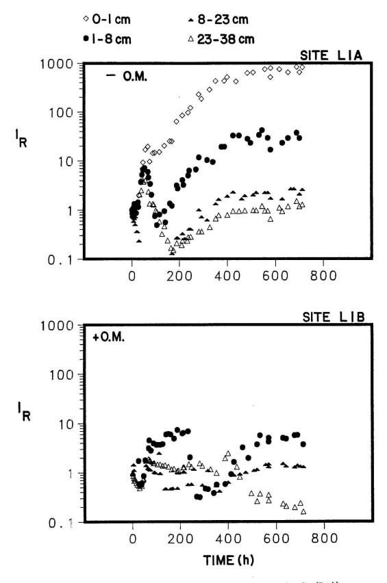
Fig. 48. Impedance ratio measurements for paired check (L1A) and organic mat covered (L1B) in-situ hydraulic monitoring sites during the 1987 Organic Mat test. + O.M. = with organic mat, - O.M. = check.
