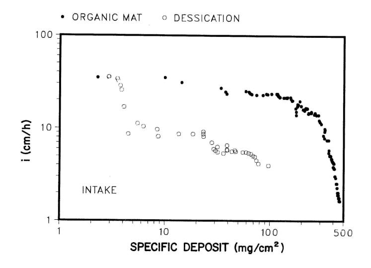
Fig. 64. Infiltration rate vs. cumulative suspended solids delivered to the basin, for the Organic Mat, and Organic Mat + Desiccation tests.
