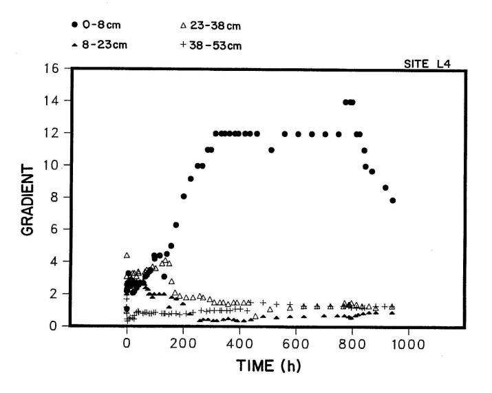
Fig. 26. Hydraulic gradient measurements for site L4 during the Fall 1986 large basin test.
