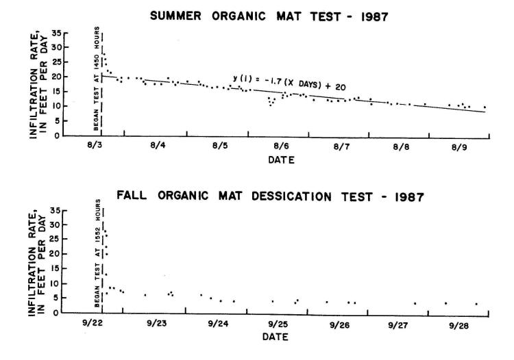
Fig. 61. Comparison of infiltration rates for 1987 Organic Mat tests before and after desiccation.
