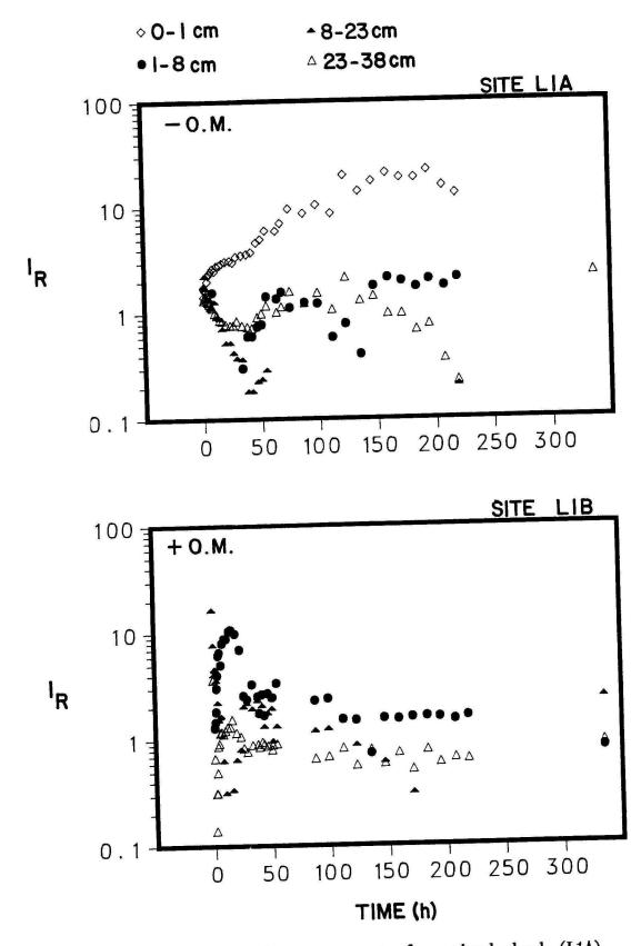
Fig. 50. Impedance ratio measurements for paired check (L1A) and organic mat covered (L1B) in-situ hydraulic monitoring sites during the 1987 Organic Mat test - after natural renovation by desiccation. + 0.M. = with organic mat, - 0.M. = check.
