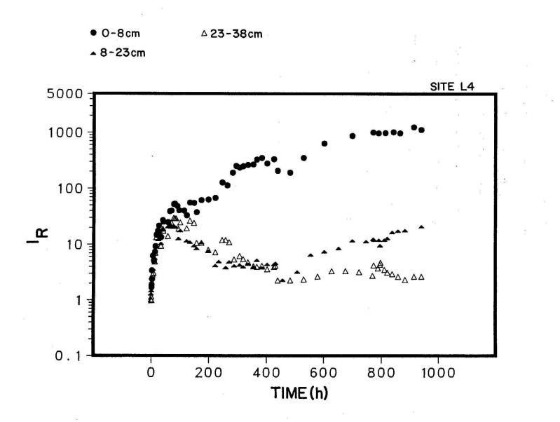
Fig. 27. Impedance ratio measurements for site L4 during the Fall 1986 large basin test.
