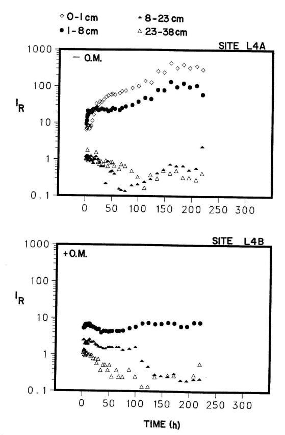
Fig. 59. Impedance ratio measurements for paired check (L4A) and organic mat covered (L4B) in-situ hydraulic monitoring sites during the 1987 Organic Mat test - after natural renovation by desiccation. + 0.M. = with organic mat, - 0.M. = check.
