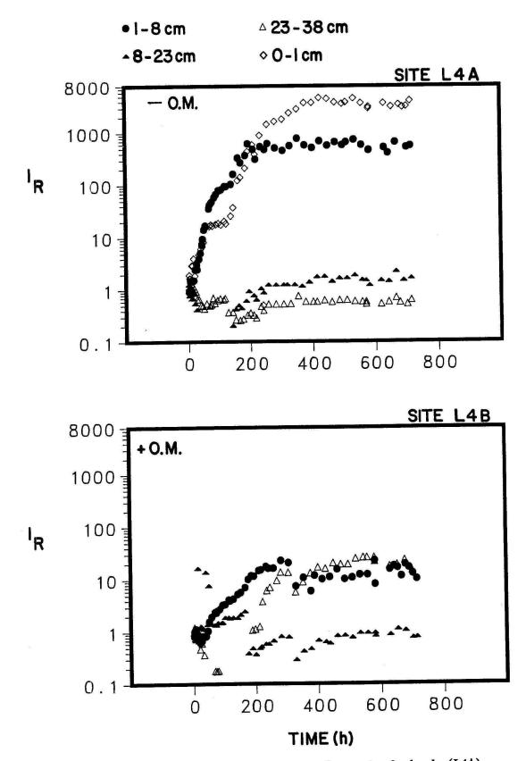
Fig. 58. Impedance ratio measurements for paired check (L4A) and organic mat covered (L4B) in-situ hydraulic monitoring sites during the 1987 Organic Mat test. + O.M = with organic mat, - O.M. = check.
