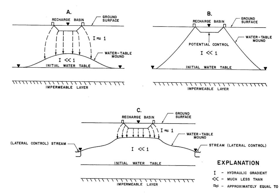
Fig. 7. Water-table mounds and the effect of selected boundary conditions on mound height and shape.
