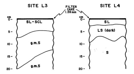
Fig. 28. Large basin morphology at tensiometer installations after completion of the Fall 1986 test. S = sand, SL = sandy loam, LS = loamy sand, SCL = sandy-clay loam, f. = fine, m. = medium, co. = coarse, g. = gravelly. densities of disturbed and structureless clay soil materials by Gupta and Larson (1979).
