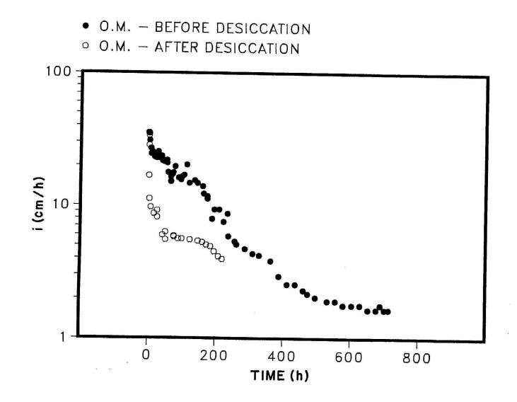
Fig. 45. Infiltration rate measured at the intake for the 1987 Organic-Mat test before and after natural renovation by desiccation.
