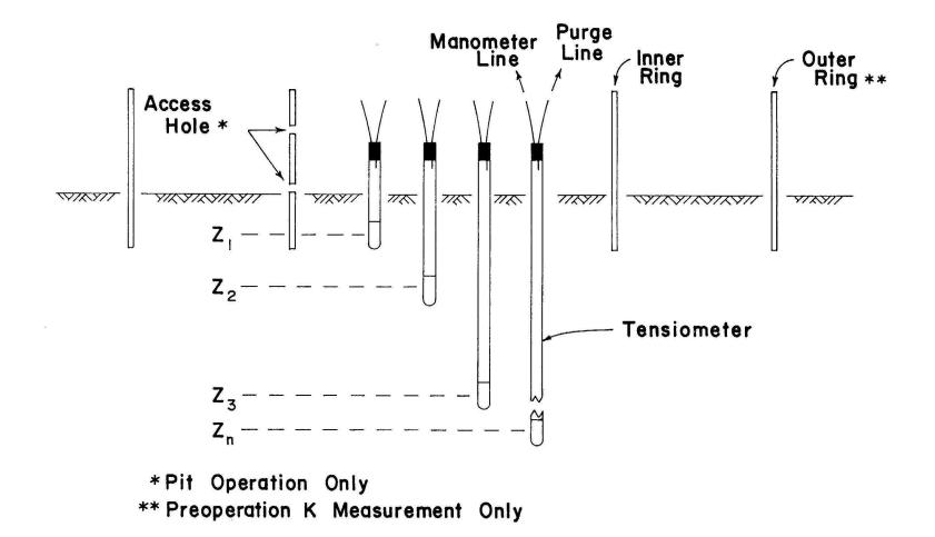
Fig. 12. Apparatus for determining in-situ K(S) and for monitoring local flux and layered impedance development in the basin subsoil during basin operation.
