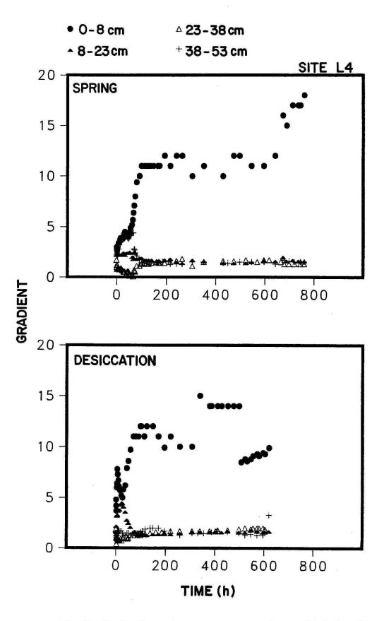
Fig. 41. Hydraulic gradient measurements for site L4 during the Spring 1987 test and following desiccation.
