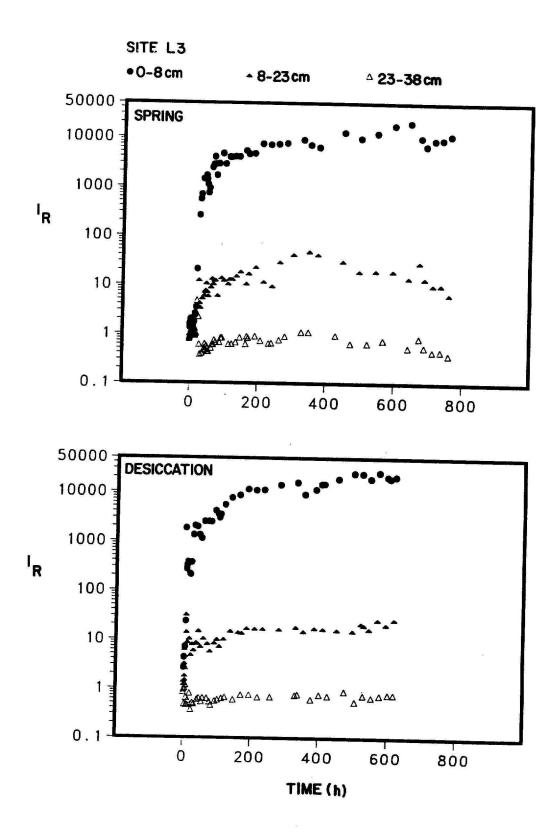
Fig. 40. Impedance ratio measurements for site L3 during the Spring 1987 test and following desiccation.
