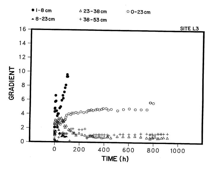
Fig. 24. Hydraulic gradient measurements for site L3 during the Fall 1986 large basin test.
