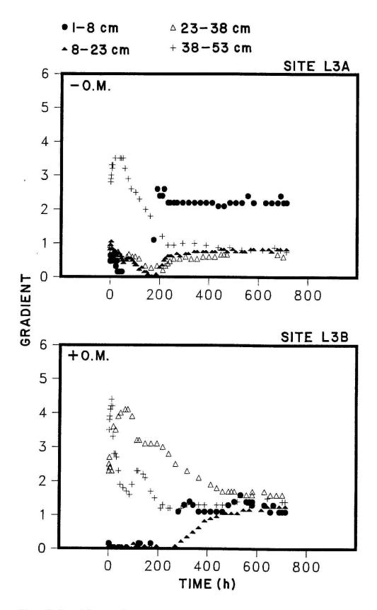
Fig. 54. Hydraulic gradient measurements for paired check (L3A) and organic mat covered (L3B) in-situ hydraulic monitoring sites during the 1987 Organic Mat test. + 0.M. = with organic mat, - 0.M. = check.
