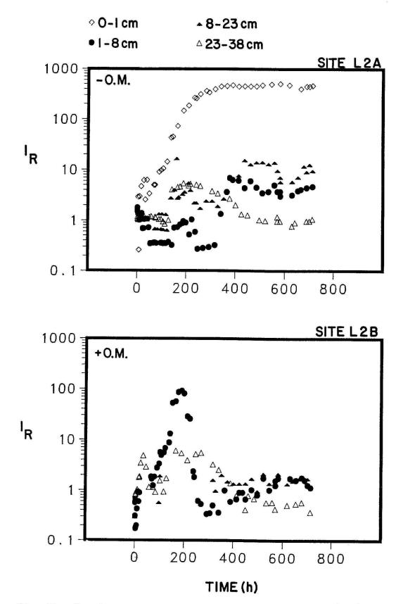
Fig. 52. Impedance ratio measurements for paired check (L2A) and organic mat covered (L2B) in-situ hydraulic monitoring sites during the 1987 Organic Mat test.
