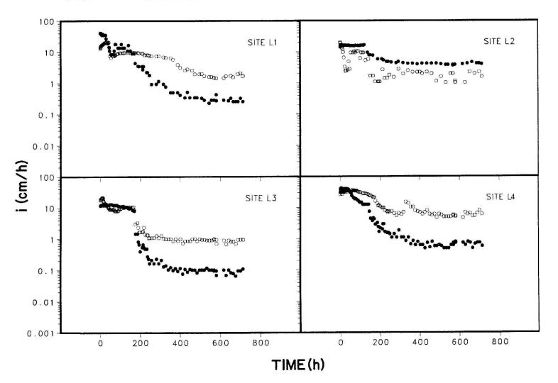
Fig. 49. Infiltration rate measured at in-situ basin monitoring sites L1, L2, L3, and L4 for check (non-covered) and organic-mat covered treatments.
