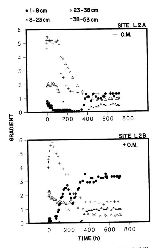
Fig. 51. Hydraulic gradient measurements for paired check (L2A) and organic mat covered (L2B) in-situ hydraulic monitoring sites during the 1987 Organic Mat test. + O.M. = with organic mat, - O.M. = check.
