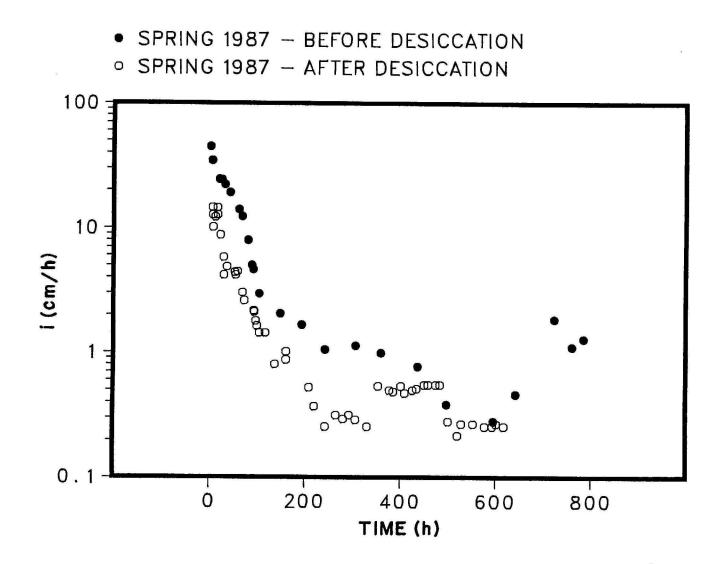
Fig. 33. Infiltration rate as measured at the basin intake for the Spring, 1987, test before and after natural renovation by desiccation.
