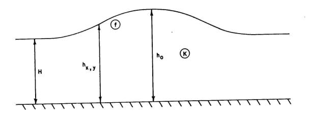
Fig. 8. Geometry and symbols for a rectangular infiltration area and underlying water-table mound in an unconfined aquifer (from Bouwer, 1978).
