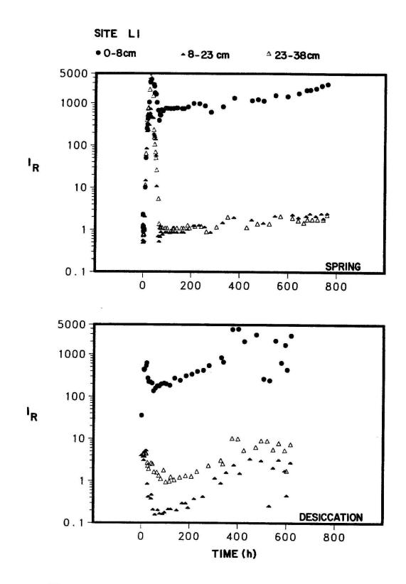
Fig. 36. Impedance ratio measurements for site L1 during the Spring 1987 test and following desiccation.
