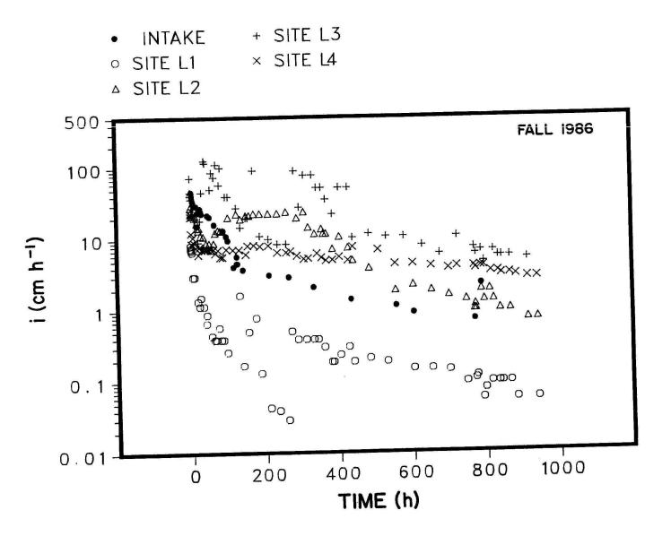
Fig. 19. Large basin infiltration for Fall 1986 determined at the intake to the basin, and at local monitoring sites L1, L2, L3, and L4.
