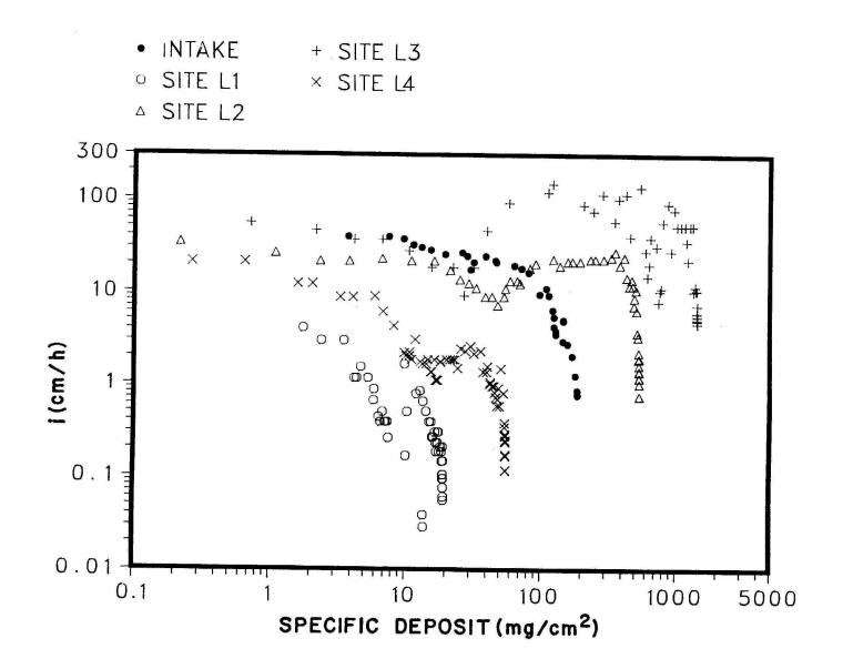
Fig. 62. Infiltration rate vs. cumulative suspended solids delivered to the basin during the Fall 1986 test.
