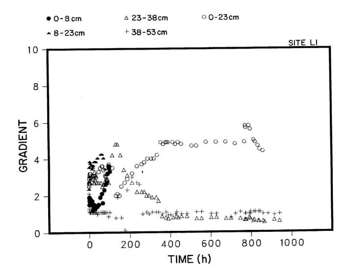
Fig. 20. Hydraulic gradient measurements for site L1 during the Fall 1986 large basin test.
