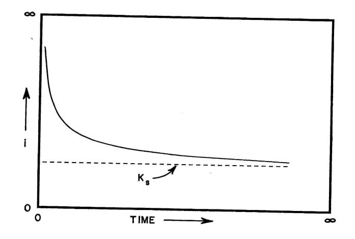
Fig. 6. Unscaled plot of infiltration vs. time.
