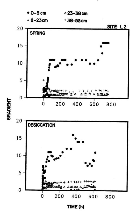
Fig. 37. Hydraulic gradient measurements for site L2 during the Spring 1987 test and following desiccation.
