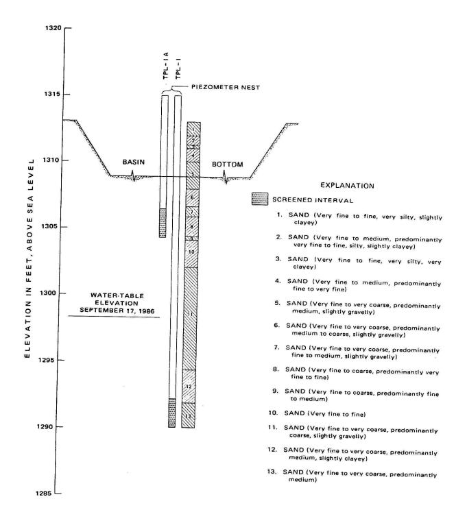
Fig. 14. Vertical profile at the center of the large test basin, showing piezometer depth placement.
