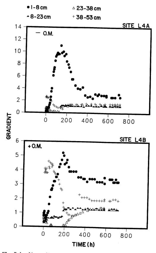
Fig. 57. Hydraulic gradient measurements for paired check (L4A) and organic mat covered (L4B) in-situ hydraulic monitoring sites during the 1987 Organic Mat test. + 0.M. = with organic mat. - 0.M. = check.
