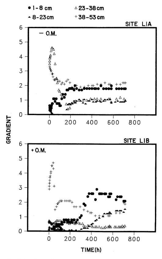
Fig. 47. Hydraulic gradient measurements for paired check (L1A) and organic mat covered (L1B) in-situ hydraulic monitoring sites during the 1987 Organic Mat test. + O.M. = with organic mat. - O.M. = check.
