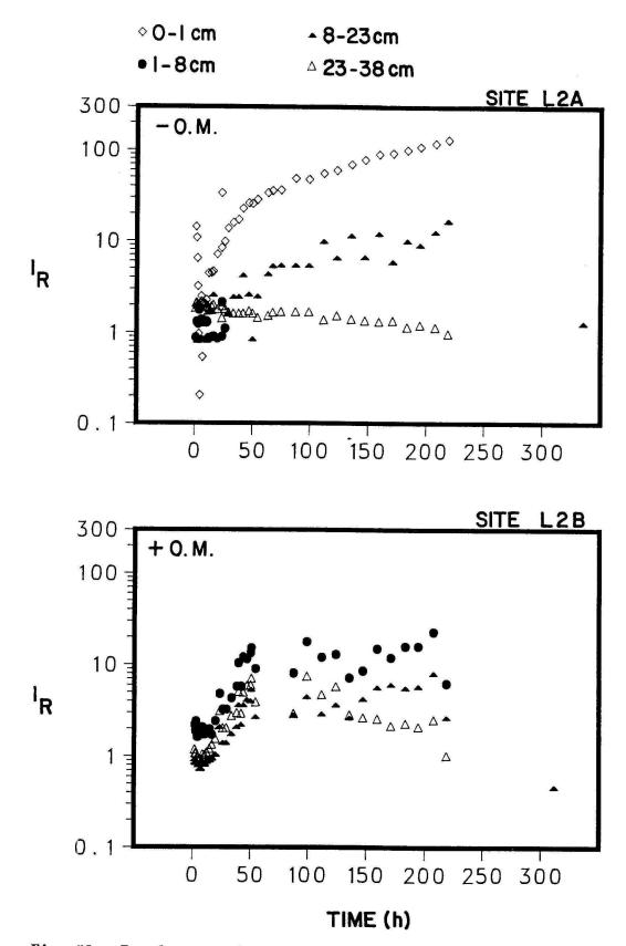
Fig. 53. Impedance ratio measurements for paired check (L2A) and organic mat covered (L2B) in-situ hydraulic monitoring sites during the 1987 Organic Mat test - after natural renovation by desiccation. + 0.M. = with organic mat, - 0.M. = check.
