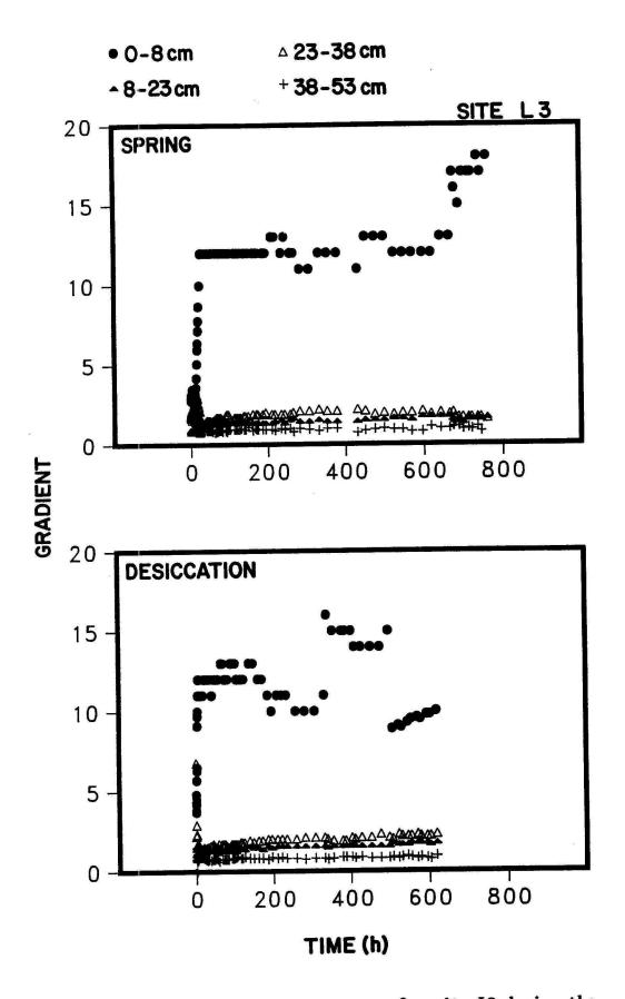
Fig. 39. Hydraulic gradient measurements for site L3 during the Spring 1987 test and following desiccation.
