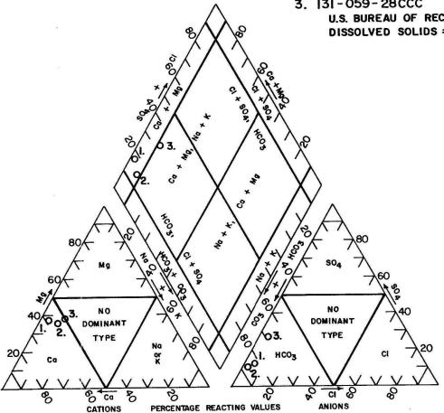
Hydrochemical facies of ground water in the Oakes Aquifer test area displayed on a Piper diagram. Fig. 5.
