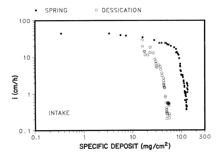
Fig. 63. Infiltration rate vs. cumulative suspended solids delivered to the basin, before and after desiccation during for the Spring, 1987, basin test.
