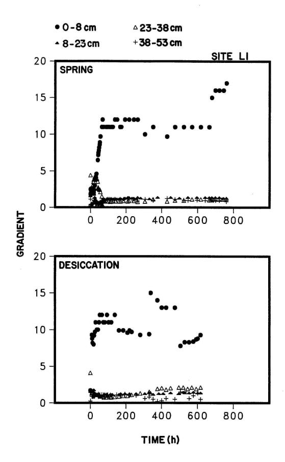
Fig. 35. Hydraulic gradient measurements for site L1 during the Spring 1987 test and following desiccation.
