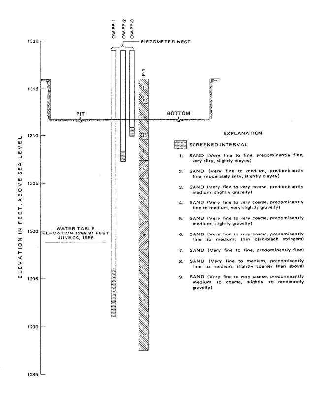
Fig. 11. Vertical profile at center of preliminary test basin showing piezometer depth placement.
