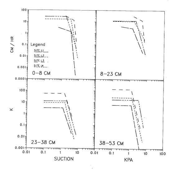
Fig. 18. Unsaturated hydraulic conductivity function [K(S)] profiles for sites L1, L2, L3, and L4 (large basin) during the Fall, 1986, basin test.
