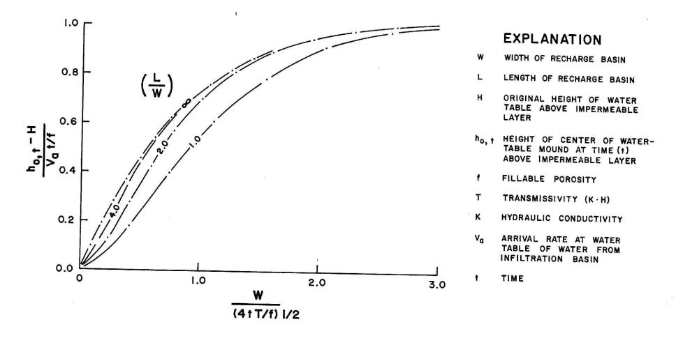
Fig. 9. Dimensionless plot of the rise at the center (ho) of the mound beneath a rectangular recharge area for different ratios of length to width (from Bianchi and Muckel, 1970).
