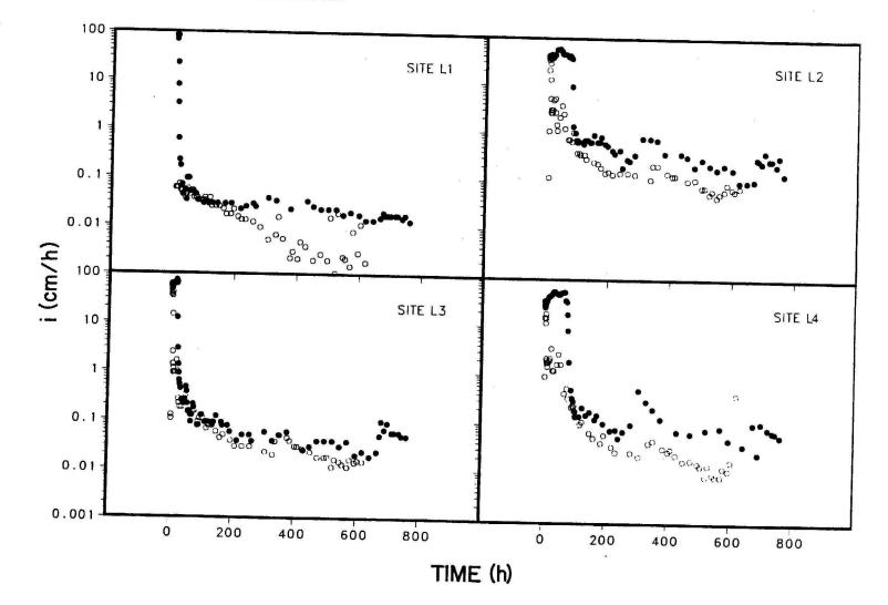
Fig. 34. Infiltration rate measured at in-situ basin positions L1, L2, L3, and L4 during the Spring 1987 test before and after natural renovation by desiccation.
