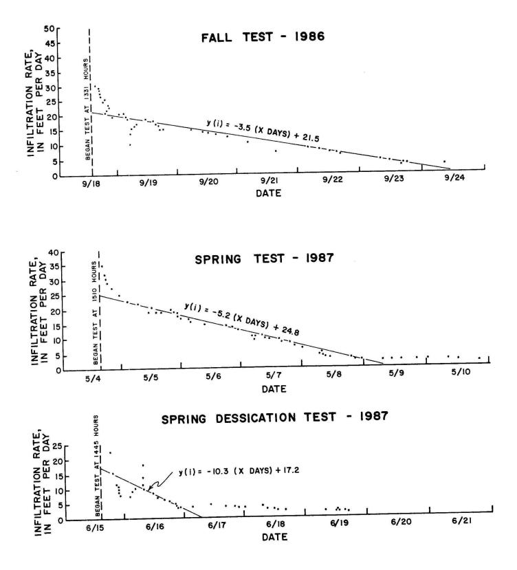
Fig. 60. Comparison of Fall 1986 and Spring 1987 (before and after desiccation) infiltration rates vs. time.
