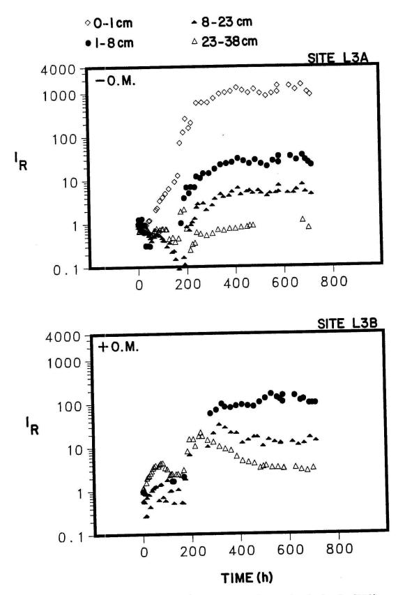
Fig. 55. Impedance ratio measurements for paired check (L3A) and organic mat covered (L3B) in-situ hydraulic monitoring sites during the 1987 Organic Mat test. + O.M. = with organic mat, - O.M. = check.
