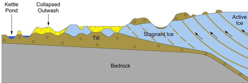
**Figure 2.** Cross section showing the collapsed glacial topography that arises from ice-sheet stagnation and wasting.
