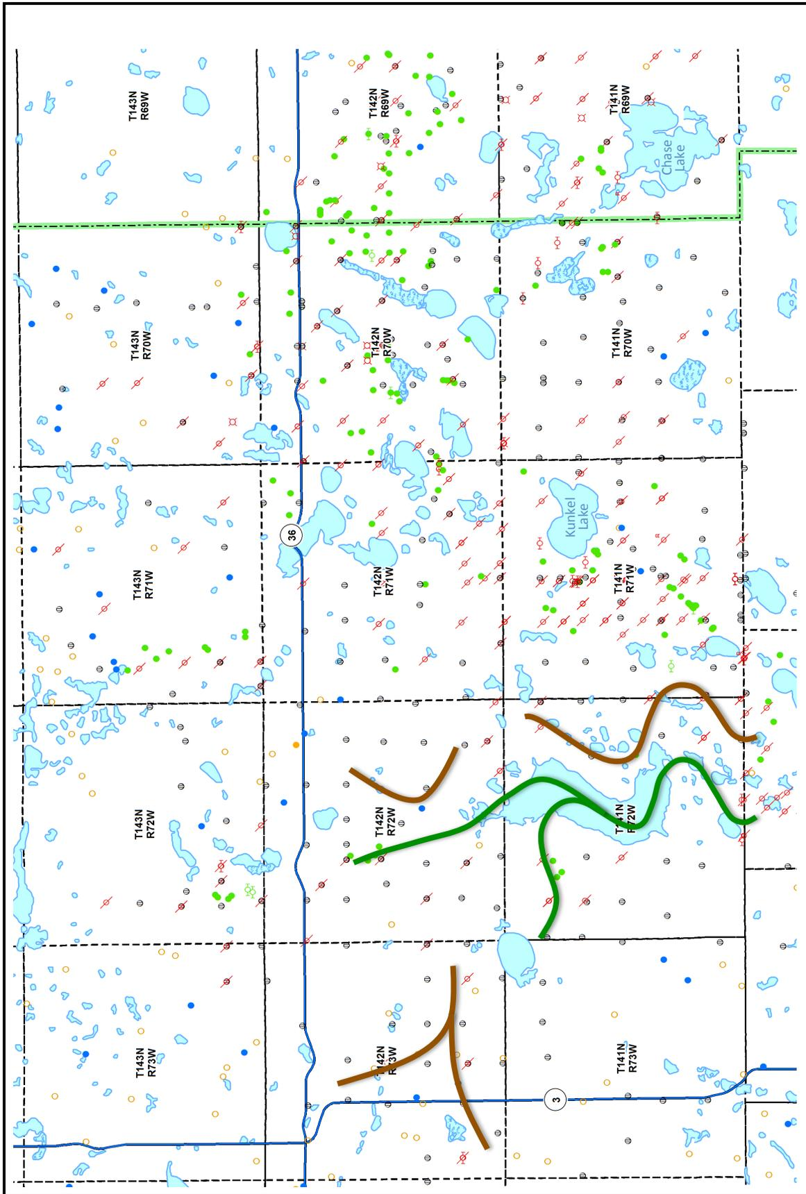
**Figure 9.** Approximate longitudinal axes of buried meandering stream deposits in the Horsehead Lake area. The middle aquifer (axes shown in green) lies at an elevation of approximately 1650-1710 ft. The western branch of the lower aquifer (axes shown in brown) is found at 1560-1650 ft. Notice that Horsehead Lake follows the meanders in these buried channel deposits.
