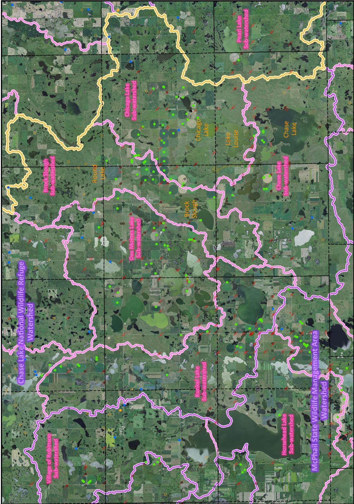
**Figure 15.** Basin and watershed boundaries. The yellow line separates the HUC8 Apple Creek and Pipestem River sub-basins. The purple lines delineate HUC10 watersheds, and the pink lines separate HUC12 sub-watersheds. According to the water level data summarized on Figure 14, groundwater east of Round Lake and Brock Slough and west of the Apple / Pipestem sub-basin divide eventually discharges to Chase Lake.
