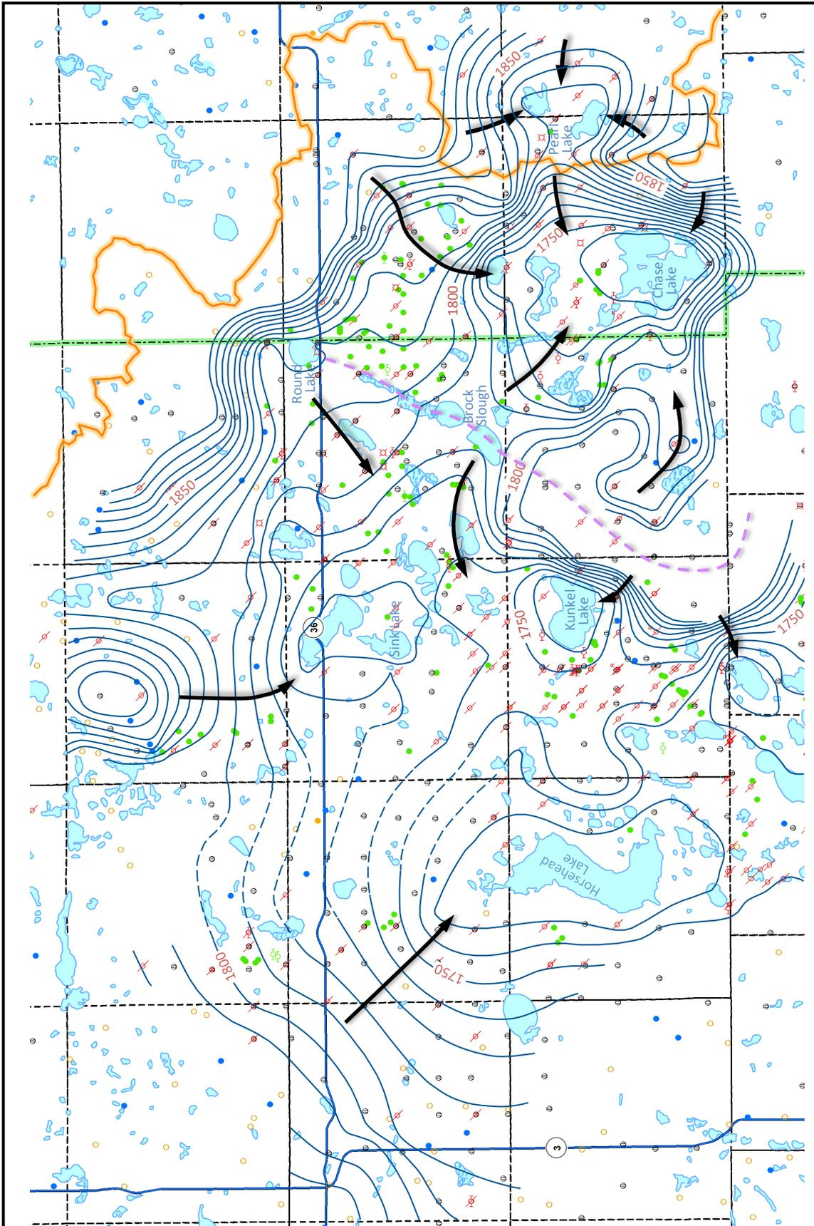
**Figure 14.** Potentiometric surface for the upper aquifer (April 2010). Black arrows indicate the direction of groundwater flow. Note the presence of two major groundwater divides: the Apple Creek / Pipestem River sub-basin divide shown in orange, and a northeast-southwest trending divide shown in purple. The latter divide is caused in part by the arcuate recessional moraine west of Chase Lake (Figure 4).
