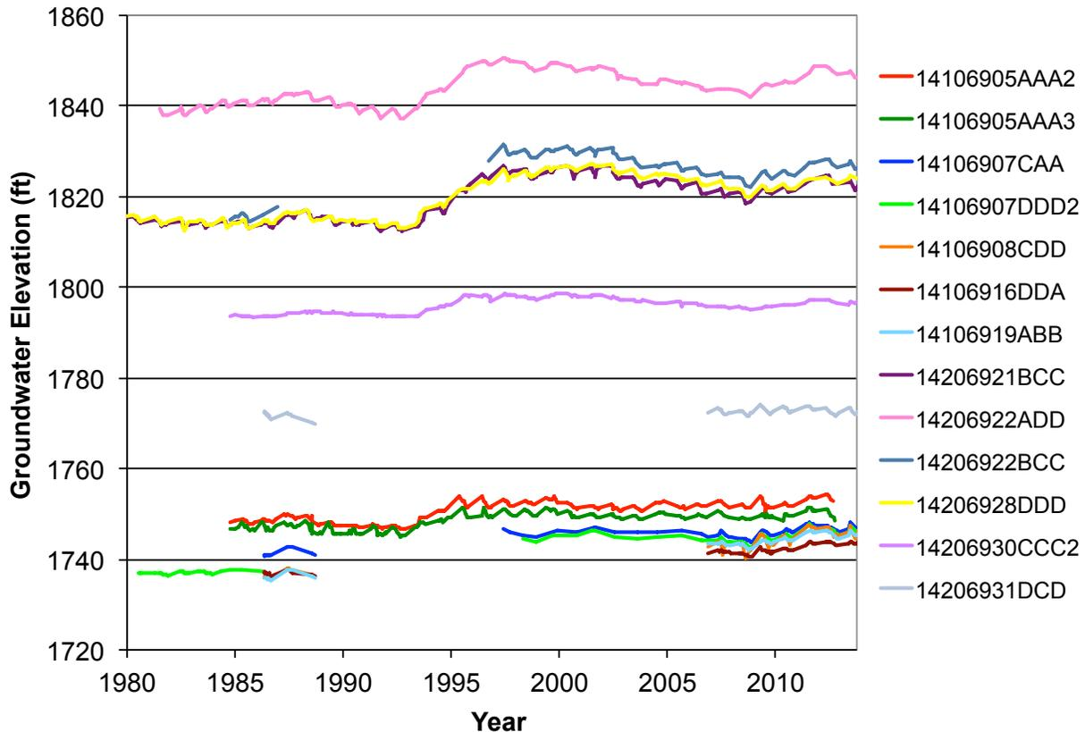
**Figure 16.** Hydrographs for the 13 upper aquifer wells in Chase Lake (T141N R69W) and Marstonmoor (T142N R69W) Townships that have water level records in the 1980s. The chart shows that water levels increased significantly in the mid- to late-1990s, and they are not significantly affected by irrigation.
