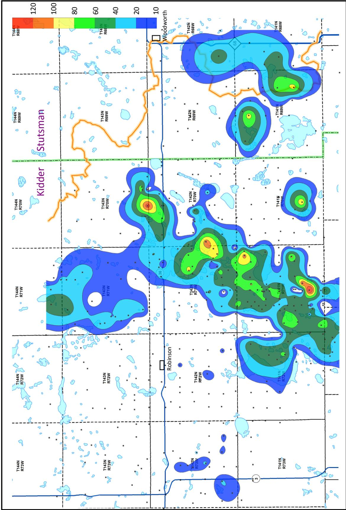
**Figure 7.** Thickness of sand and gravel (feet) in the lower aquifer. Orange line is the eastern boundary of the Apple Creek sub-basin. The lower aquifer in T141N R70W may be connected to the main body of the lower aquifer in T141N R71W.
