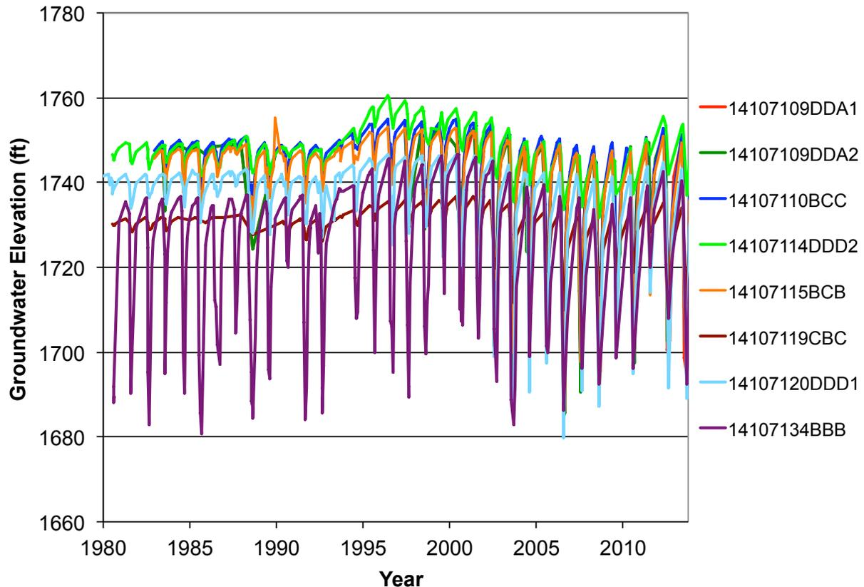
**Figure 22.** Hydrographs for the eight lower aquifer wells in Buckeye Township (T141N R71W) with water level records in the 1980s. Although seasonal drawdowns can exceed 60 feet, annual changes in springtime water levels are typically less than one foot per year, and springtime water levels are as high or higher today than they were 30 years ago.
