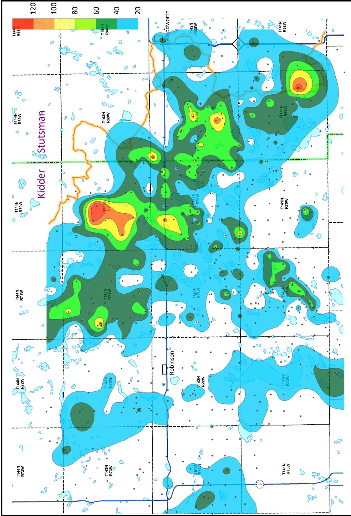
**Figure 6.** Saturated thickness of sand and gravel (feet) in the upper aquifer. The map includes sand and gravel deposits that lie between the upper and lower aquifers. Black dots represent data locations. Orange line is the Apple Creek / Pipestem River sub-basin divide.
