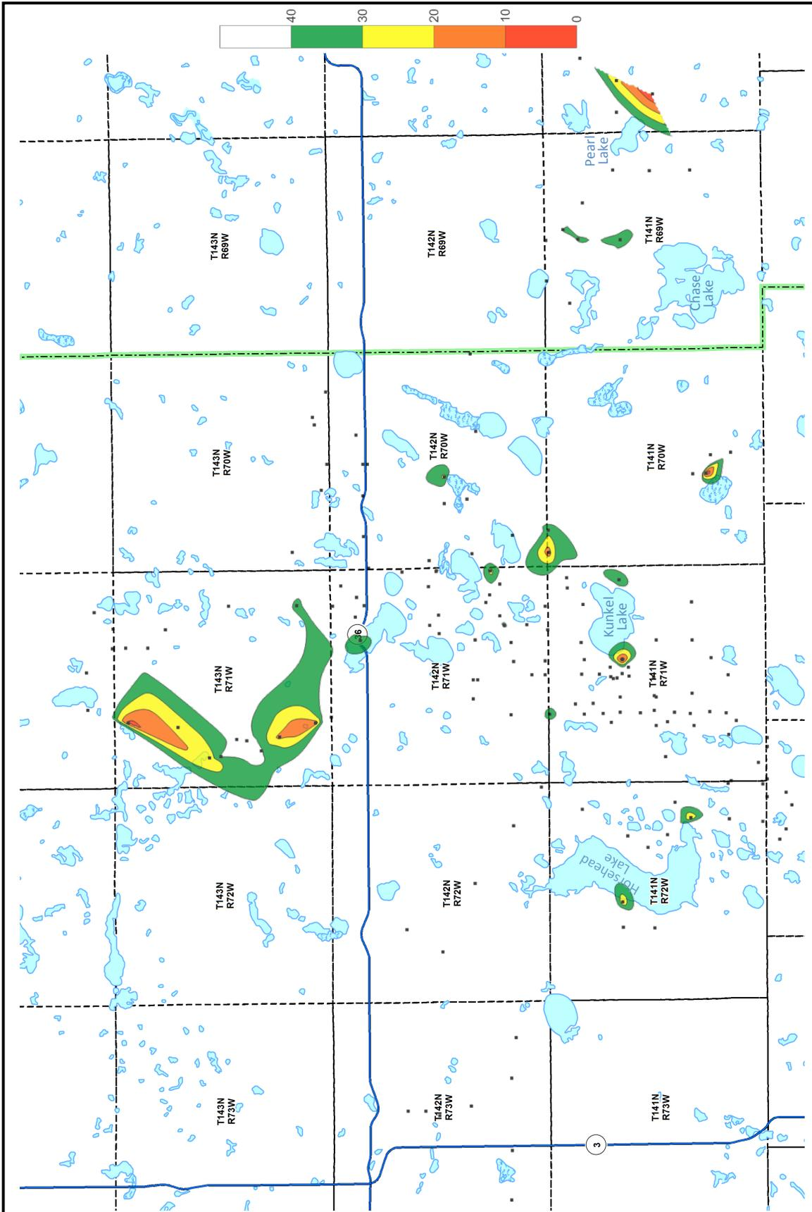
**Figure 13.** Aquitard thickness. Black dots are test hole or well locations where both the upper and lower aquifers are present. Colored contours delineate areas where the total thickness of silt and clay between the aquifers is less than 40 feet. These areas contain several of the known and probable points of groundwater exchange between the two aquifers.
