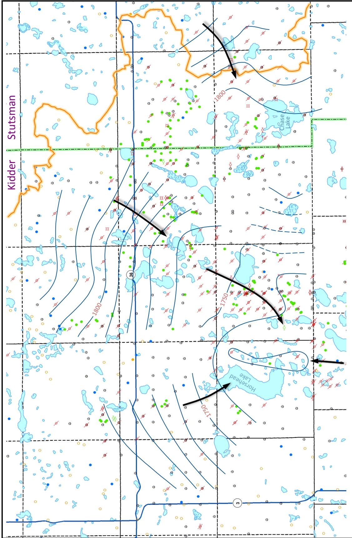
**Figure 19.** Potentiometric surface for the lower aquifer (April 2010). In Stutsman County, the lower aquifer groundwater ultimately discharges to Chase Lake. In Kidder County, the lower aquifer groundwater discharges to the middle aquifer that lies roughly 22 feet below Horsehead Lake (Figures 9 and 11). If the middle and upper aquifers are connected beneath the lake, the lower aquifer groundwater subsequently discharges to the lake.
