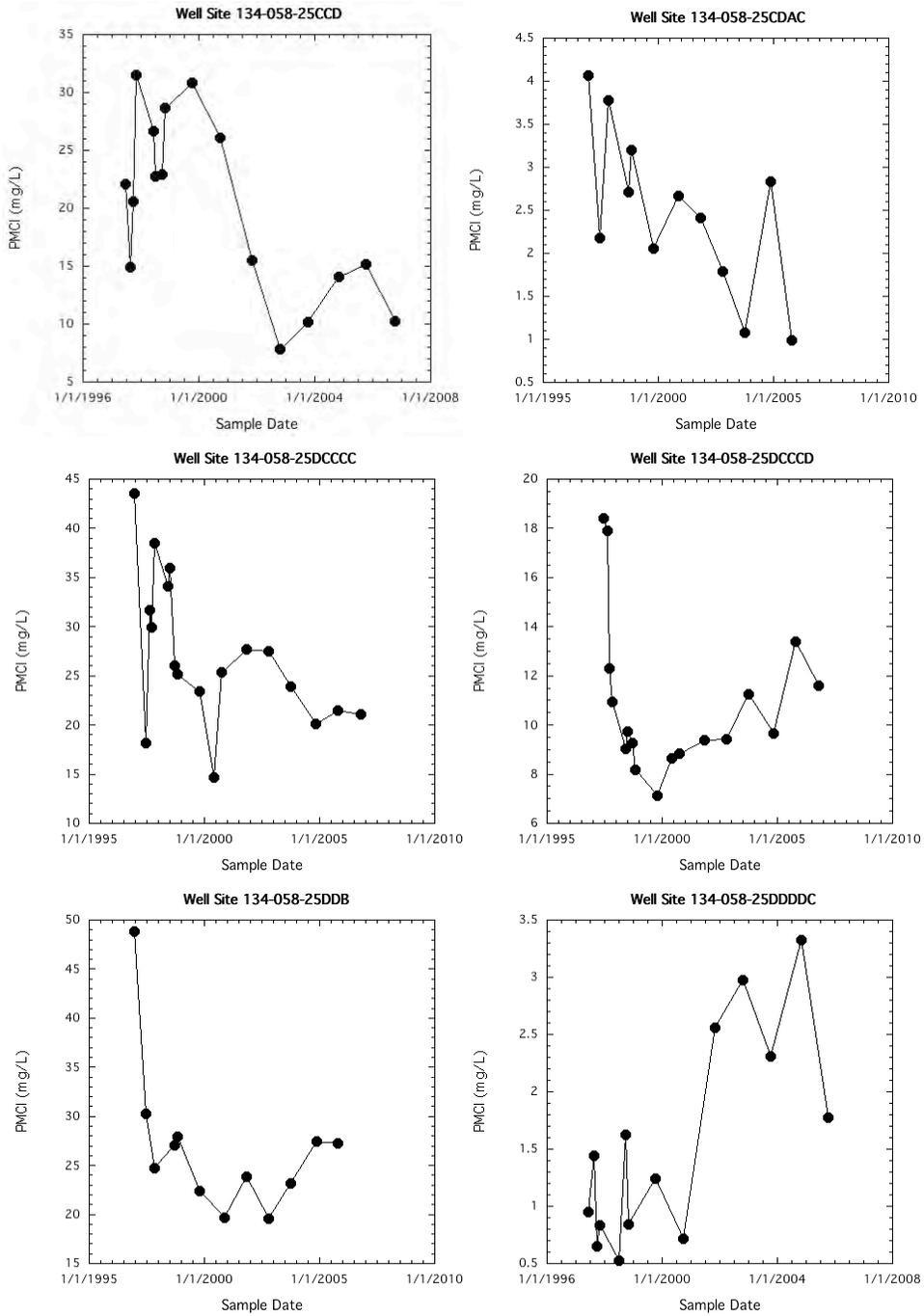
Figure 46. Temporal distribution of Potential Mixed Concentration Index (PMCI) for well sites located in Section 134-058-25.
