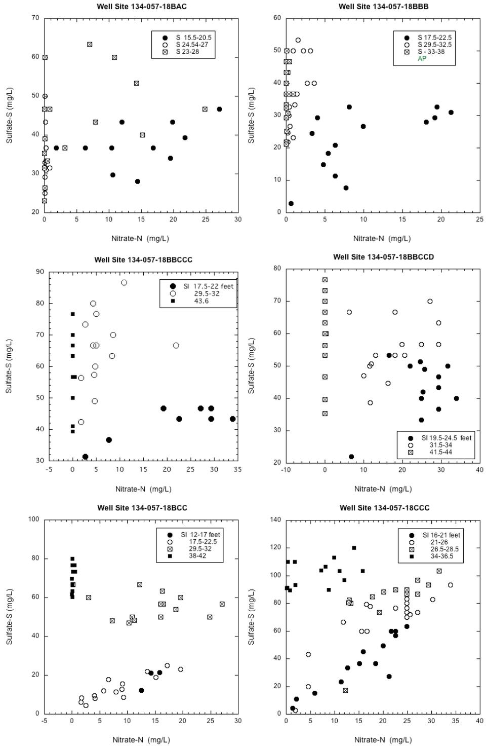
Figure 38. Sulfate-S vs. nitrate-N distribution with time and depth for well sites on 134-057-18.
