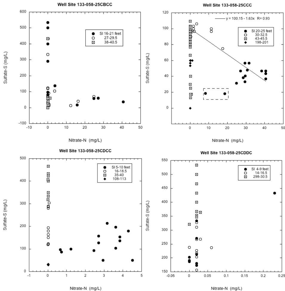
Figure 58. Sulfate-S vs. nitrate-N distribution with time and depth for well sites on 133-058-25.
