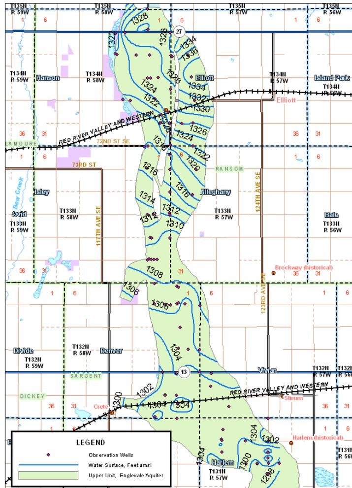
Figure 2. Piezometric map of upper unit of the Englevale aquifer, interpolated from water-level data collected on October 17, 1997.
