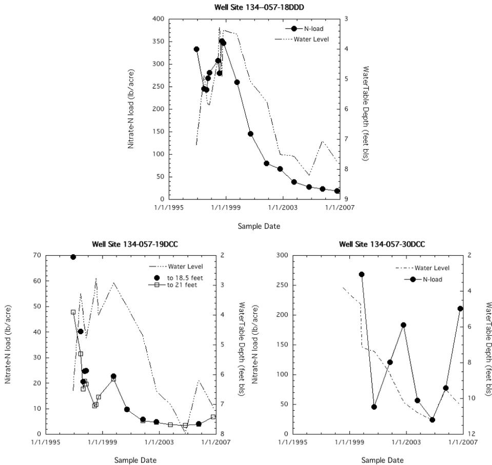
Figure 28. Nitrate-N load trends for Sections 134-057-18DDD, -19DCC and -30DCC well nests.
