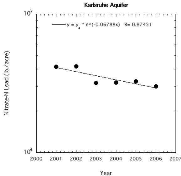
Figure 10. Nitrate-N load dissipation in the Karlsruhe aquifer from 2000 through 2006.
