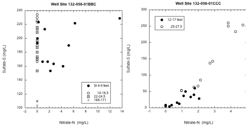
Figure 70. Sulfate-S vs. nitrate-N distribution with time and depth for well sites on 132-058-01.
