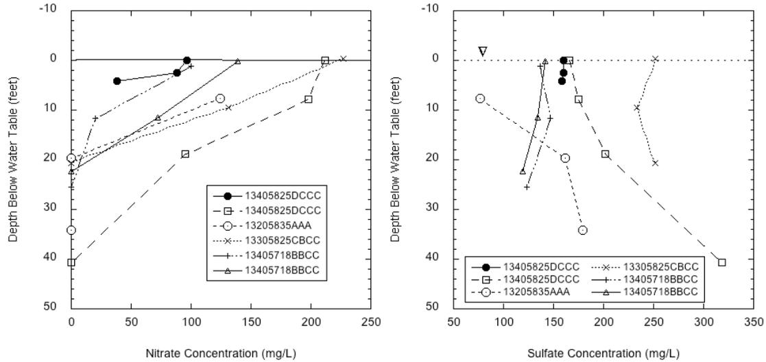
Figure 21. Depth (bwt) profiles for nitrate (as nitrate) concentrations (left), and sulfate (right) on Englevale aquifer sites sampled for isotope analysis.
