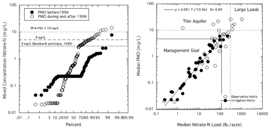
Figure 16. Comparison of probability distributions for pre- and post-1996 nitrate-N mixed concentrations in irrigation wells (left); and comparison of the relationship between toxicological standards and nitrate-N loading rates for irrigation wells and observation wells (right).
