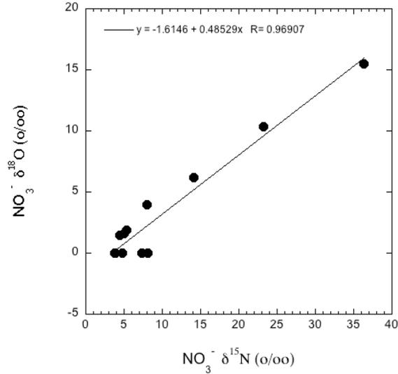
Figure 18. Composite  $^{18}\text{O}$  vs.  $^{15}\text{N}$  data for Englevale Fall 2006 water samples.
