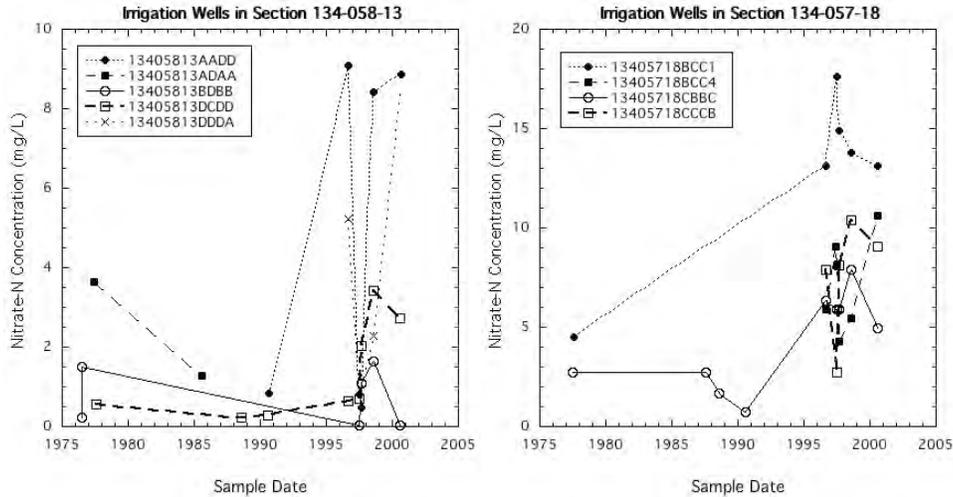
Fig. 24. Temporal variation of nitrate-N concentrations for selected irrigation wells in Sections 134-057-18 and 134-058-13.
