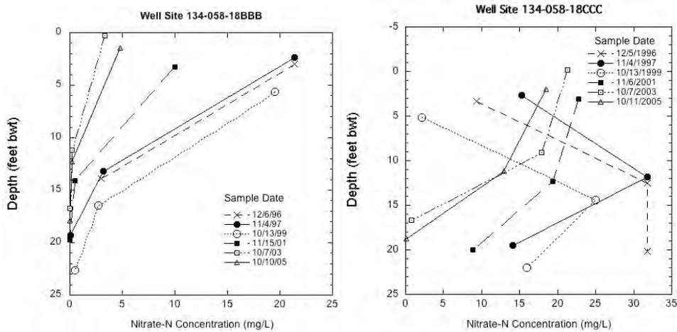
Figure 36. Vertical distribution of nitrate-N concentrations on well sites 134-057-18BBB (left) and -18CCC (right).
