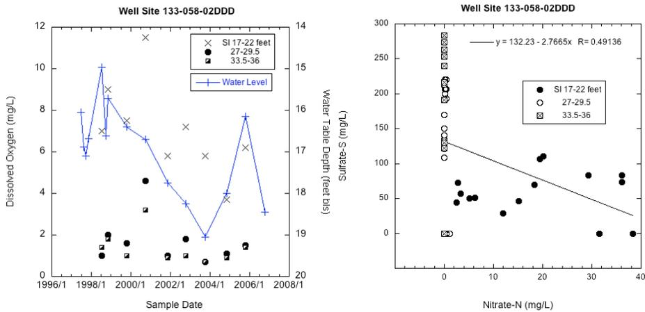
Figure 62. Dissolved Oxygen (left) and sulfate-S distribution (right) with time and depth for well site 133-058-02DDD.
