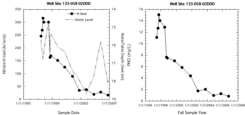
Figure 60. Nitrate-N load (left) and PMCI (right) trends over time for well site 133-058-02DDD.
