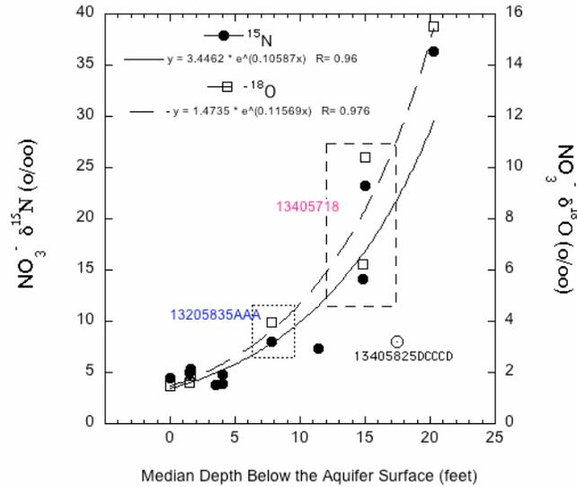
Figure 19. Composite  $^{18}\text{O}$  vs. and  $^{15}\text{N}$  data vs. depth below the water table for Englevale Fall 2006 water samples.
