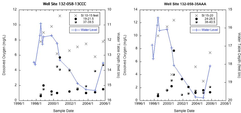
Figure 75. Dissolved Oxygen distribution with time and depth for 132-058-13CCC and 132-058-35AAA well nests.
