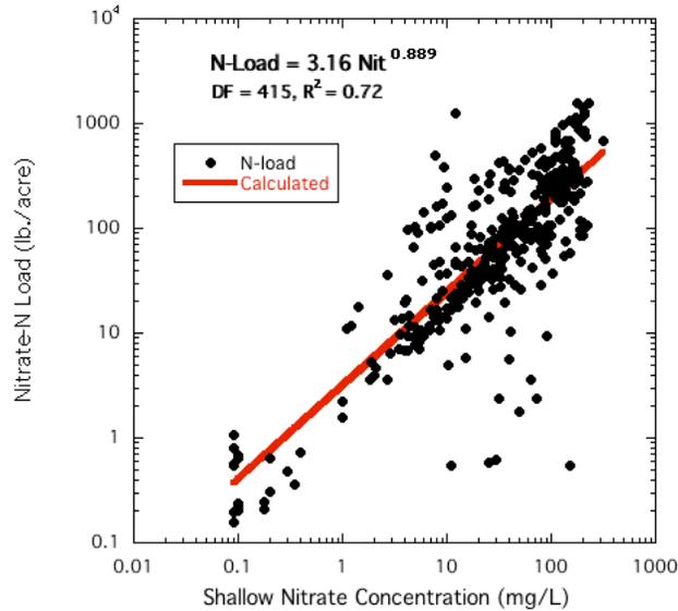
Figure 14. Total nitrate-N load and nitrate concentration in the shallowest well for each measurement on each well site.
