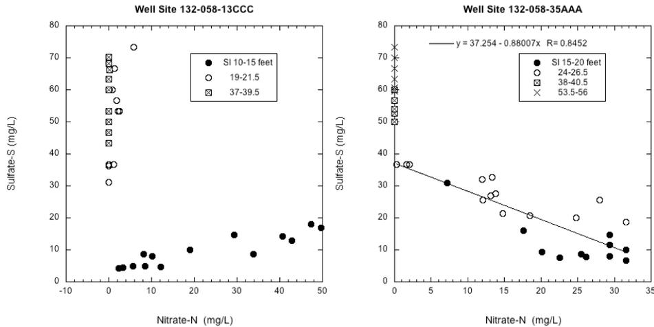
Figure 76. Sulfate-S vs. nitrate-N distribution with time and depth for well nest 132-058-13CCC and 132-058-35AAA.
