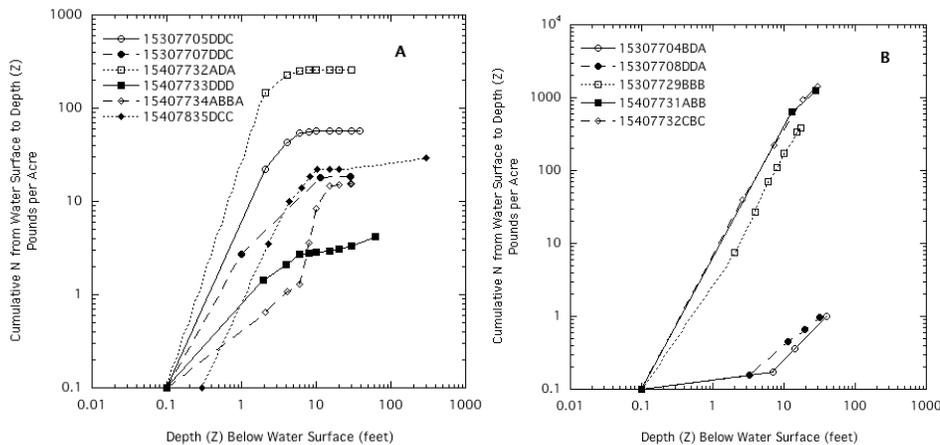
Figure 4. Cumulative nitrate load density with depth, in lb./ac. for: (A) selected multi-port samplers and (B) selected well nests.
