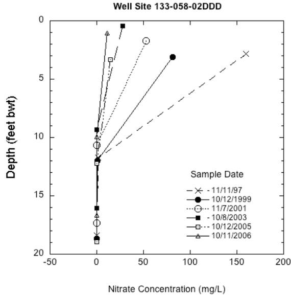
Figure 61. Nitrate concentration depth distribution with time for well site 133-058-02DDD.
