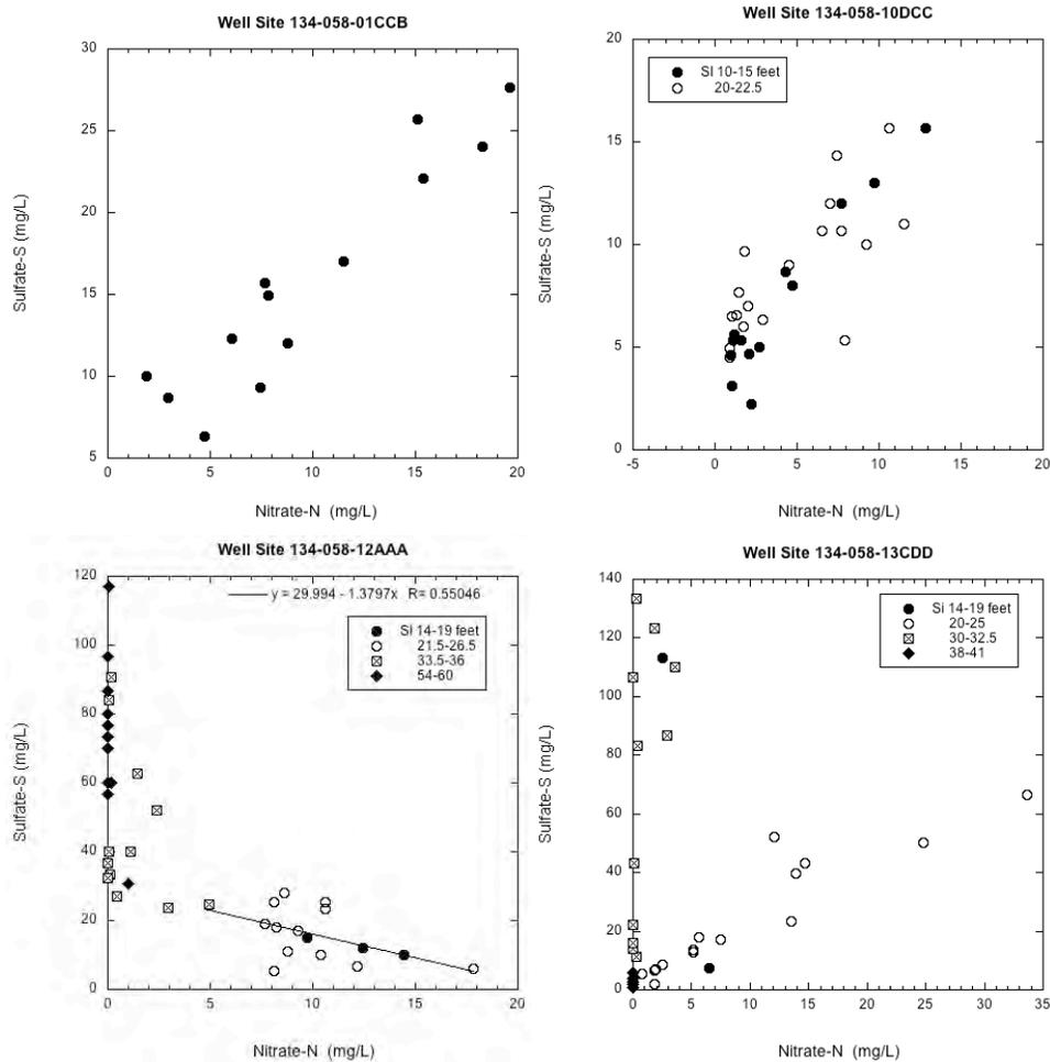
Figure 43. Sulfate-S vs. nitrate-N distribution with time and depth for 134-058, well sites 134-058-01CCB , -10DCC, -12AAA, and -13CDD.
