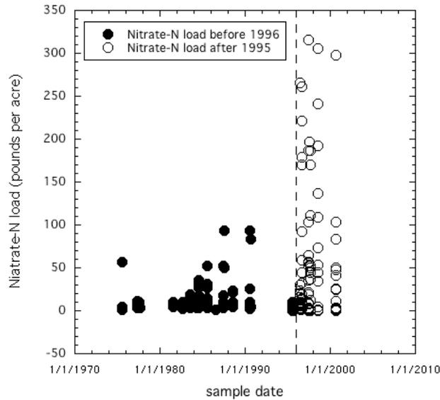
Figure 15. Nitrate-N loads for irrigation wells in the Englevalle aquifer.
