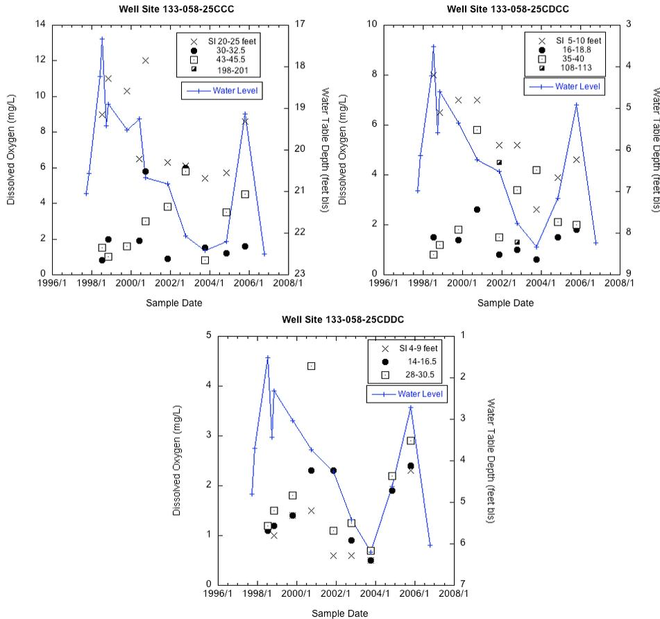
Figure 57. Dissolved Oxygen distribution with time and depth for well sites on 133-058-25.
