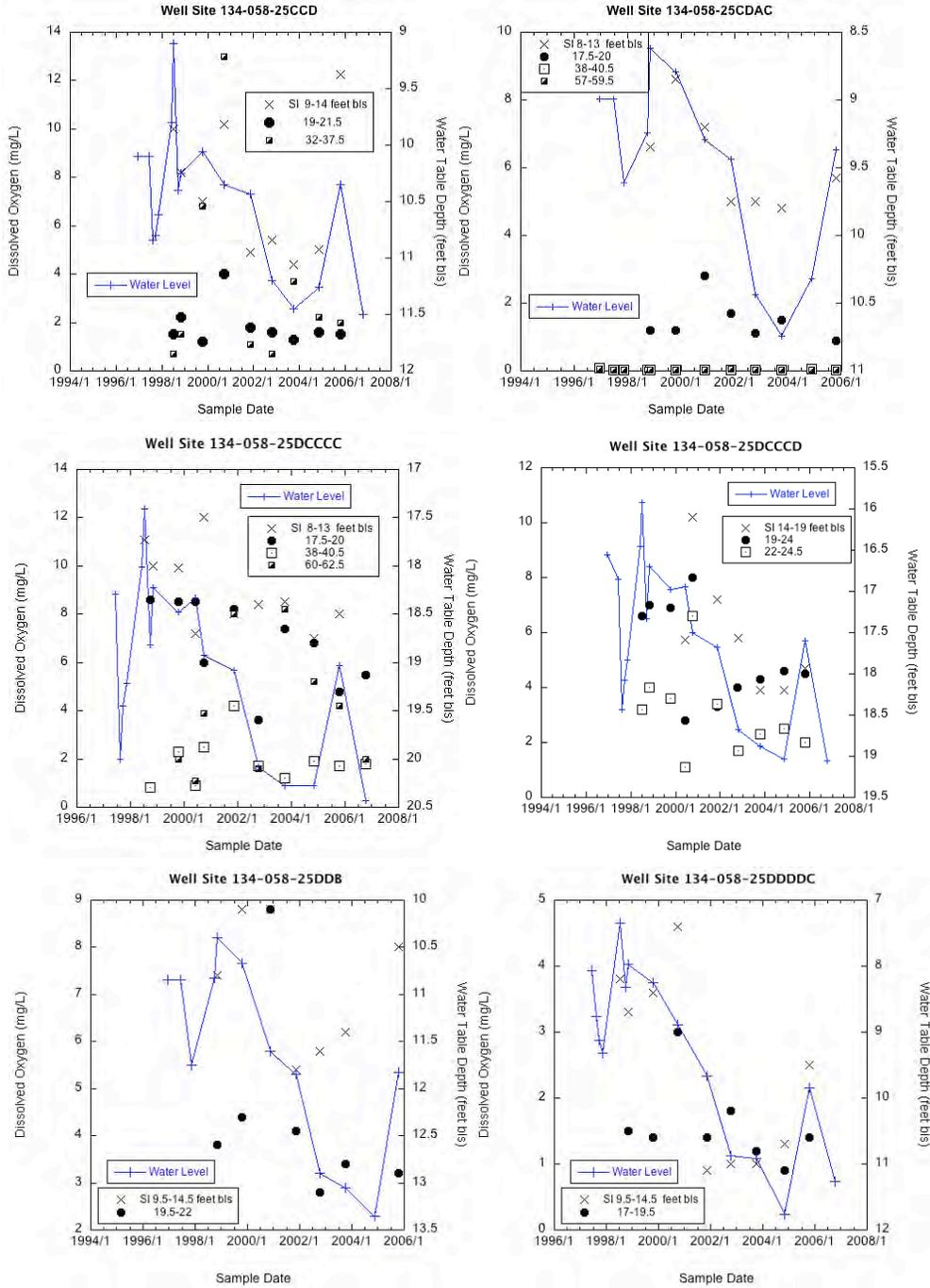
Figure 49. Temporal distribution of dissolved oxygen for well sites located in Section 134-058-25.
