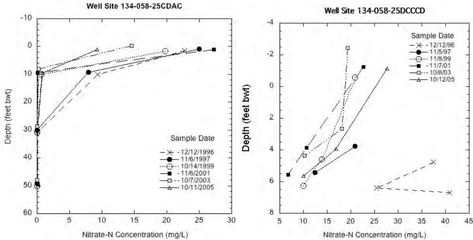
Figure 48. Vertical distribution of nitrate concentrations on well sites 134-058-25CDAC (left) and -25DCCCD (right).
