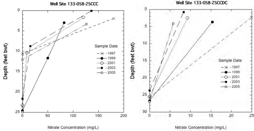
Figure 56. Vertical distribution of nitrate concentrations on well sites 133-058-25CCC (left) and -25CCDC (right).
