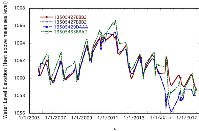
Figure 8. Water level elevations for local observations wells from 2005 through summer, 2017
