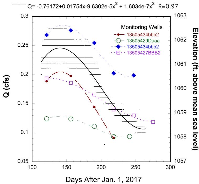
Figure 6. Discharge from the Venlo drain discharge outlet, and elevations for water levels at four local observation wells, April through October, 2017.
