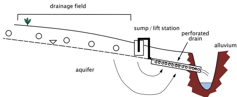
Figure 1. Schematic illustration of uncontrolled drain field discharge through a perforated pipe.
