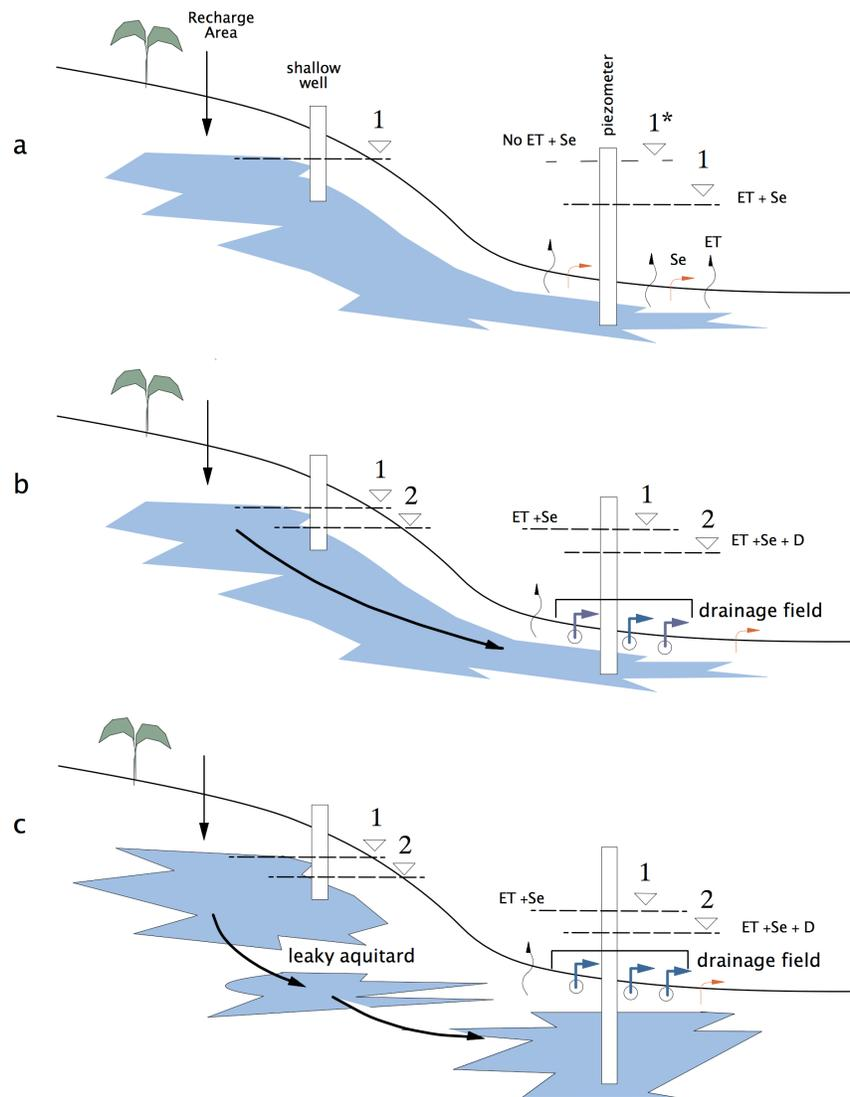
Figure 11. Illustration of potential effects of tile drainage in the discharge area of a confined aquifer having locally artesian pressure head: (a) artesian head without drainage; (b) artesian head with subsurface drains; (c) artesian head with drains in a low transmissivity aquifer.
