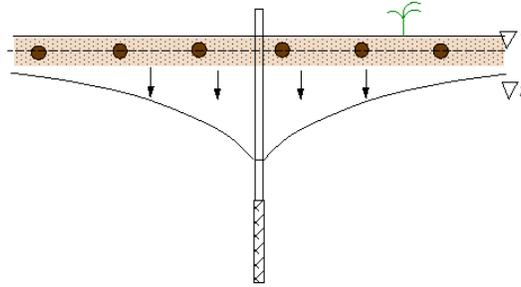
Figure 25. Potential effects of tile drainage in a thin, fine soil layer overlying an unconfined aquifer drawdown and consequent saturated thickness during pumping.
