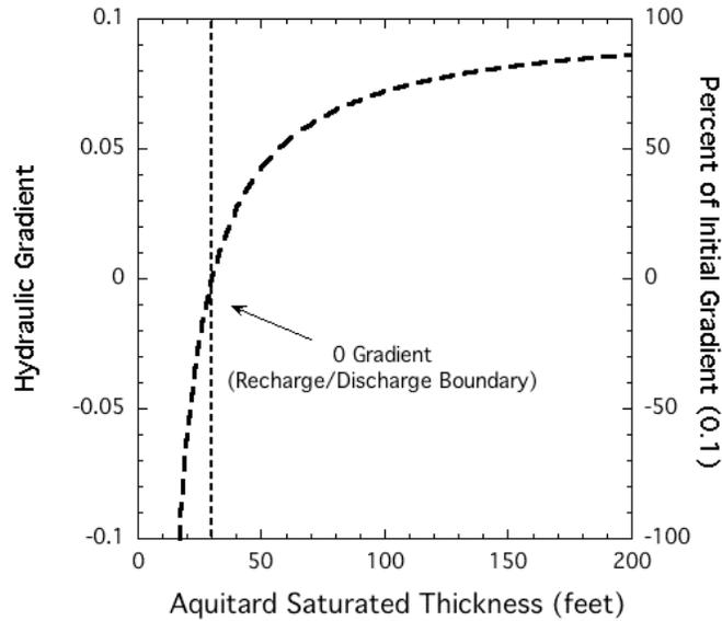
Figure 17. Hydraulic gradient (left vertical axis) and relative gradient (right vertical axis) caused by three feet of drainage drawdown for varying aquitard saturated thicknesses above the aquifer, where the initial hydraulic gradient ( $i$ ) is 0.1.
