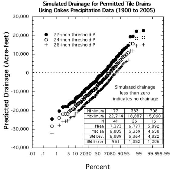
Figure 9. Simulated total state annual drainage distribution based on current (2007) estimated permitted drained acreage, measured 20th century precipitation at Oakes, and drainage thresholds derived from Lamberton, MN (Chung and others 2001) and Waseca, MN (Randall and others 2005) experimental data.
