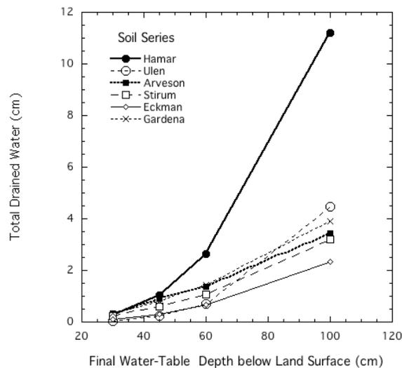
Figure B-6. Incremental drainage to varying depths, from a soil initially saturated to land surface, on six representative soil profiles.
