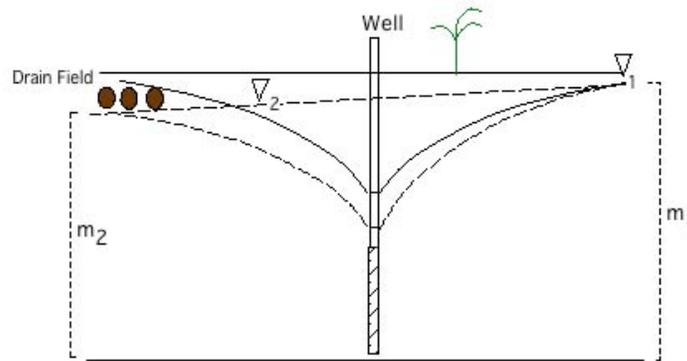
Figure 23. Potential effects of tile drainage in an unconfined aquifer having coarse materials to land surface on drawdown and consequent saturated thickness during pumping.
