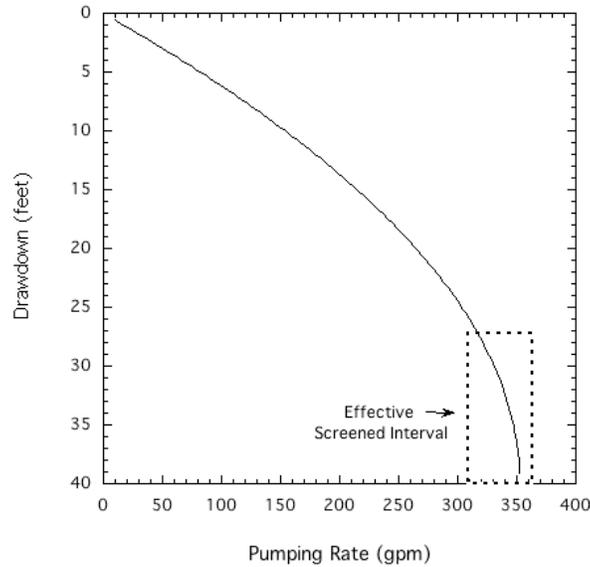
Figure 21. Effect of pumping rate on water-table drawdown at a well.
