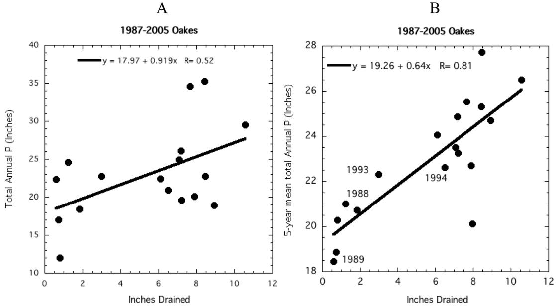
Figure 4. Annual drainage, and five-year mean annual drainage vs. precipitation (P) summary for 1987 through 2005 for the Oakes Test Area of the Garrison Diversion, Dickey County, ND.
