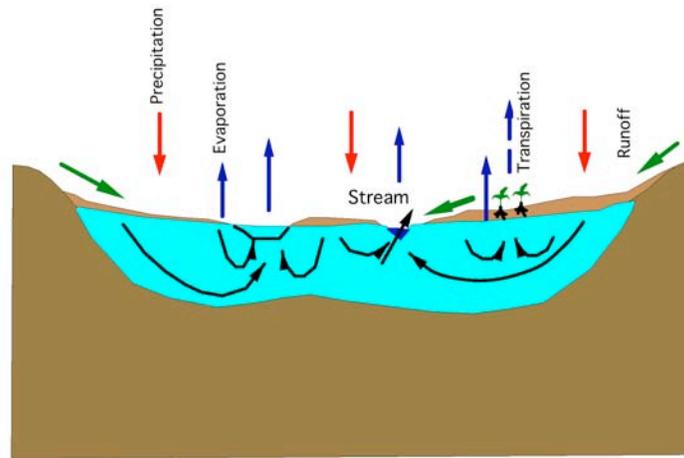
Figure 12. Natural recharge and discharge from an unconfined surficial glacial aquifer.
