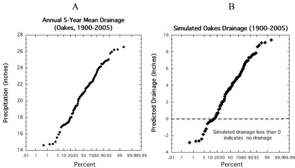
Figure 6. Percent distributions for: (A) 20th century five-year mean annual precipitation at Oakes, ND; and (B) simulated drainage from the Oakes Test Area calculated using the data distribution on (A).
