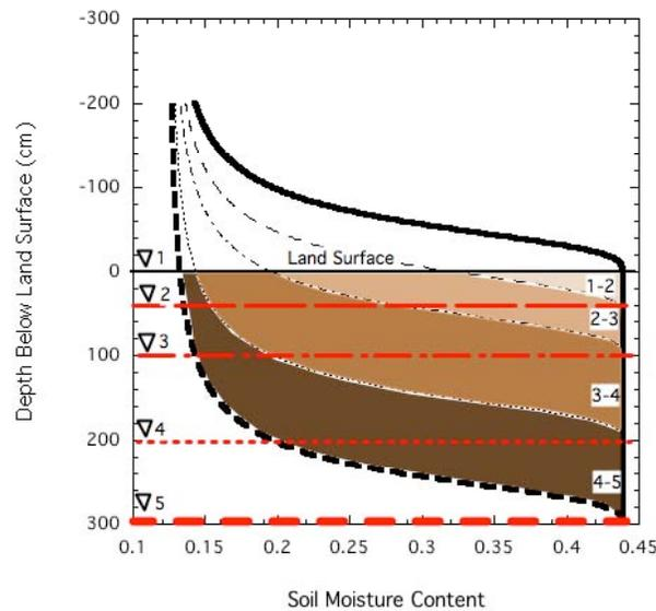
Figure B-3. Illustration of incremental drainage with receding water table from land surface to 50, 100, 200 and 300 cm depths.
