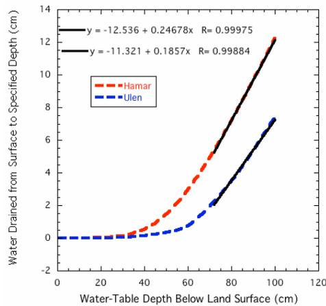
Figure B-4. Cumulative drainage for incremental declines in a water table below land surface.
