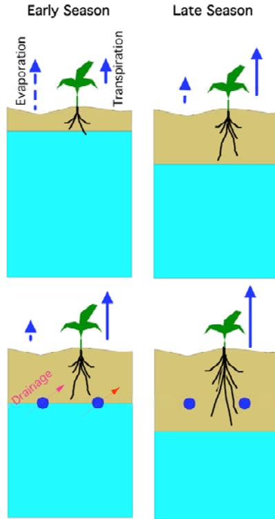
Figure 13. Effects of tile drainage on root extension, evaporation and transpiration.
