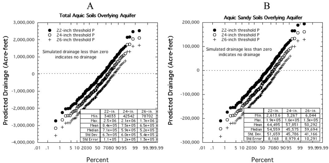
Figure 11. Simulated 20th century distribution of drainage for estimated maximum potential drainage on: (A) all *aquic* soils, and (B) all *aquic* sandy soils overlying aquifers in the 18-county area analyzed.
