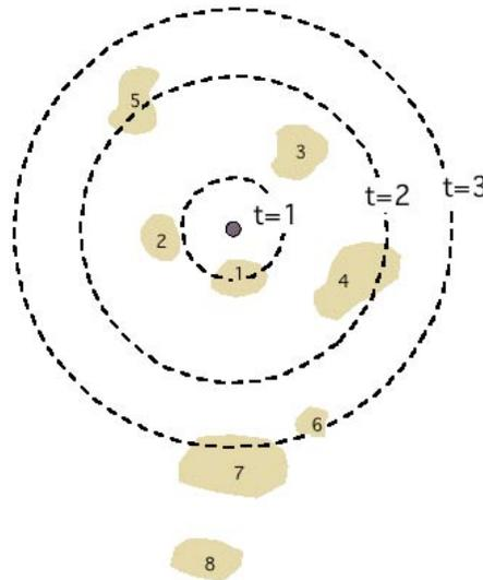
Figure 22. Illustration of time effects on well-operation interactions with evaporative fields.
