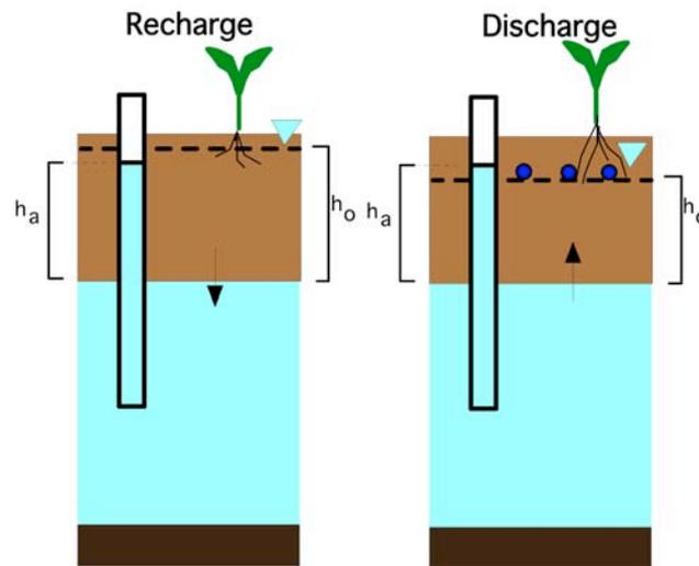
Figure 16. The potential effect of subsurface drainage on local recharge to, or discharge from, a confined aquifer having a piezometric head with elevation close to that of the water table and near land surface.  $h$  is the change in water table (from left to right in the illustration).
