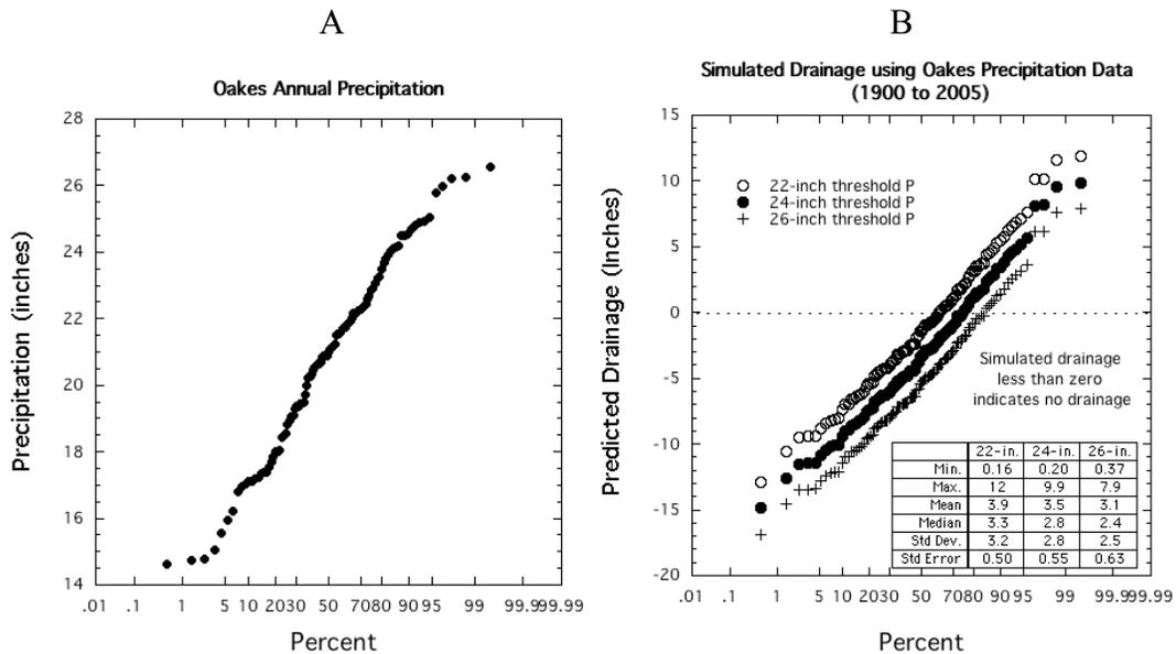
Figure 7. Annual precipitation distribution for 1900 through 2005 at Oakes (A), and the estimated drainage distribution for precipitation thresholds of 22, 24 and 26 inches.
