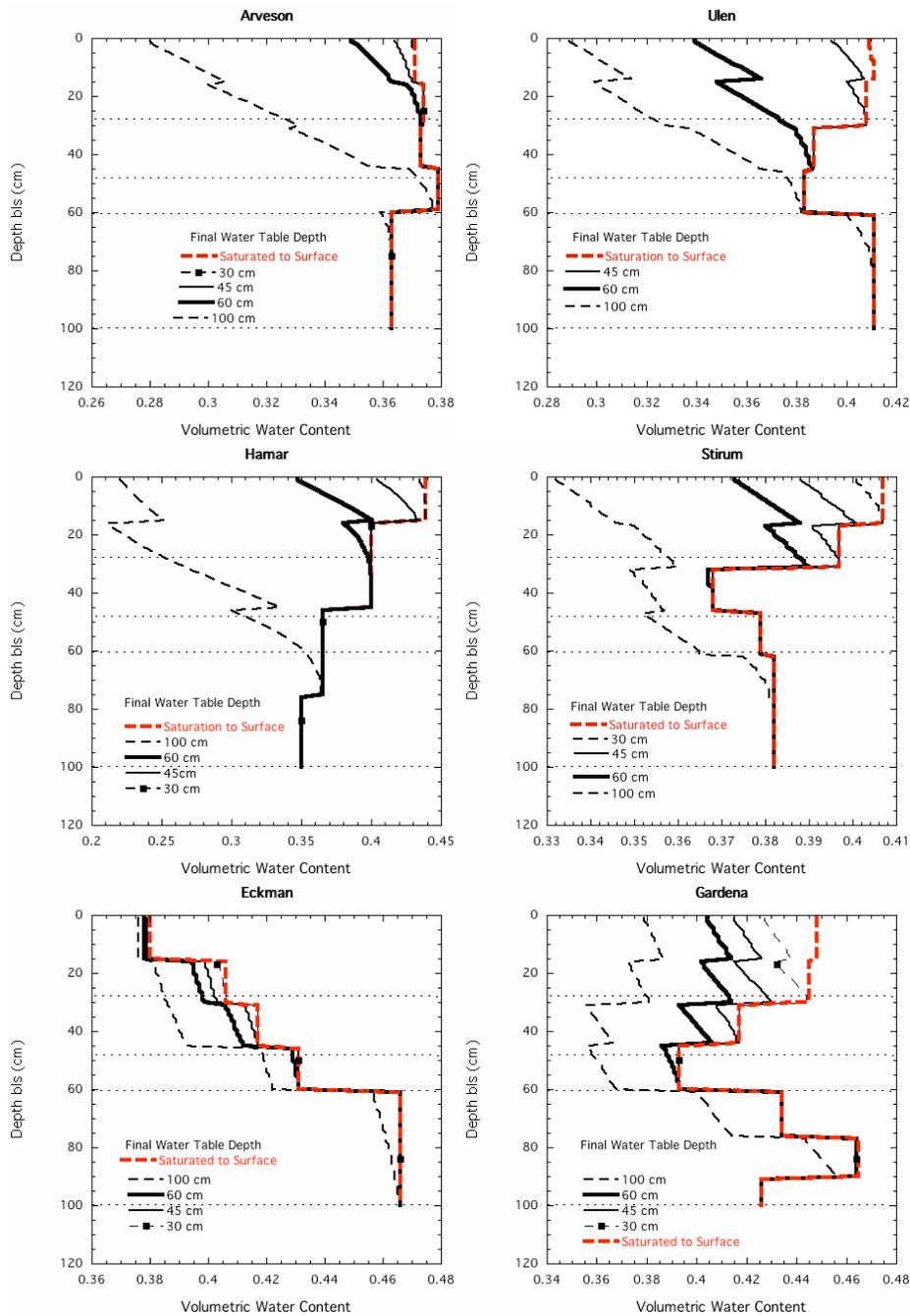
Figure B-5. Equilibrium soil volumetric water content distribution for soil profiles saturated to the land surface, and with water tables at 30, 45, 60 and 100 cm below land surface. Soils illustrated include the Arveson sandy loam, Ulen sandy loam, Hamar loamy sand, Stirum sandy loam, Eckman silt loam, and Gardena loam.
