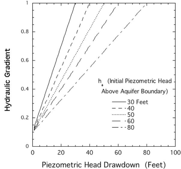
Figure 18. The effect of aquifer pressure drawdown through pumpage on hydraulic gradients governing aquifer recharge through a saturated aquitard of varying thickness, and having an initial gradient ( $i_o$ ) of 0.1.
