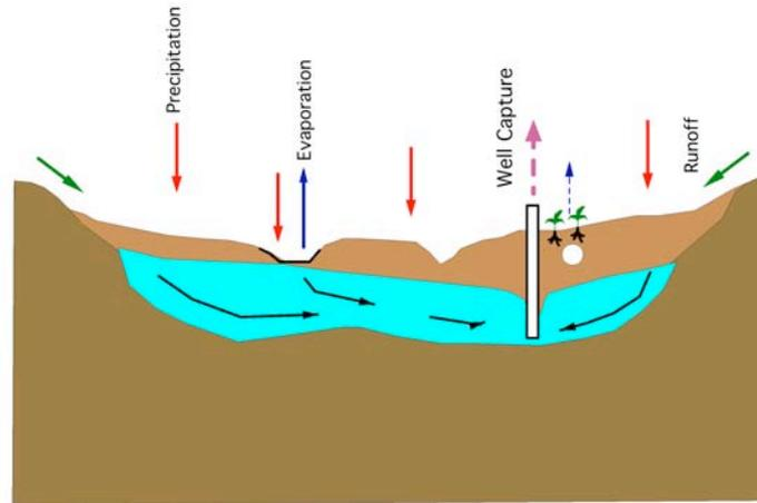
Figure 15. Potential effect of a well field on subsurface drainage and natural discharge.
