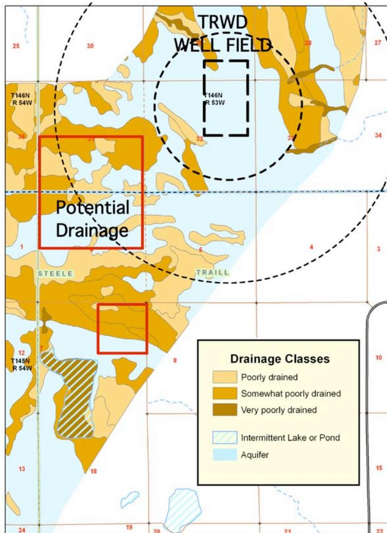
Figure 27. Proposed tile drainage locations and Traill Rural Water District (TRWD) well field in relation to area soil drainage classes. Concentric circles are: inner- half mile radius from well-field center, and outer-mile radius from well-field center. Poorly drained and somewhat poorly drained soils correspond to Calciaquoll and Endoaquoll soils.
