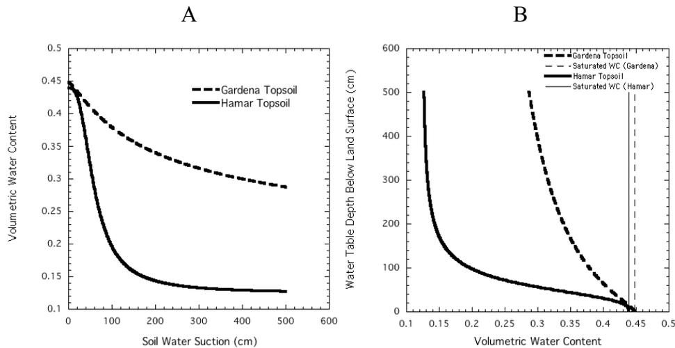
Figure B-2. Comparison of the soil-volumetric moisture-retention vs. pressure-head curve (A) with a homogeneous soil moisture profile above a water table (B).
