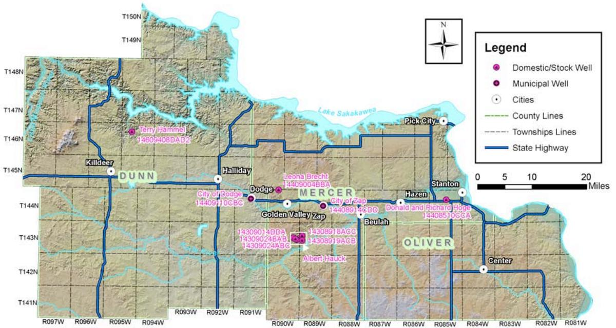
also monitored in 1984 and in 1994. Nine wells are located in low-lying areas along the valleys of Spring Creek, Knife River, and their tributaries where the land surface elevation is lower than the pressure head of the aquifer. One stock well, 146-094-08DAD2, is located in the valley of a Little Missouri River tributary. Pressure heads in three observation wells are measured annually and have been included within this report. The location of the 3 observation wells is shown in Figure 6.
