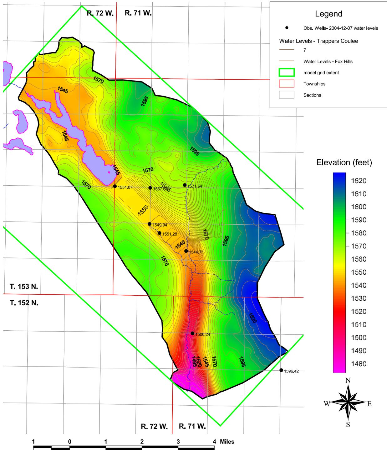
Figure 119. Water table elevations (feet) from steady-state simulation, run B21hh.
