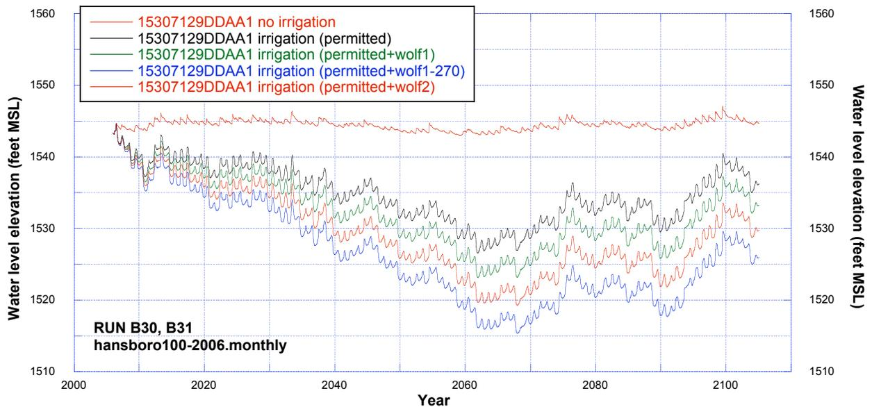
**Figure 157.** Comparisons of simulated water levels at observation well 153-071-29DDAA1 (Trappers Coulee aquifer) using hansboro100-2005.monthly recharge dataset for cases of no irrigation, permitted irrigation, and additional irrigation.
