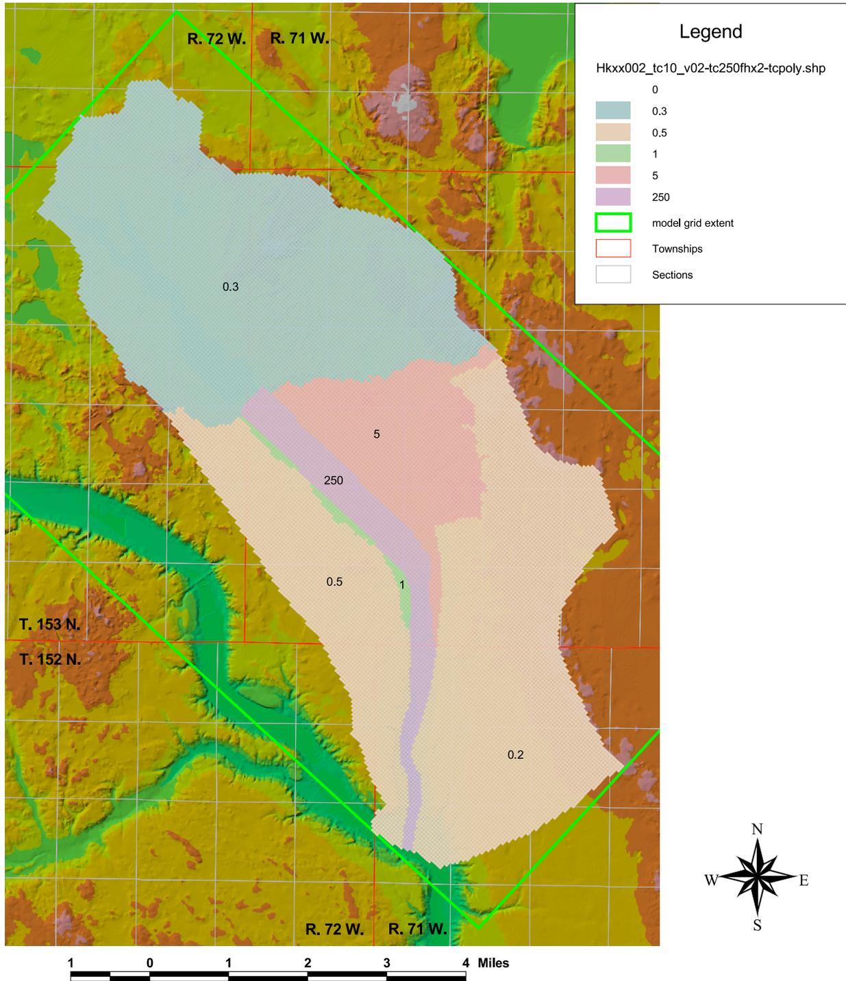
**Figure 115.** Layer 2 hydraulic conductivity (feet per day) for GRID10. File "Volumes/G5data2/esmond/model02outwash/GRID10/hy/HKxx002\_tc10\_v02-tc250fhx2-tc.mf".
