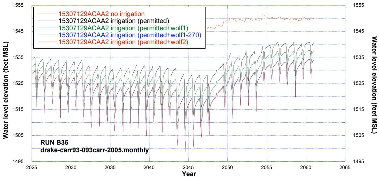
**Figure 159.** Simulated water levels at irrigation well 153-071-29ACAA2 (Trappers Coulee aquifer) using drake-carr93carr-2005.monthly recharge dataset for cases of no irrigation, permitted irrigation, and additional irrigation.
