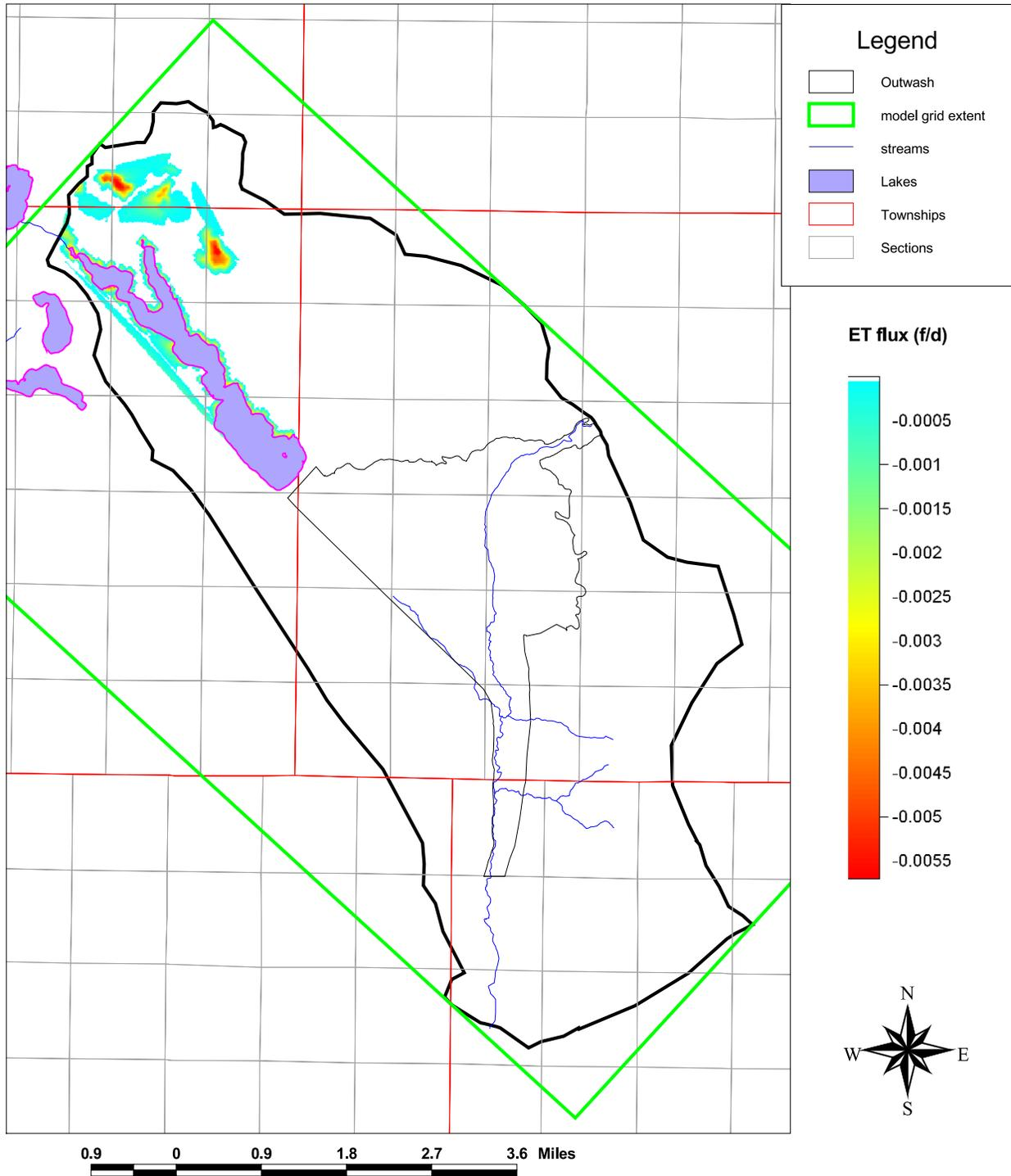
**Figure 124.** Discharge by evapotranspiration (feet per day) in layer 1, steady-state model run B21hh.
