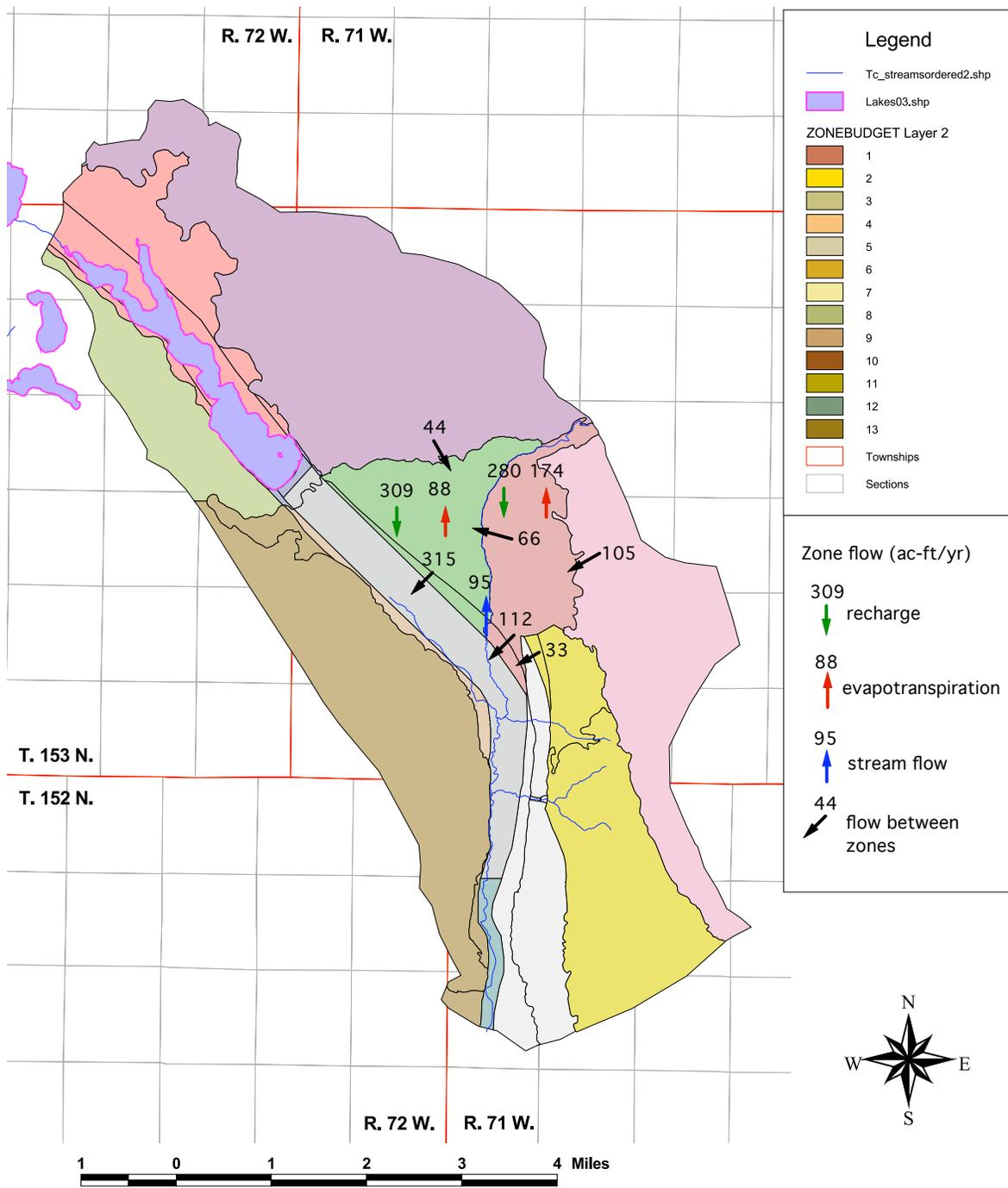
**Figure 126.** Hydrologic budget of the outwash plain of the Trappers Coulee aquifer (ZONEBUDGET zones 04 and 05). Simulation tc10B21hh.
