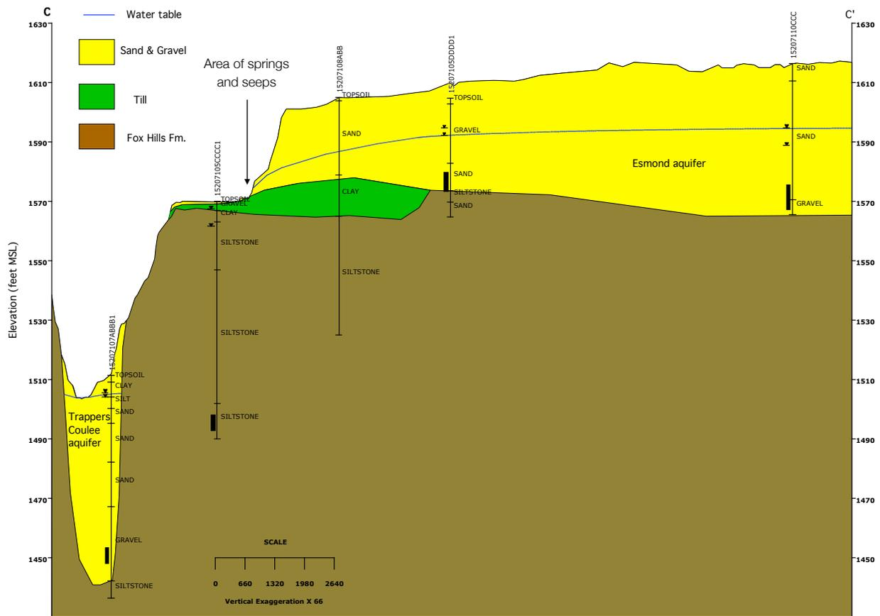
**Figure 10.** Cross-section C-C' of Trappers Coulee and Esmond aquifers.
