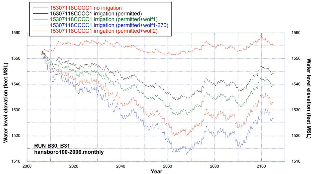
**Figure 155.** Comparisons of simulated water levels at observation well 153-071-18CCCC1 (Trappers Coulee aquifer) using hansboro100-2005.monthly recharge dataset for cases of no irrigation, permitted irrigation, and additional irrigation.
