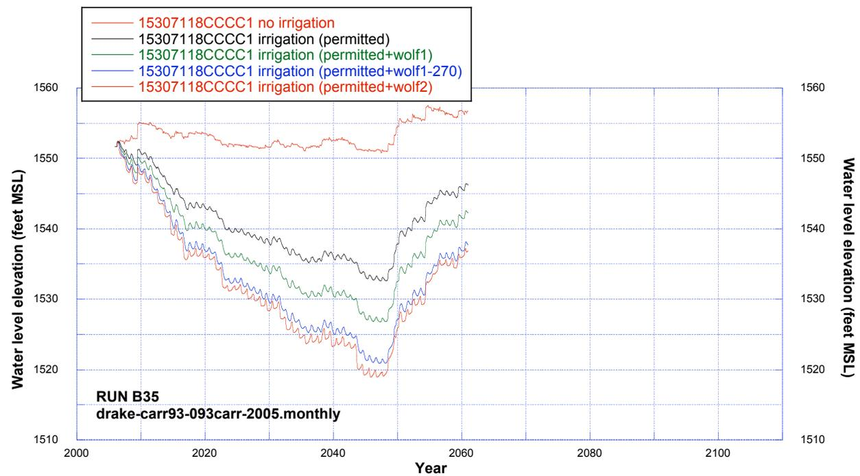
**Figure 139.** Comparisons of simulated water levels at observation well 153-071-18CCCC1 (Trappers Coulee aquifer) using drake-carr93carr-2005.monthly recharge dataset for cases of no irrigation, permitted irrigation, and additional irrigation.
