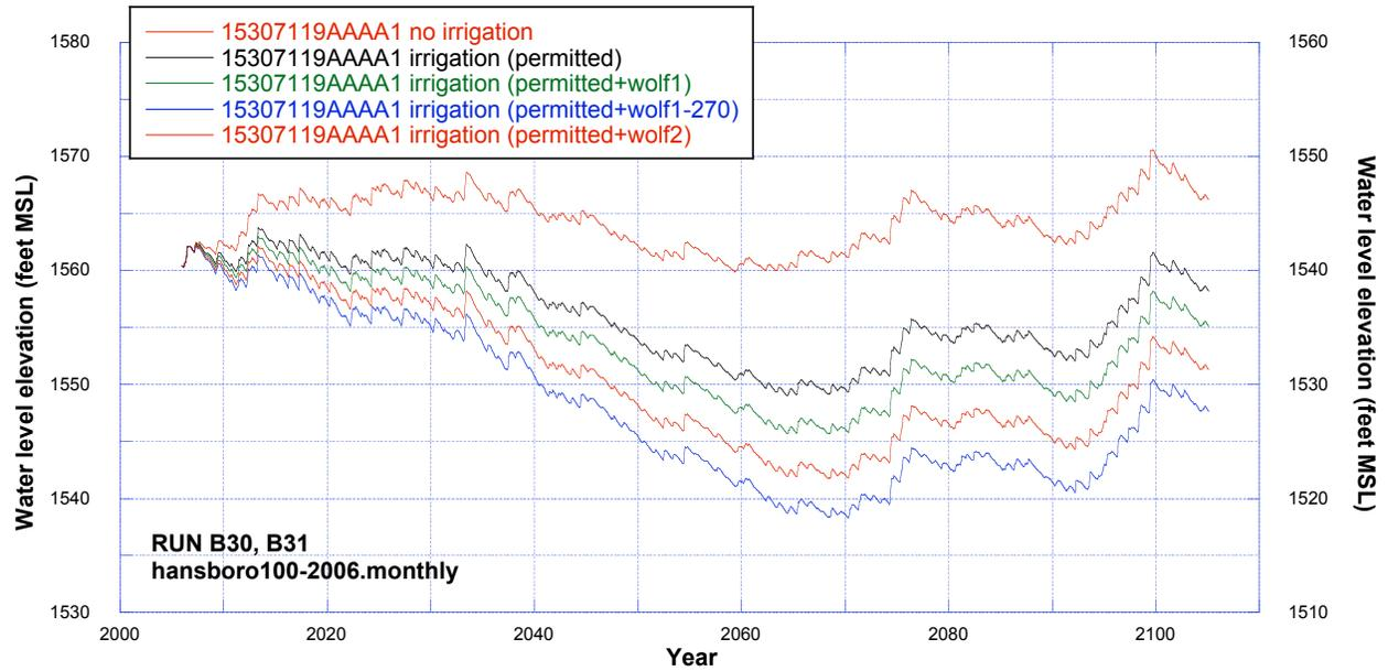
**Figure 154.** Comparisons of simulated water levels at observation well 153-071-19AAAA1 (Fox Hills aquifer) using hansboro100-2005.monthly recharge dataset for cases of no irrigation, permitted irrigation, and additional irrigation.
