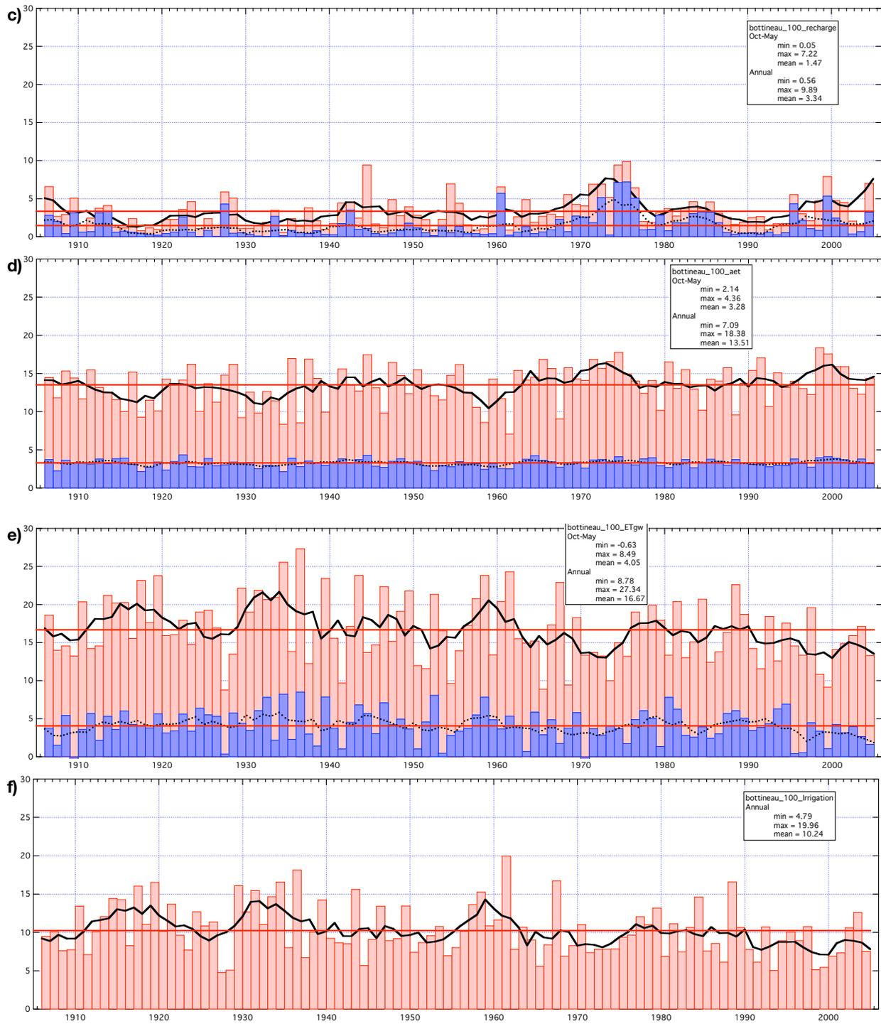
**Figure 98 continued.** Long-term stress period VB2K run bottineau\_100. **a)** precipitation, **b)** PET, **c)** recharge, **d)** AET, **e)** ETgw, and **f)** irrigation water use per acre. All data in inches per year.
