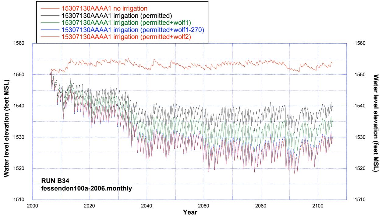
**Figure 152.** Comparisons of simulated water levels at observation well 153-071-30AAAA1 (Trappers Coulee aquifer) using fessenden100a-2005.monthly recharge dataset for cases of no irrigation, permitted irrigation, and additional irrigation.
