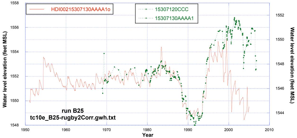
**Figure 134.** Comparison of observed water levels at 153-071-20CCC and 153-071-30AAA1 (replacement well for 153-071-20CCC) with simulated water levels from run B25 (rugby01\_f03.monthly) using reported water use.
