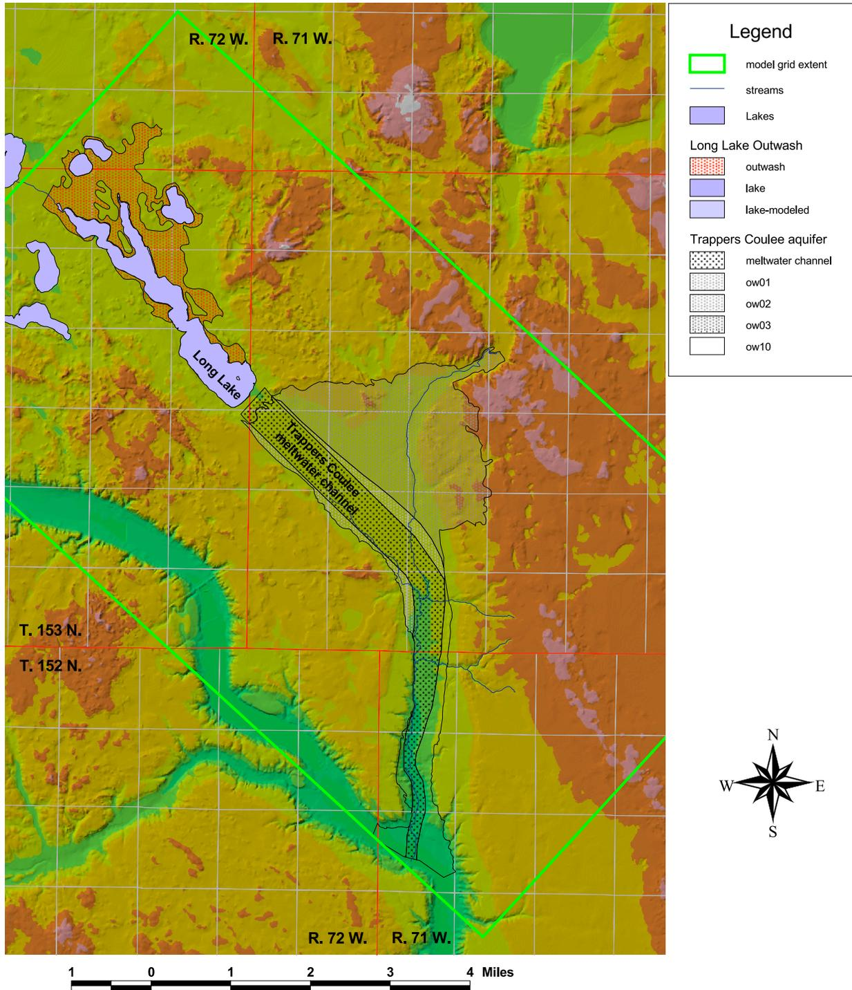
**Figure 104.** Location of outwash and surface hydrology simulated in Trappers Coulee model.
