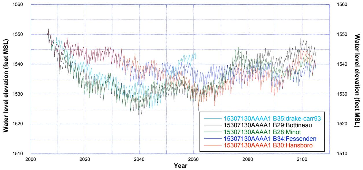
**Figure 137.** Comparisons effects of climate on simulated water levels at observation well 153-071-30AAAA1 using permitted irrigation.
