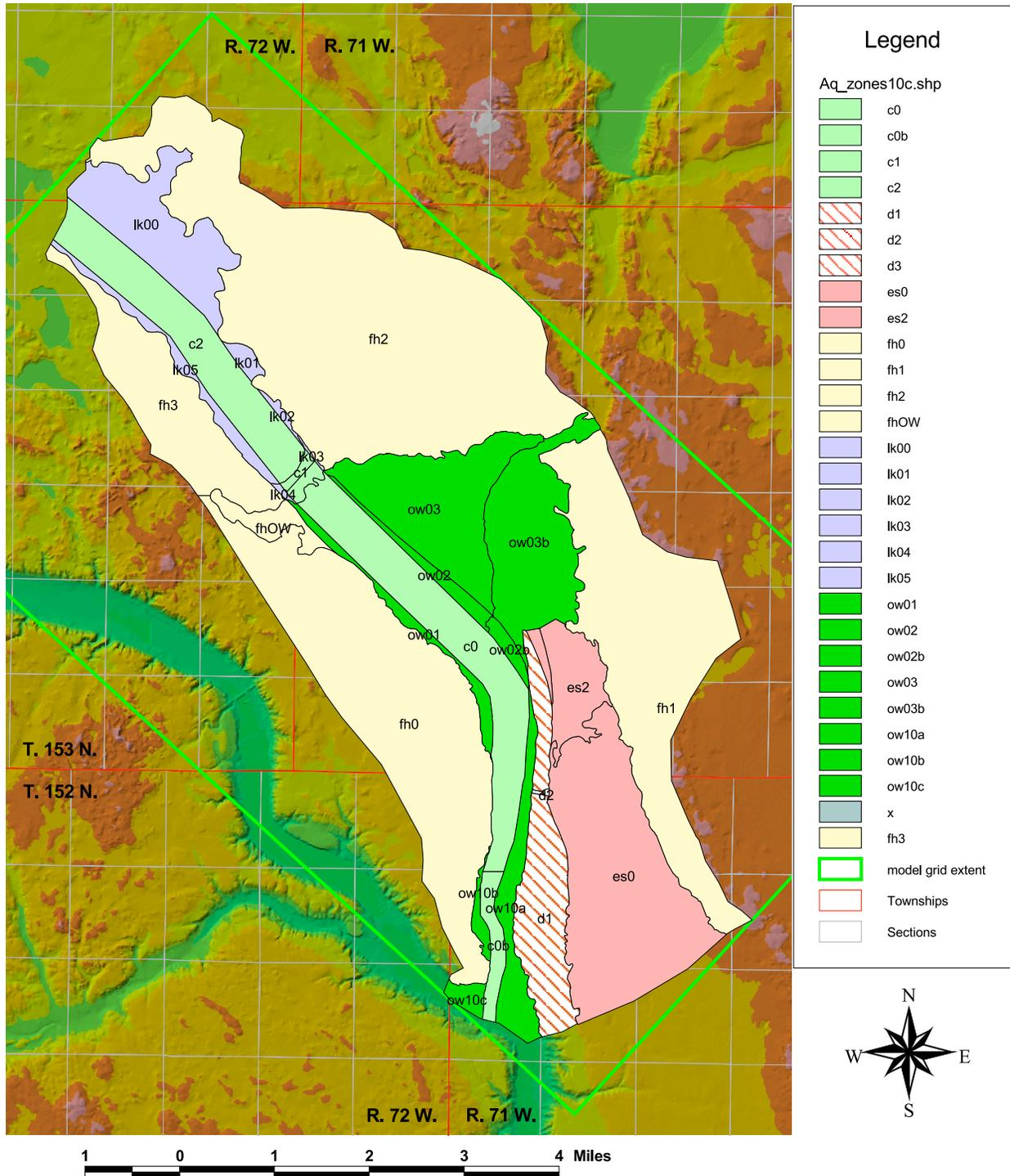
**Figure 110.** Layer 2 hydraulic property zones. Different combinations of property zones were used to assign various hydraulic properties or multipliers to arrays. File “esmond/model02outwash/GRID10/zone/zones/aq\_zones10c.shp”.
