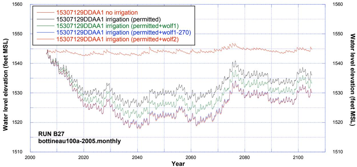
**Figure 145.** Comparisons of simulated water levels at observation well 153-071-29DDAA1 (Trappers Coulee aquifer) using bottineau100a-2005.monthly recharge dataset for cases of no irrigation, permitted irrigation, and additional irrigation.
