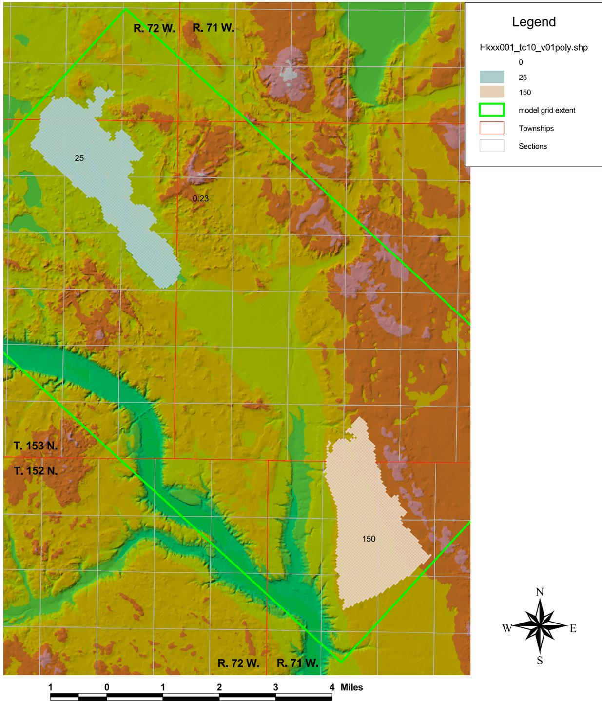
**Figure 111.** Layer 1 hydraulic conductivity (feet per day) for GRID10. File "Volumes/G5data2/esmond/model02outwash/GRID10/hy/HKxx001\_tc10\_v01.mf".
