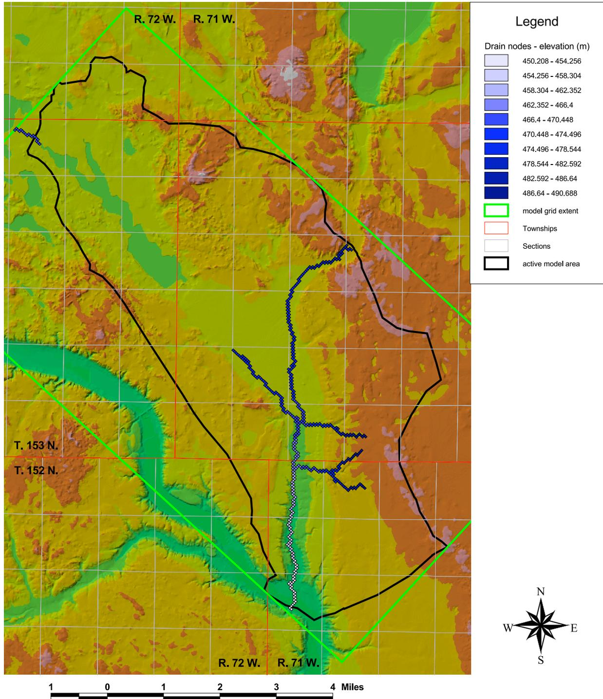
**Figure 117** Location of drain package nodes used to simulate aquifer discharge to Trappers Coulee. Drain nodes were assigned to all model nodes from digitized streams. Those drain nodes outside the active model nodes are inactive.
