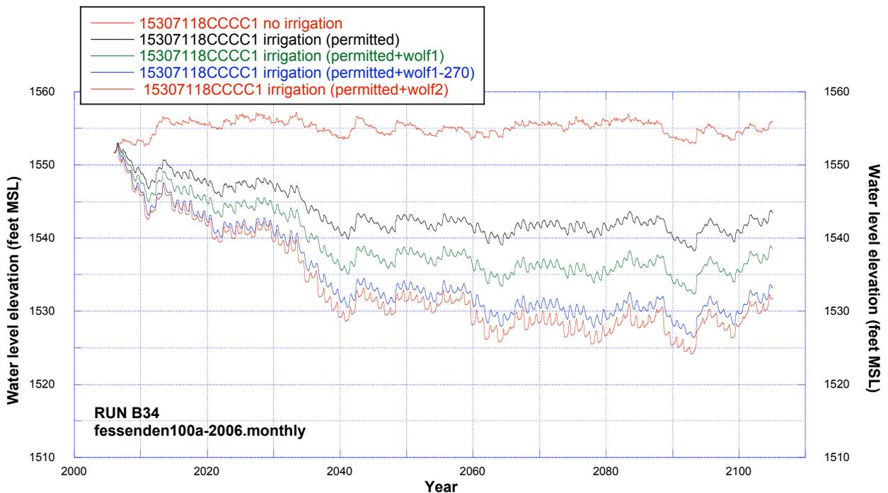
**Figure 151.** Comparisons of simulated water levels at observation well 153-071-18CCCC1 (Trappers Coulee aquifer) using fessenden100a-2005.monthly recharge dataset for cases of no irrigation, permitted irrigation, and additional irrigation.
