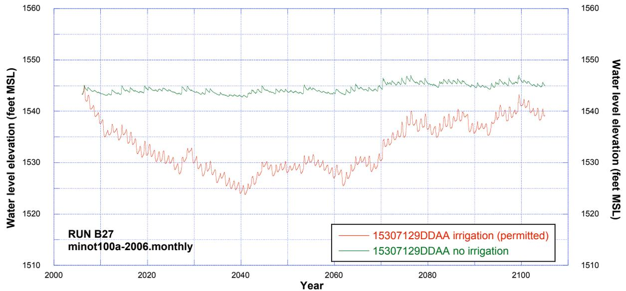
**Figure 149.** Comparisons of simulated water levels at observation well 153-071-29DDAA1 (Trappers Coulee aquifer) using minot100a-2005.monthly recharge dataset for cases of no irrigation and permitted irrigation.
