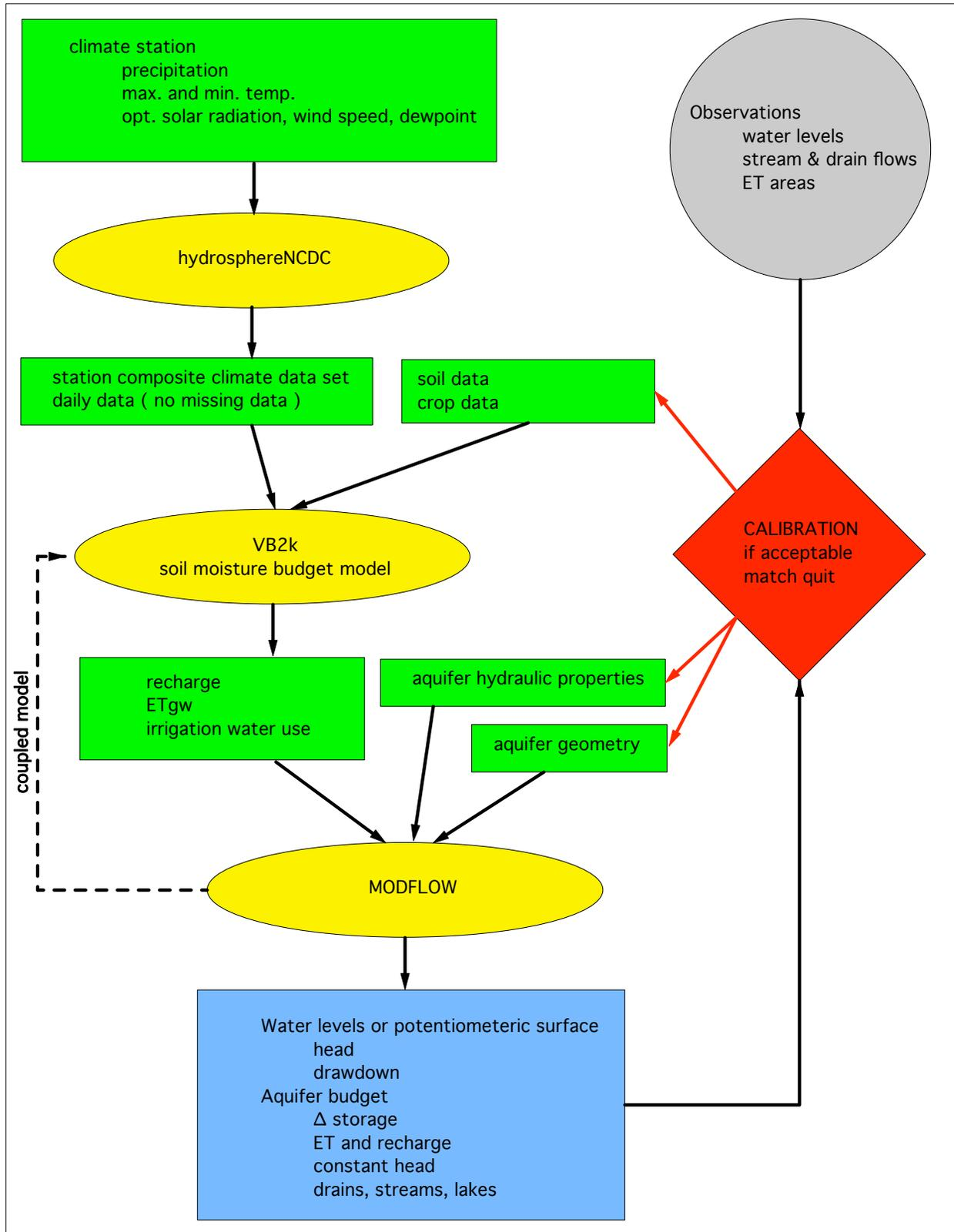
**Figure 103.** Flow chart of modeling process showing input and output.
