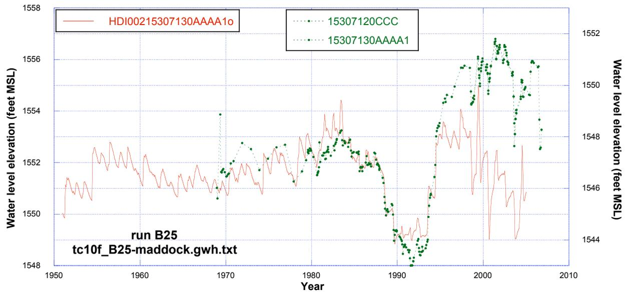
**Figure 135.** Comparison of observed water levels at 153-071-20CCC and 153-071-30AAA1 (replacement well for 153-071-20CCC) with simulated water levels from run B25 (maddock02\_f03.monthly) using reported water use.
