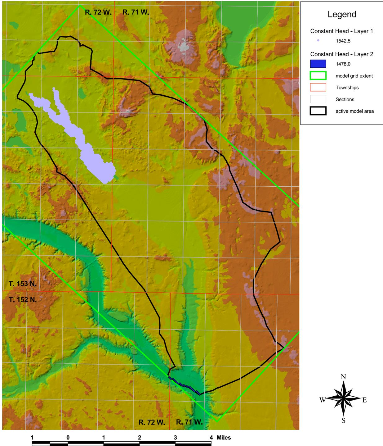
**Figure 116** Location of constant head nodes used to simulate Long Lake and Sheyenne River.
