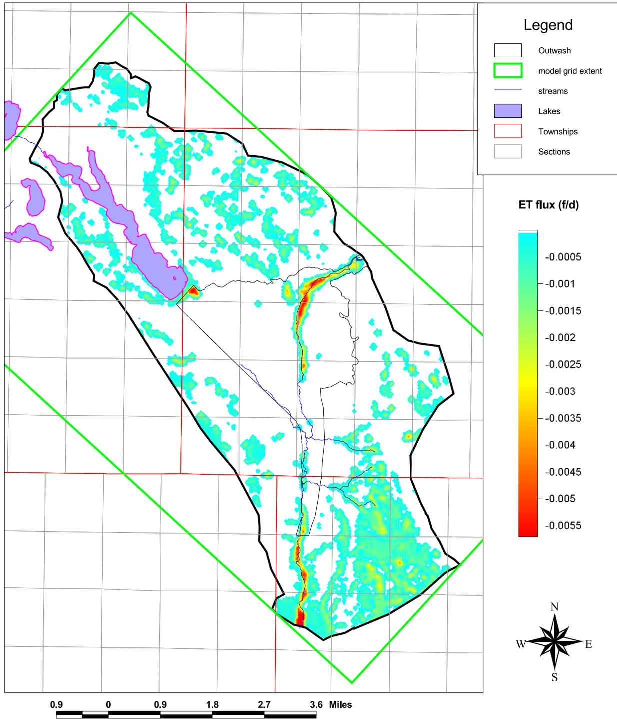
**Figure 123.** Discharge by evapotranspiration (feet per day) in layer 2, steady-state model run B21hh.
