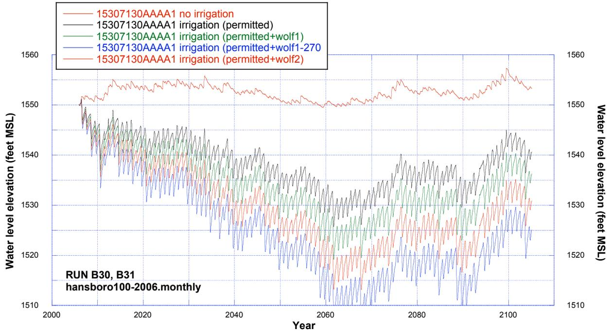
**Figure 156.** Comparisons of simulated water levels at observation well 153-071-30AAAA1 (Trappers Coulee aquifer) using hansboro100-2005.monthly recharge dataset for cases of no irrigation, permitted irrigation, and additional irrigation.
