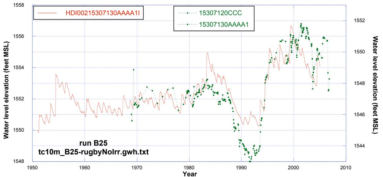
**Figure 133.** Comparison of observed water levels at 153-071-20CCC and 153-071-30AAA1 (replacement well for 153-071-20CCC) with simulated water levels from run B25 (rugby01\_f03.monthly) with no irrigation.
