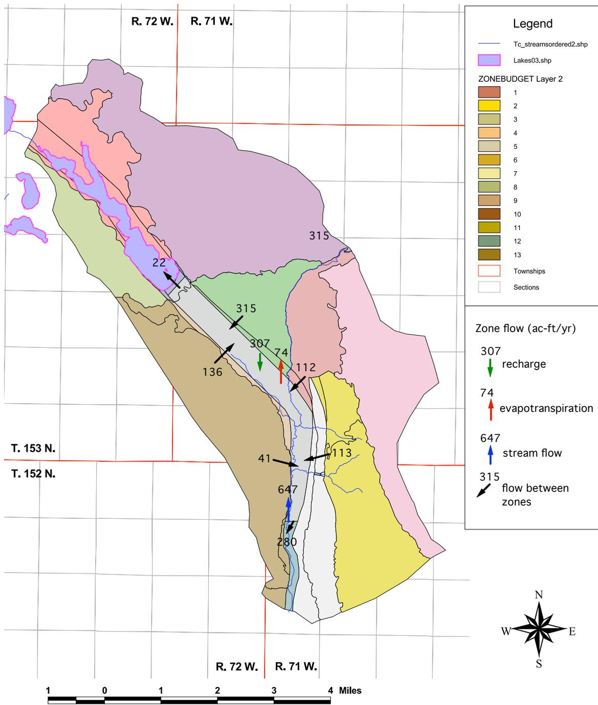
**Figure 125.** Hydrologic budget of the Trappers Coulee meltwater trench (ZONEBUDGET zone 01). Simulation tc10B21hh.
