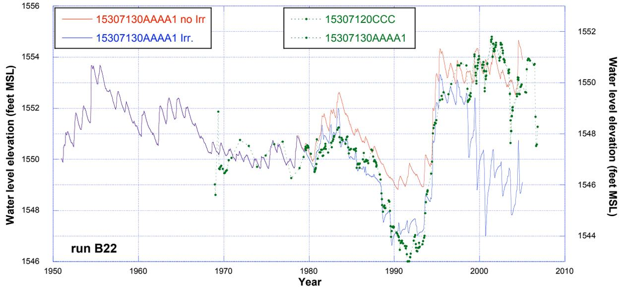
**Figure 128.** Comparison of observed water levels at 153-071-20CCC and 153-071-30AAA1 (replacement well for 153-071-20CCC) with simulated water levels from run B22 (drake\_f03.monthly) using reported water use and no irrigation use.
