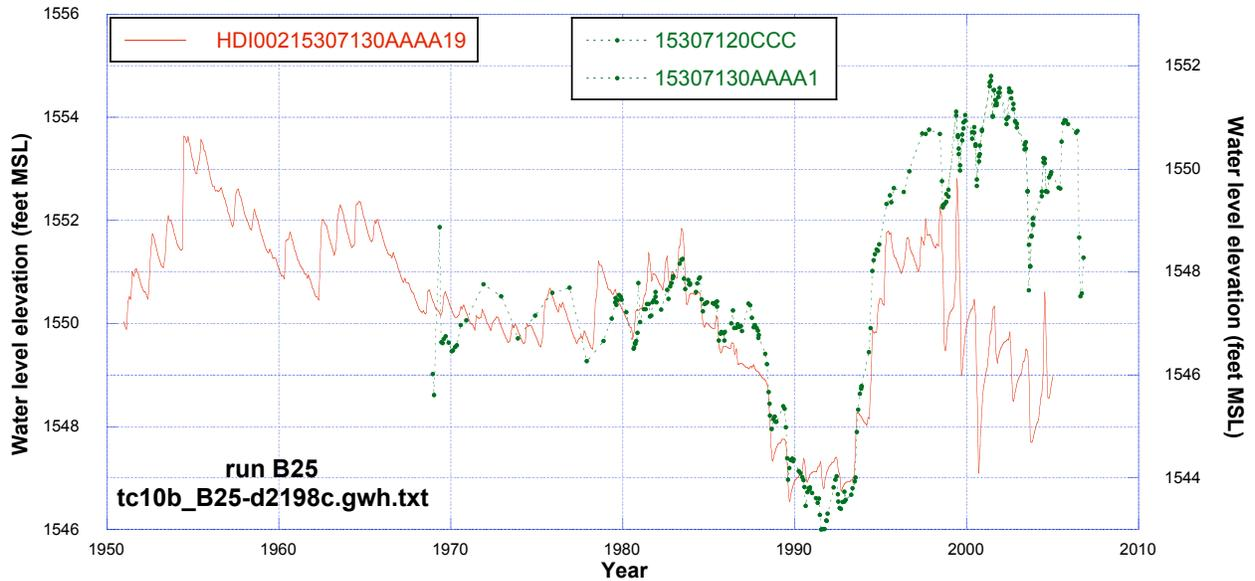
**Figure 132.** Comparison of observed water levels at 153-071-20CCC and 153-071-30AAA1 (replacement well for 153-071-20CCC) with simulated water levels from run B25 (drake2198c\_f03.monthly) using reported water use.
