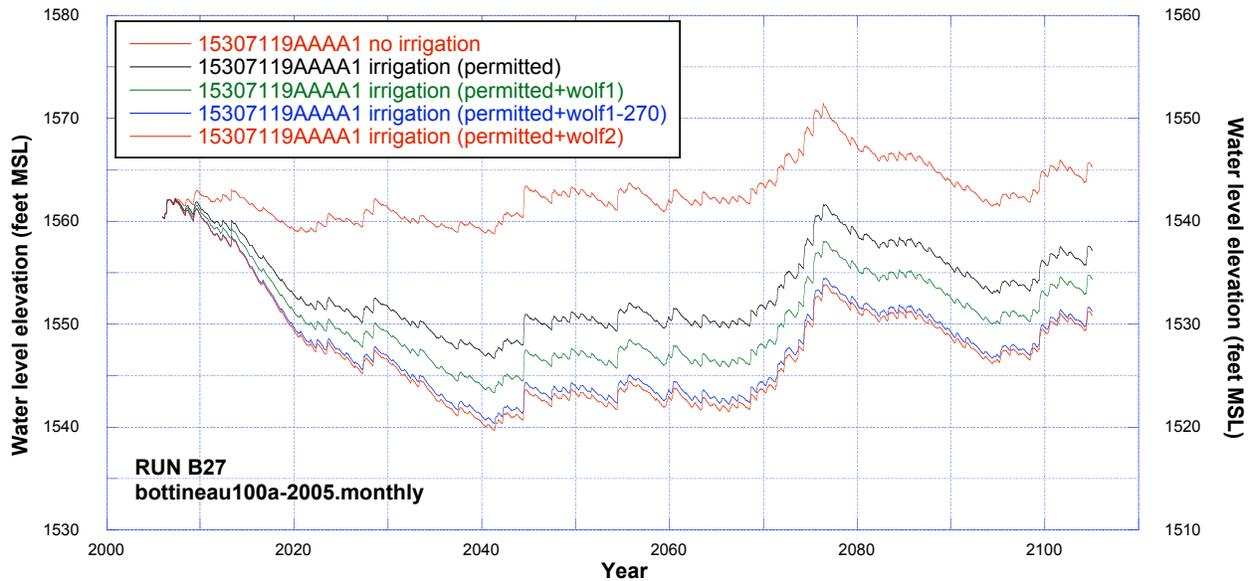
**Figure 142.** Comparisons of simulated water levels at observation well 153-071-19AAAA1 (Fox Hills aquifer) using bottineau100a-2005.monthly recharge dataset for cases of no irrigation, permitted irrigation, and additional irrigation.
