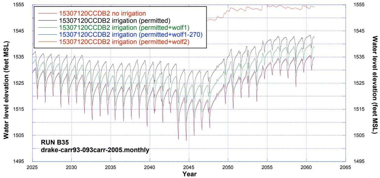
**Figure 158.** Simulated water levels at irrigation well 153-071-20CCDB2 (Trappers Coulee aquifer) using drake-carr93carr-2005.monthly recharge dataset for cases of no irrigation, permitted irrigation, and additional irrigation.
