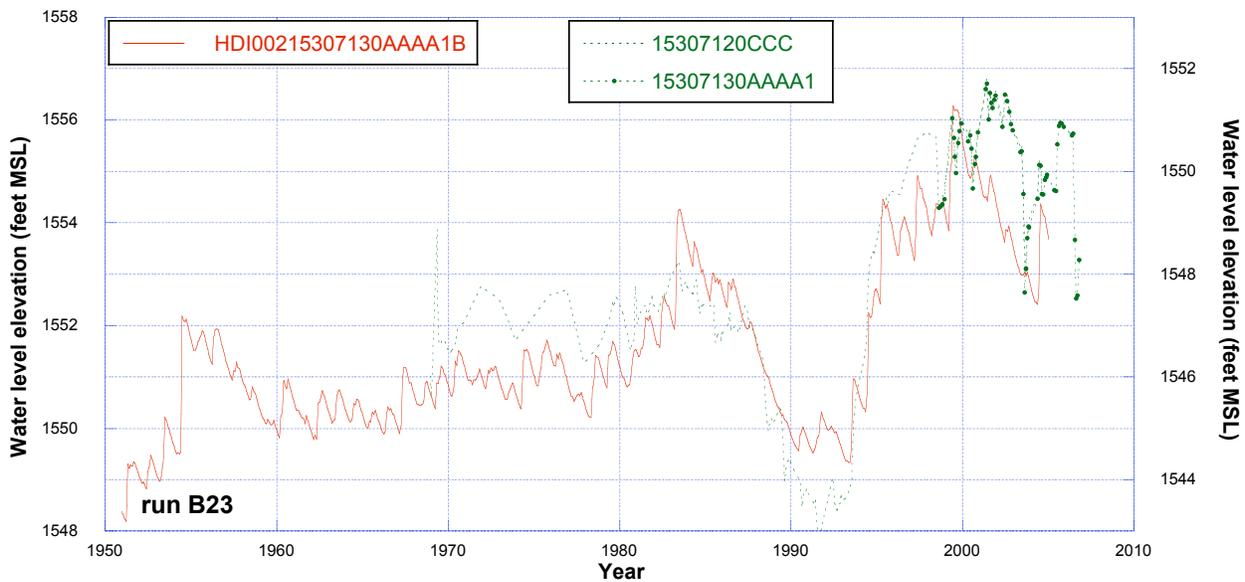
**Figure 129.** Comparison of observed water levels at 153-071-20CCC and 153-071-30AAA1 (replacement well for 153-071-20CCC) with simulated water levels from run B23 (rugby01\_f03.monthly) with no irrigation.
