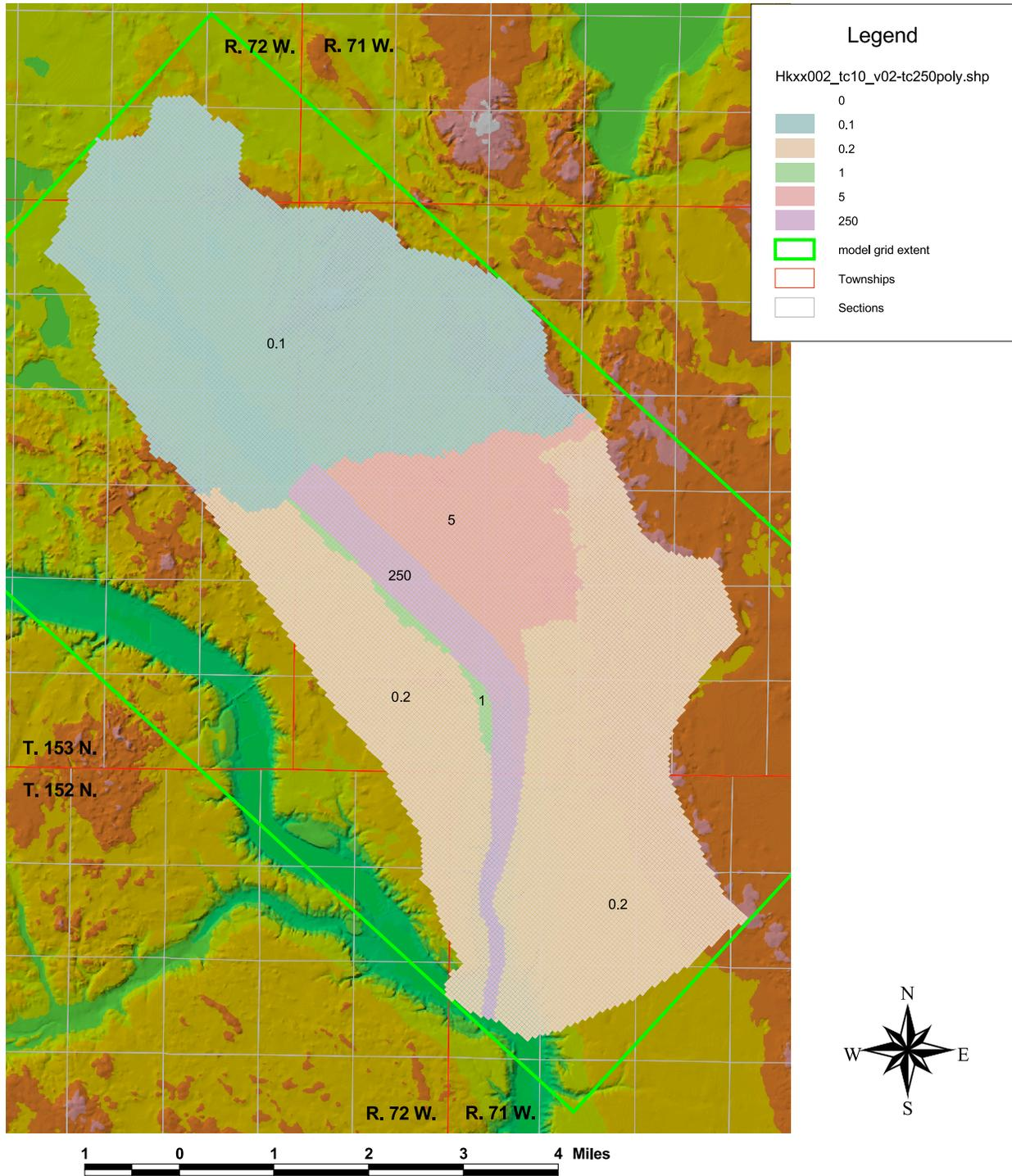
**Figure 113.** Layer 2 hydraulic conductivity (feet per day) for GRID10. File "Volumes/G5data2/esmond/model02outwash/GRID10/hy/HKxx002\_tc10\_v02-tc250.mf".
