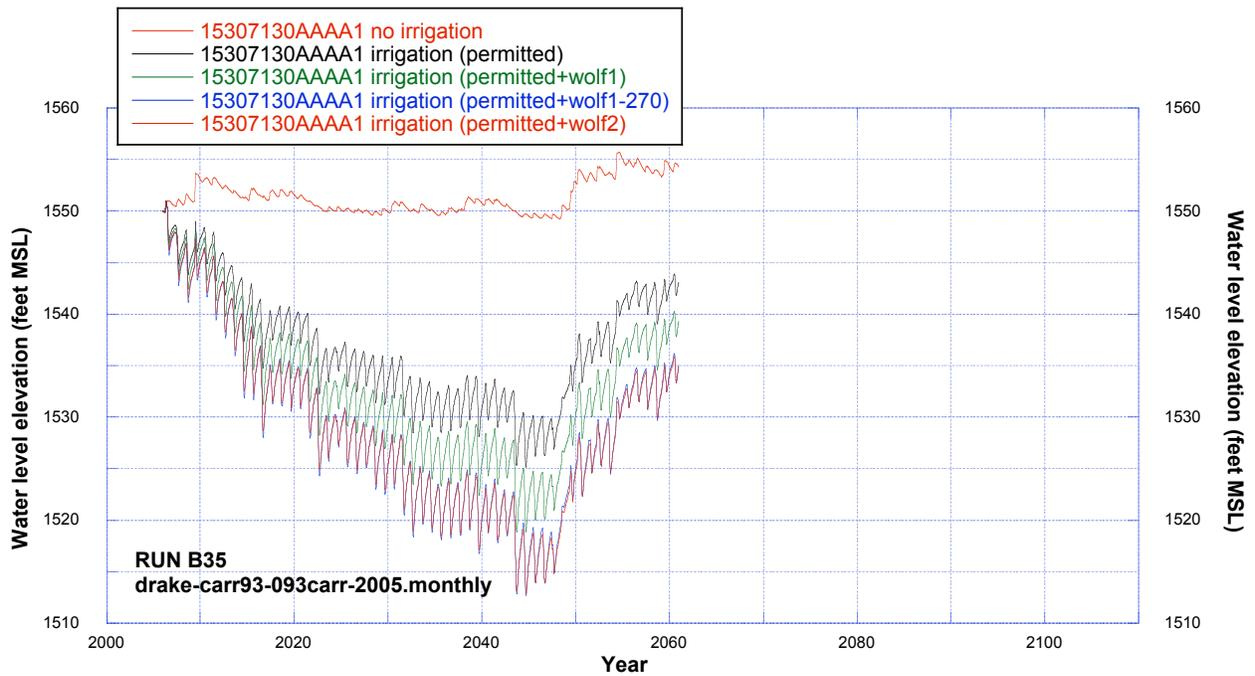
**Figure 140.** Comparisons of simulated water levels at observation well 153-071-30AAAA1 (Trappers Coulee aquifer) using drake-carr93carr-2005.monthly recharge dataset for cases of no irrigation, permitted irrigation, and additional irrigation.
