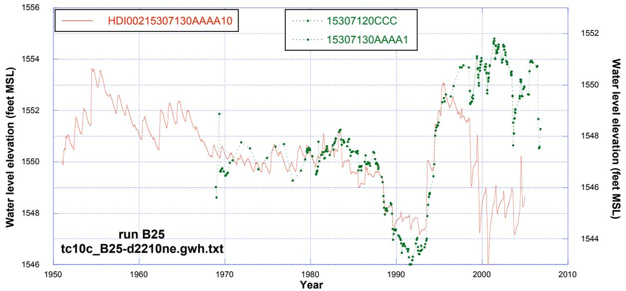
**Figure 130.** Comparison of observed water levels at 153-071-20CCC and 153-071-30AAA1 (replacement well for 153-071-20CCC) with simulated water levels from run B25 (drake2210ne\_f03.monthly) using reported water use.
