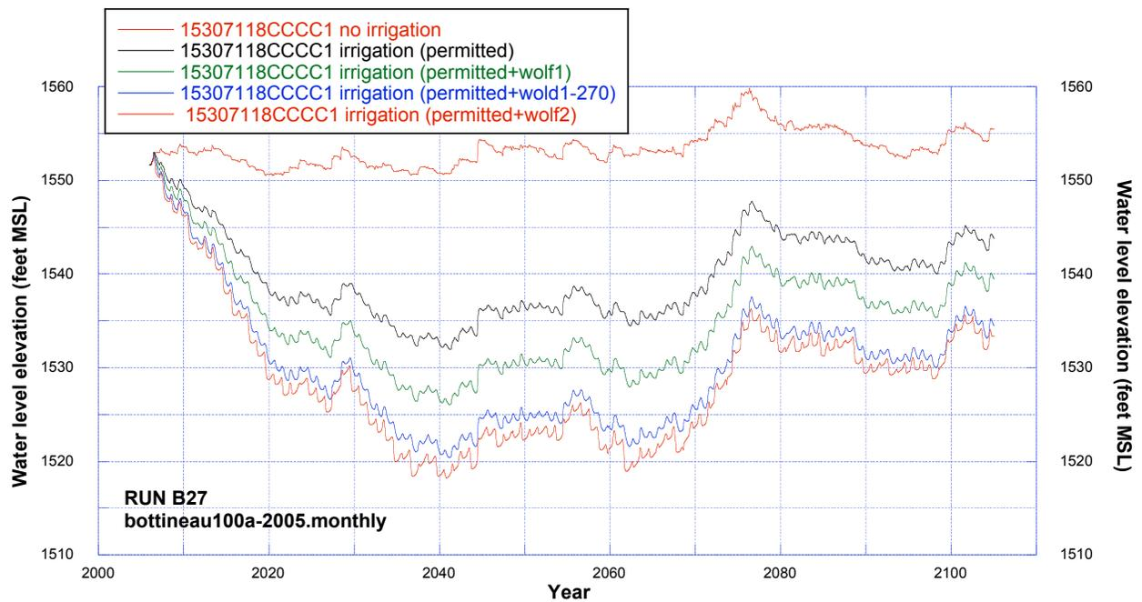
**Figure 143.** Comparisons of simulated water levels at observation well 153-071-18CCCC1 (Trappers Coulee aquifer) using bottineau100a-2005.monthly recharge dataset for cases of no irrigation, permitted irrigation, and additional irrigation.
