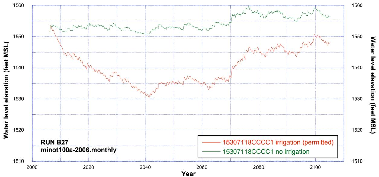
**Figure 147.** Comparisons of simulated water levels at observation well 153-071-18CCCC1 (Trappers Coulee aquifer) using minot100a-2005.monthly recharge dataset for cases of no irrigation and permitted irrigation.
