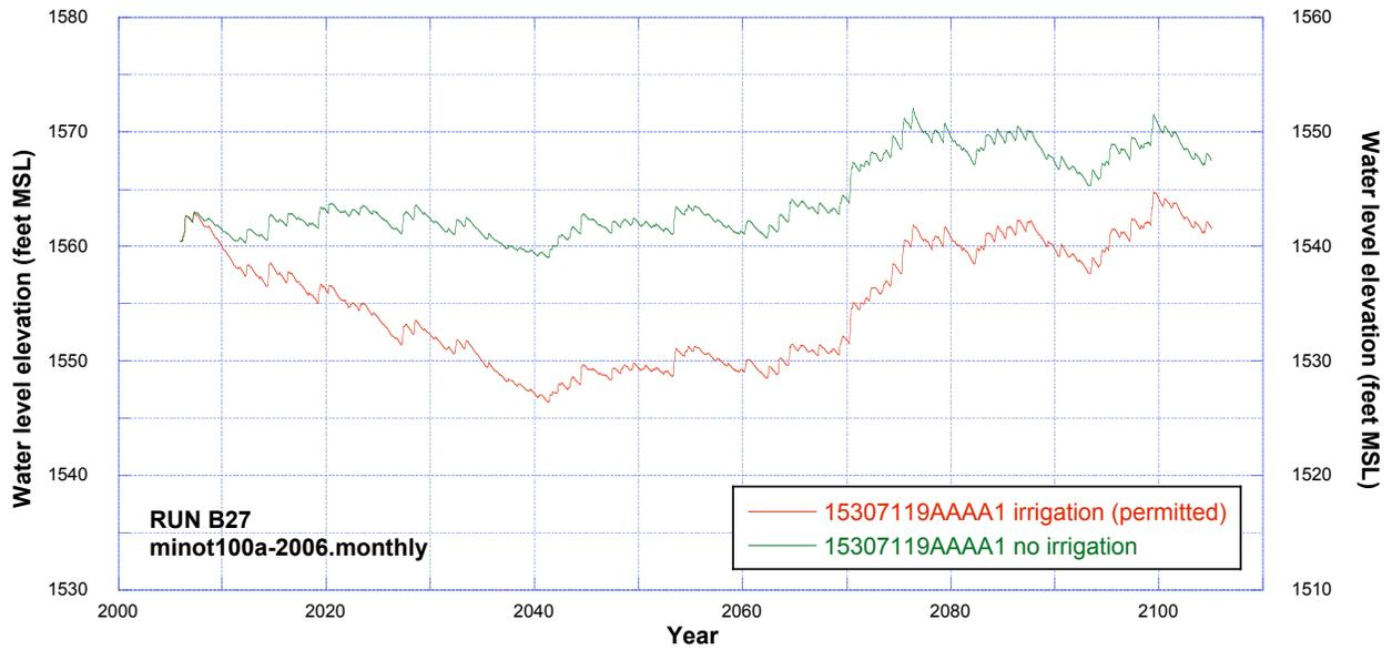
**Figure 146.** Comparisons of simulated water levels at observation well 153-071-19AAAA1 (Fox Hills aquifer) using minot100a-2005.monthly recharge dataset for cases of no irrigation and permitted irrigation.
