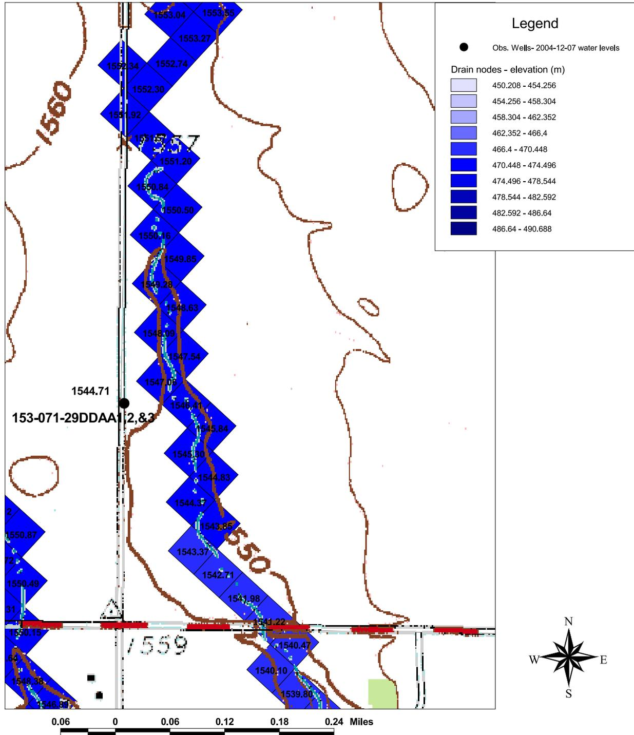
**Figure 121.** Shows drain node elevations (feet) in Trappers Coulee near NDSWC observation wells at 15307129DDAA (see figure 20). Observed water level in 15307129DDAA1 on 12/07/04 is shown. Topography from USGS Esmond 7.5-Minute Quadrangle Map.
