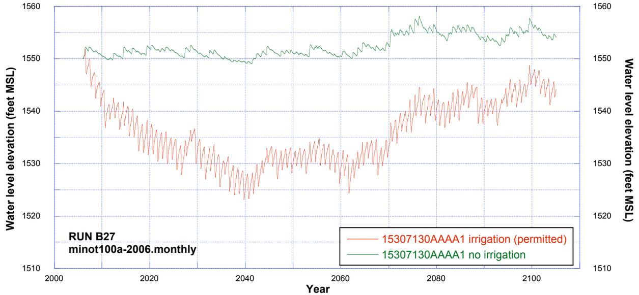
**Figure 148.** Comparisons of simulated water levels at observation well 153-071-30AAAA1 (Trappers Coulee aquifer) using minot100a-2005.monthly recharge dataset for cases of no irrigation and permitted irrigation.
