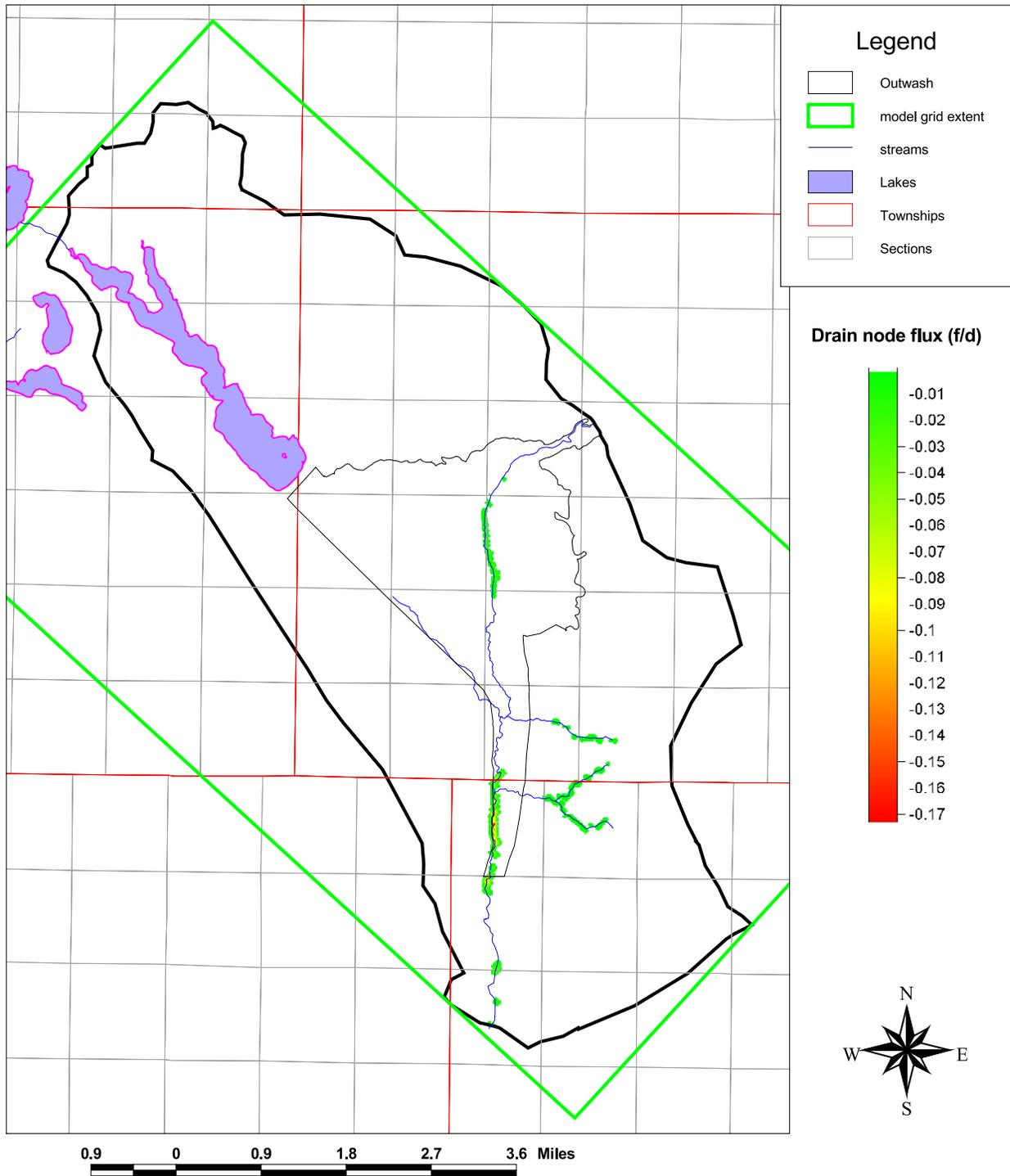
Figure 122. Flow from drain (feet per day) nodes in layer 2, steady-state model run B21hh.
