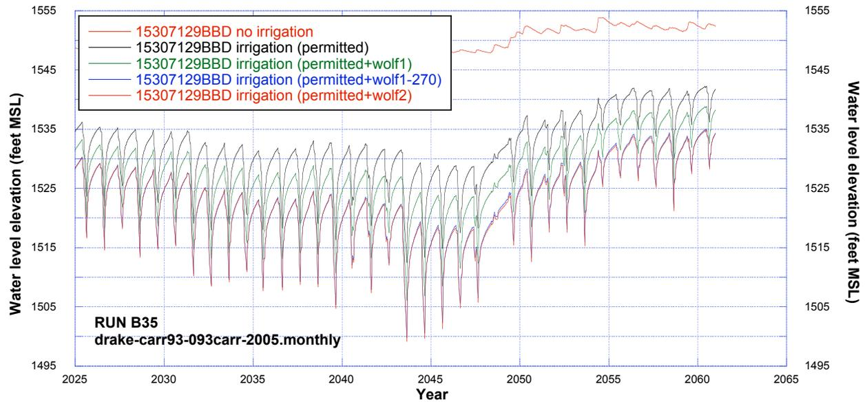
**Figure 160.** Simulated water levels at irrigation well 153-071-29BBD (Trappers Coulee aquifer) using drake-carr93carr-2005.monthly recharge dataset for cases of no irrigation, permitted irrigation, and additional irrigation.
