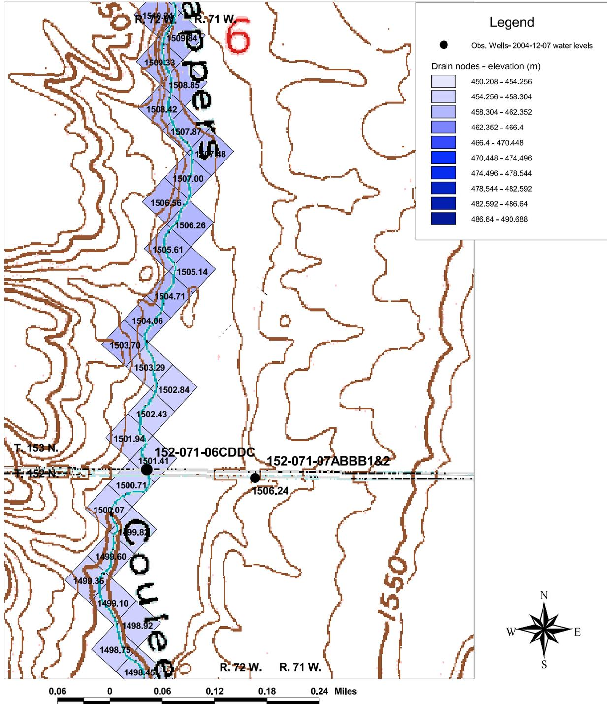
**Figure 120.** Shows drain node elevations (feet) in Trappers Coulee and observed water level elevation in 15207107ABBB1 on 12/07/04. Topography from USGS Esmond 7.5-Minute Quadrangle Map. At NDSWC stream gage site 15207106CDDC the bottom of stream elevation is approximately 1504 feet. The water level at 15207107ABBB is approximately 2 feet higher than in the stream at 15207106CDDC (see figure 21).
