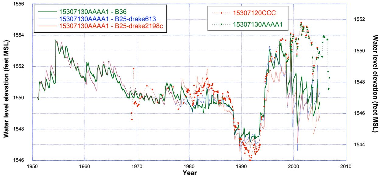
**Figure 136.** Comparisons of simulated water levels at observation well 153-071-30AAAA1 using reported water use and drake613\_f03.monthly, drake2198c\_f03.monthly, and drake-carr93-093carr.monthly (B36) climate datasets to observed water levels at 153-071-20CCC and 153-071-30AAA1 (replacement well for 153-071-20CCC).
