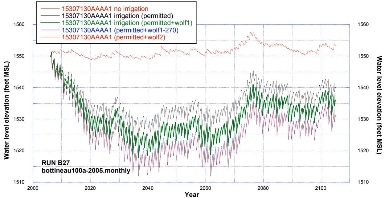
**Figure 144.** Comparisons of simulated water levels at observation well 153-071-30AAAA1 (Trappers Coulee aquifer) using bottineau100a-2005.monthly recharge dataset for cases of no irrigation, permitted irrigation, and additional irrigation.
