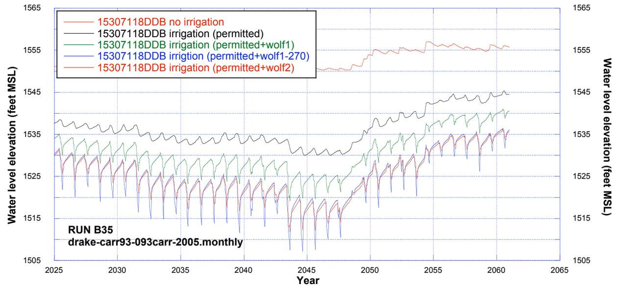
**Figure 161.** Simulated water levels at proposed irrigation well 153-071-18DDB (Trappers Coulee aquifer) using drake-carr93carr-2005.monthly recharge dataset for cases of no irrigation, permitted irrigation, and additional irrigation.
