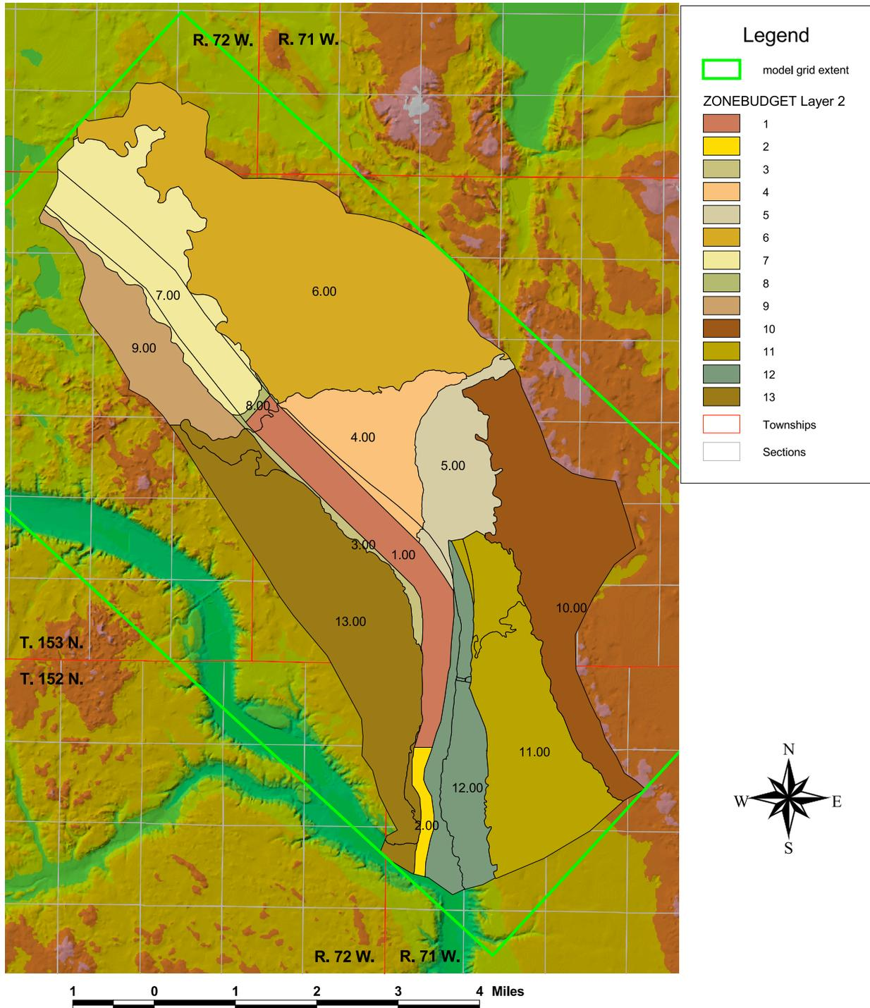
**Figure 108.** Layer 2 budget zones used by ZONEBUDGET. File "esmond/model02outwash/GRID10/zone\_budget/arcview/ZBDG002\_tc10\_v01.shp".
