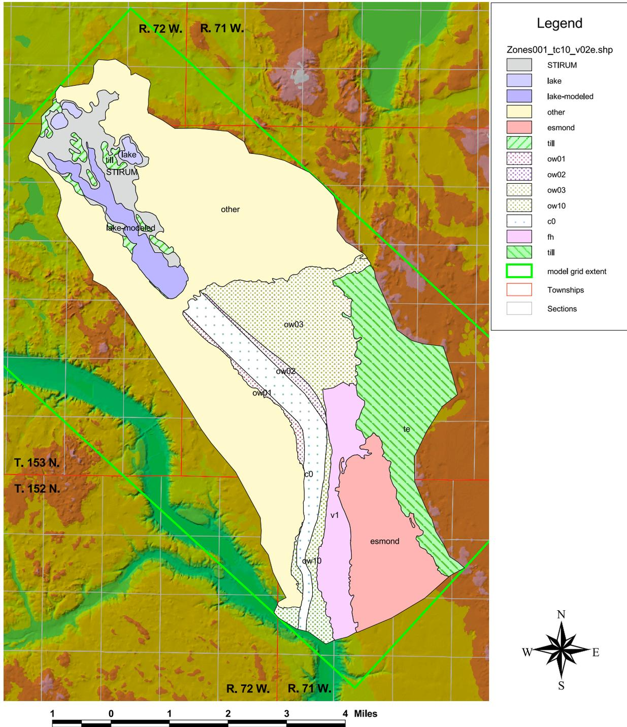
**Figure 109.** Layer 1 hydraulic property zones. Different combinations of property zones were used to assign various hydraulic properties or multipliers to arrays. File "esmond/model02outwash/GRID10/zone/zones/zones001\_tc10\_v02e.shp".
