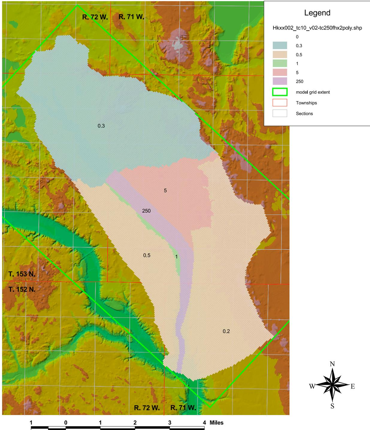
**Figure 114.** Layer 2 hydraulic conductivity (feet per day) for GRID10. File "Volumes/G5data2/esmond/model02outwash/GRID10/hy/HKxx002\_tc10\_v02-tc250fhx2.mf".
