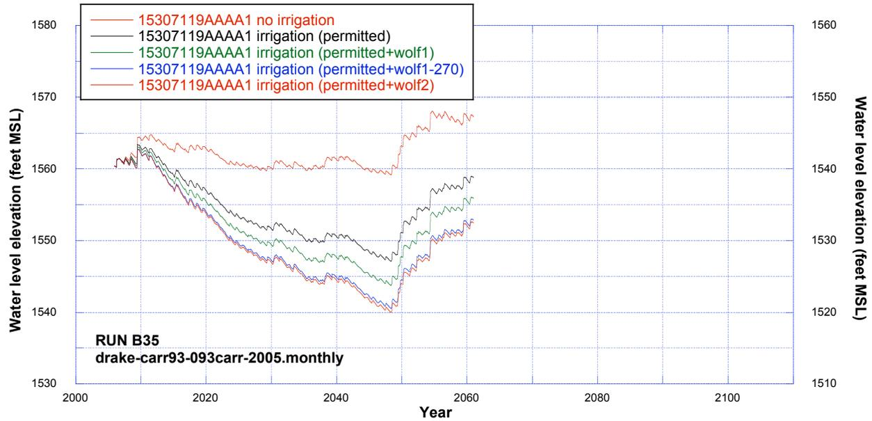
**Figure 138.** Comparisons of simulated water levels at observation well 153-071-19AAAA1 (Fox Hills aquifer) using drake-carr93carr-2005.monthly recharge dataset for cases of no irrigation, permitted irrigation, and additional irrigation.
