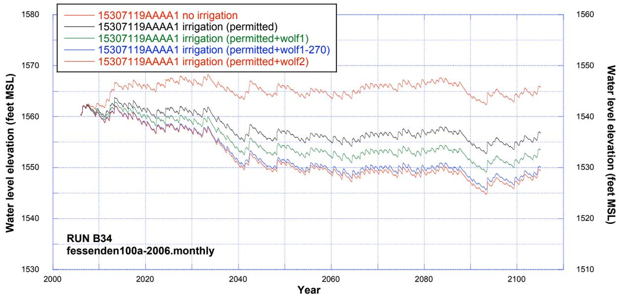
**Figure 150.** Comparisons of simulated water levels at observation well 153-071-19AAAA1 (Fox Hills aquifer) using fessenden100a-2005.monthly recharge dataset for cases of no irrigation, permitted irrigation, and additional irrigation.
