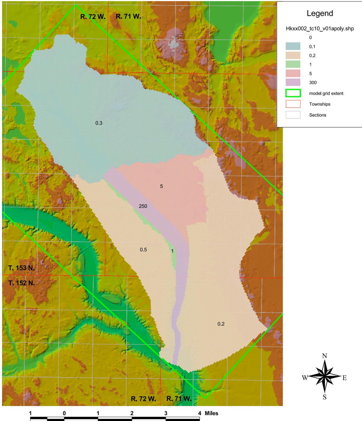
**Figure 112.** Layer 2 hydraulic conductivity (feet per day) for GRID10. File "Volumes/G5data2/esmond/model02outwash/GRID10/hy/HKxx002\_tc10\_v01a.mf".
