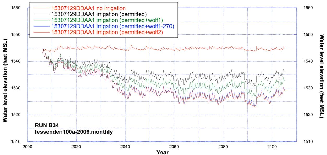
**Figure 153.** Comparisons of simulated water levels at observation well 153-071-29DDAA1 (Trappers Coulee aquifer) using fessenden100a-2005.monthly recharge dataset for cases of no irrigation, permitted irrigation, and additional irrigation.
