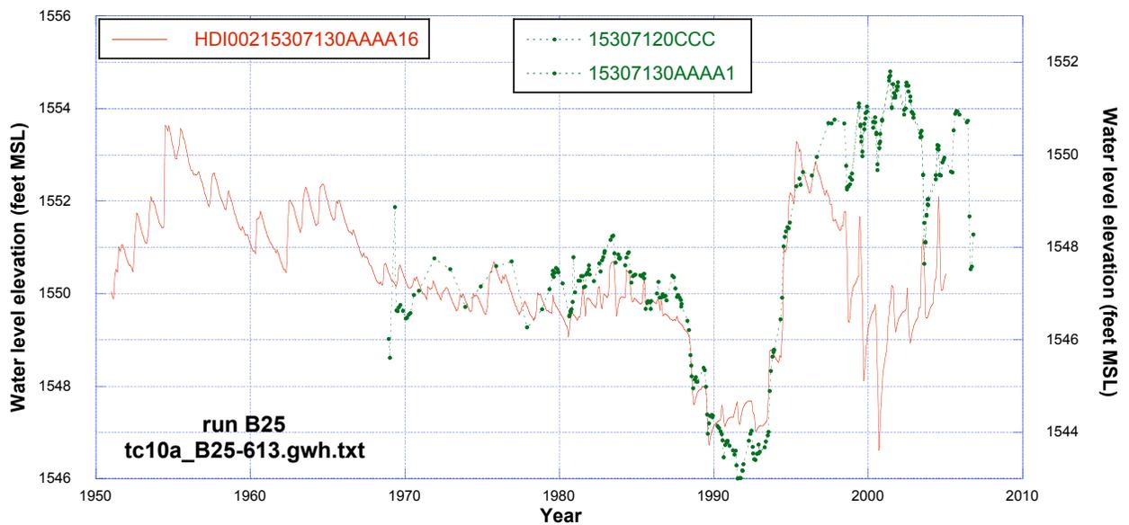
**Figure 131.** Comparison of observed water levels at 153-071-20CCC and 153-071-30AAA1 (replacement well for 153-071-20CCC) with simulated water levels from run B25 (drake613\_f03.monthly) using reported water use.
