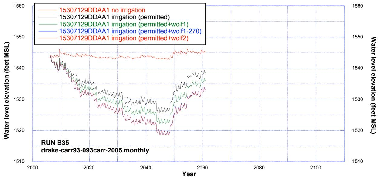
**Figure 141.** Comparisons of simulated water levels at observation well 153-071-29DDAA1 (Trappers Coulee aquifer) using drake-carr93carr-2005.monthly recharge dataset for cases of no irrigation, permitted irrigation, and additional irrigation.
