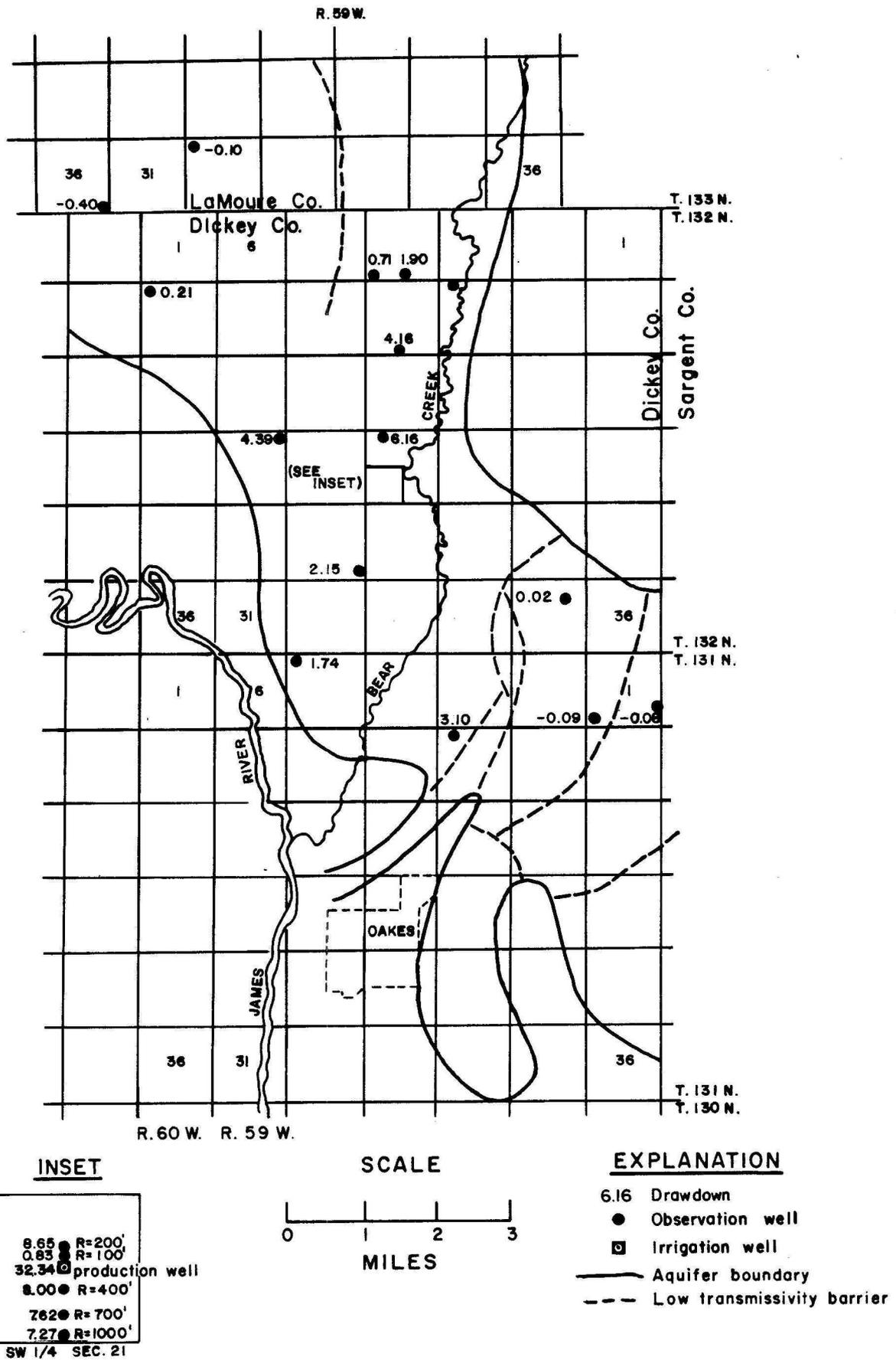
**FIGURE 14.-Curt Knutson aquifer test:
