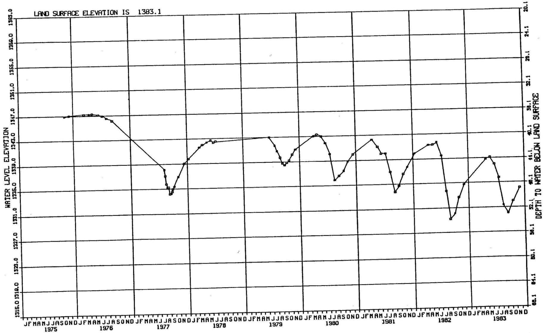
FIGURE 21.-Hydrograph of observation well 133-60-36DDD
