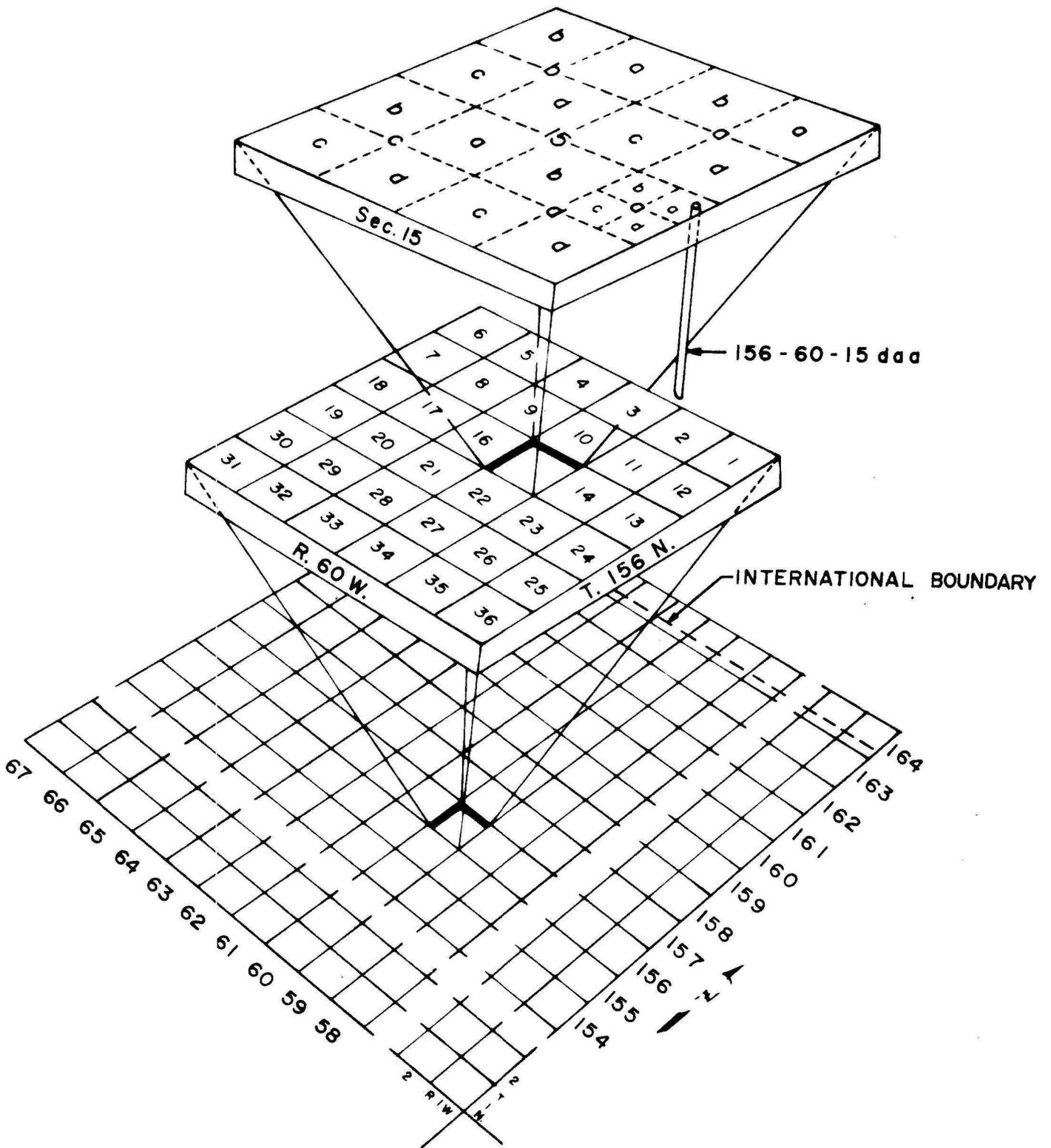
FIGURE 2-- DIAGRAM SHOWING WELL-NUMBERING SYSTEM
