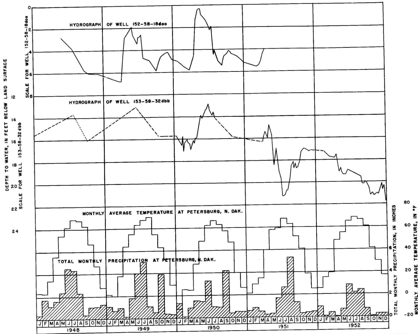
FIGURE 7.—HYDROGRAPHS OF TWO WELLS IN THE MICHIGAN CITY AREA AND GRAPHS SHOWING MONTHLY AVERAGE TEMPERATURE AND TOTAL MONTHLY PRECIPITATION AT PETERSBURG, N. DAK., FOR THE YEARS 1948-52, INCLUSIVE.
