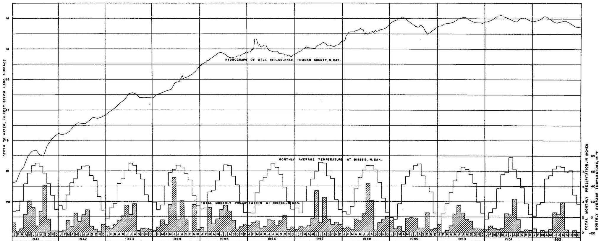
FIGURE 8.—HYDROGRAPH OF WELL 160-66-28b01, TOWNER COUNTY, N. DAK., AND GRAPHS SHOWING MONTHLY AVERAGE TEMPERATURE AND TOTAL MONTHLY PRECIPITATION AT BISBEE, N. DAK., FOR THE YEARS 1941-52, INCLUSIVE.
