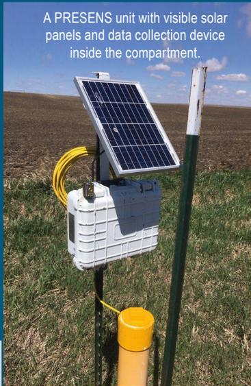
A PRESENS unit with visible solar panels and data collection device inside the compartment.
