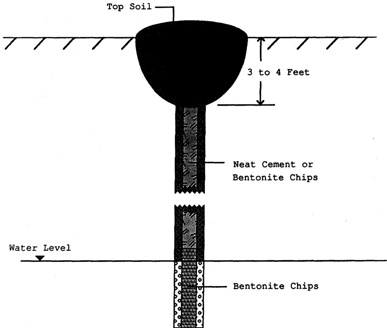
Figure 3. Monitoring well abandonment procedure.
