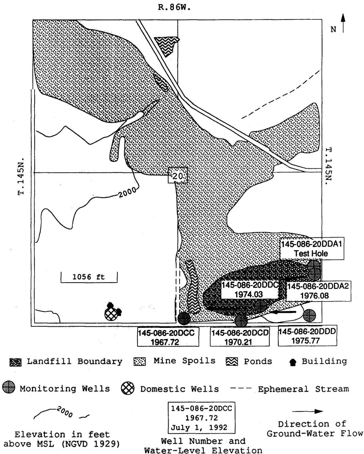
Figure 4. Location of monitoring wells and the direction of ground-water flow at the Devils Lake landfill.
