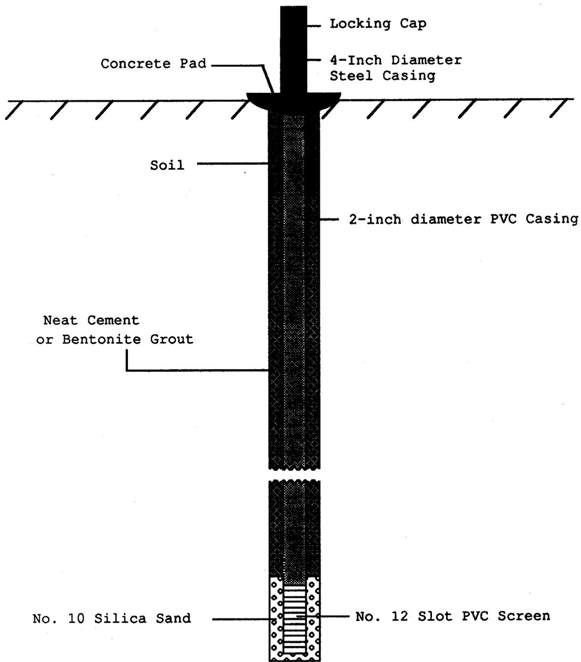
Figure 2. Construction design used for monitoring wells installed at the Hazen landfill.
