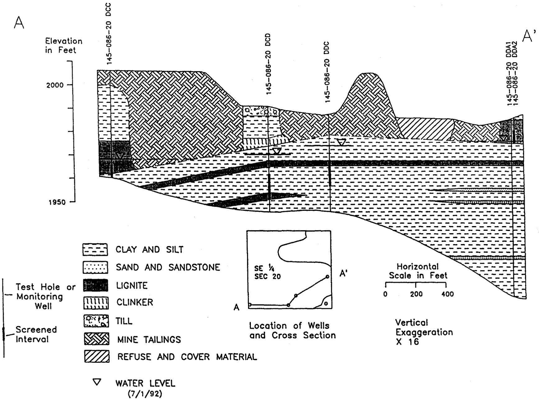
Figure 6. Geohydrologic section A-A' in the Hazen landfill
