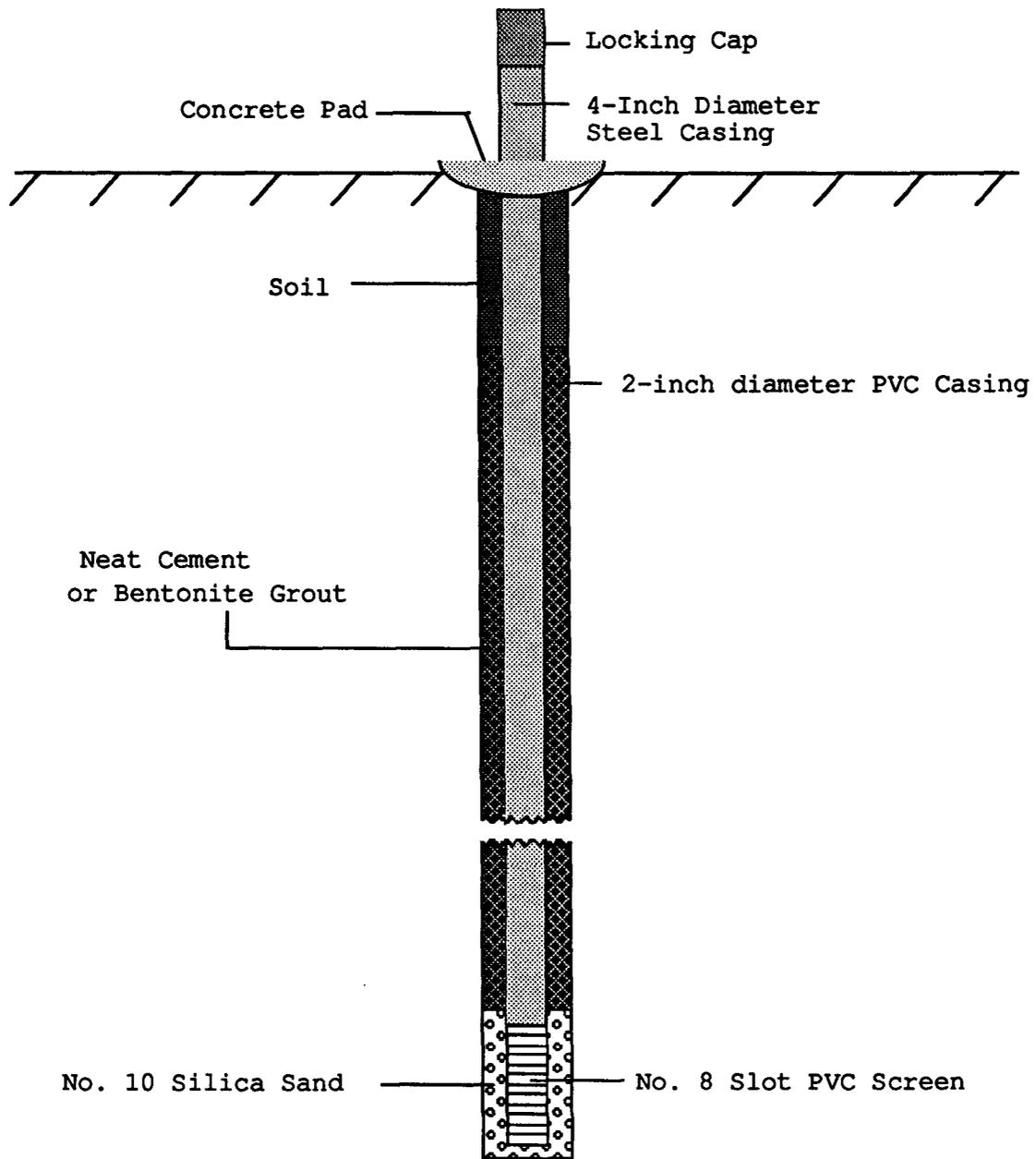
Figure 2. Construction design used for monitoring wells installed at the Casper Volk landfill.
