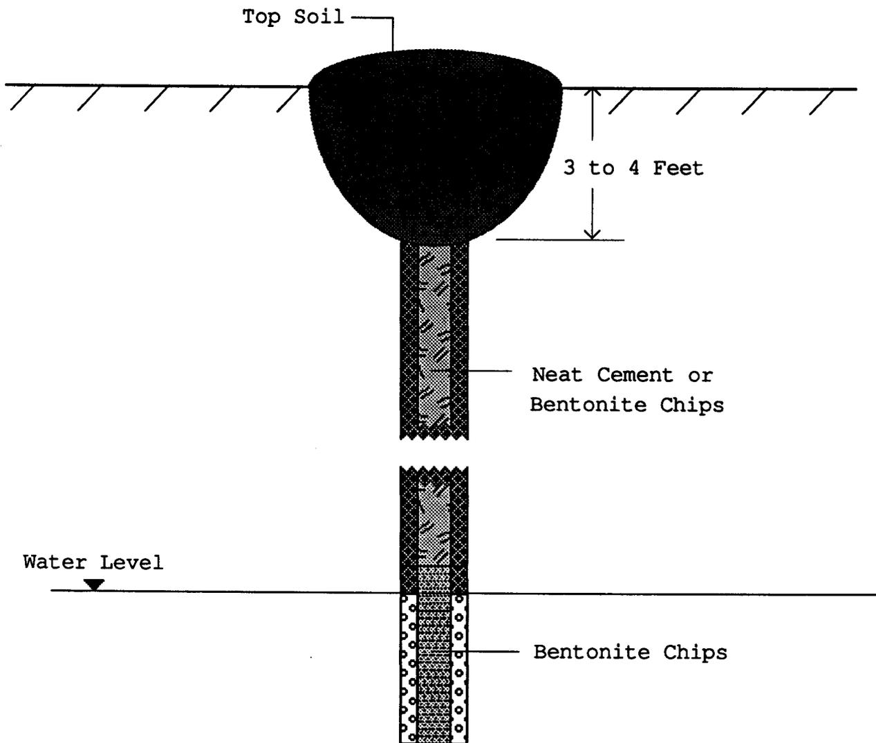
Figure 3. Monitoring well abandonment procedures.
