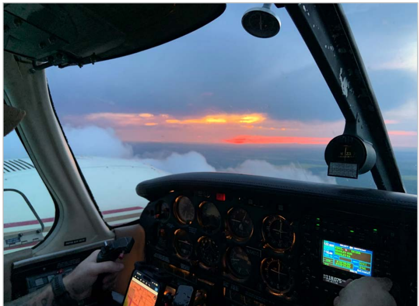
Fig. 16. Seed 1 (N39655) conducts a seeding mission on 5 July 2024 for District II. During this 1hr 45min flight both burners were lit, and 8 burn-in-place pyrotechnics were consumed. At the bottom left you can see the pilot utilizing telemetry data. Photo by Peyton Underwood.
