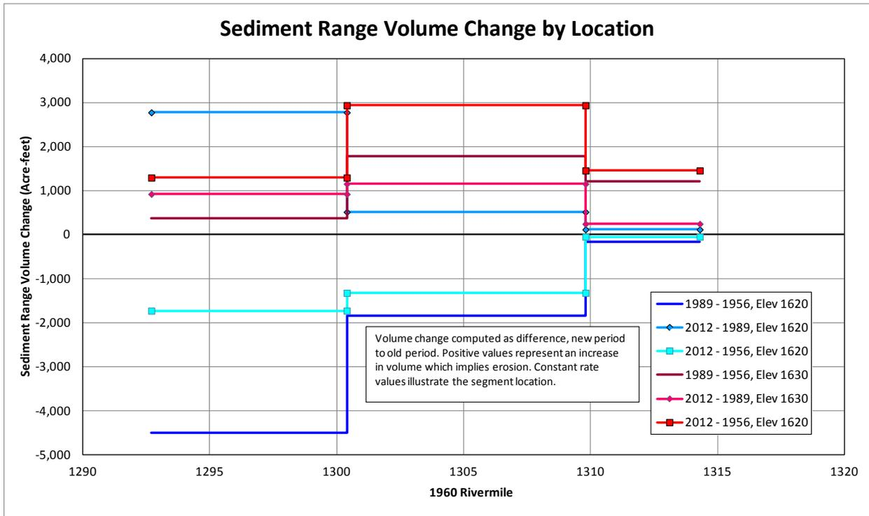
Figure 16. Sediment Range Volume Change by Location
