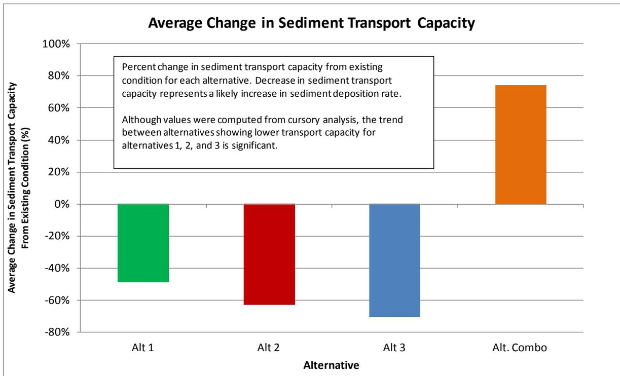
Figure 26. Average Change in Sediment Transport Capacity
