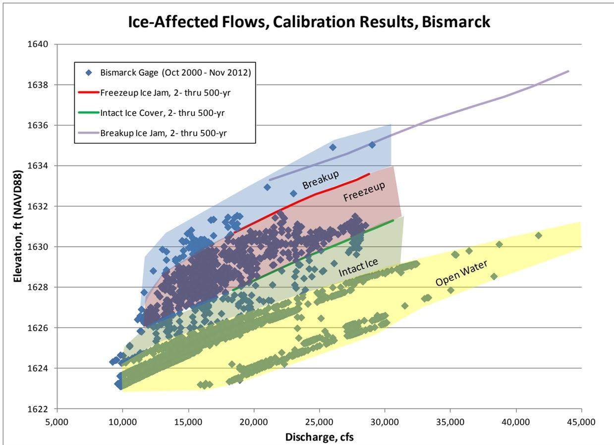
Figure 3. Ice-Affected Flow Regimes Used in HEC-RAS Calibration
