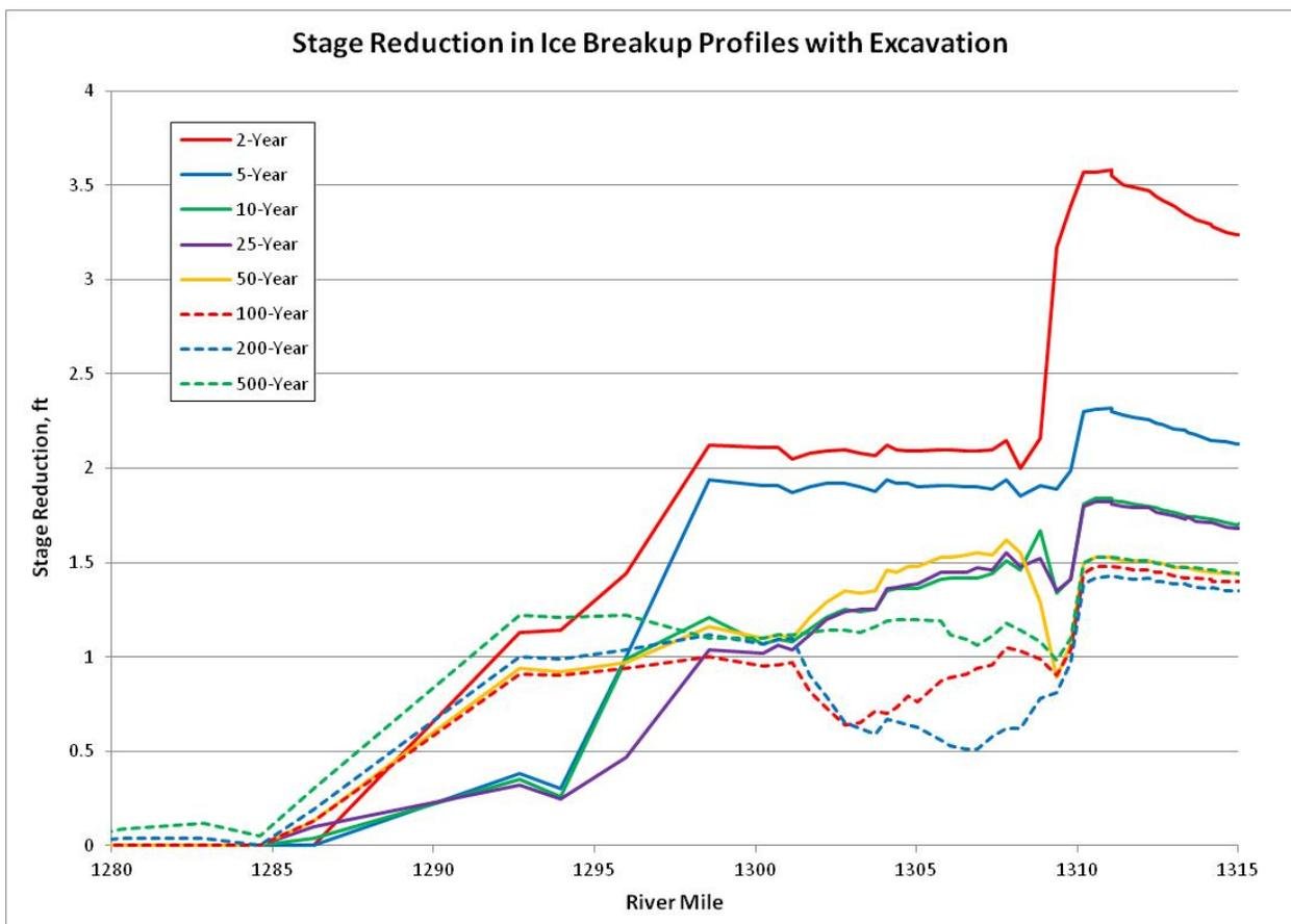
Figure 29. Stage Reduction for Ice Breakup with Channel Excavation Alternative 3
