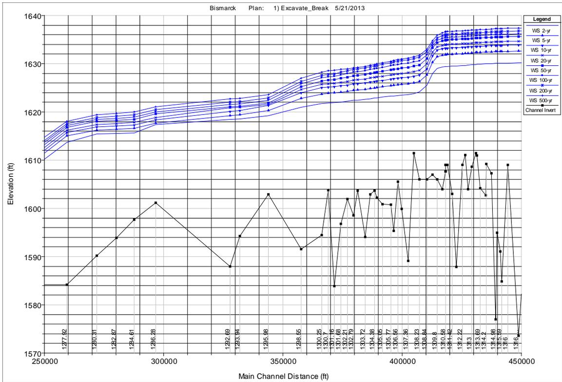
Figure 27. Alternative 3 Ice-Affected Breakup Flow Profiles, Missouri River
