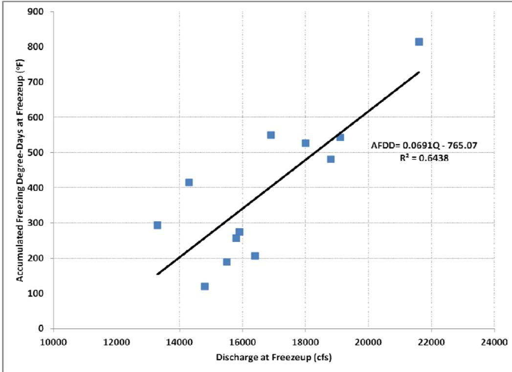
Figure 9 Accumulated Freezing Degree-Days (AFDD) at freezeup as a function of discharge
