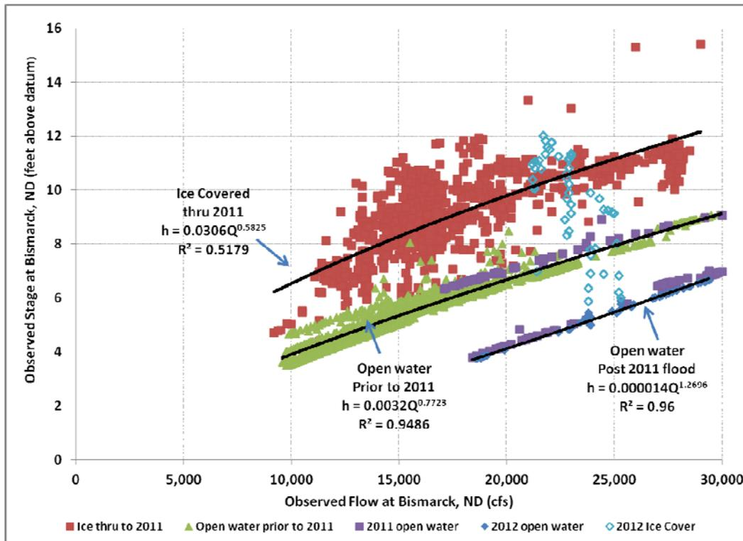
Figure 11 Open water and ice covered rating curves for period before 2011 flood and after
