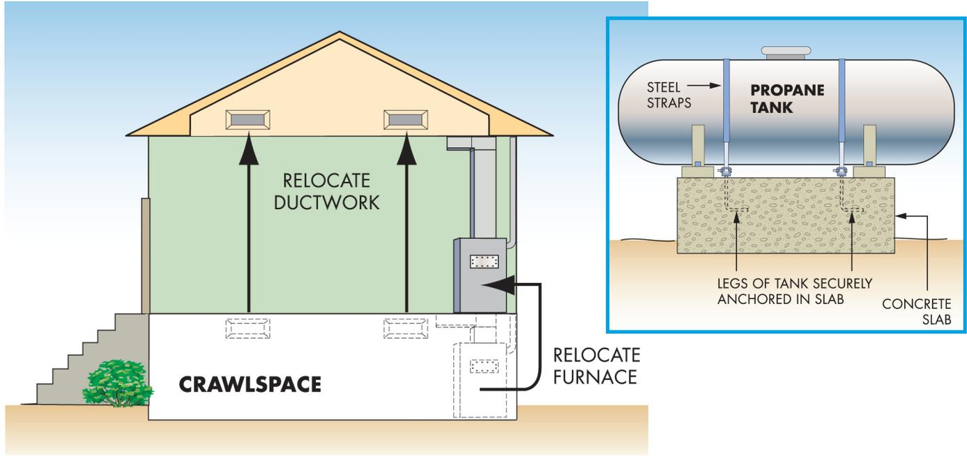
Move your hot water heater and furnace out of the basement; or build small platforms for them. Anchor heating oil and propane gas tanks to prevent floatation. **Do not** store valuables in a floodprone basement. Use water-resistant materials when you repair.
