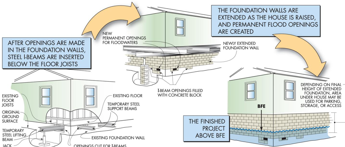
This is one way to elevate an existing building to comply with building code and floodplain regulations (also see FEMA P-312, Homeowner's Guide to Retrofitting). If an NFIP-insured building is damaged by flood and the community determines it is substantially damaged, the owner may be eligible for an **Increased Cost of Compliance payment** (see page 90).
