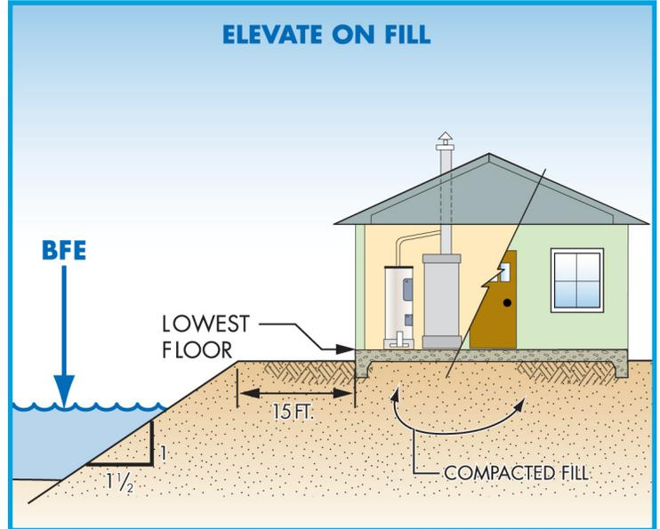
**CAUTION!** Enclosures (including crawlspaces) have some special requirements (see page 63). Note: When the walking surface of the lowest floor is at the minimum elevation, under-floor utilities are not allowed. Fill used to elevate buildings must be placed properly (see page 65).
