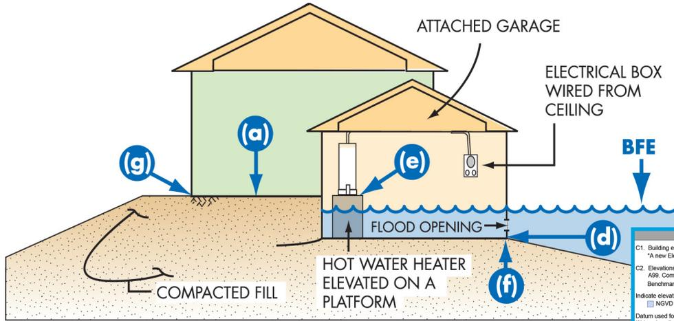
The slab-on-grade house was elevated on fill 1 foot above the BFE, and the vented garage is 3 feet below the BFE.
