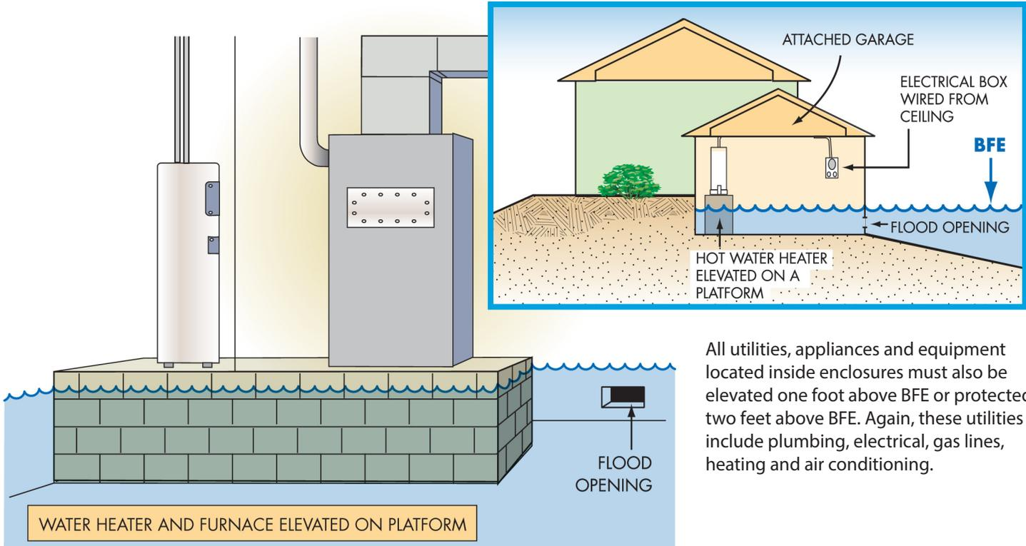
All utilities, appliances and equipment located inside enclosures must also be elevated one foot above BFE or protected two feet above BFE. Again, these utilities include plumbing, electrical, gas lines, heating and air conditioning.
