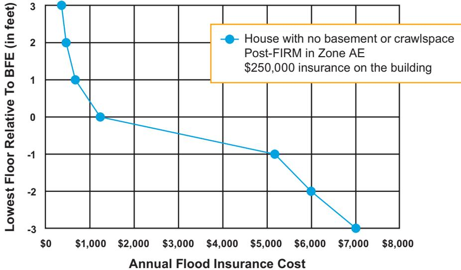
Want to save some money and have peace of mind at the same time? Then add freeboard to build higher than the minimum elevation requirement! Freeboard is a factor of safety, usually one or two feet above the BFE. **In North Dakota, one foot of freeboard is required** for residential and non-residential structures, while critical facilities have a higher standard.
