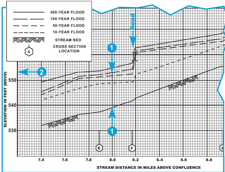
The FIS includes flood profiles that can be used to determine the BFE at a specific site. Profiles also show estimated water surface elevations for floods other than the 1% annual chance flood.
