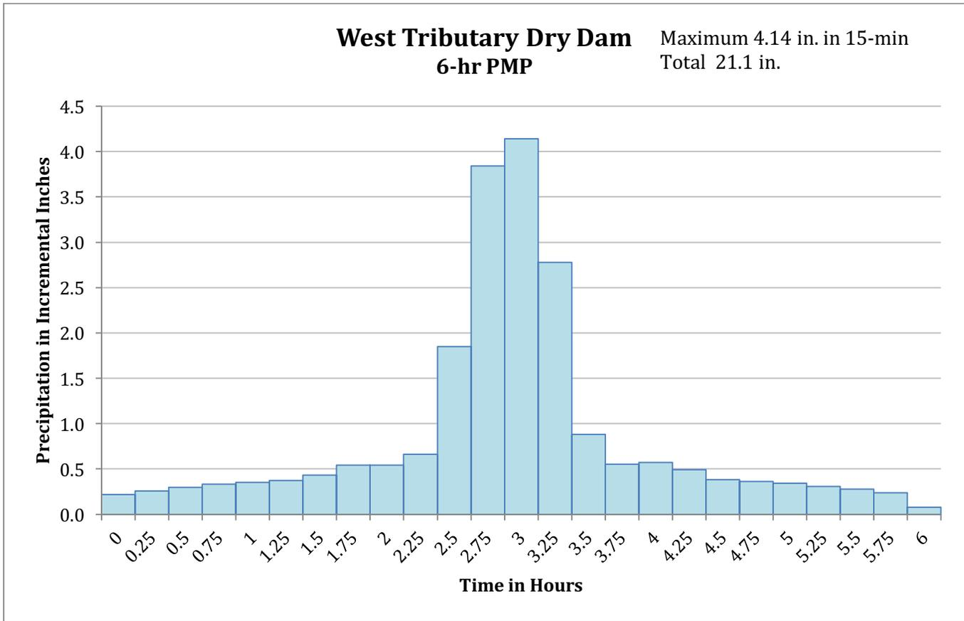
**Figure 2.** Balanced PMP Hyetograph.
