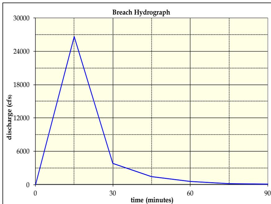
**Figure 9.** Calculated Breach Hydrograph.
