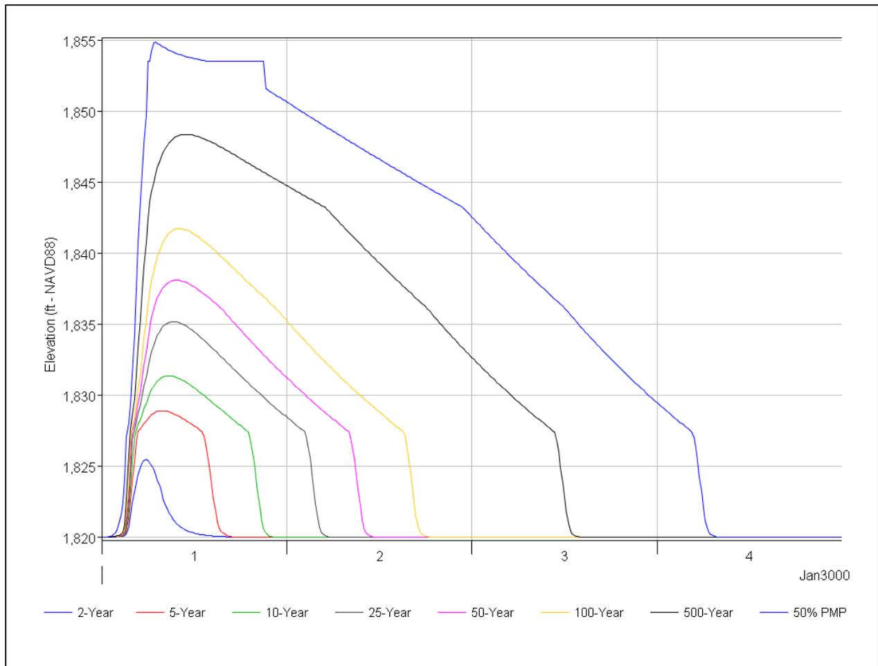
**Figure 8.** Reservoir Elevation for Frequency Events.
