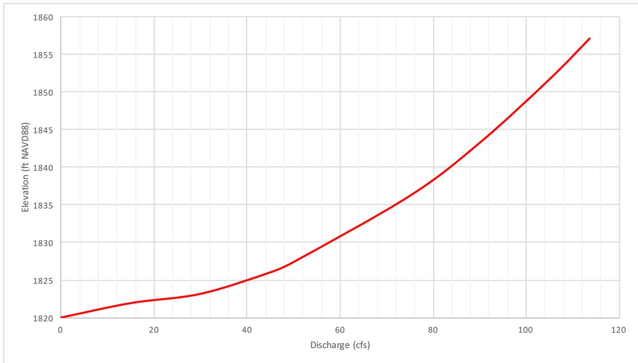
Figure 6. Principal Spillway Elevation-Discharge Curve.
