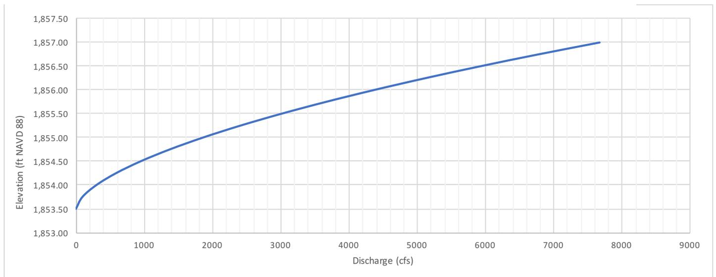
Figure 7. Emergency Spillway Elevation-Discharge Curve.
