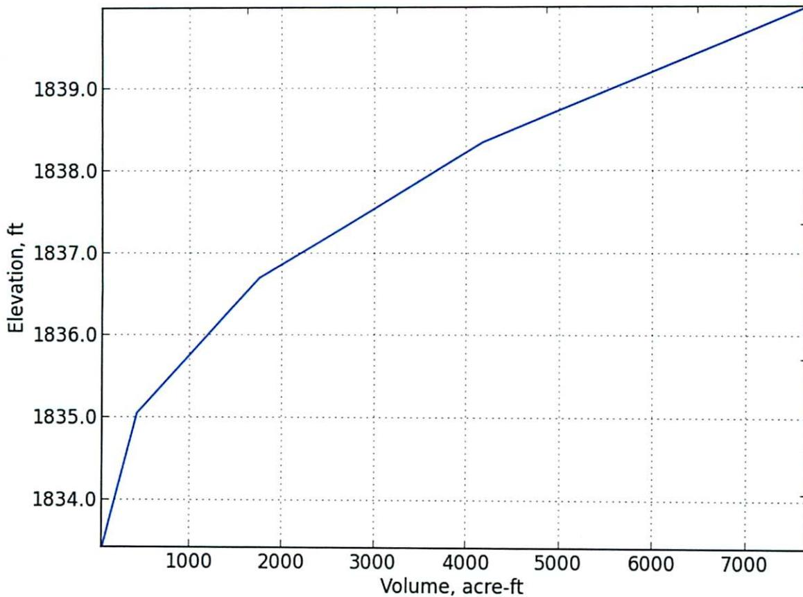
**Figure 5.** Tolley Slough elevation-capacity curve.
