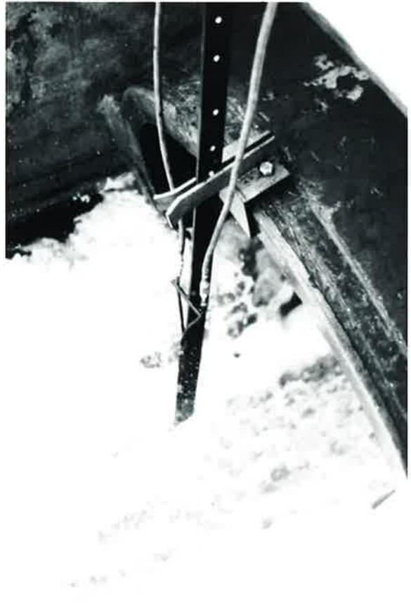
Photo 7. Pitot Tube in Place with Restraining Bracket
