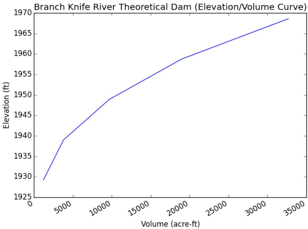
**Figure 4.** Branch Knife River subbasin theoretical dam (elevation/volume curve).
