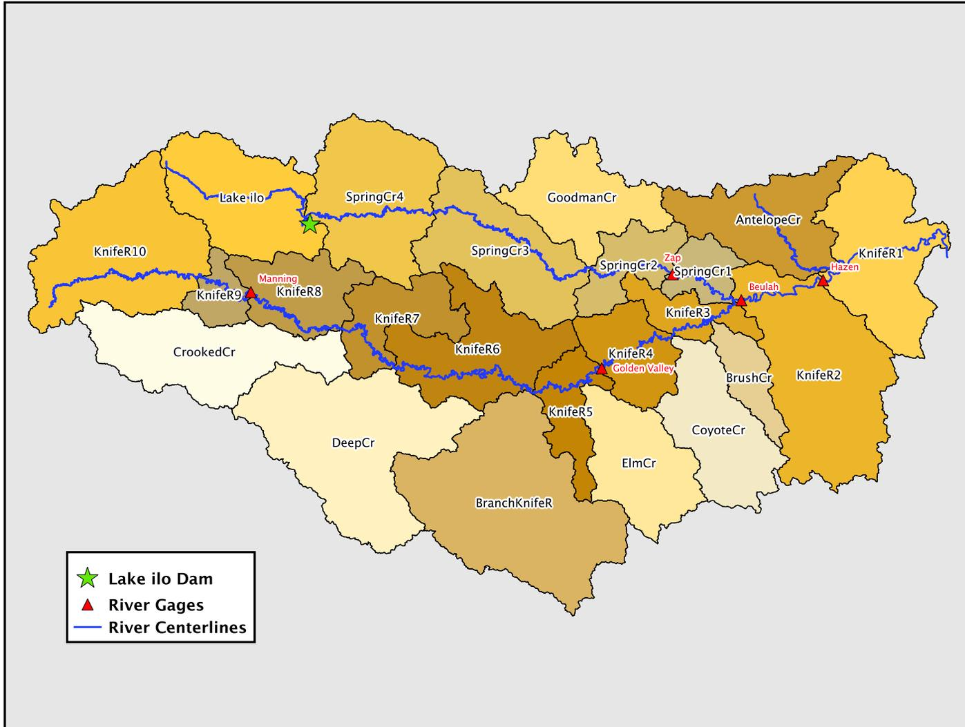
**Figure 2:** Sub-basins of the Knife River Basin used in the hydrology model.
