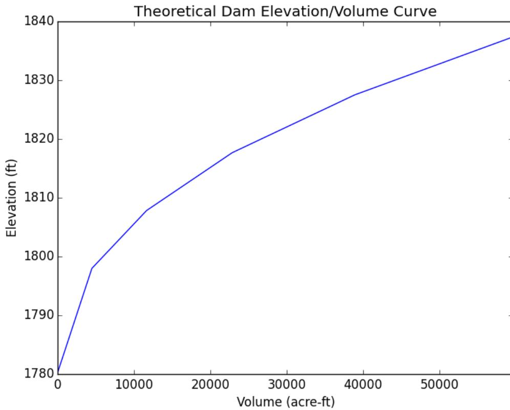
**Figure 9.** Spring Creek theoretical dam (elevation/volume curve).
