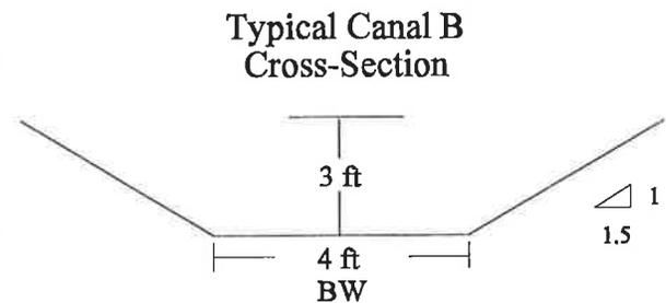
its laterals. It has a range in bottom width from 2-6 ft, and 1.5:1 side slopes, and has a designed
