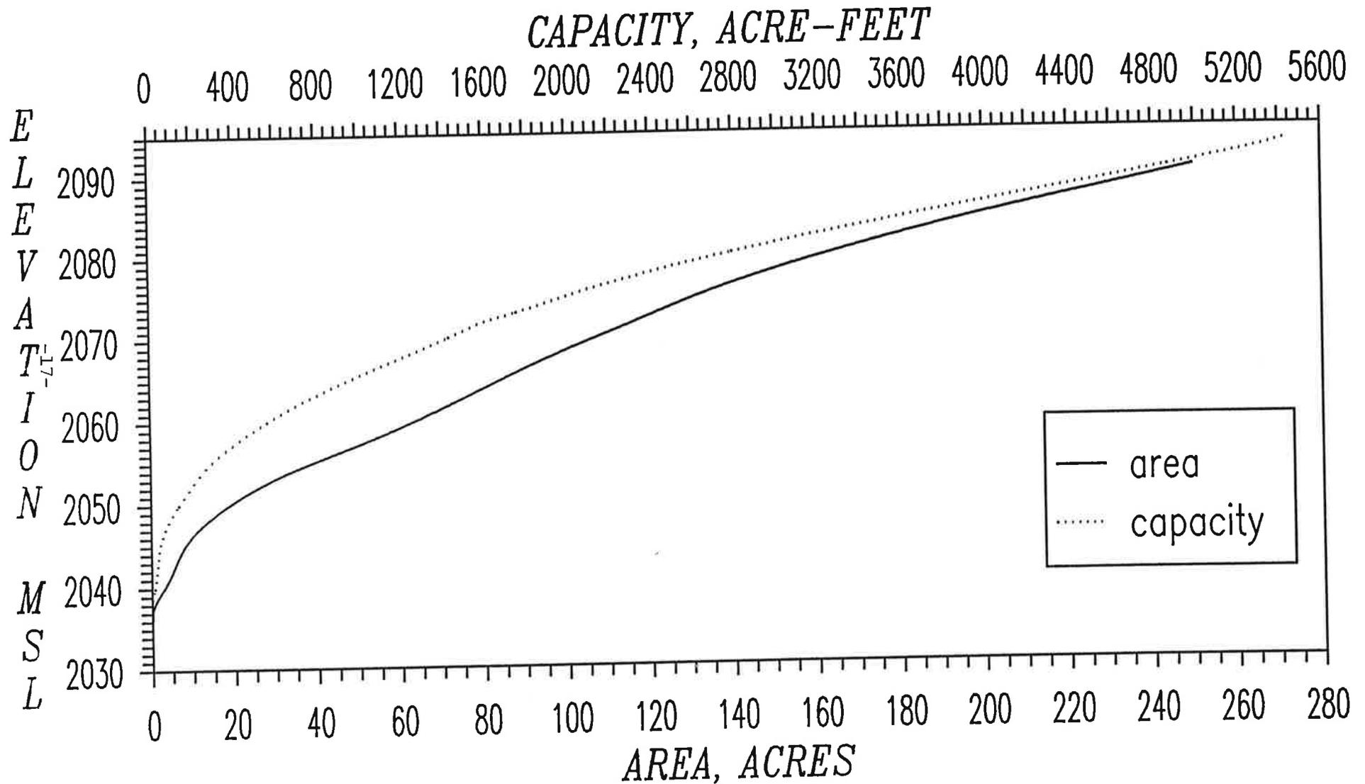
Figure 4 - Area Capacity Curve
