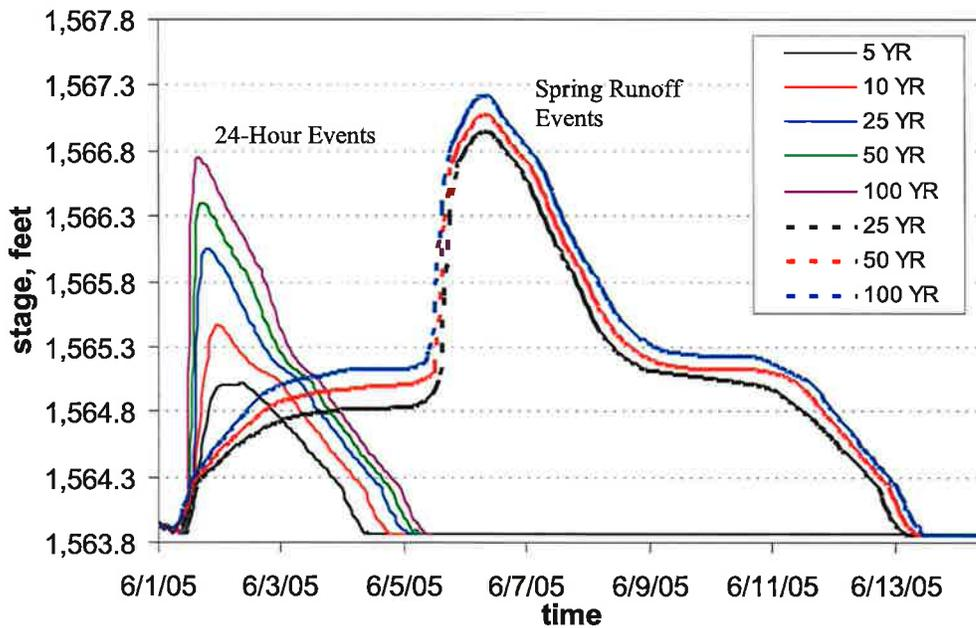
Figure 10. Stage hydrograph at cross section -6 for existing conditions.
