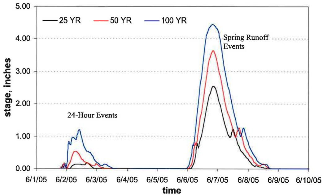
**Figure 18. Increase in stage as a result of removing Culvert #1 and raising the E-W township road.**
