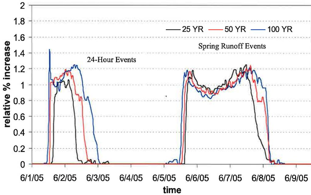
Figure 9. Relative percent difference in outflow caused by removal of Culvert #1.
