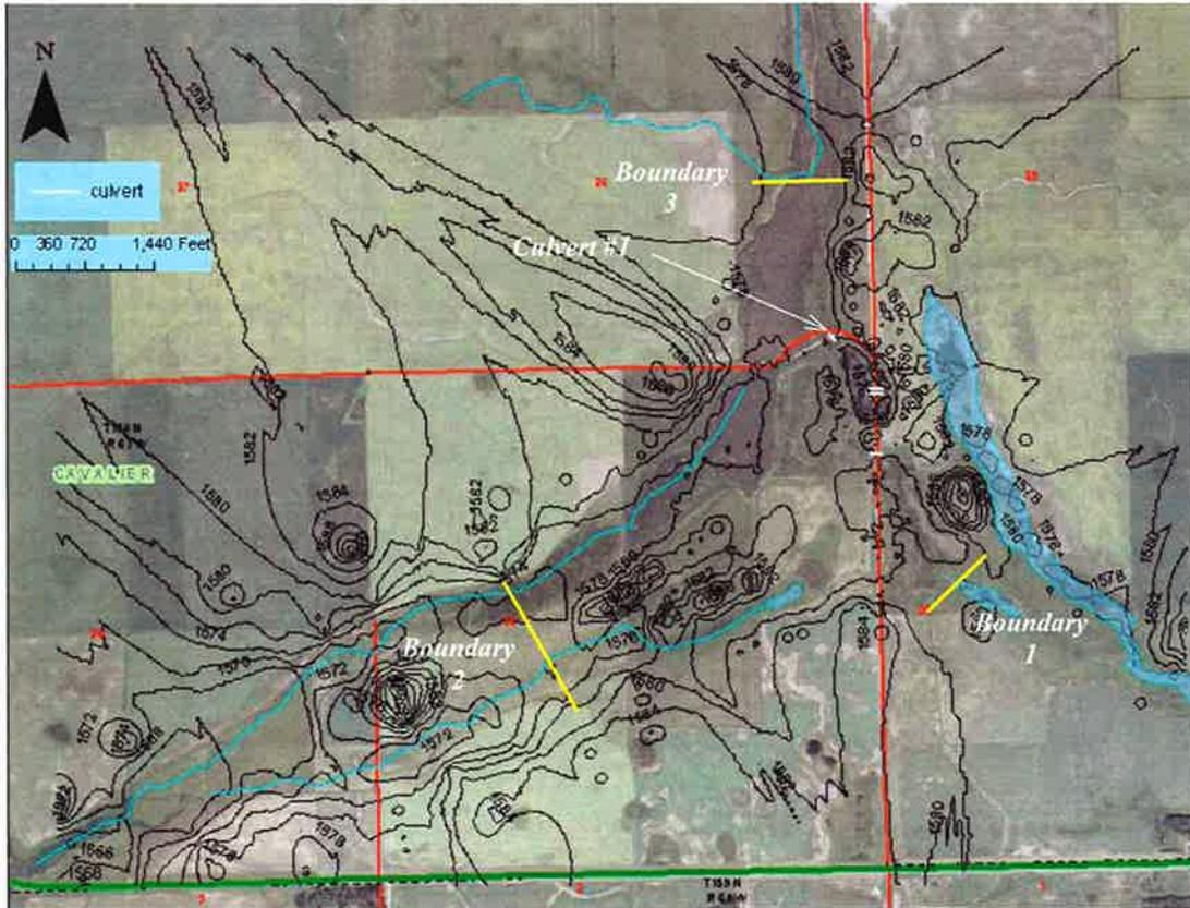
**Figure 3. Contour Map (Counter Intervals = 2 ft.) based off survey data. Culverts locations are also given on the township roads.**
