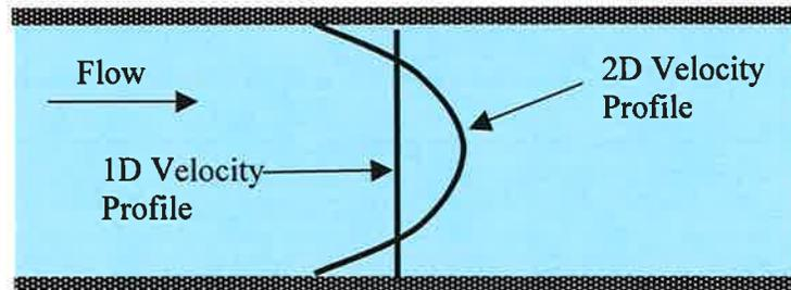
**Figure 4. One dimensional and two dimensional flow in a channel (plane view).**
