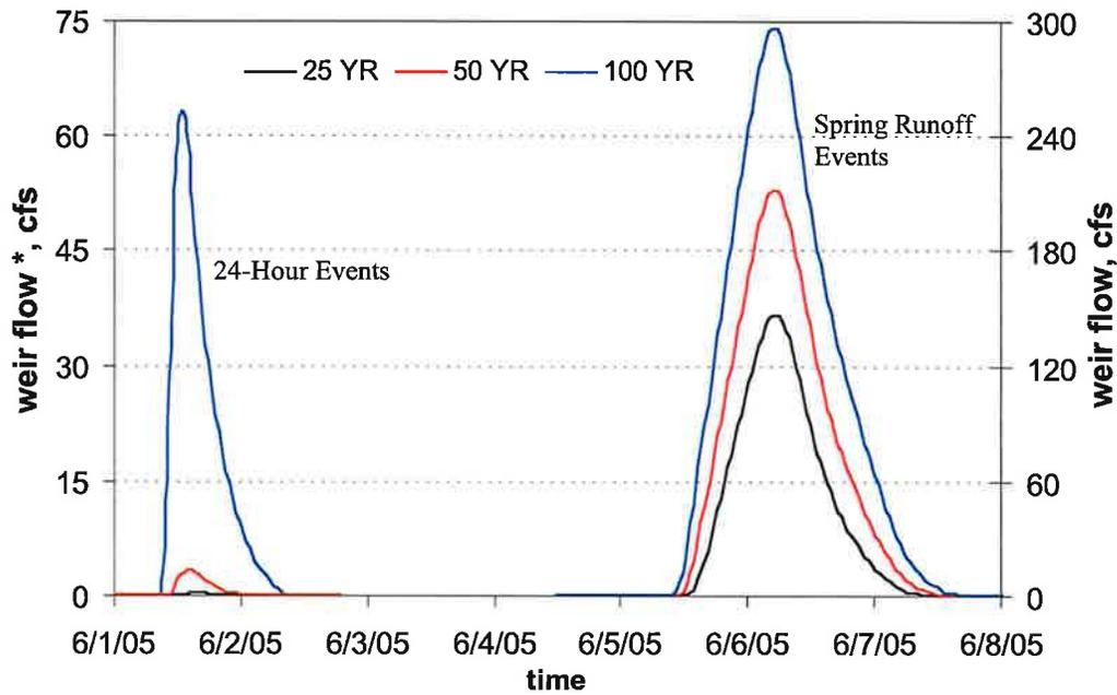
**Figure 15. Total weir flow over E-W township road. Axis with \* corresponds with 24 hour storm events.**
