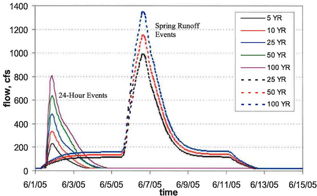
Figure 7. Inflow hydrographs for hydraulic model at *cross section 11*.
