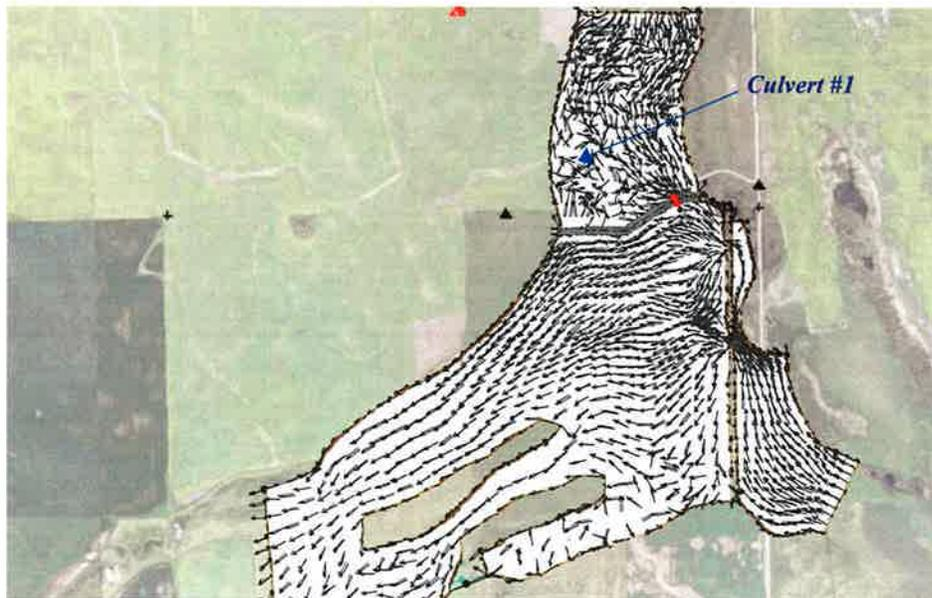
**Figure 5. Flow pattern showing divergent flow.**
