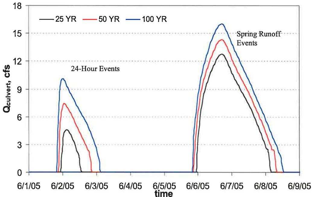
**Figure 14. Discharge of Culvert #1 to Snowflake Creek.**
