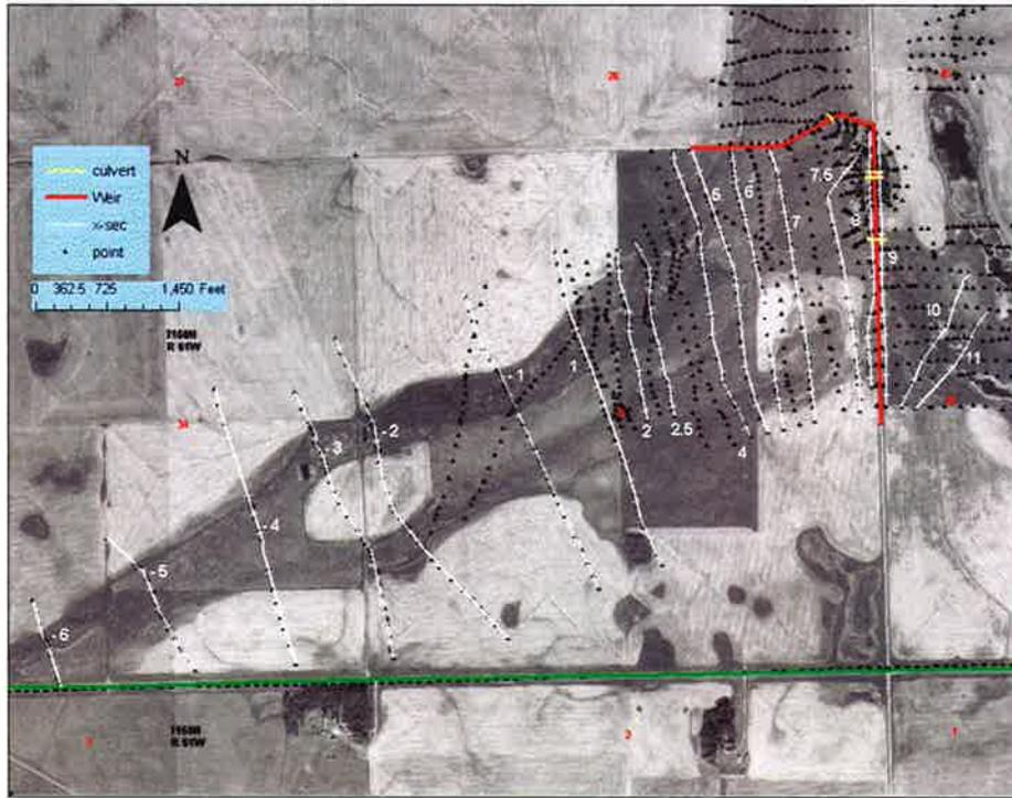
**Figure 6. Map illustrating cross sections, culverts, and roads modeled as weirs for one dimensional model. Survey points are also shown.**
