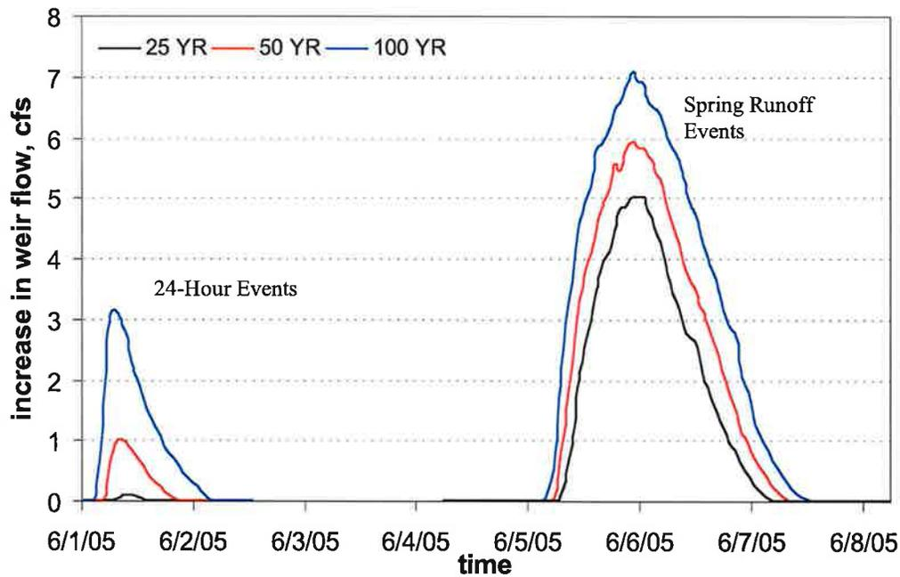
**Figure 16. Increase in discharge to Snowflake creek by weir flow over the E-W township road caused by removing Culvert #1.**
