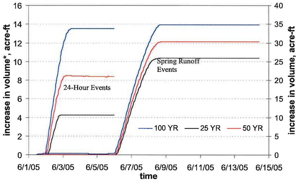
Figure 13. Increase in volume discharged as a result of removing the Culvert #1. Axis with \* corresponds with 24 hour storm events.
