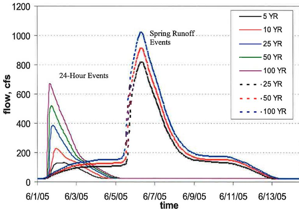
**Figure 8. Outflow hydrograph at *cross section -6* for hydraulic model with existing conditions.**
