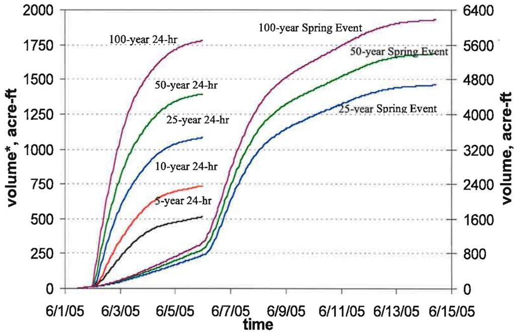
Figure 12. Volume discharged from hydraulic model at *cross section -6* for existing conditions. Axis with \* corresponds 24 hour storm events.
