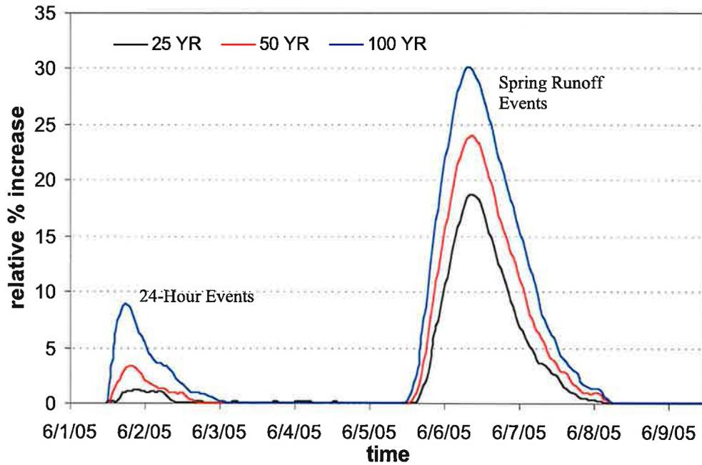
**Figure 17. Relative percent increase in discharge resulting from removal of Culvert #1 and raising the E-W township road.**
