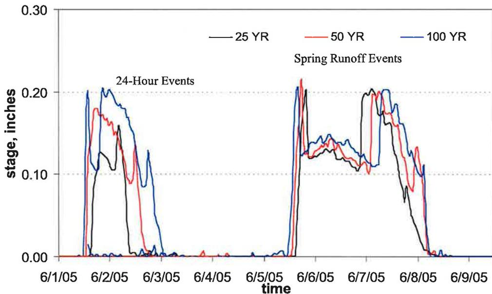
**Figure 11. Stage difference between the case of Culvert #1 removed and existing conditions.**
