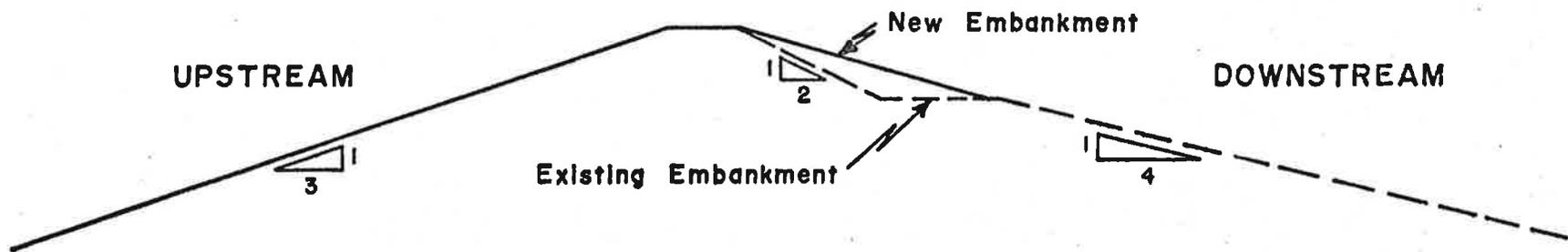
TYPICAL CROSS-SECTION BETWEEN STA. 5+00 AND STA. 9+31
