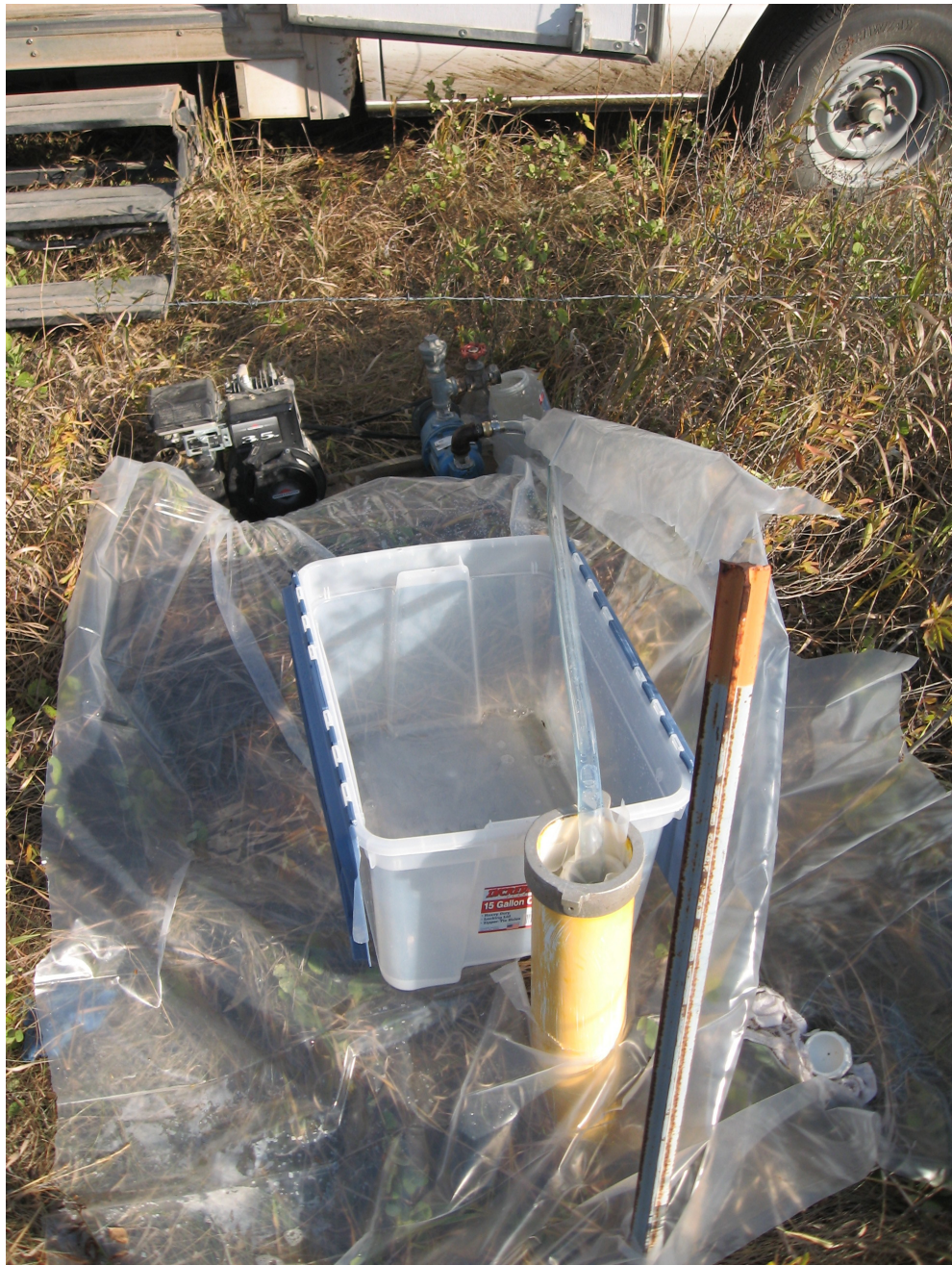
Photo 2. Evacuating well using suction (screw) pump. (2013 sampling used an electric motor powered by the truck battery through an accessory connector in place of the gasoline engine shown.)
