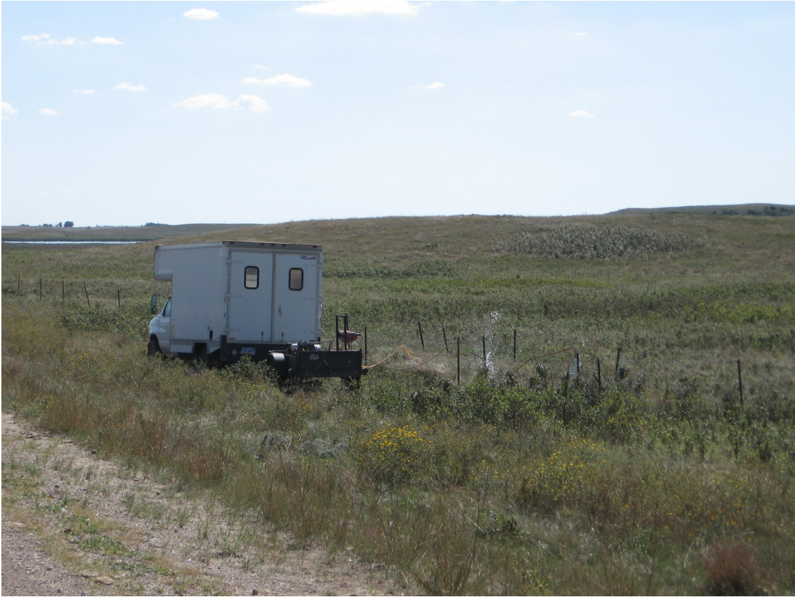
Photo 1. Air-pressure lift used for evacuating wells used for general chemistry sampling.
