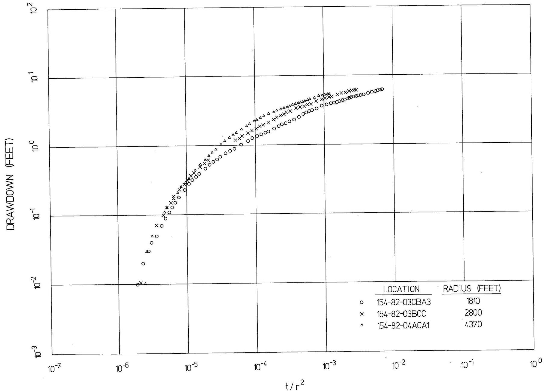
FIGURE 19. Logarithmic plots of drawdown versus  $t/r$  for 3 observation wells monitored during the 1969 Sunde Aquifer test.
