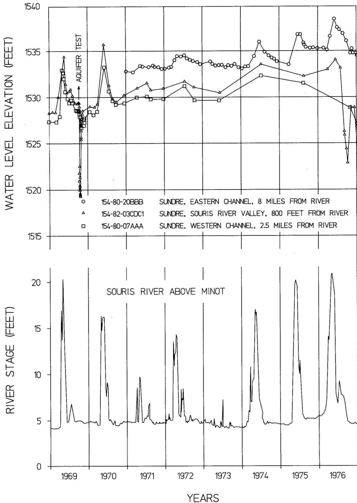
**FIGURE 10. Hydrographs of water levels from representative Sindre Aquifer observation wells versus gage height of the Souris River above Minot (1969-1976).**
