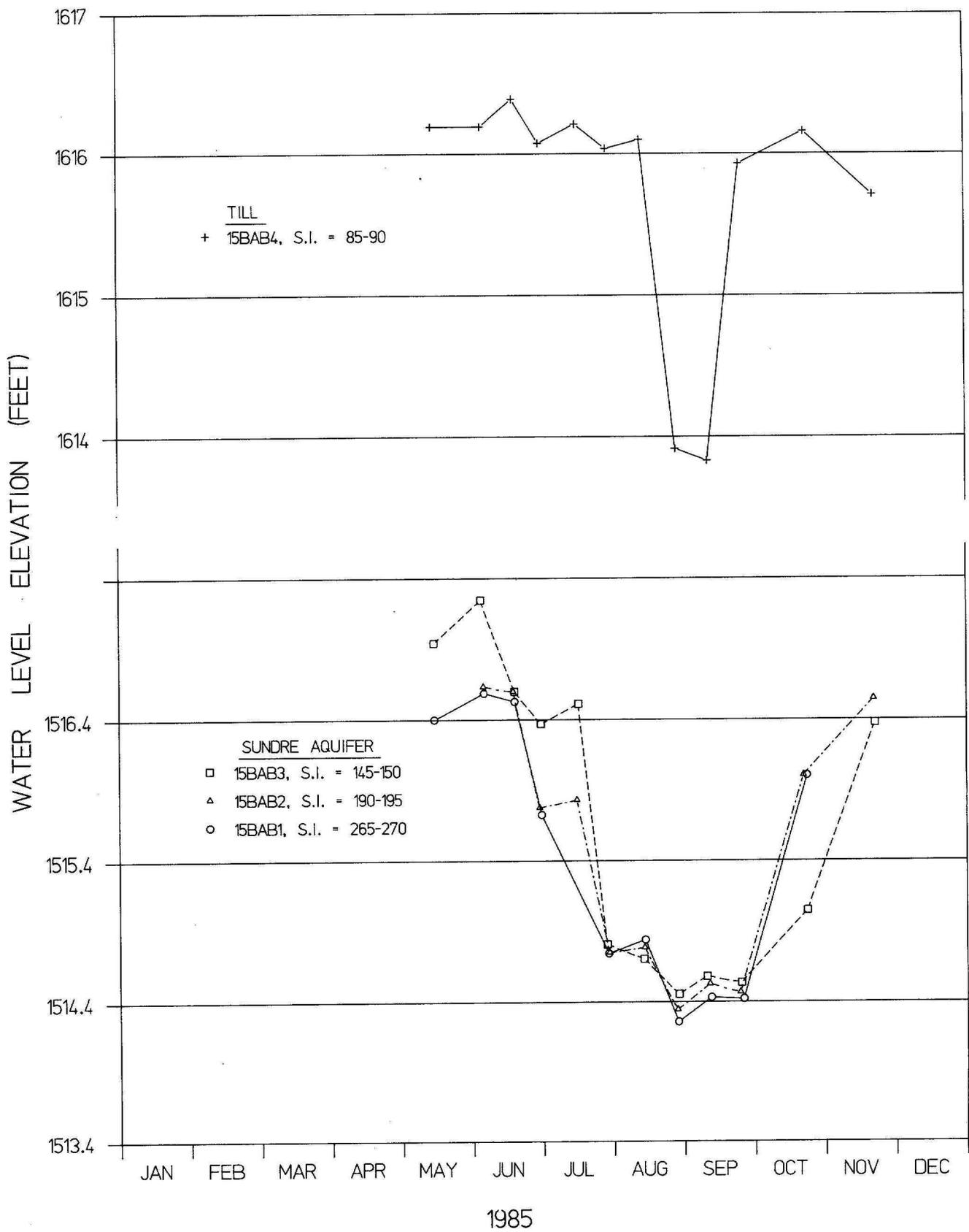
**FIGURE 28. Hydrographs of water levels from piezometer nest 154-81-15BAB showing the vertical distribution of water levels in the eastern channel of the Sunde Aquifer system.**
