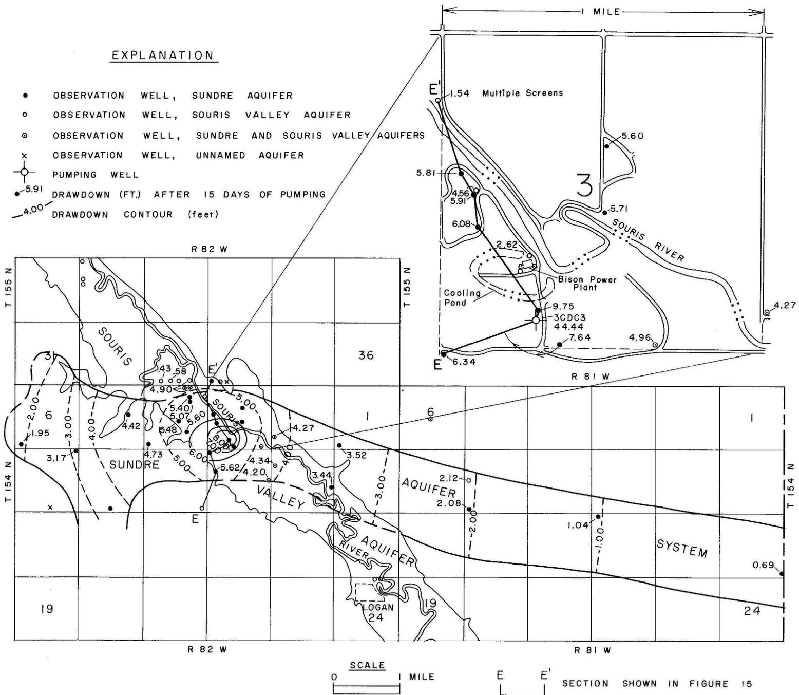
**FIGURE 14. Location of observation wells measured during the Soudre Aquifer test of 10-20-69 to 11-03-69 and drawdown in the Soudre Aquifer System after pumping [well 154-82-03CDC3] at 1950 gpm for 15 days.**
