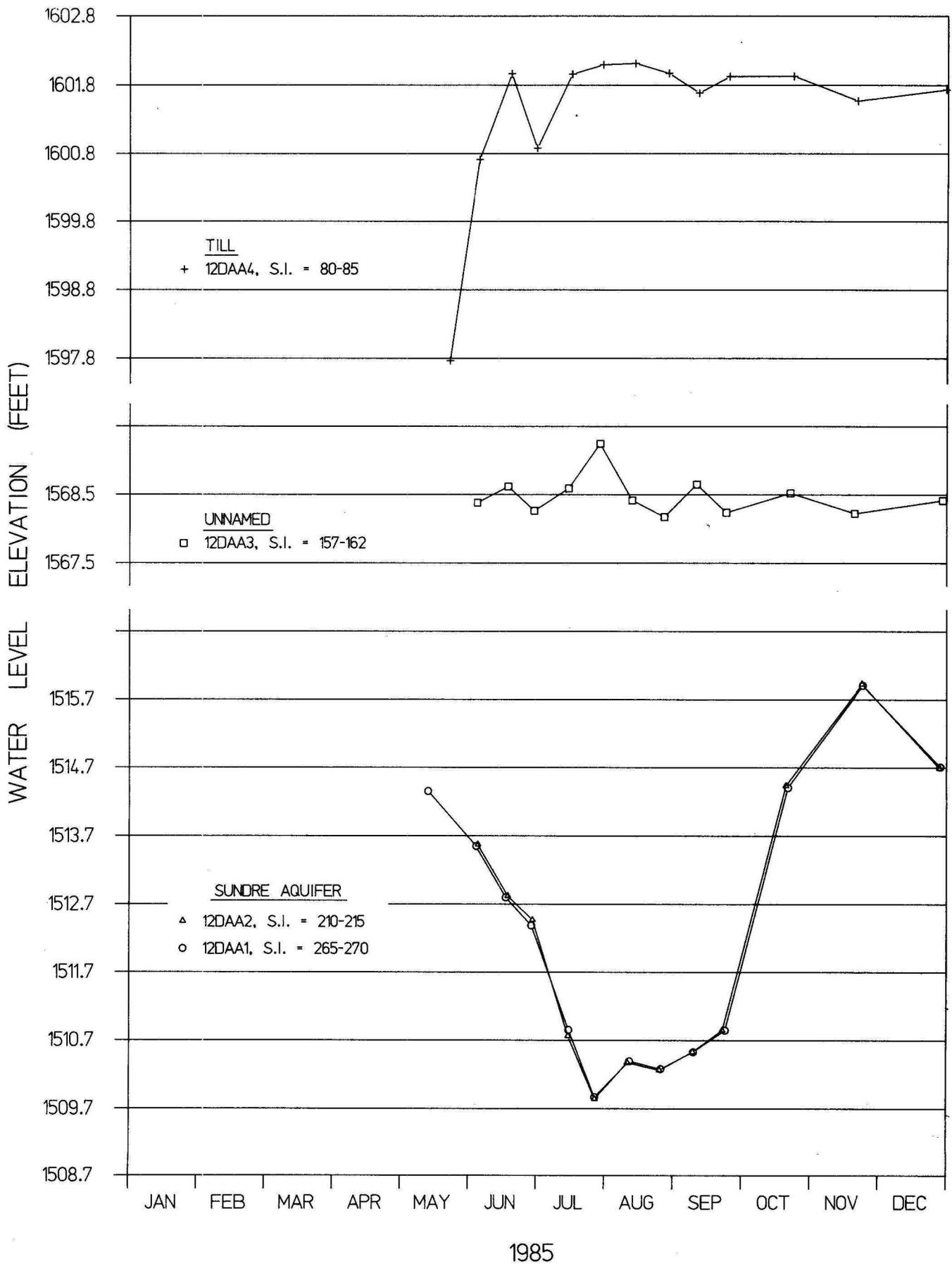
**FIGURE 27. Hydrographs of water levels from piezometer nest 154-82-12DAA showing the vertical distribution of water levels in the Souris Valley and Sindre Aquifer systems.**
