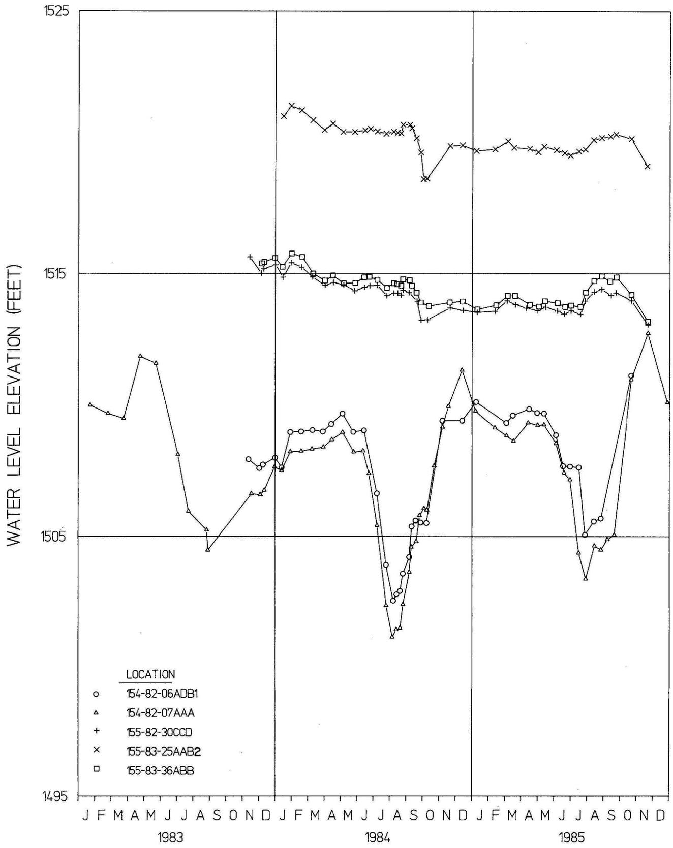
**FIGURE 30. Hydrographs comparing water levels from observation wells screened in the western channel of the Sunde Aquifer system.**
