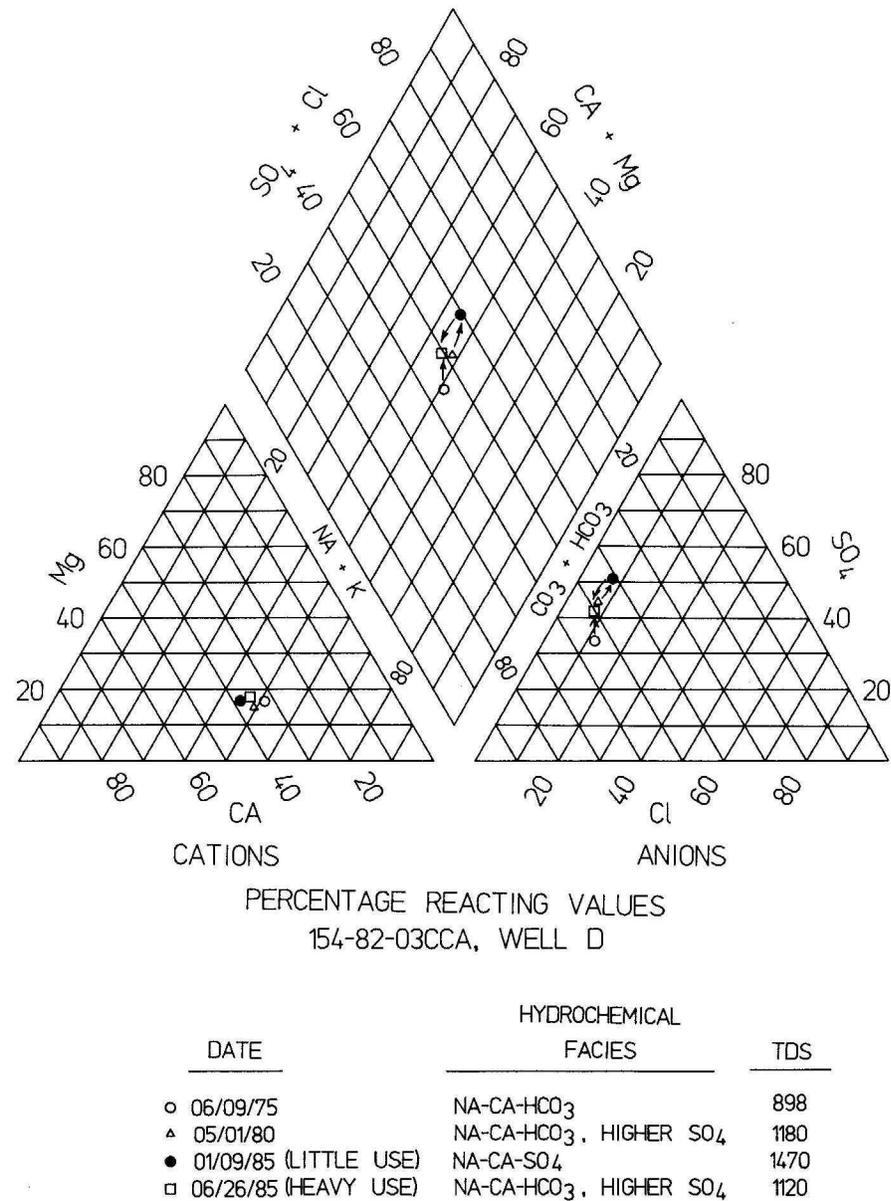
**FIGURE 49. Schoeller and Piper diagrams showing temporal variations in selected cations and anions in the Sindre Aquifer, Minot production well D.**
