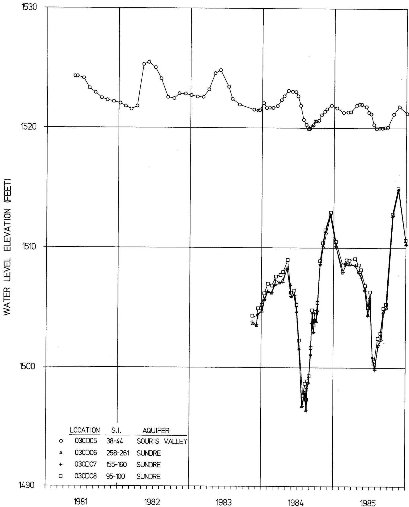
**FIGURE 26. Hydrographs of water levels from piezometer nest 154-082-03CDC showing the vertical distribution of water levels in the Souris Valley and Sindre Aquifer systems.**
