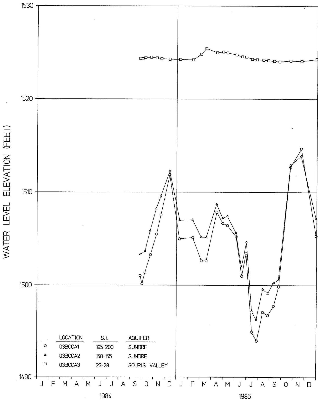
**FIGURE 21. Hydrographs of water levels from piezometer nest 154-082-03BCCA showing the vertical distribution of water levels in the Souris Valley and Sundre Aquifer systems.**
