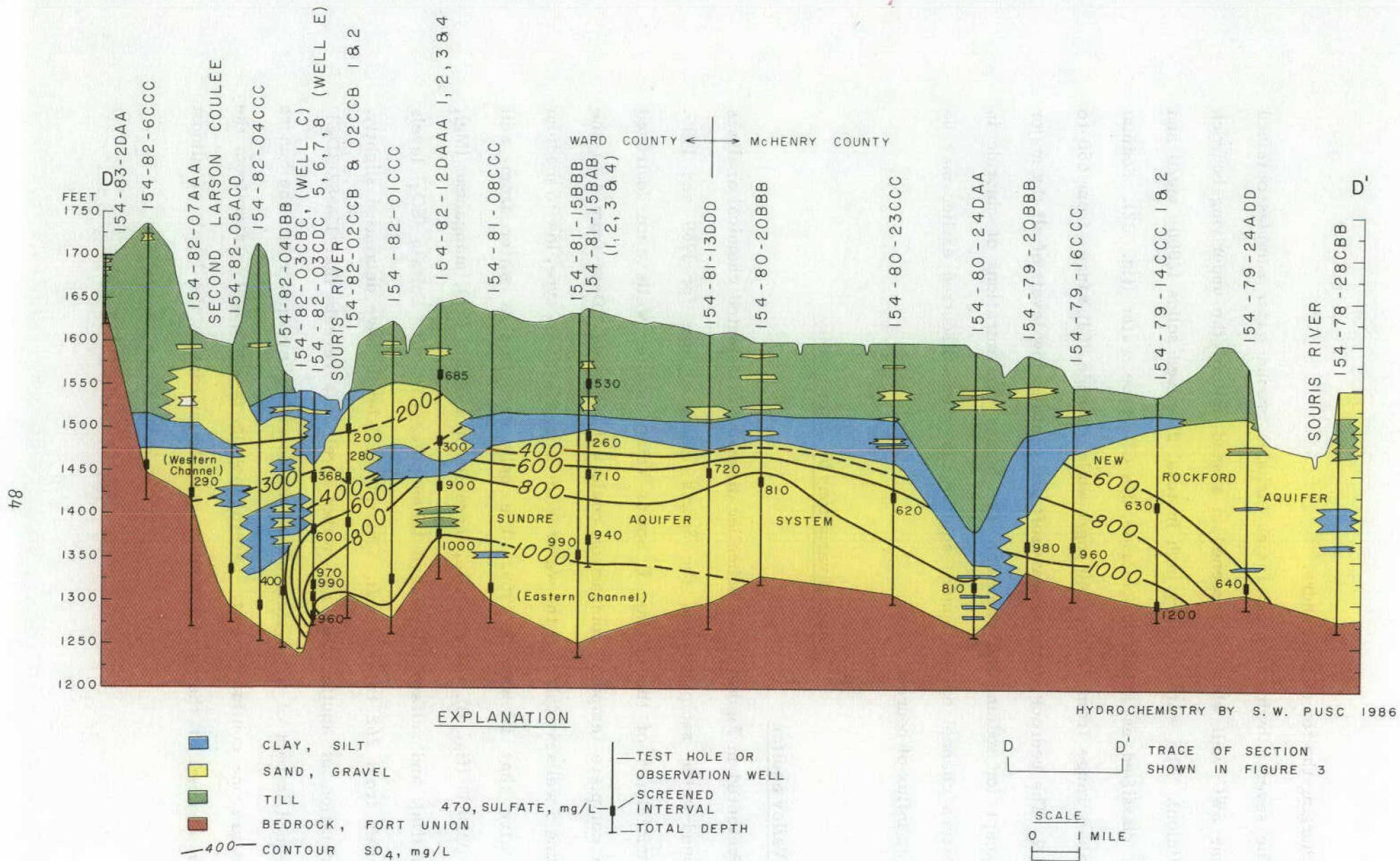
FIGURE 40. Vertical distribution of sulfate ( $SO_4$ ) in the Sindre Aquifer using water quality data from observation wells completed along the axis of the channel (6-27-85 sample).
