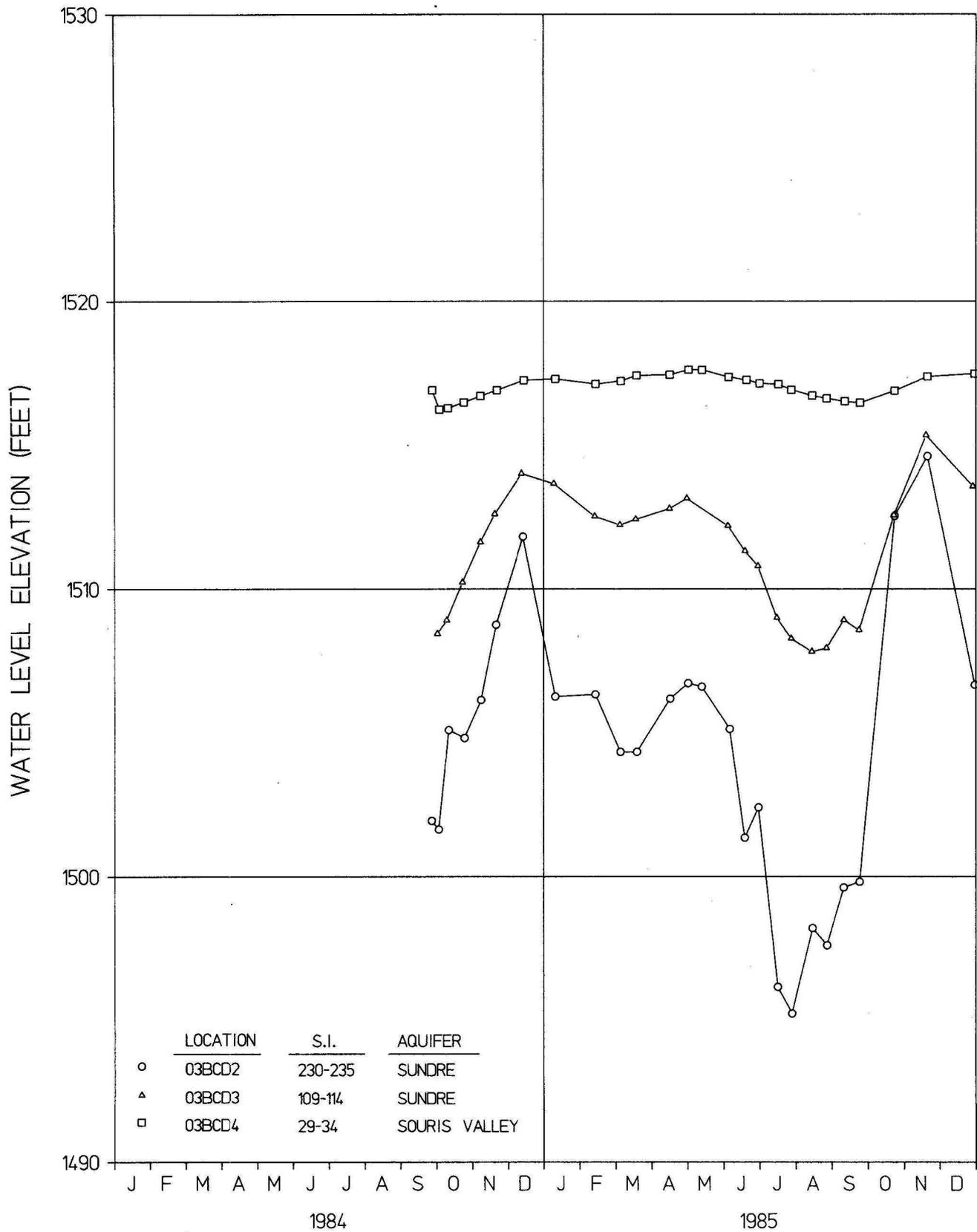
**FIGURE 22. Hydrographs of water levels from piezometer nest 154-082-03BCD showing the vertical distribution of water levels in the Souris Valley and Sandre Aquifer systems.**
