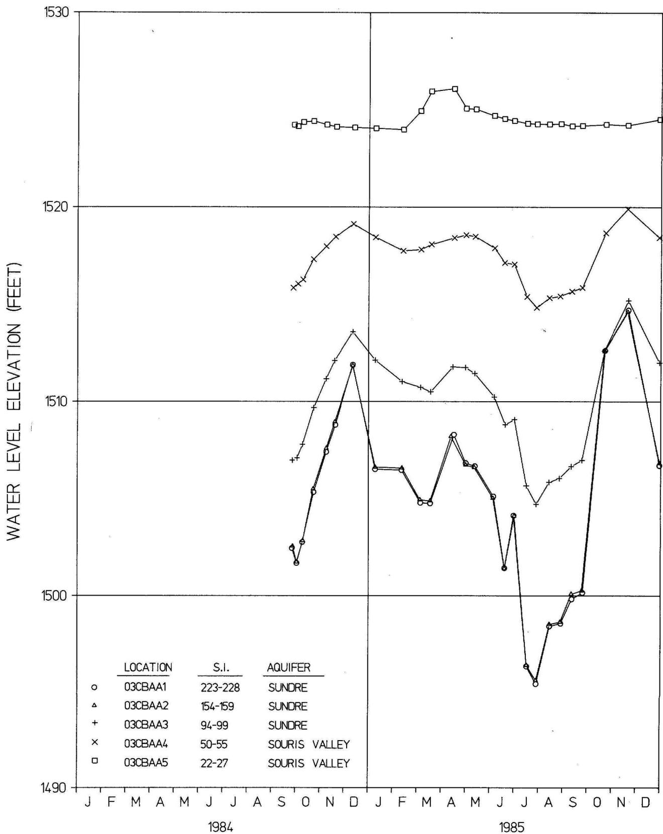
**FIGURE 23. Hydrographs of water levels from piezometer nest 154-082-03CBAA showing the vertical distribution of water levels in the Souris Valley and Sunde Aquifer systems.**
