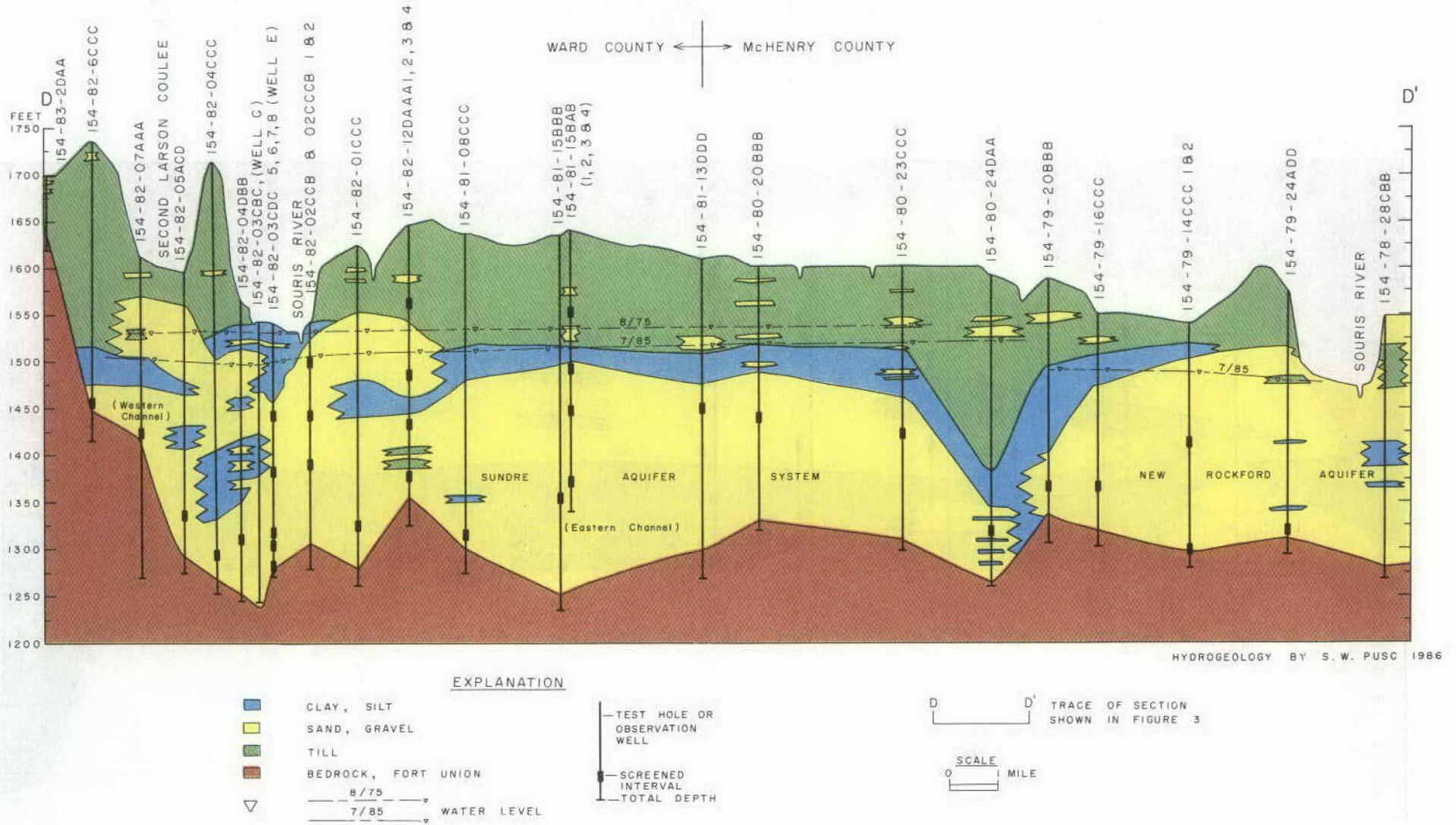
**FIGURE 7. Hydrogeologic section D-D' along the axis of the Sundre Aquifer system and the New Rockford Aquifer.**
