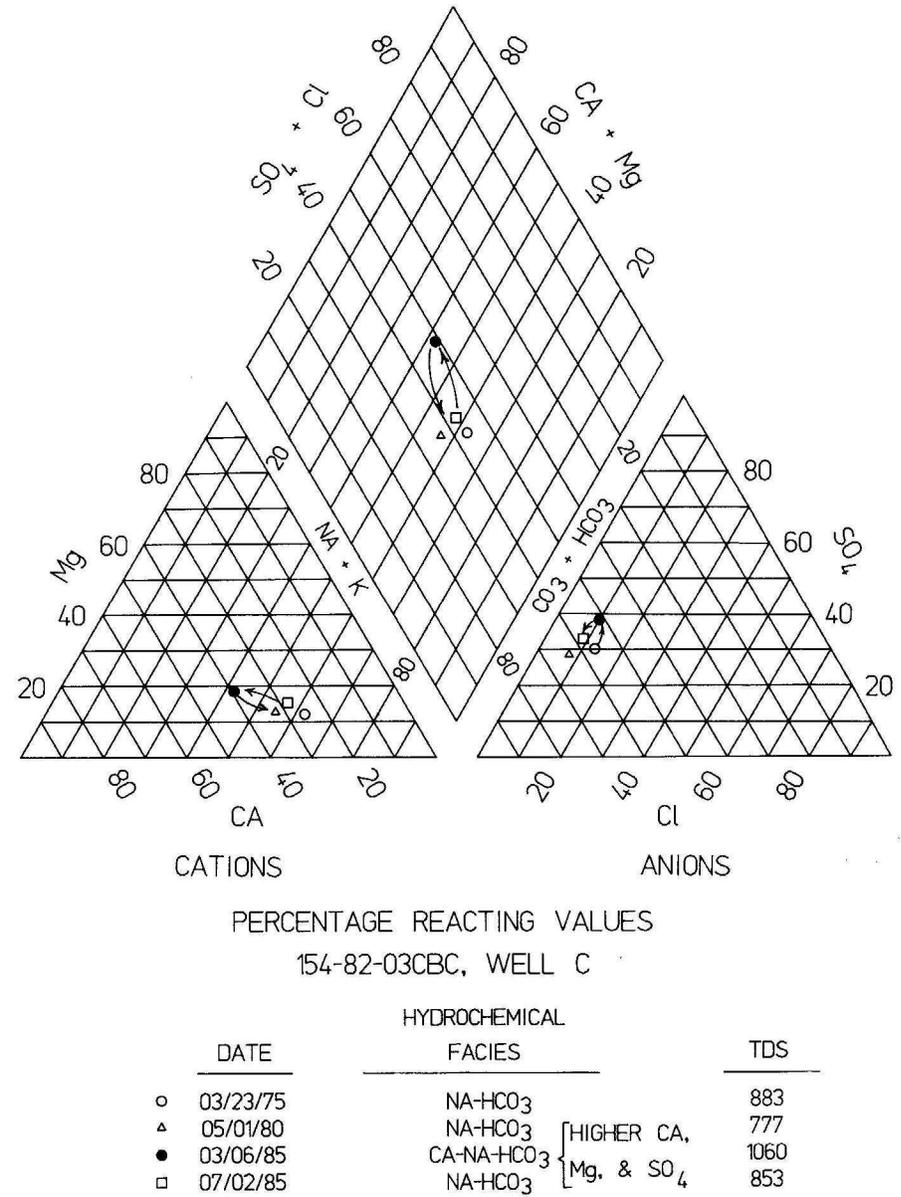
**FIGURE 46. Schoeller and Piper diagrams showing temporal variations in selected cations and anions in the Sindre Aquifer, Minot production well C.**
