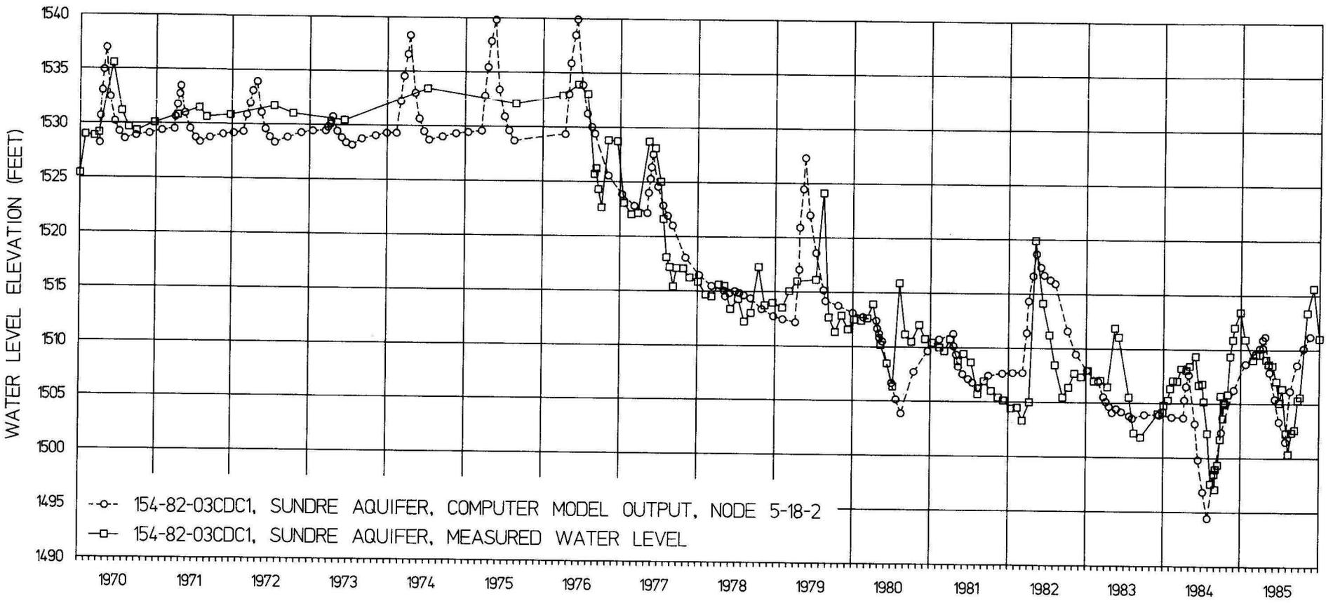
**FIGURE 53. Hydrographs comparing measured water levels versus transient computer generated water levels for 154-82-03CDC1, Sindre Aquifer in Souris River Valley.**
