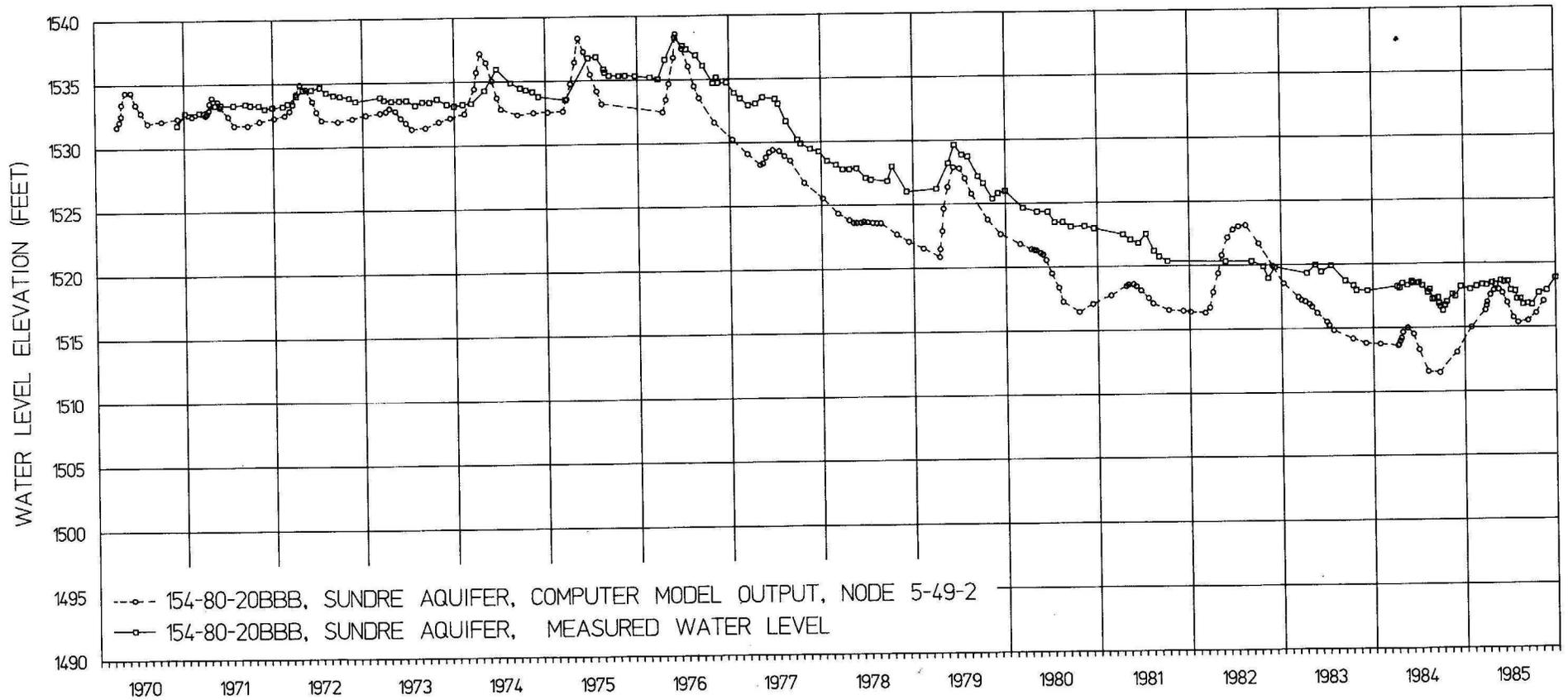
**FIGURE 54. Hydrographs comparing measured water levels versus transient computer generated water levels for 154-80-20BBB, Sundre Aquifer, eastern channel.**
