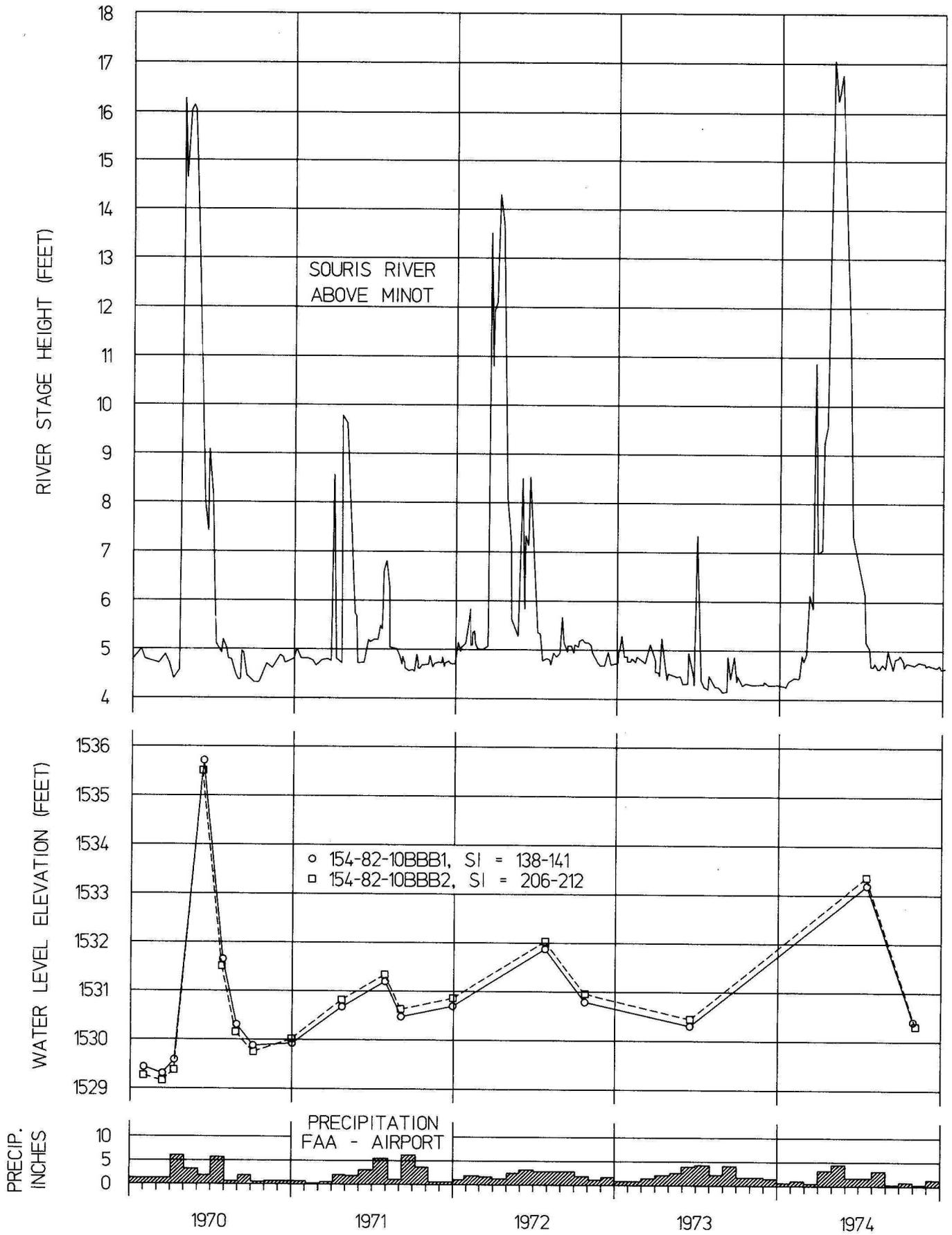
**FIGURE 8. Hydrographs of water levels from observation wells 154-82-10BBB 1 & 2 versus gage height of the Souris River above Minot.**
