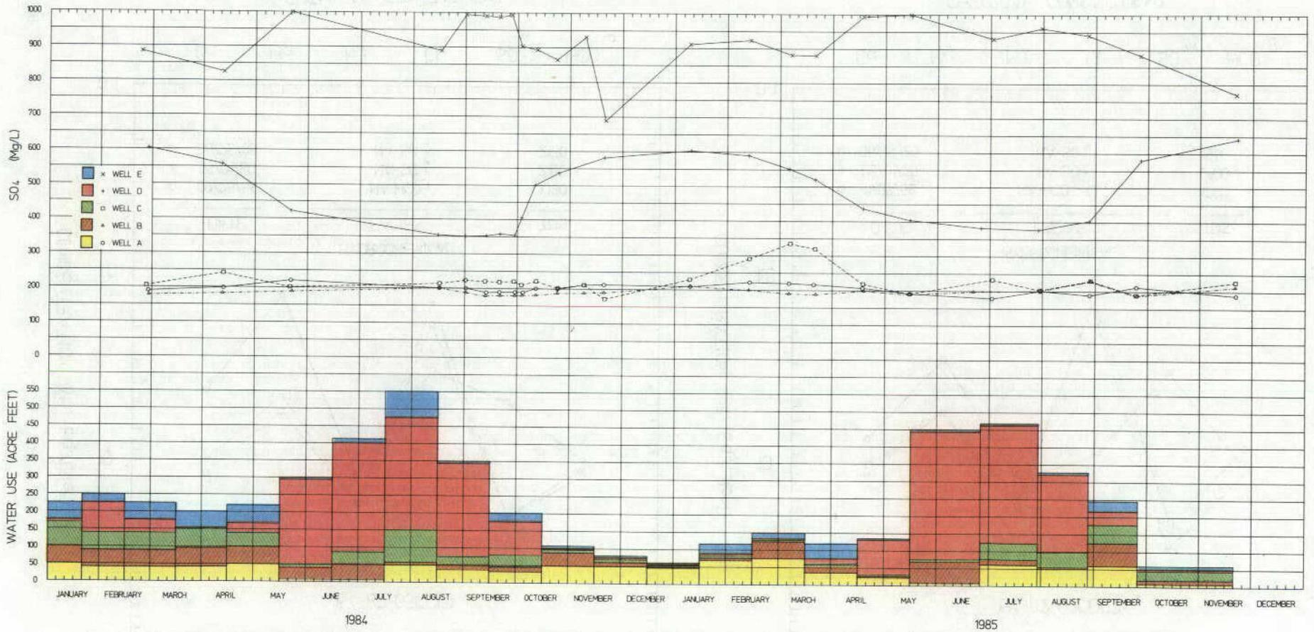
FIGURE 47. Comparison of water use and sulfate (SO<sub>4</sub>) levels in ground water from Minot production wells A, B, C, D, and E.
