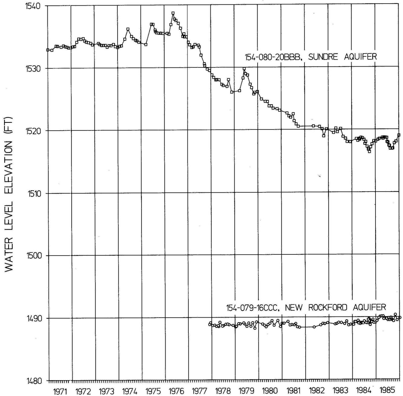
**FIGURE 29. Hydrographs comparing water level elevations in the eastern channel of the Sundre Aquifer versus water level elevations in the adjoining New Rockford Aquifer.**
