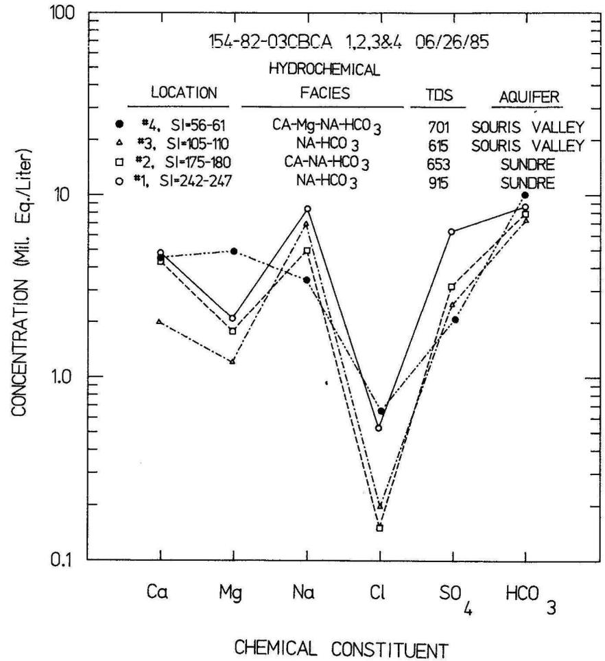
FIGURE 45. Schoeller diagrams showing temporal variations and vertical distribution in selected cations and anions in the Sundre Aquifer east and southeast of Minot production well C.
