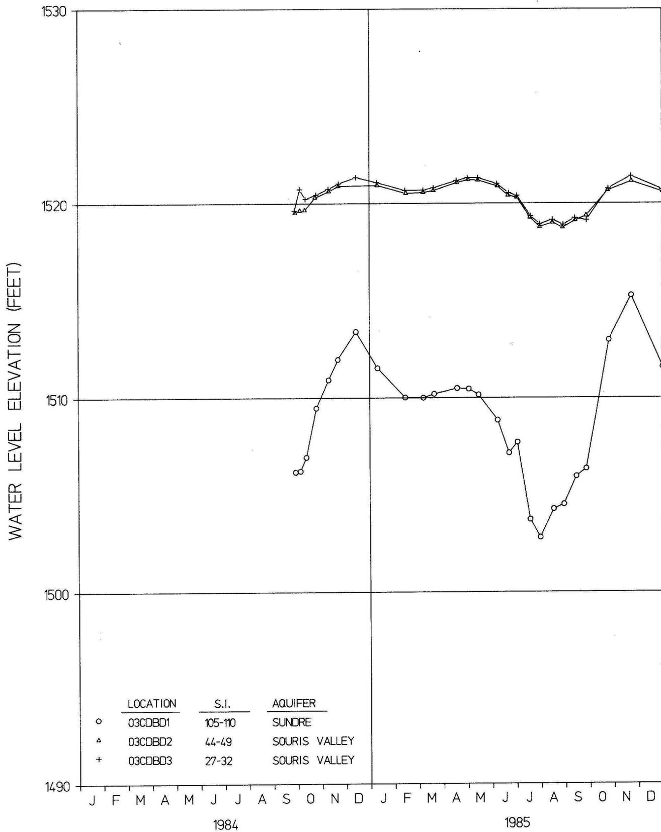
**FIGURE 25. Hydrographs of water levels from piezometer nest 154-082-03CDBD showing the vertical distribution of water levels in the Souris Valley and Sunde Aquifer systems.**
