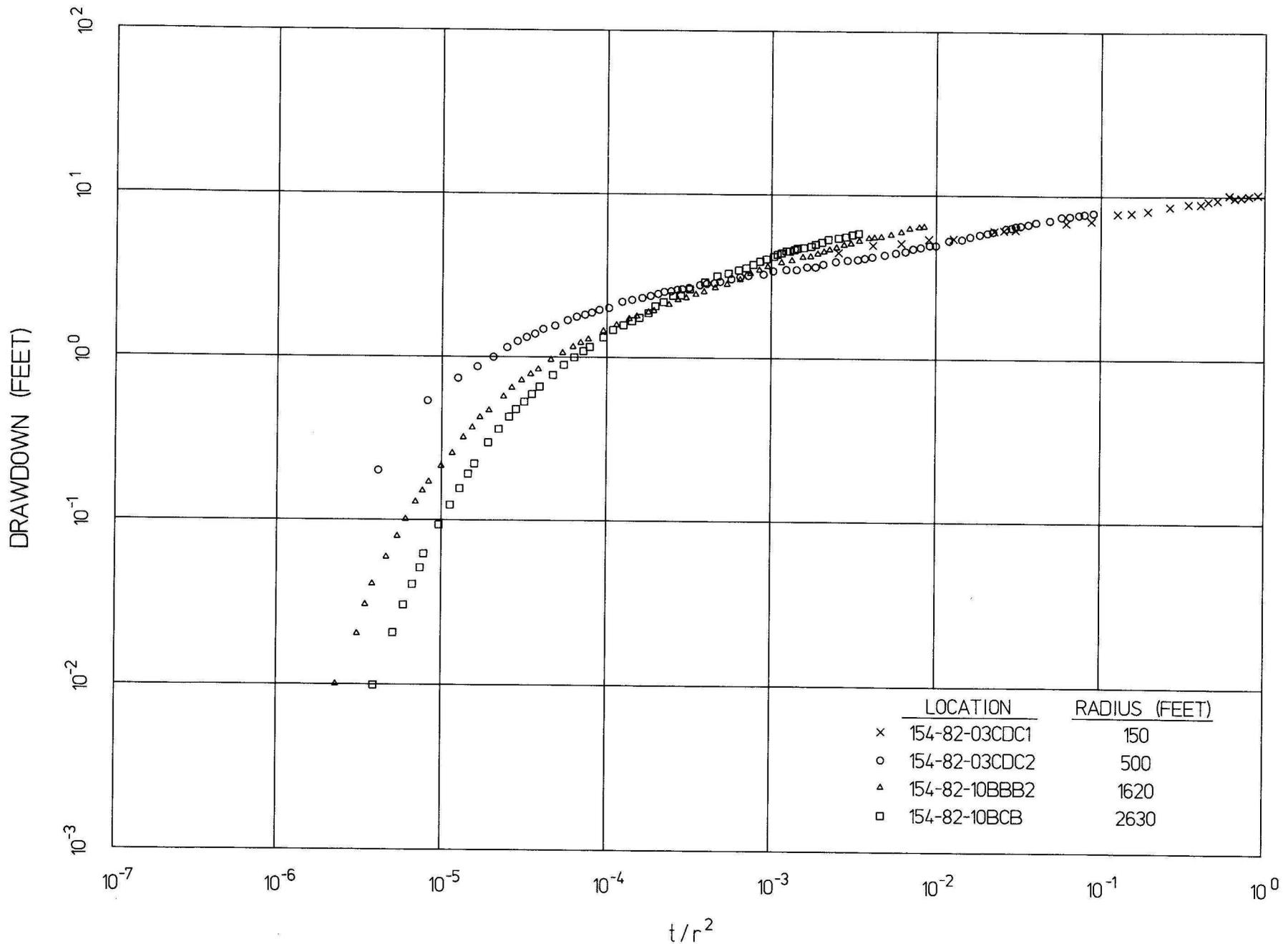
FIGURE 18. Logarithmic plots of drawdown versus  $t/r^2$  for 4 observation wells monitored during the 1969 Sunde Aquifer test.
