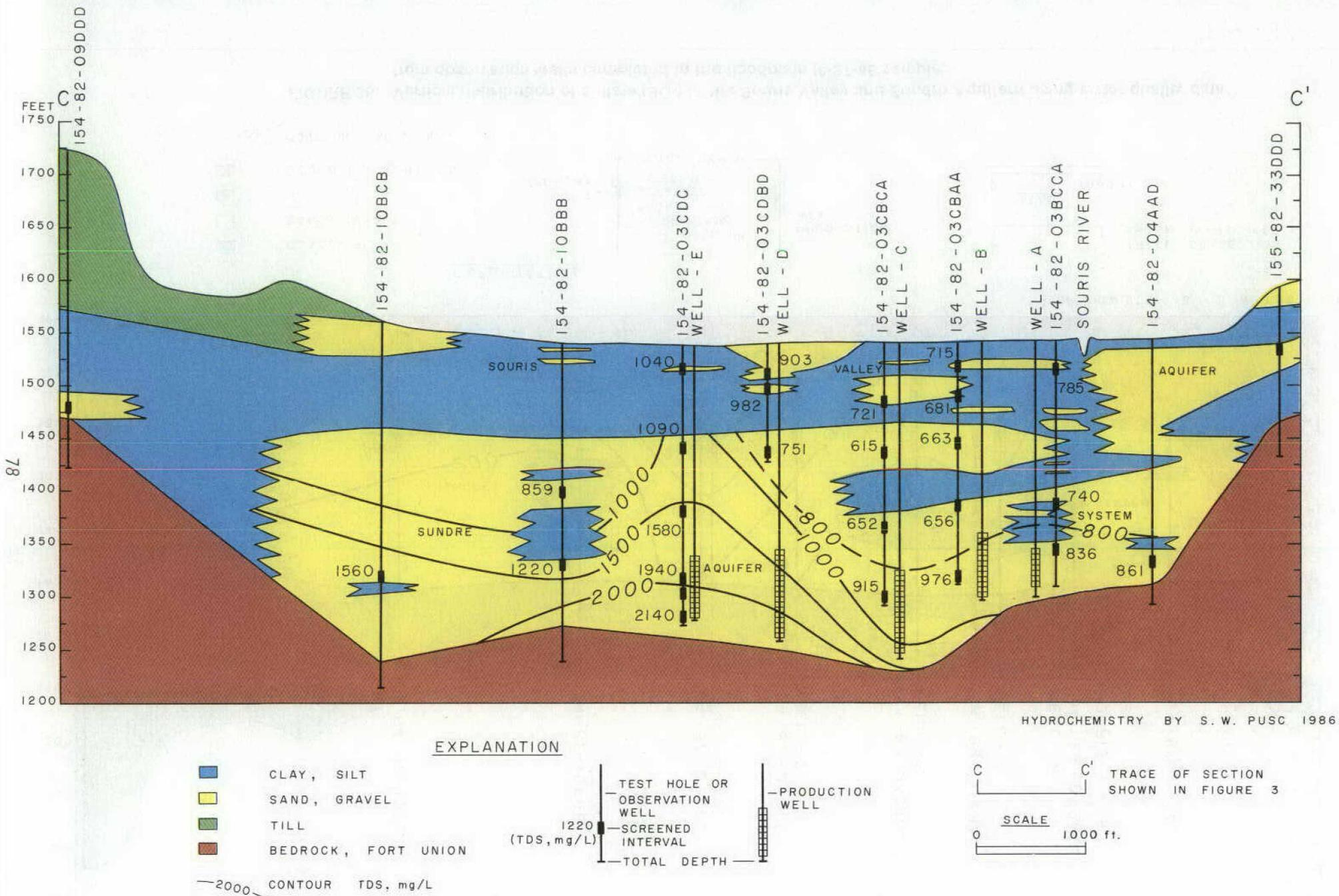
**FIGURE 35. Vertical distribution of total dissolved solids (TDS) in the Souris Valley and Sindre Aquifers using water quality data from observation wells completed in the floodplain (6-27-85 sample).**
