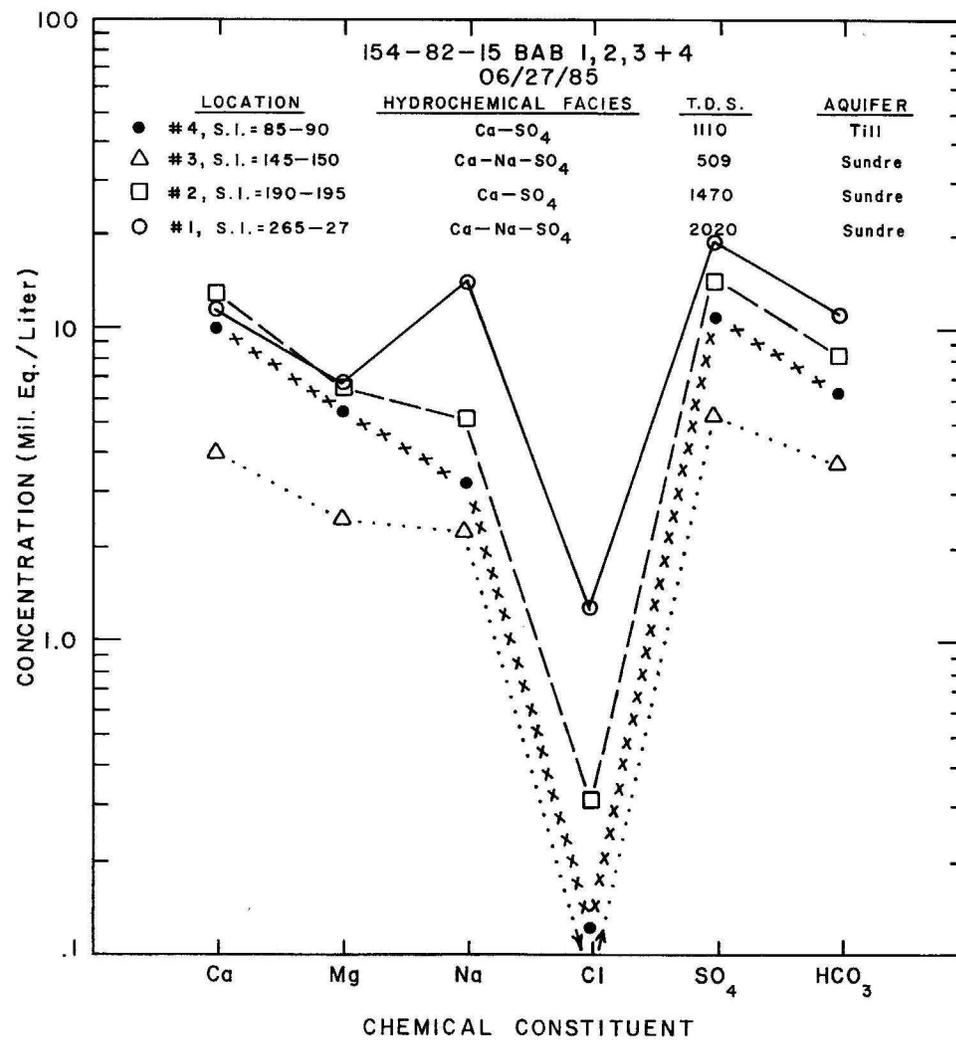
FIGURE 38. Schoeller diagrams showing the vertical distribution of selected cations and anions in the eastern channel of the Sundre aquifer.
