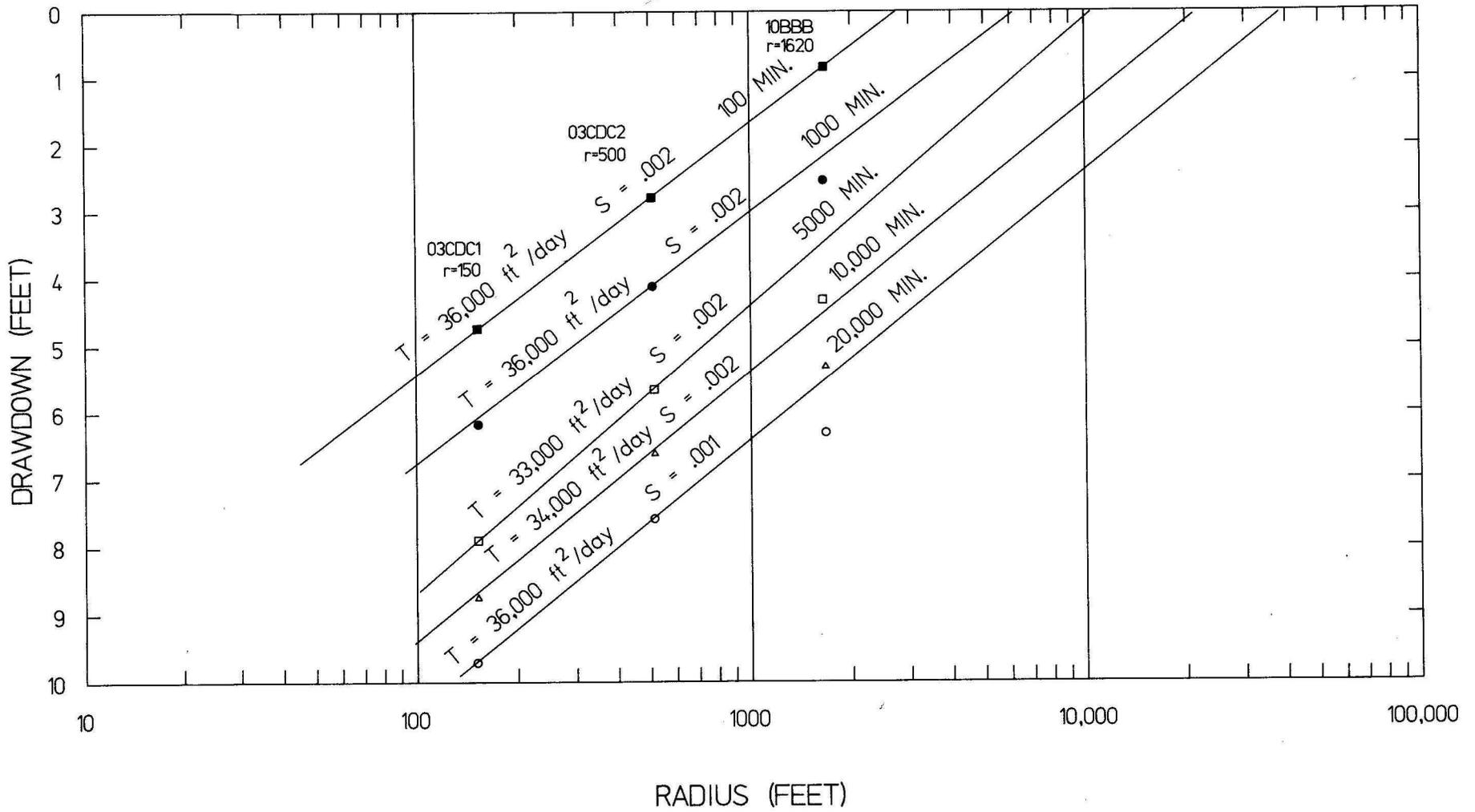
FIGURE 20. Semi-log plot of drawdown versus radius for the 1969 Sundre Aquifer test.
