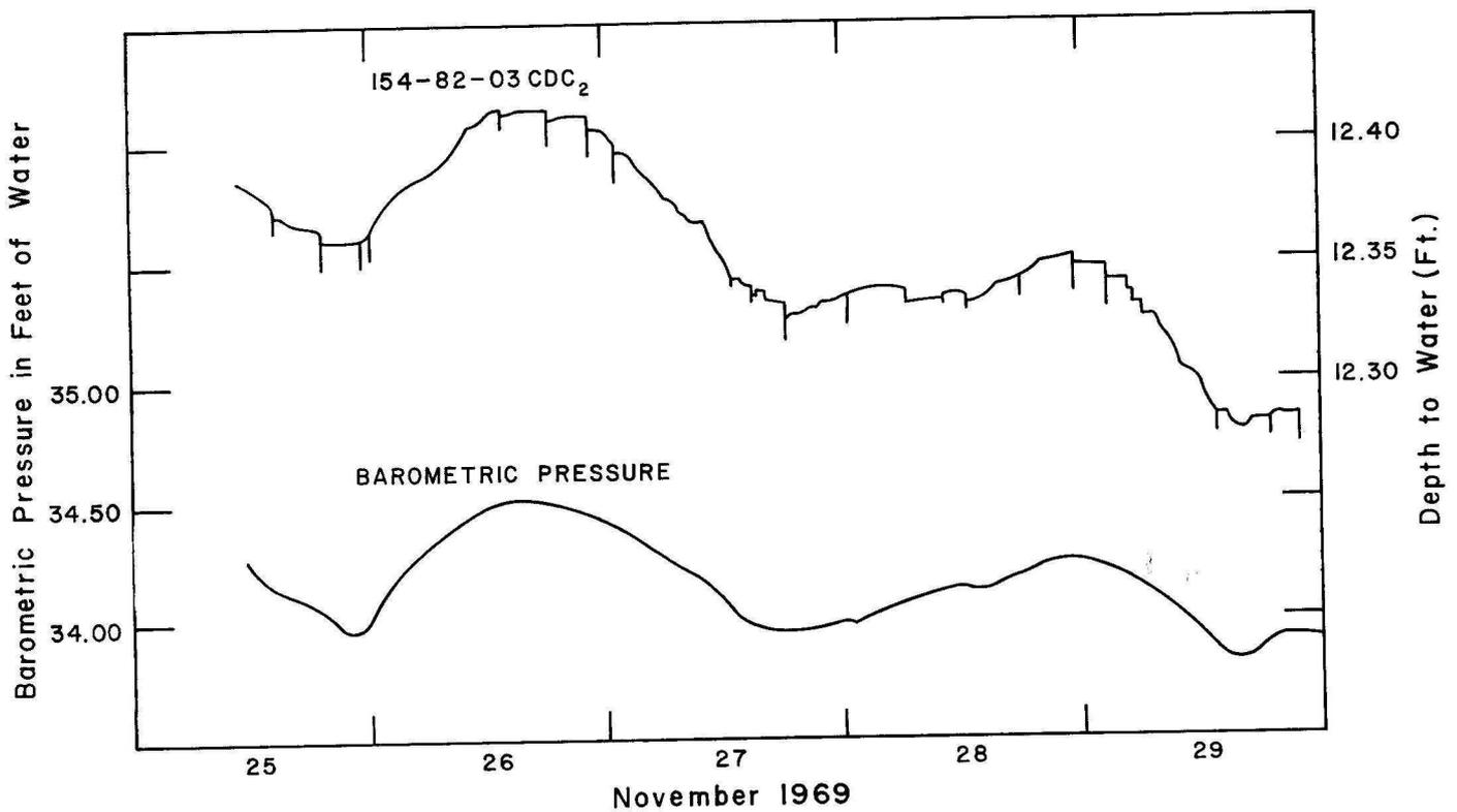
FIGURE 11. CORRELATION OF WATER LEVELS FROM OBSERVATION WELLS 154-82-03 CDC 1 AND 2 VERSUS BAROMETRIC PRESSURE
