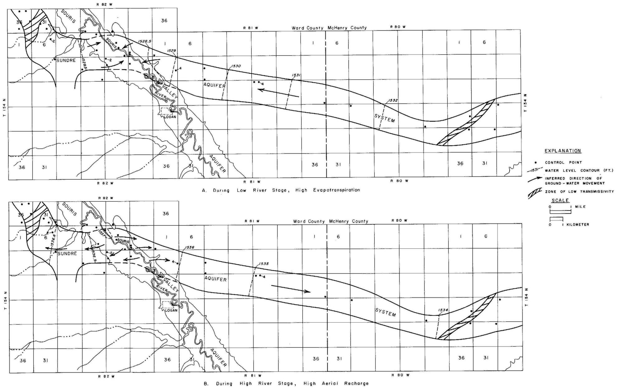
**FIGURE 55. Transient model generated water level contour maps during a low river stage event (A) and a high river stage event (B). Prior to development.**
