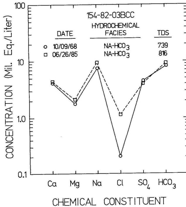
**FIGURE 43. Schoeller diagrams showing temporal variations in selected cations and anions in the Sindre Aquifer, north of the Souris River in Section 3 and near Minot production wells A & B.**
