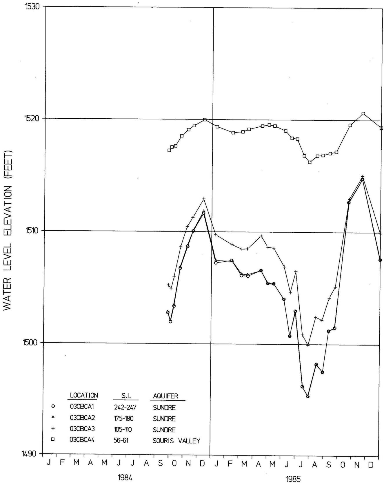
**FIGURE 24. Hydrographs of water levels from piezometer nest 154-082-03CBCA showing the vertical distribution of water levels in the Souris Valley and Sunde Aquifer systems.**
