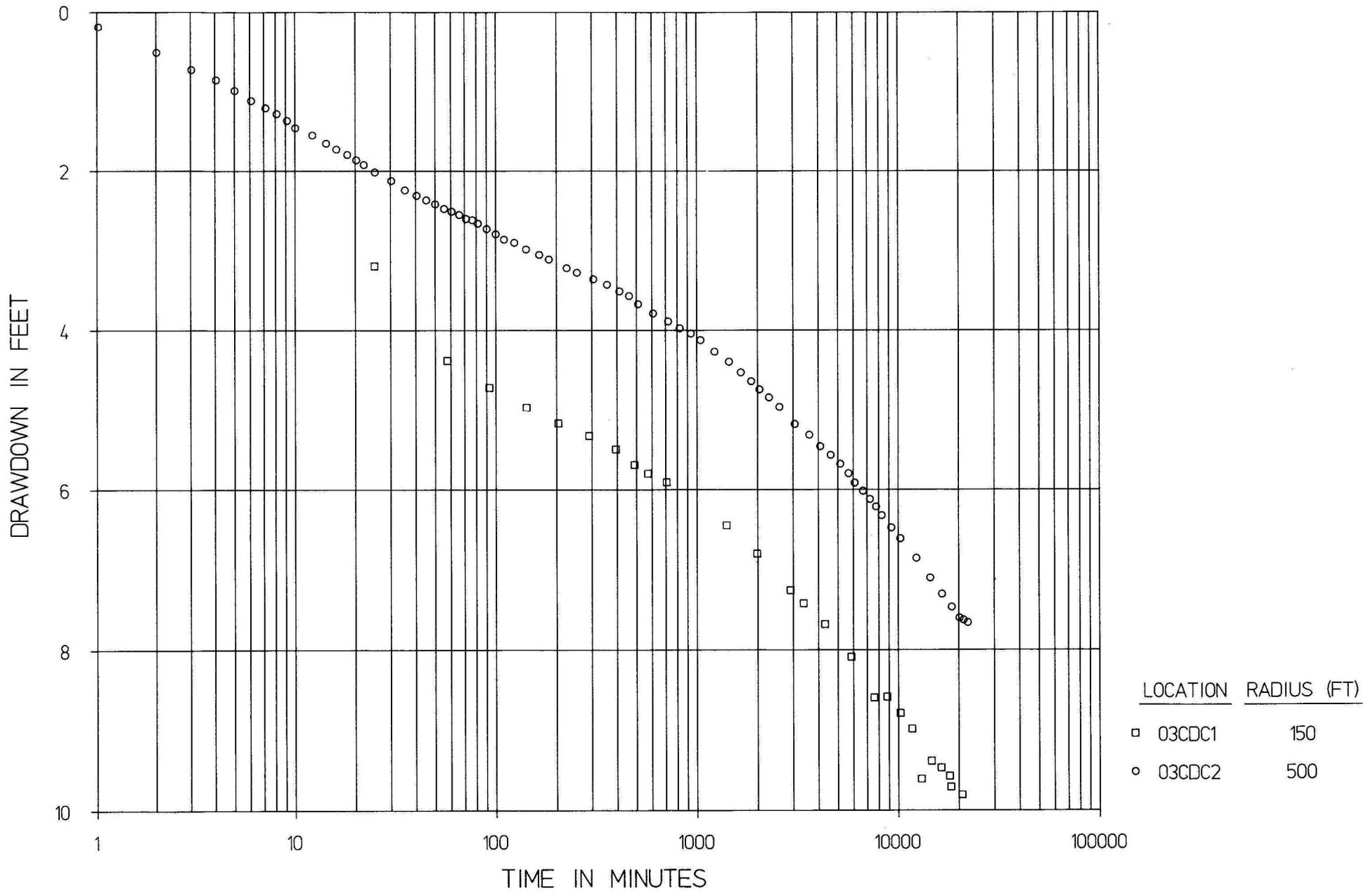
**FIGURE 17. Sem-log plot of drawdown versus time for observation wells 154-82-03CD 1 & 2 during the 1969 Sundre Aquifer test.**
