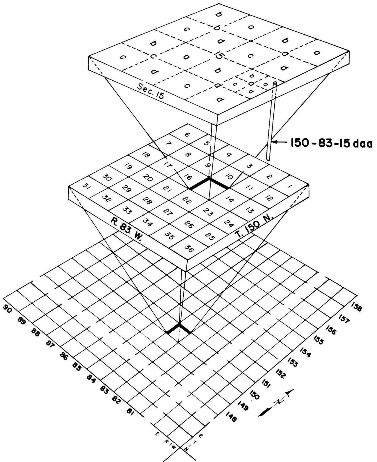
FIGURE 2--SYSTEM OF NUMBERING WELLS AND TEST HOLES.
