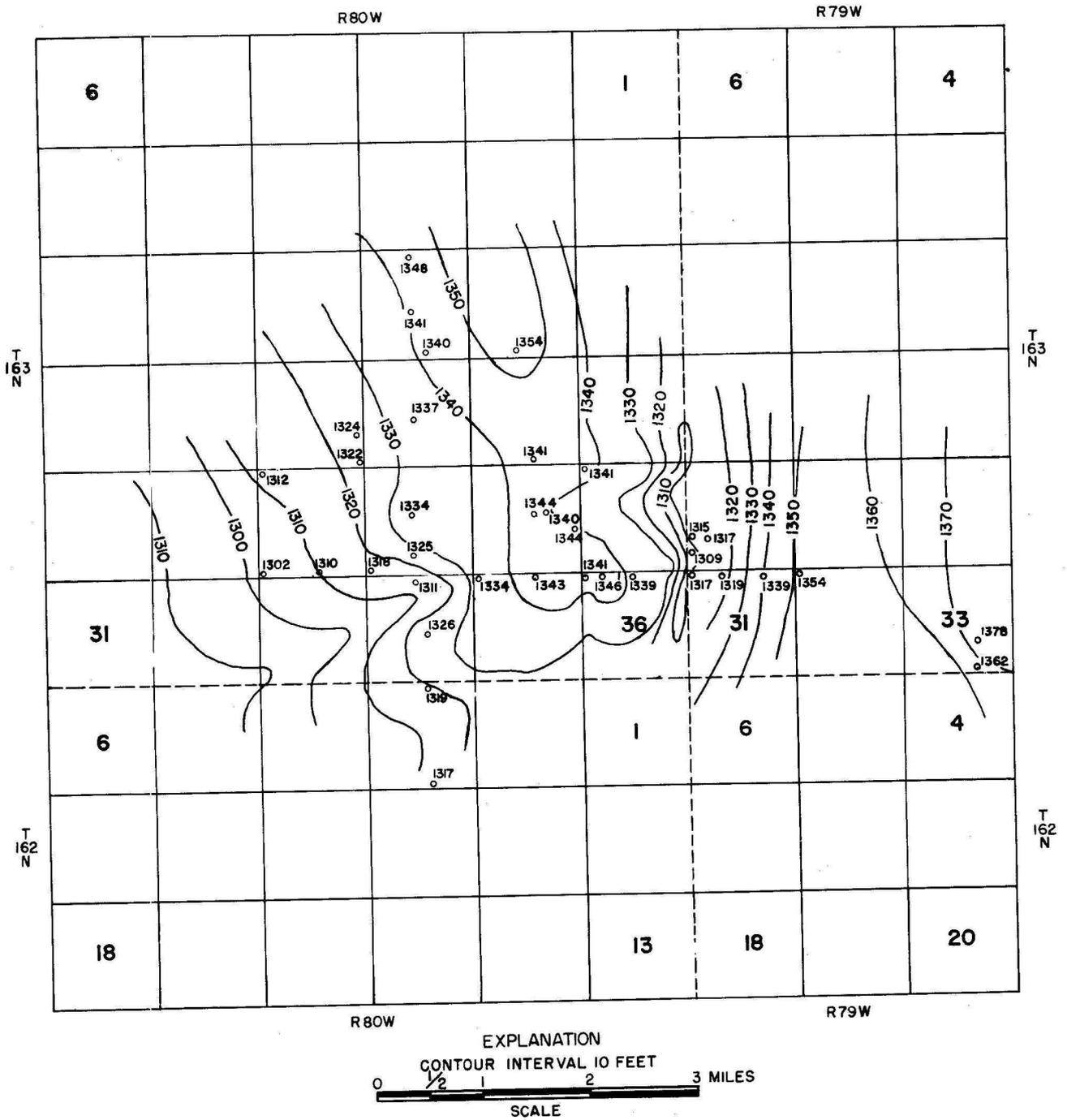
FIGURE 6 — CONTOUR MAP SHOWING APPROXIMATE ALTITUDE OF THE TOP OF THE PIERRE SHALE IN THE WESTHOPE AREA.
