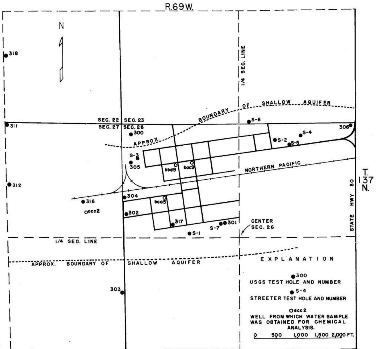
FIGURE 13.—SKETCH MAP OF STREETER SHOWING LOCATIONS OF TEST HOLES AND WELLS SAMPLED FOR CHEMICAL ANALYSIS.
