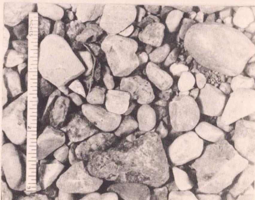
FIGURE 9.— PHOTO - LOG OF OUTWASH DEPOSITS OBTAINED FROM USGS TEST 307 (I36-70-15ddd).
