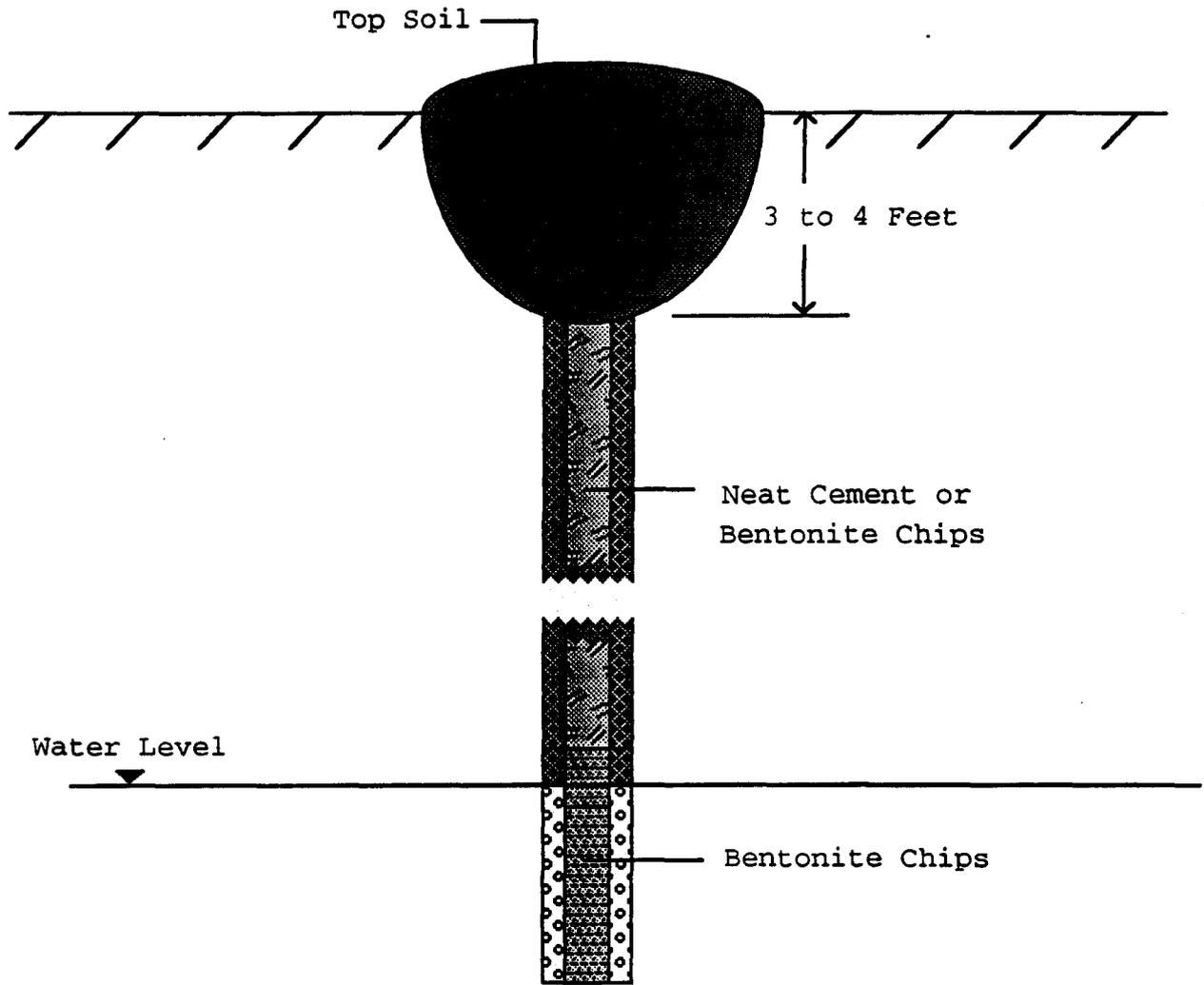
Figure 3. Monitoring well abandonment procedure.
