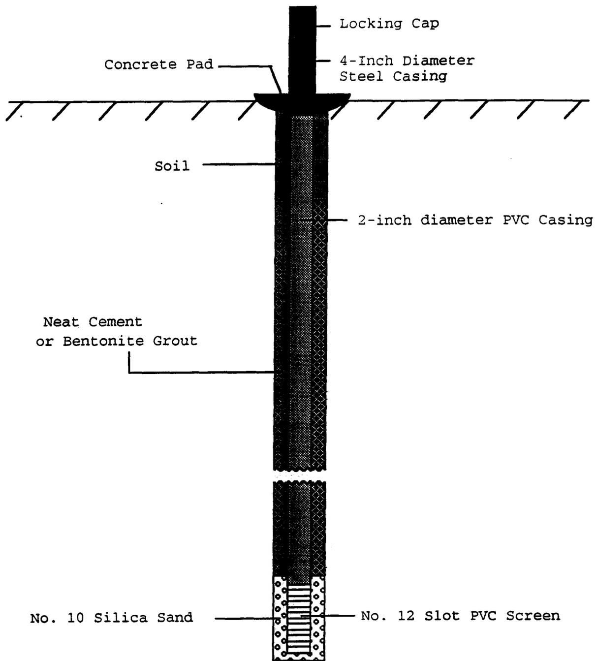
Figure 2. Construction design used for monitoring wells installed at the Valley City landfill.
