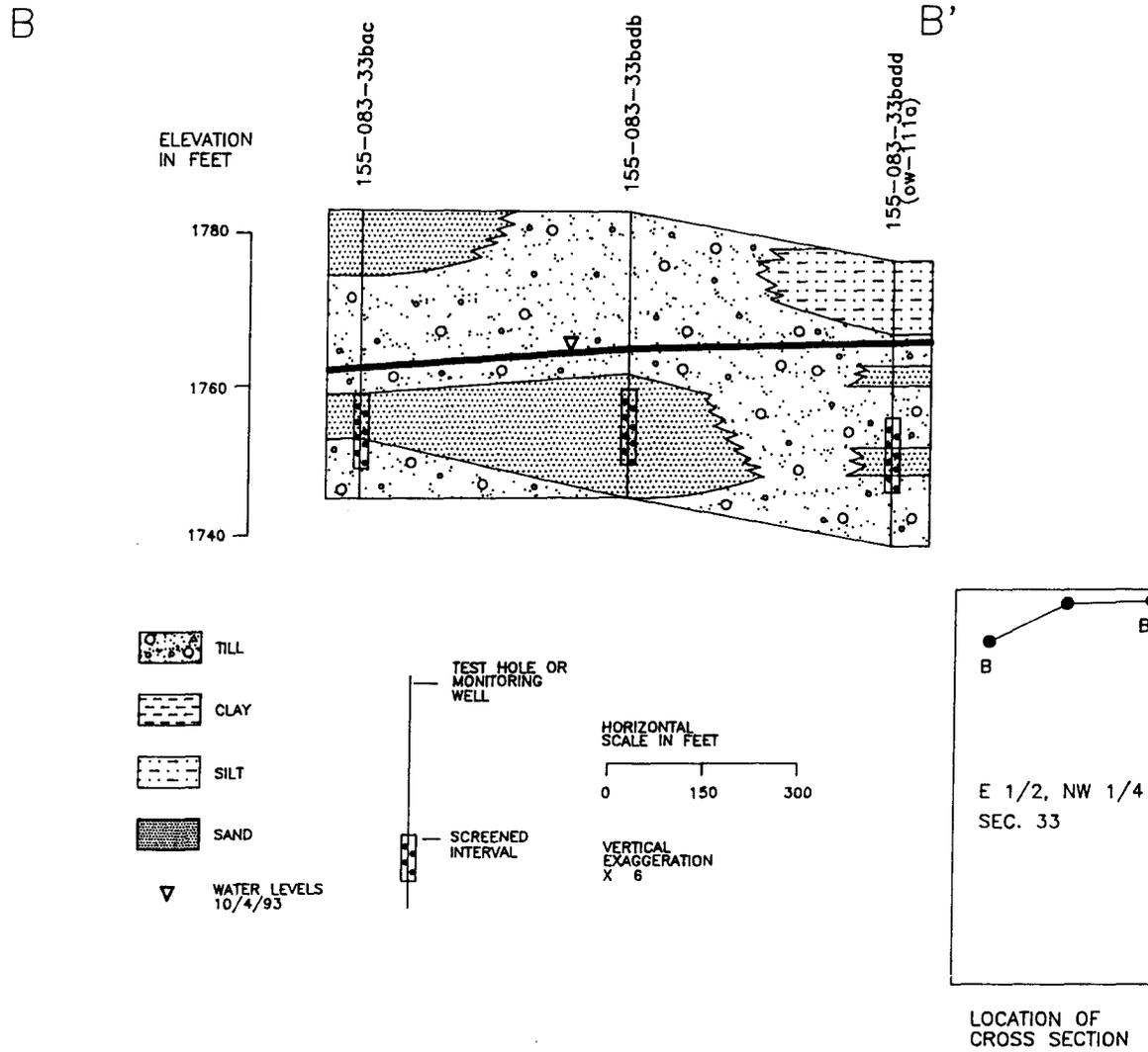
Figure 5. Geohydrologic section B-B' in the Minot landfill.
