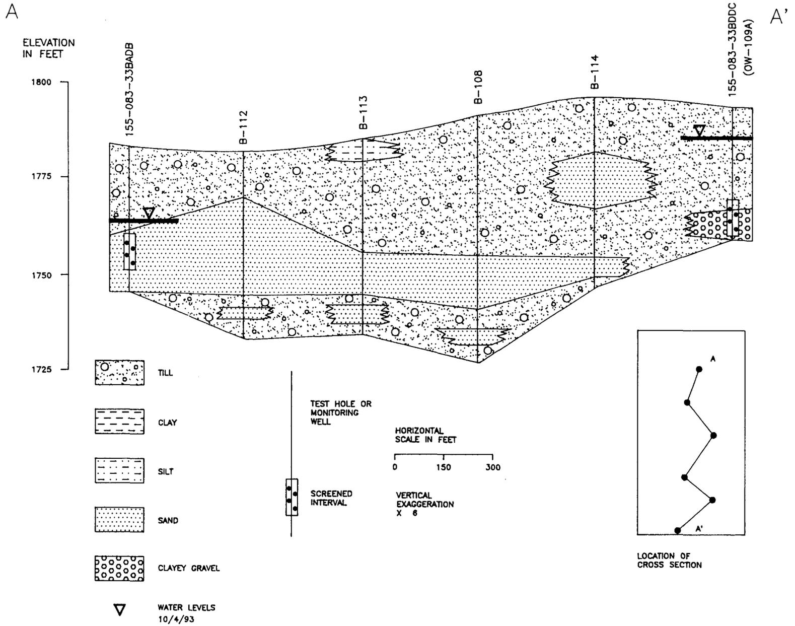
Figure 4. Geohydrologic section A-A' in the Minot landfill.
