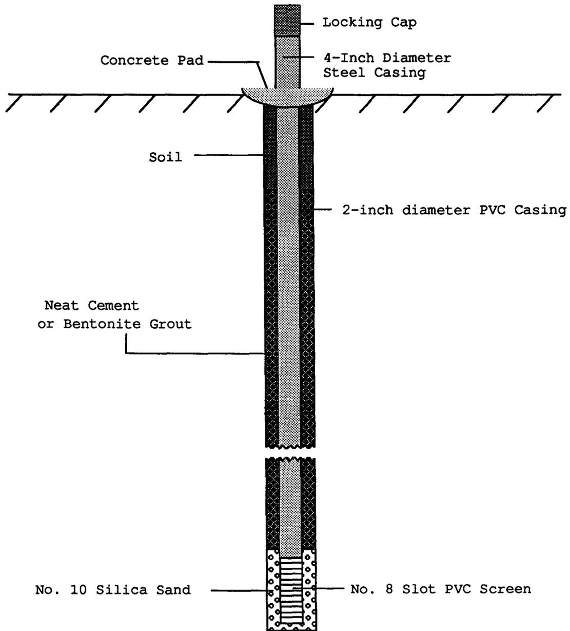
Figure 2. Construction design used for monitoring wells installed at the Minot municipal landfill.
