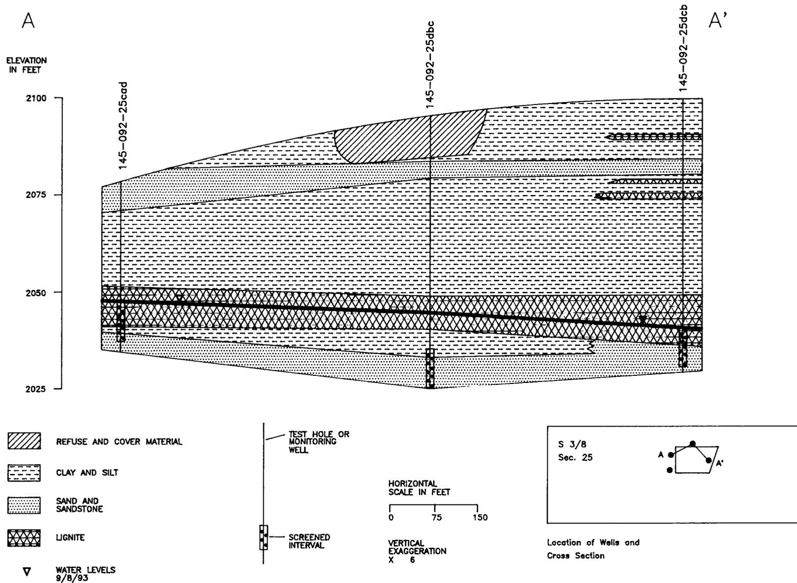
Figure 6. Geohydrologic section A-A' in the Halliday landfill.
