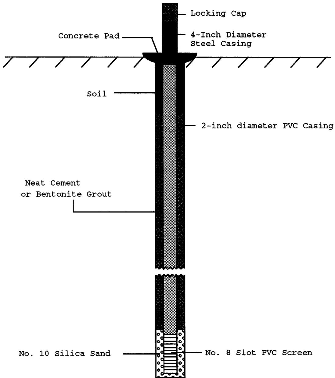
Figure 2. Construction design used for monitoring wells installed at the Halliday landfill.
