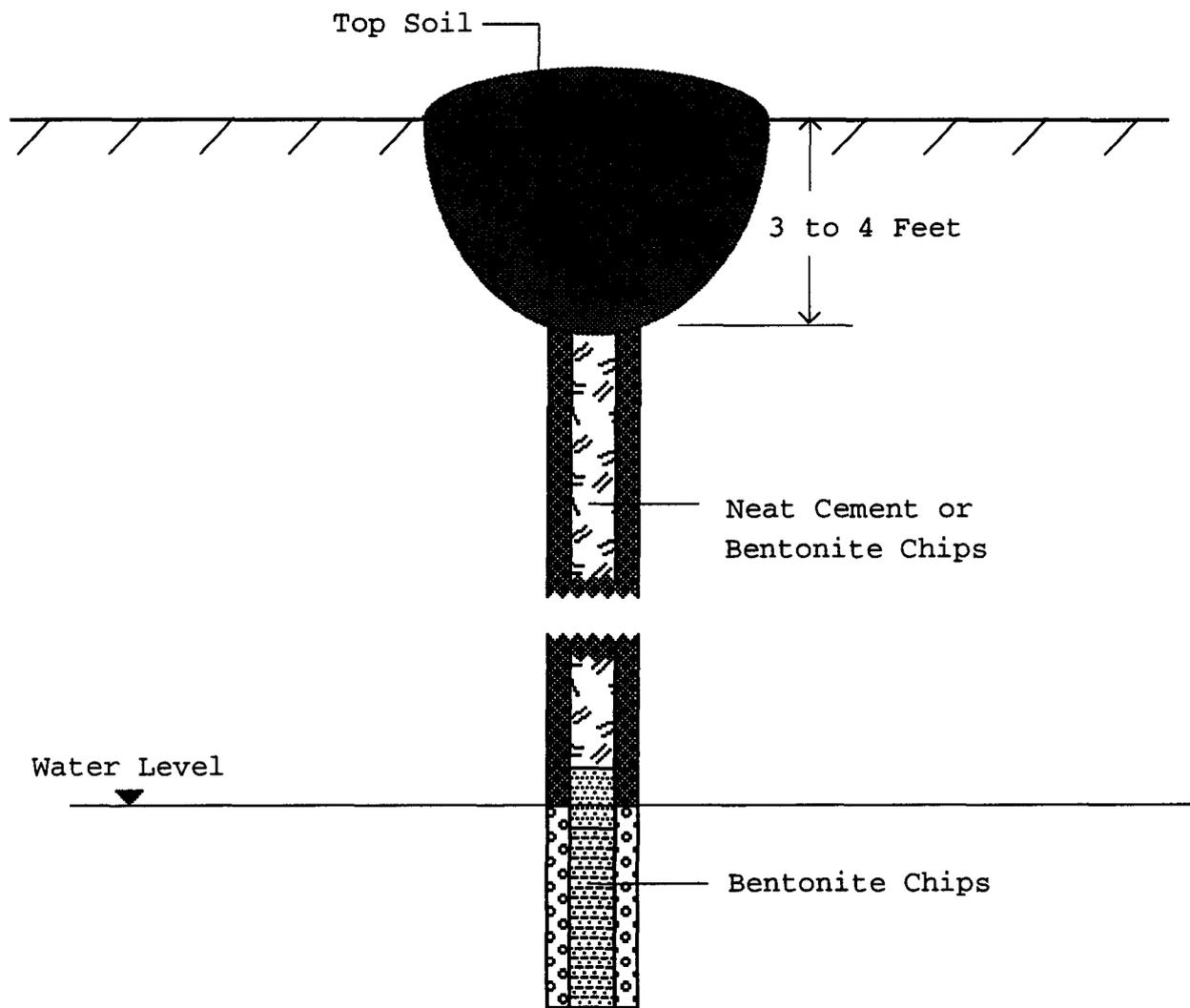
Figure 3. Monitoring well abandonment procedures.
