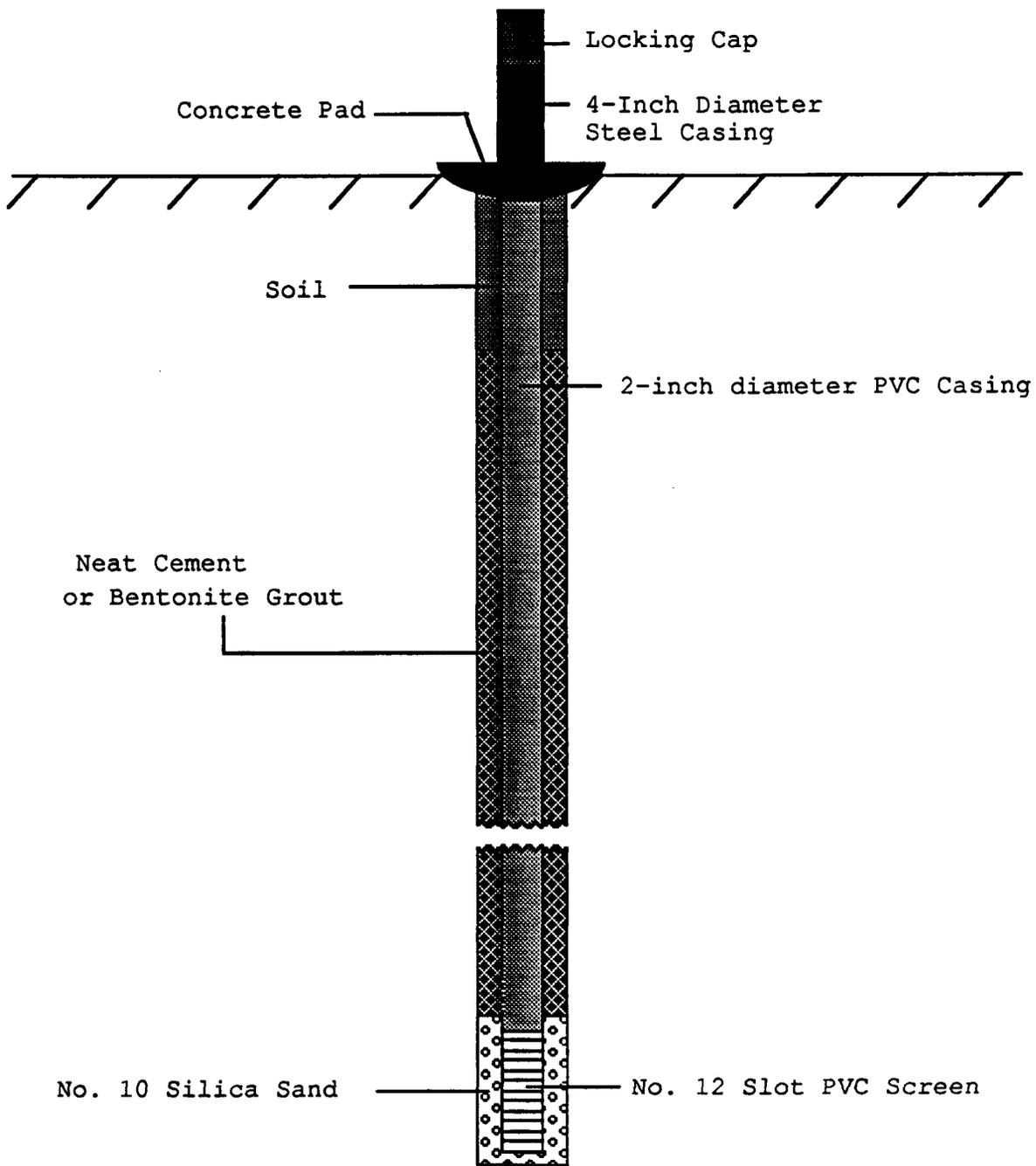
Figure 2. Construction design used for monitoring wells installed at the Glen Ullin landfill.
