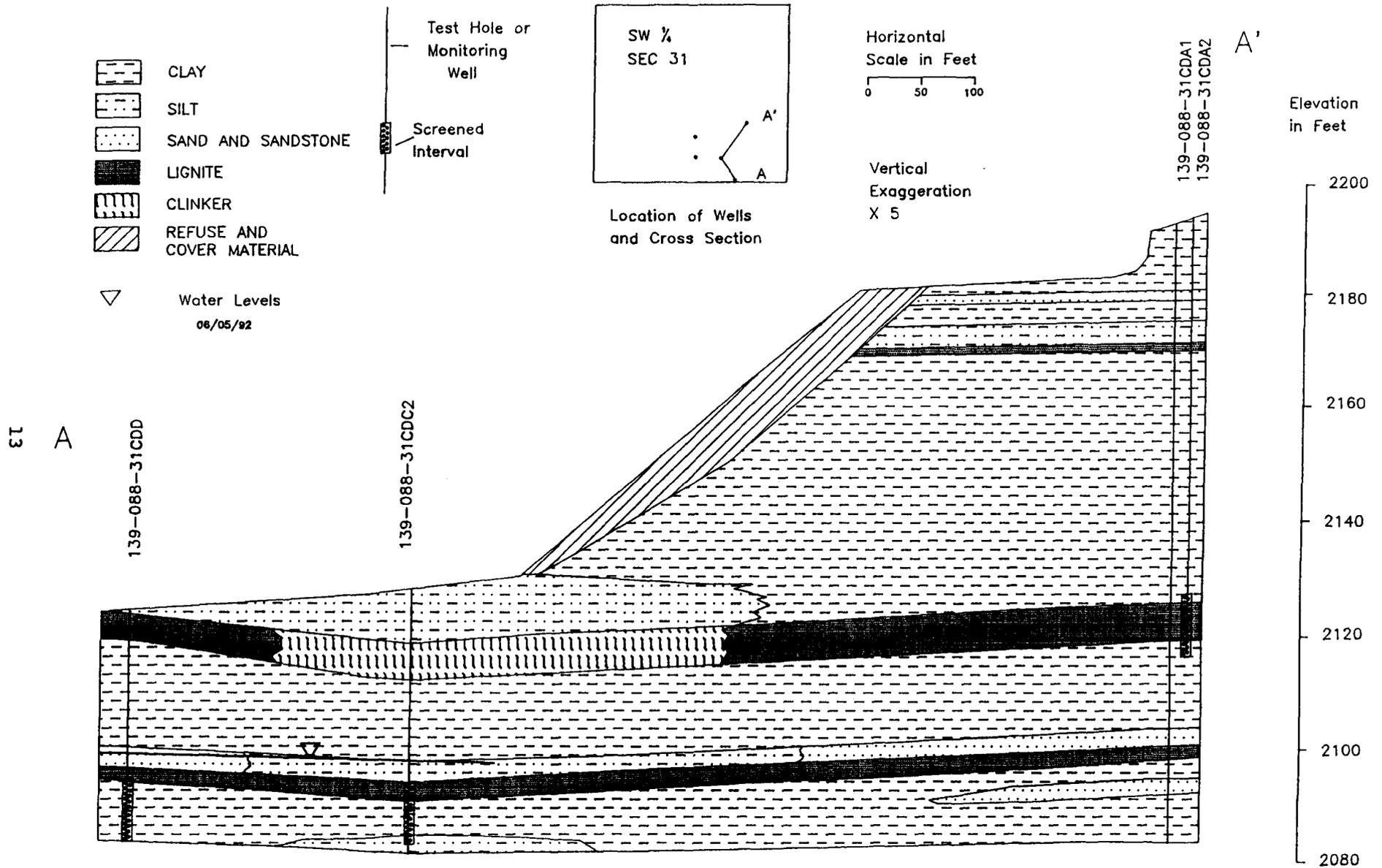
Figure 5. Geohydrologic section A-A' in the Glen Ullin landfill
