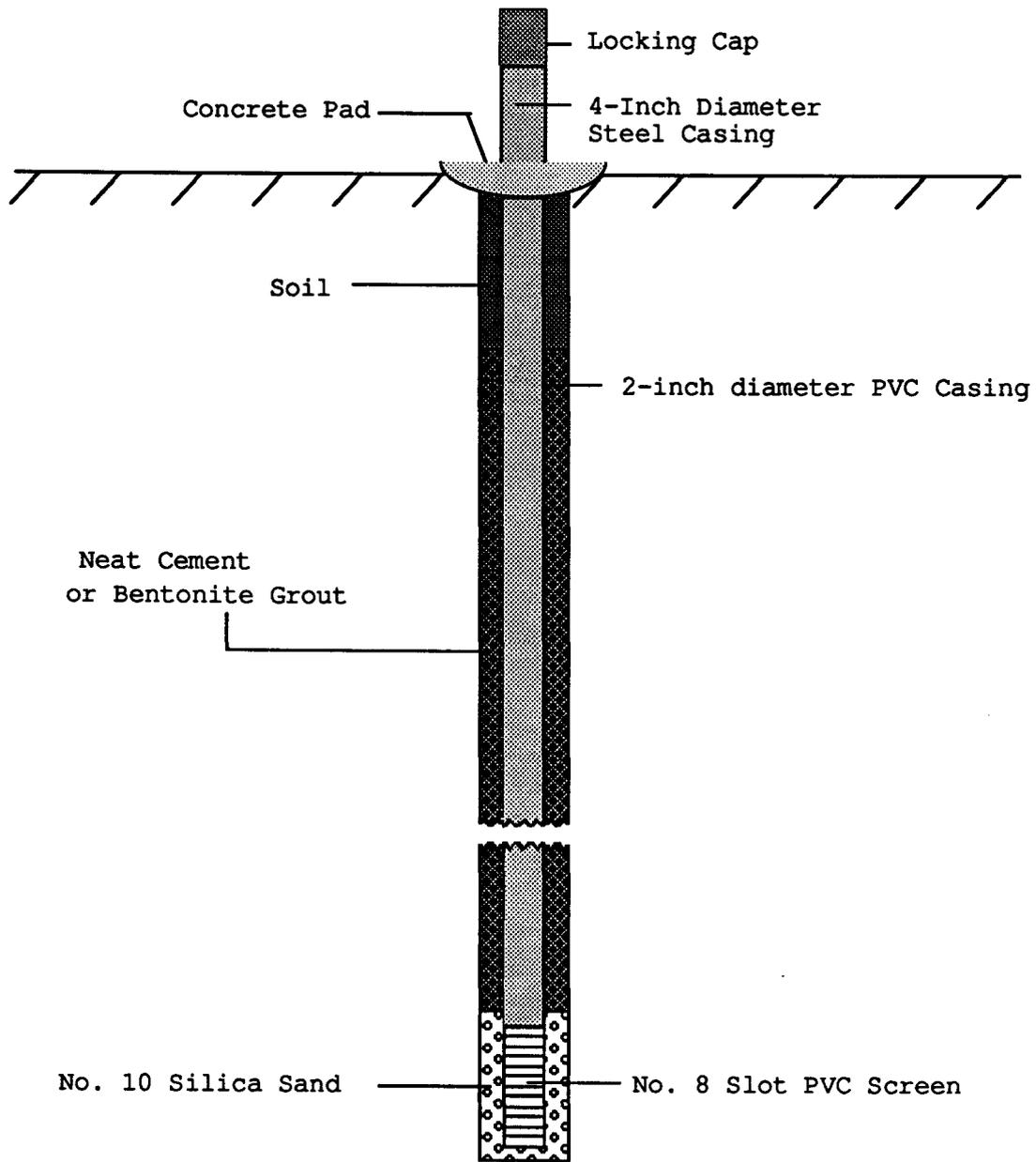
Figure 2. Construction design used for monitoring wells installed at the Dickinson landfill.
