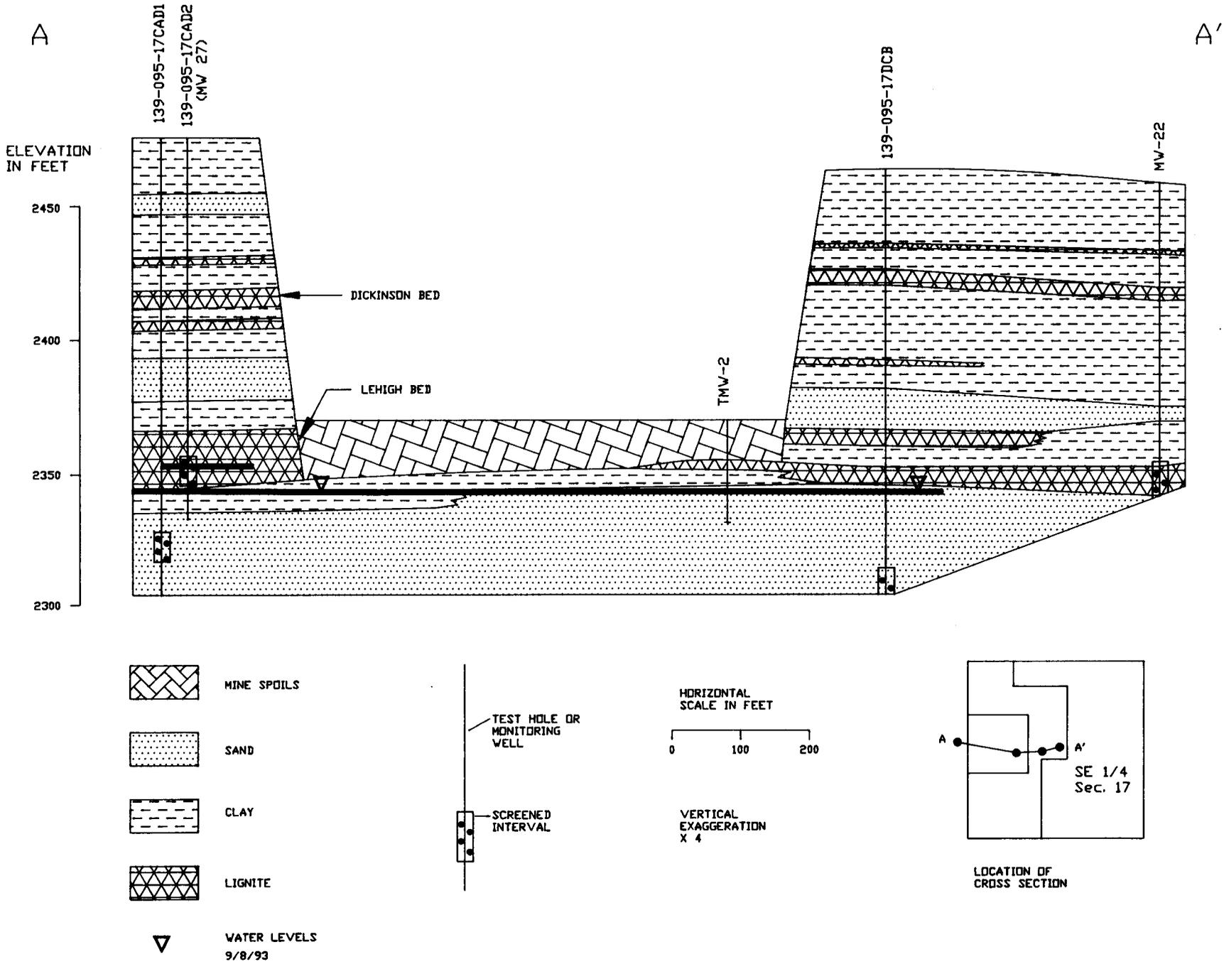
Figure 5. Geohydrologic section A-A' in the Dickinson landfill.
