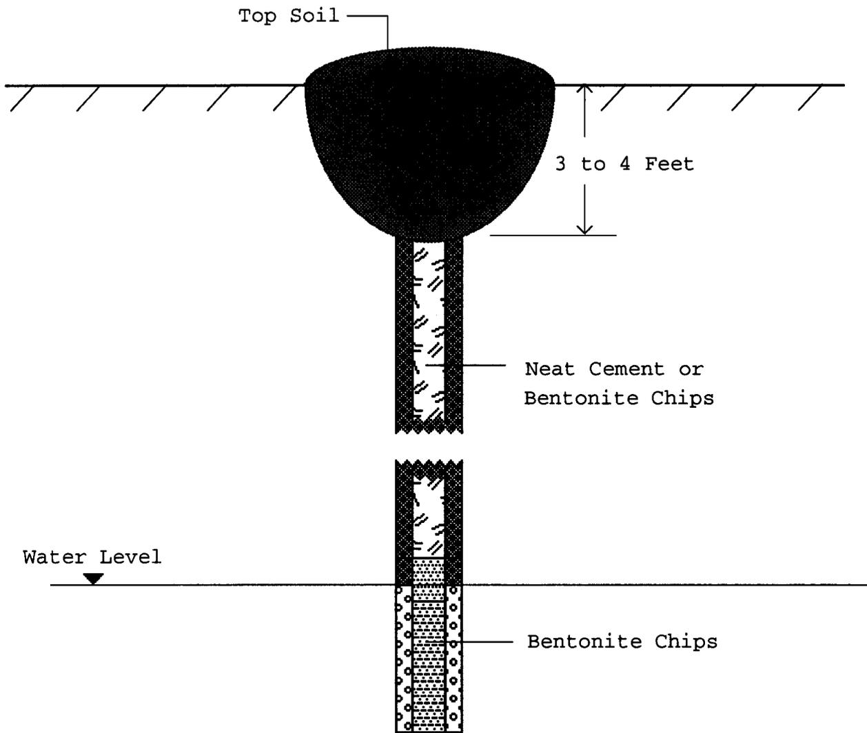
Figure 3. Monitoring well abandonment procedures.
