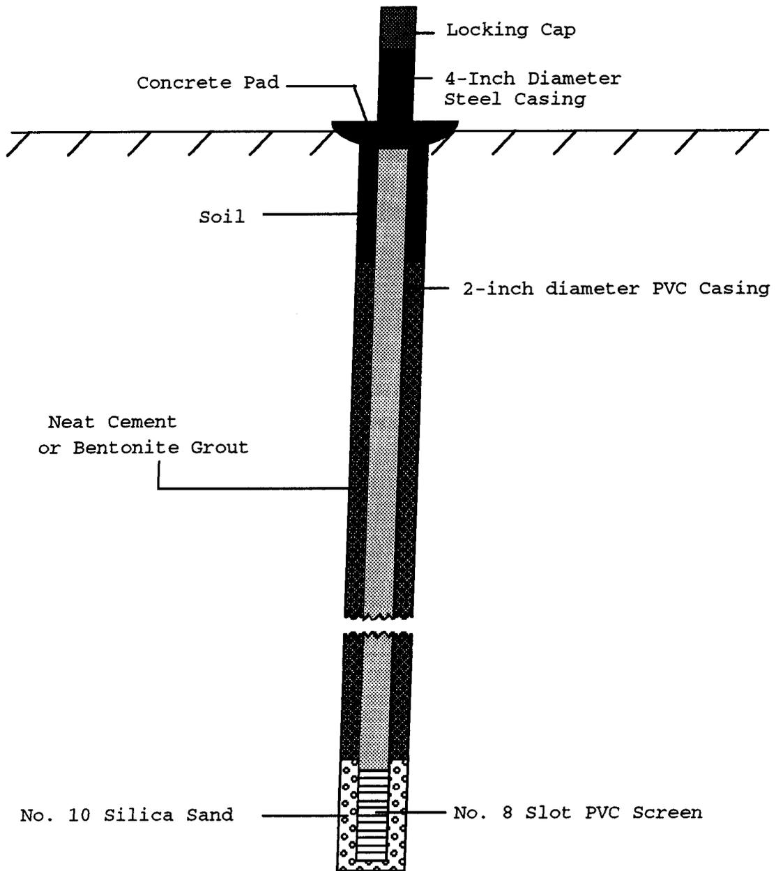
Figure 2. Construction design used for monitoring wells installed at the Alsen landfill.
