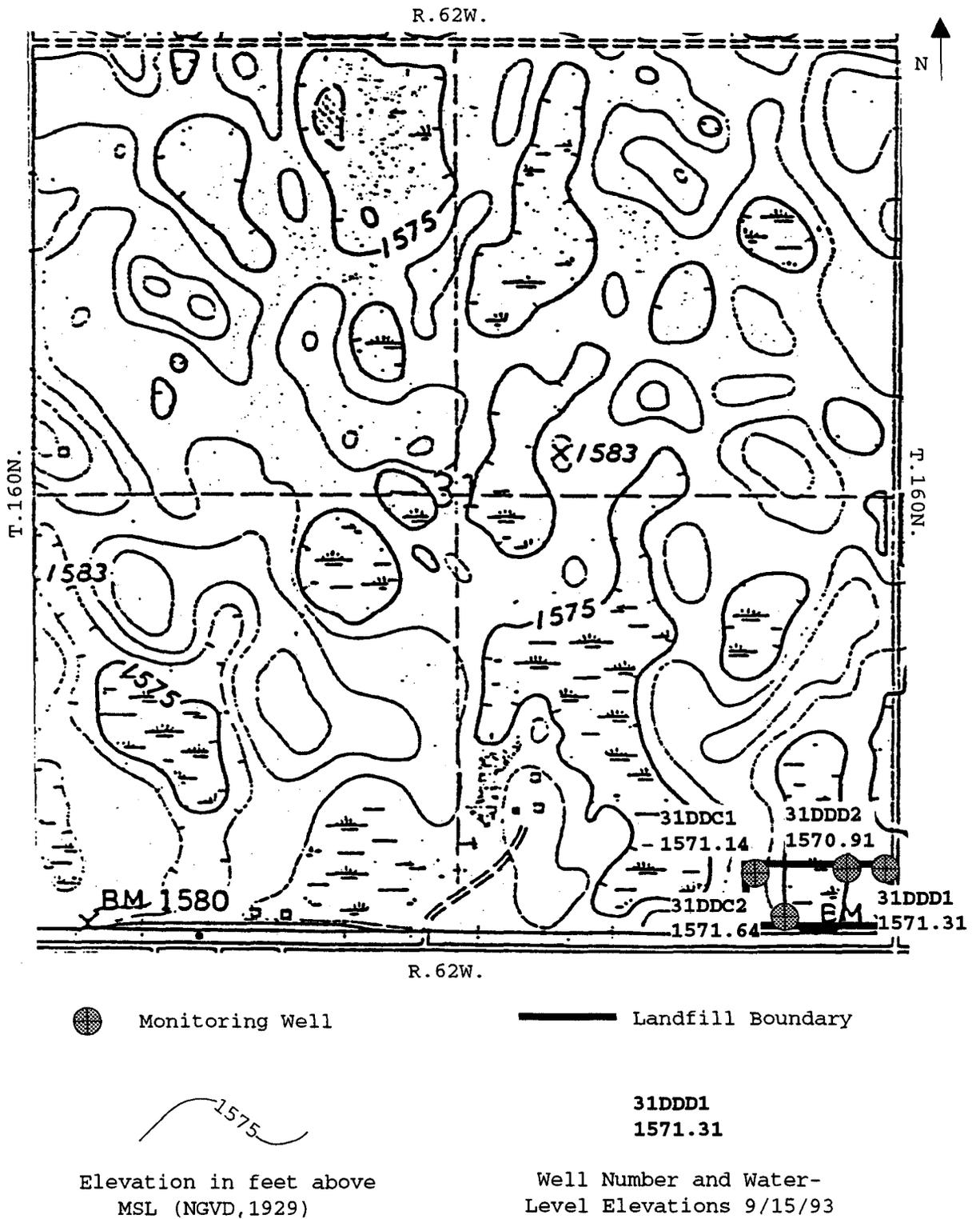
Figure 6. Location of monitoring wells at the Alsen landfill.
