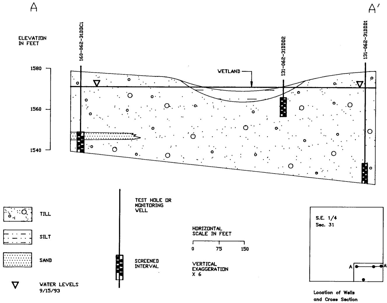
Figure 5. Geohydrologic section A-A' in the Alsen Landfill.
