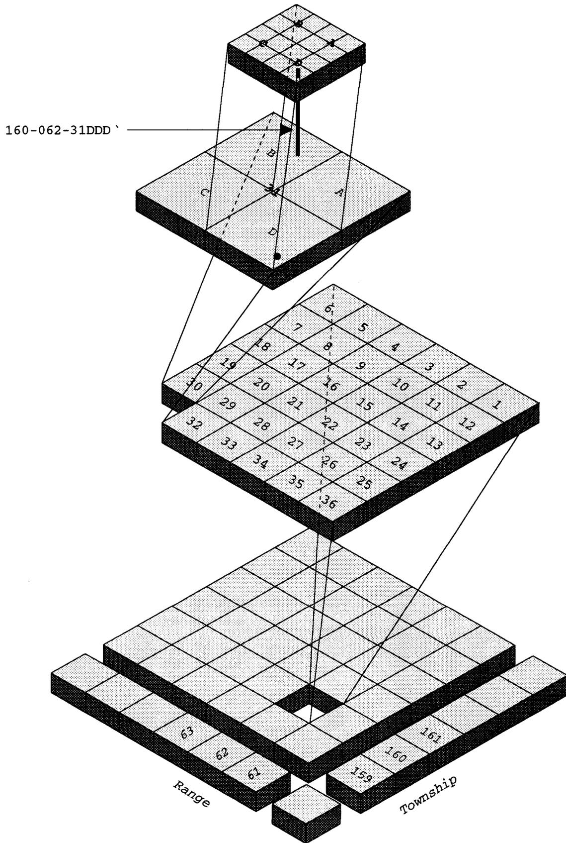
Figure 4. Location-numbering system for the Alsen landfill.
