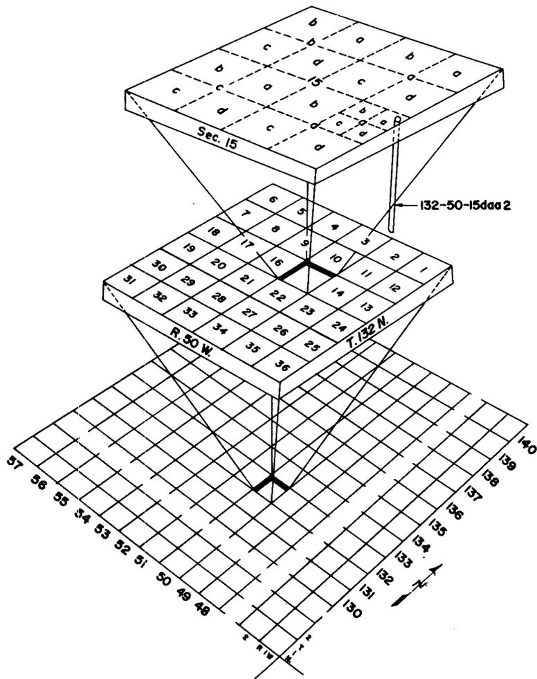
**Figure 2.** System of numbering test holes and wells.
