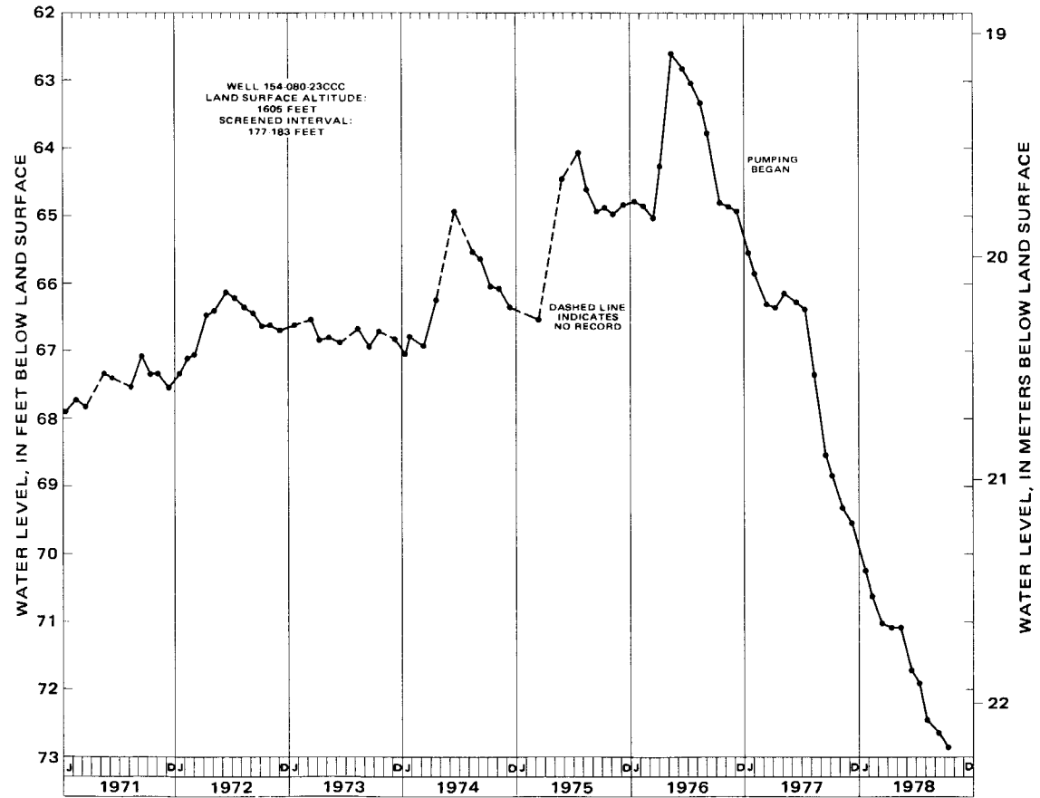
FIGURE 11.—Water-level fluctuations in the western part of the New Rockford aquifer system affected by pumping of the Minot well field.
