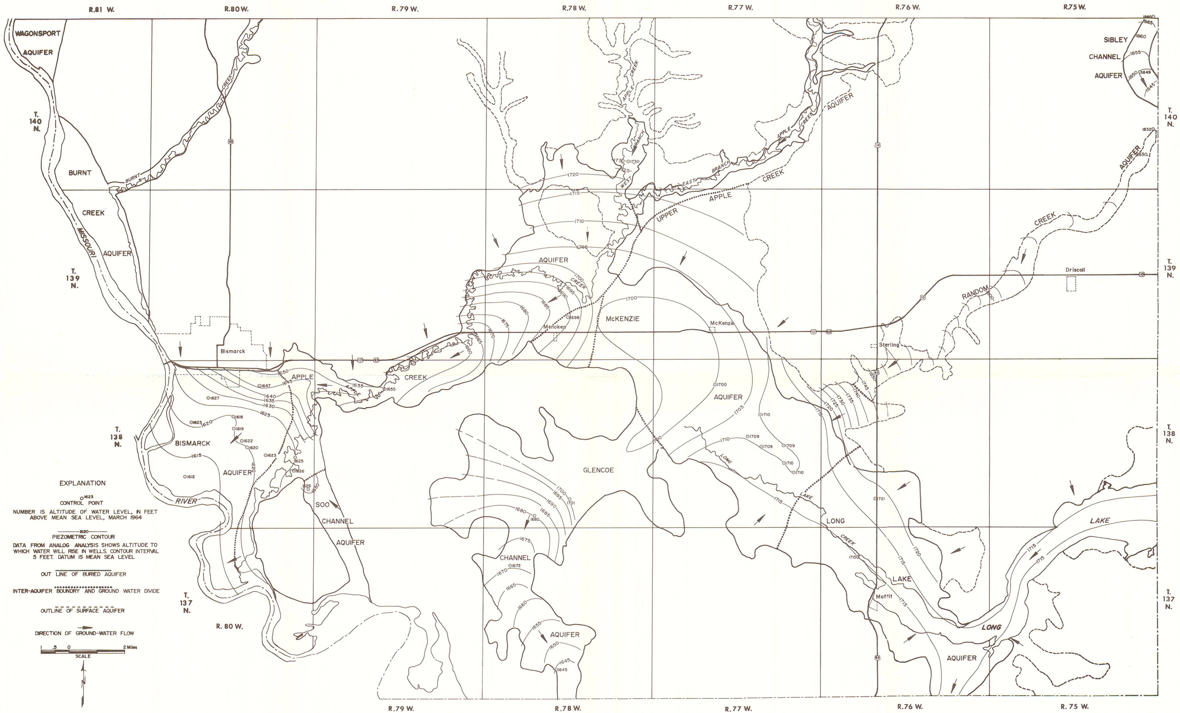
FIGURE 13. Map showing configuration of piezometric surface and direction of ground-water movement in melt-water channel aquifers in southern Burleigh County.
