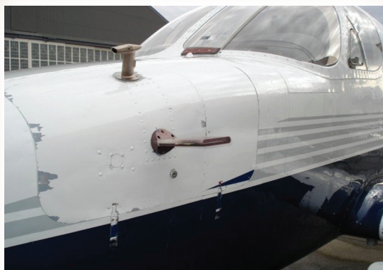
Temperature Sensor (top) and Liquid Water Probe.
