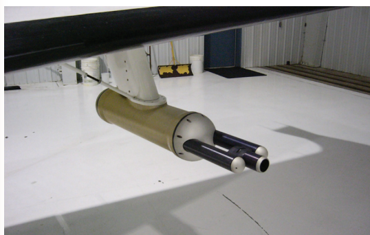
Forward Scattering Spectrometer Probe (FSSP) measures cloud droplets.
